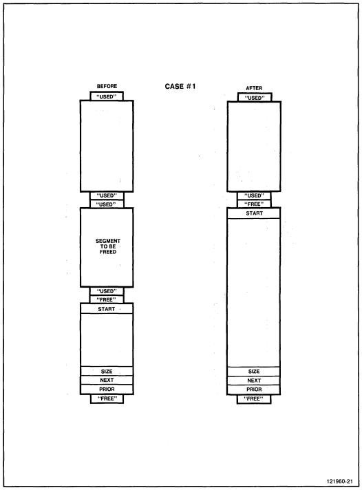
Figure 3-8. Possibilities for Combining Segments (Cont'd.)
