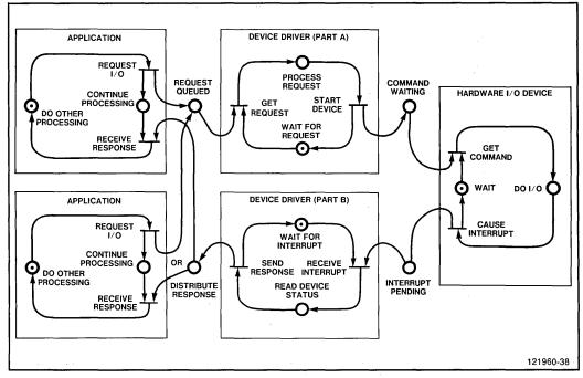
Figure 8-3. Synchronization with Two-Part Device Driver
