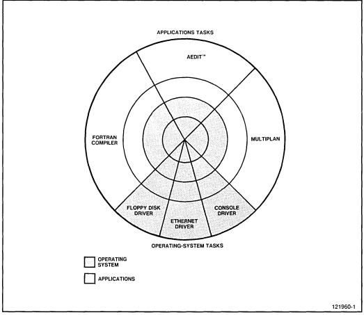
Figure 1-7. Independent Operating-System Tasks
