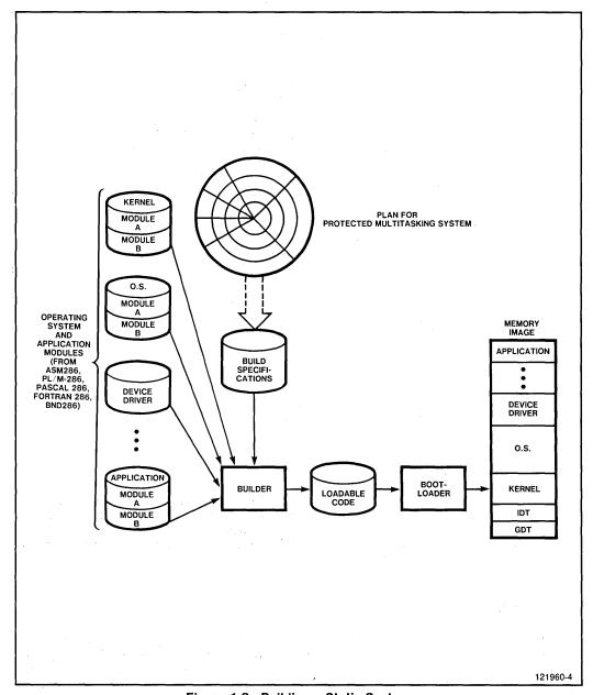
Figure 1-8. Building a Static System
