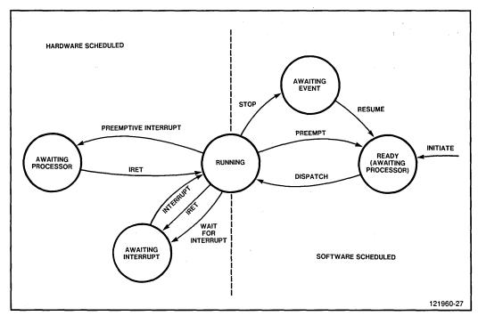
Figure 4-3. Expanded Scheduling State Transition Diagram
