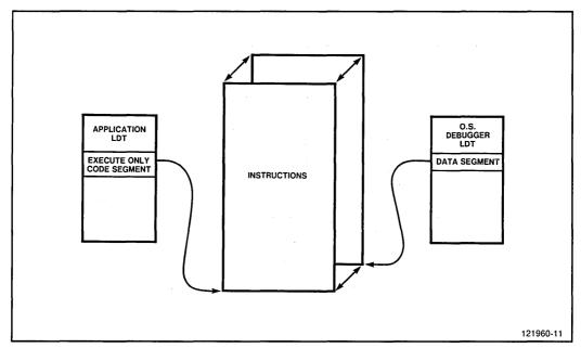
Figure 2-11. Aliasing for Debugger
