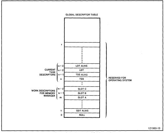
Figure 3-6. Example GDT Layout
