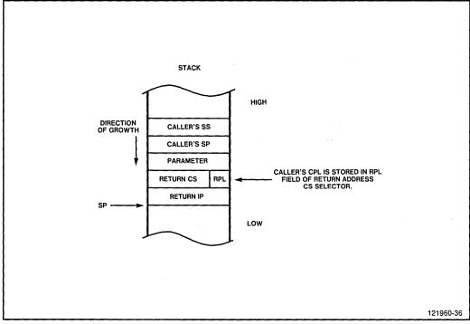
Figure 6-3. Interrupt Procedure's Stack
