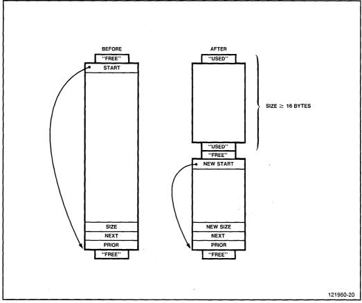
Figure 3-7. Splitting an Available Block of Memory
