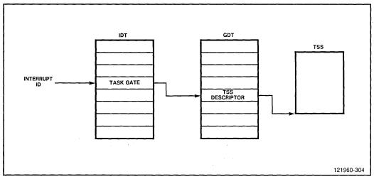
Figure 6-1. Interrupt Vectoring for Tasks
