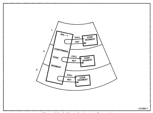
Figure 2-5. Calling a Conforming Segment
