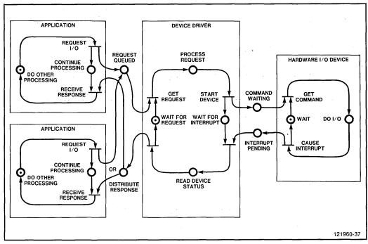
Figure 8-2. Synchronization with Simple Device Driver
