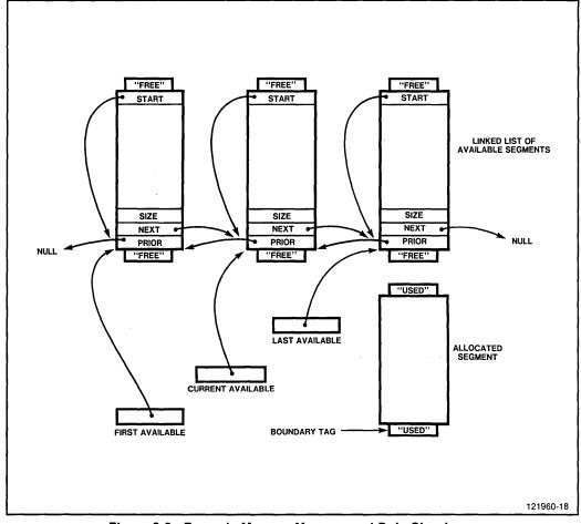
Figure 3-3. Example Memory-Management Data Structures
