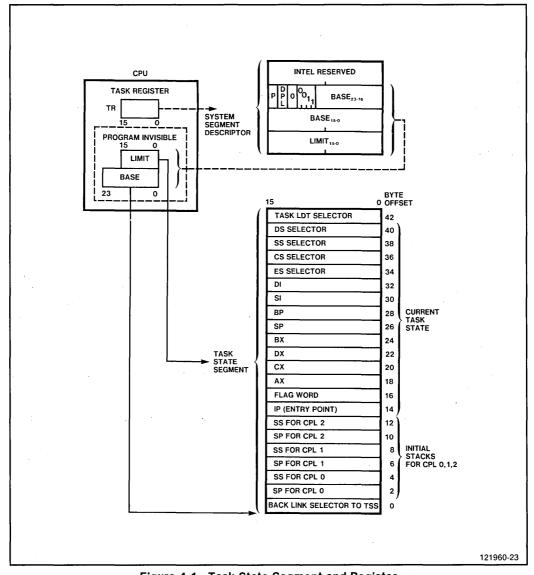
Figure 4-1. Task State Segment and Register
