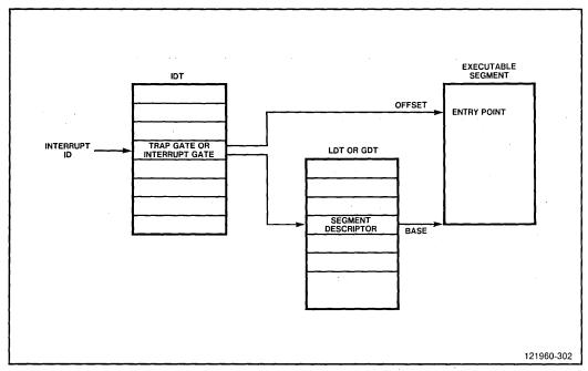
Figure 6-2. Interrupt Vectoring for Procedures
