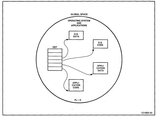
Figure 1-6. A One-Level Unprotected Structure
