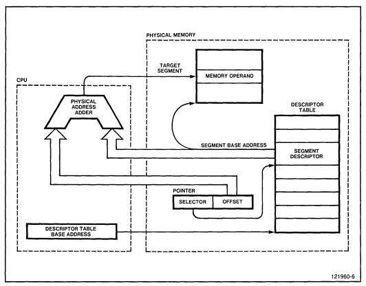
Figure 2-1. Abstraction of Addressing Mechanism
