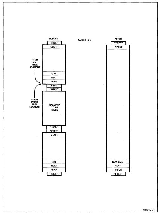
Figure 3-8. Possibilities for Combining Segments
