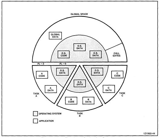
Figure 1-5. A Two-Level Protection Structure
