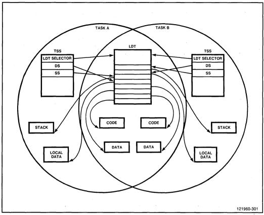
Figure 5-1. Segment Sharing via Common LDT
