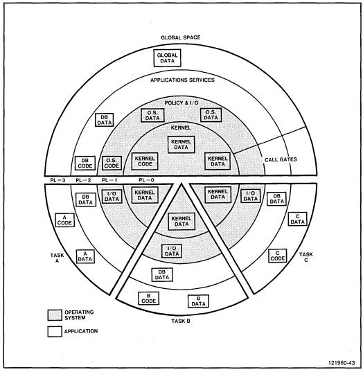
Figure 1-4. A Four-Level Protection Structure
