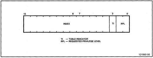
Figure 2-10. Format of a Selector
