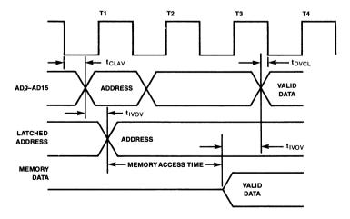
Figure 1B. 186 System Memory Timing Diagram
