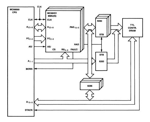
Figure 3. MC68000 with MC68451 Configuration
