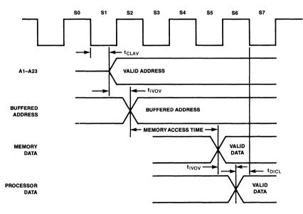
Figure 2B. 68000 System Memory Timing Diagram
