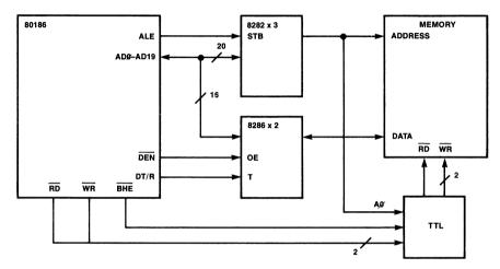
Figure 1A. Typical Simple 80186 System
