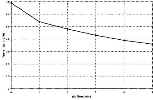
48/56 Pin Cerpack Theta JA vs. Airflow
