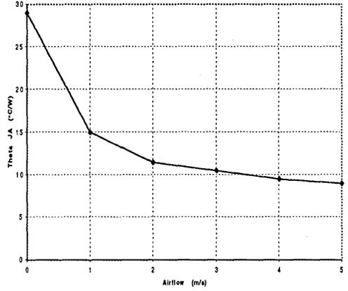
447 Pin PGA Theta JA vs. Airflow
