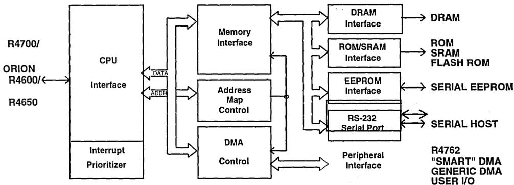
FIGURE 1: 4761 BLOCK DIAGRAM
