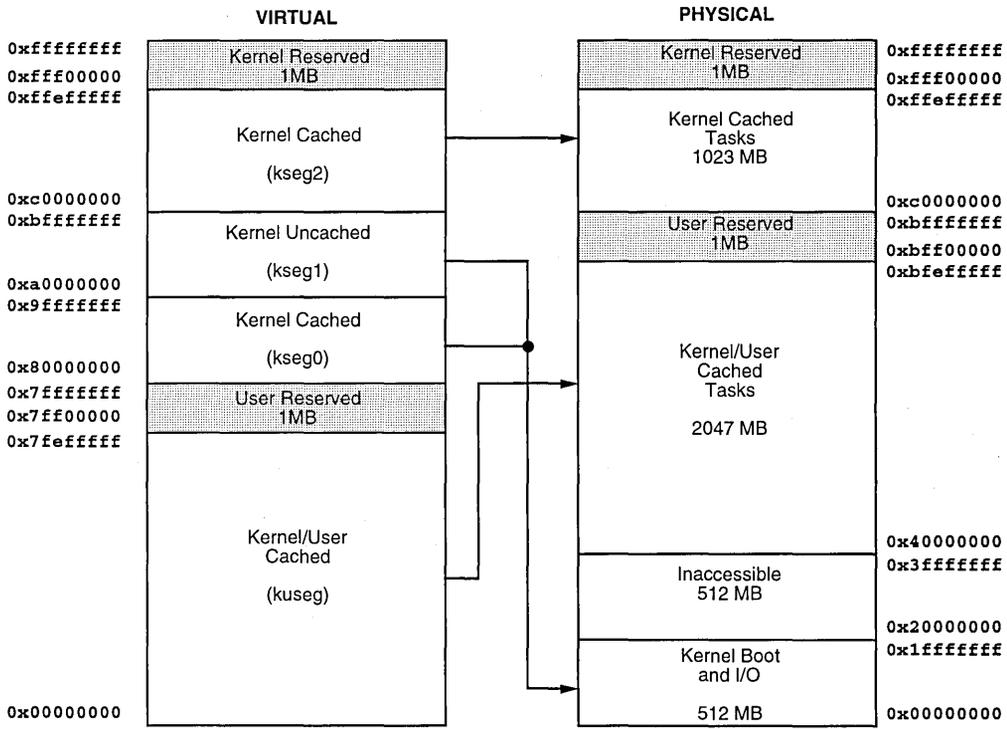
Figure 3. Virtual to Physical Mapping of Base Architecture Versions
