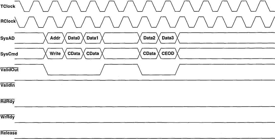
Figure 7: Processor Block Write
