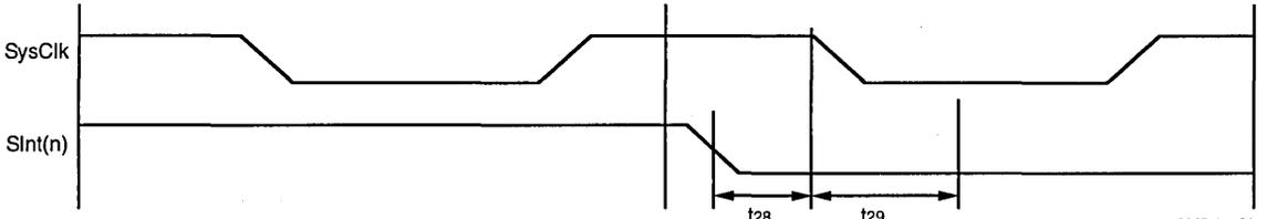
Figure 17. Synchronized Interrupt Input Timing
