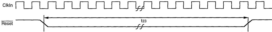
Figure 10(b). Warm Reset Sequence (Internal Pull-Ups Used)
