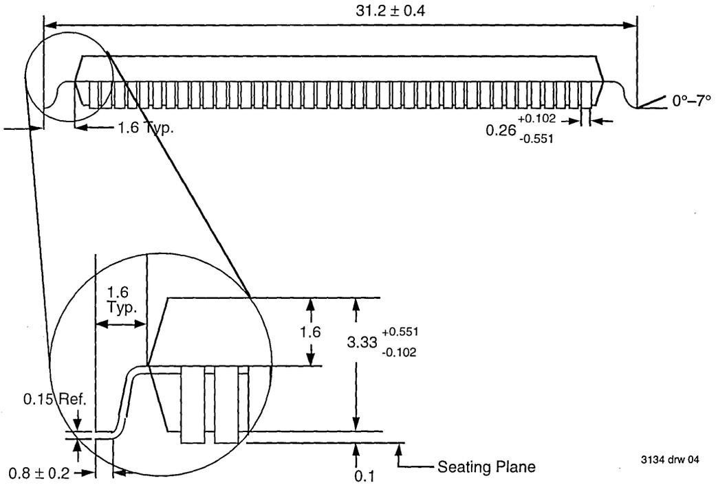
Figure 10.2 Expanded View of Figure 10.1 Detail
