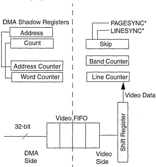
Figure 5.3 Video Block Diagram
