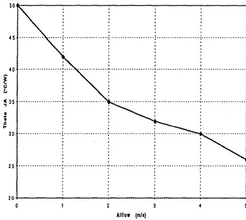
32 Pin PLCC vs. Airflow
