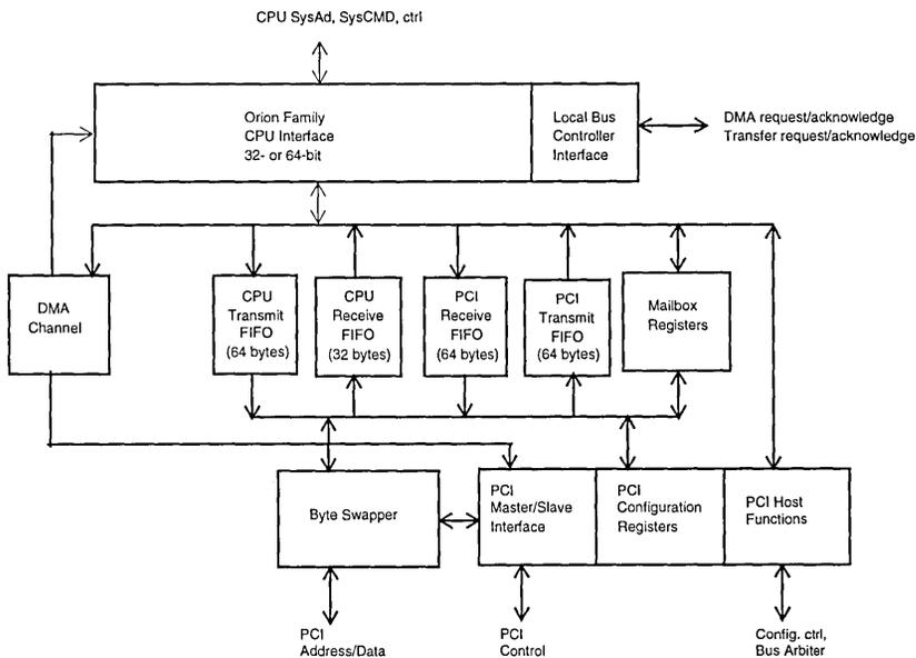
FIGURE 1: R4762 BLOCK DIAGRAM
