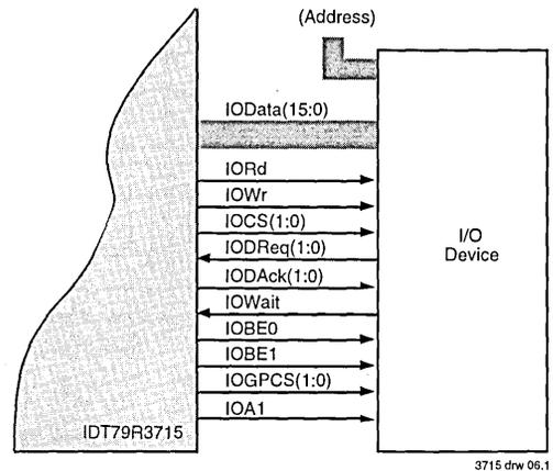
Figure 2.5 General Purpose I/O Device Interface
