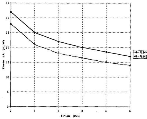
208 Pin PQFP vs. Airflow
