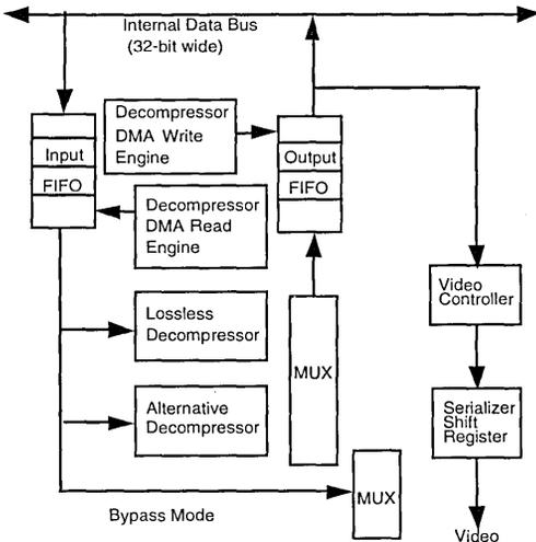
Figure 2.13.a: Decompressor Block Diagram
