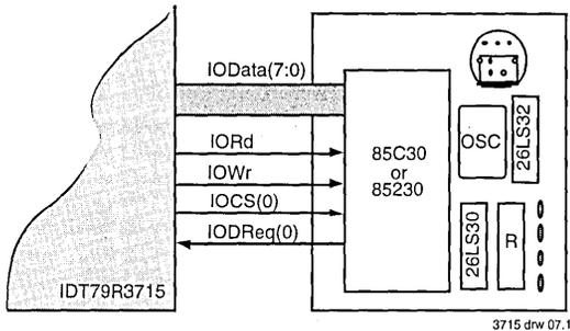
Figure 2.4 DMA-Supported AppleTalk I/O Port
