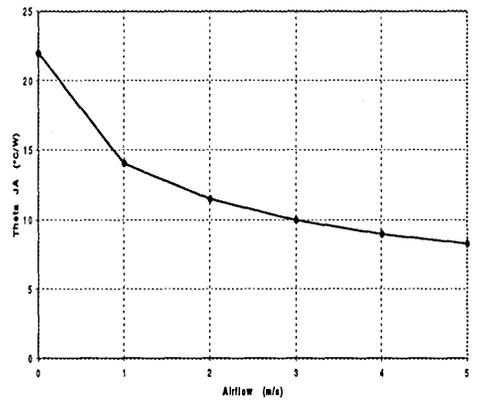
28 Pin Plastic Dip Theta JA vs. Airflow
