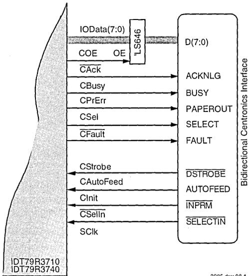
Figure 2.11: IEEE P1284 Bidirectional Centronics I/O Port
