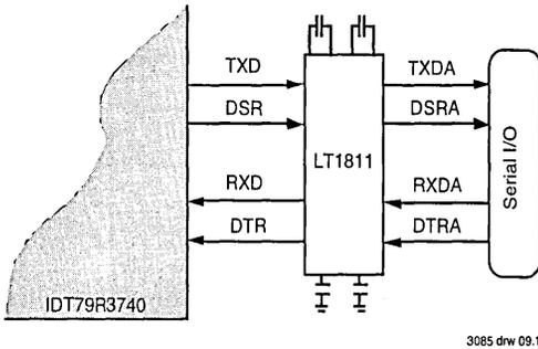
Figure 2.14: UART Serial Interface Implementation
