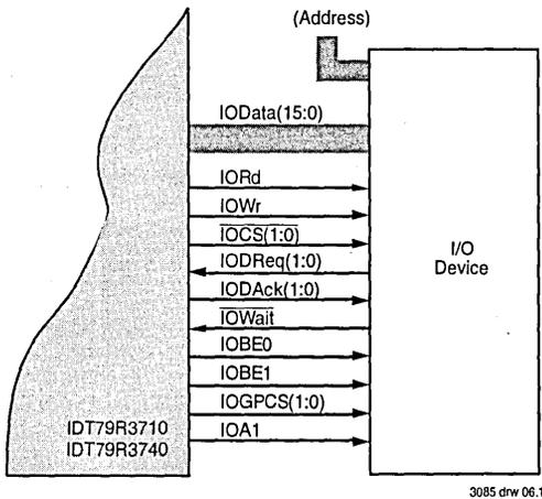
Figure 2.10: General Purpose I/O Device Interface
