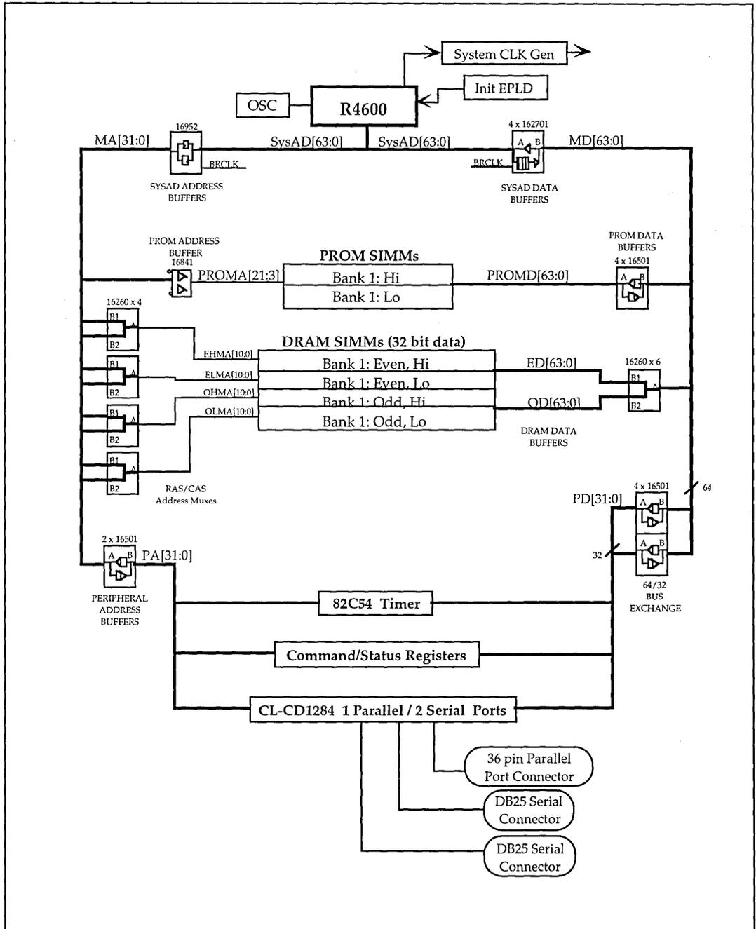
Figure 1 79S464 R4600 Evaluation Board Block Diagram
