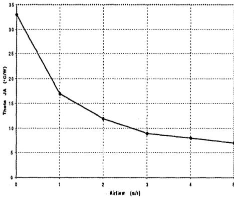
144 Pin PGA Theta JA vs. Airflow
