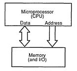
Figure 9. A Simple Microprocessor Memory System
