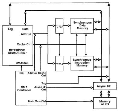
Figure 9. IDT79R3001 DMA Interface
