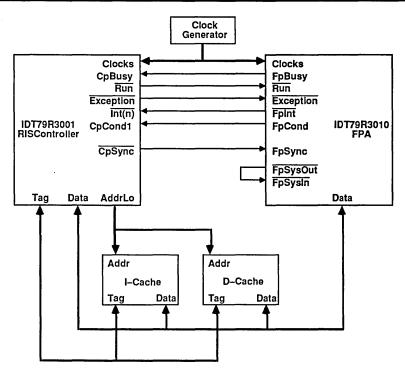
Figure 8. IDT79R3001 Interface to IDT79R3010 Floating Point Co-Processor
