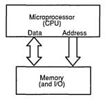
Figure 9. A Simple Microprocessor Memory System
