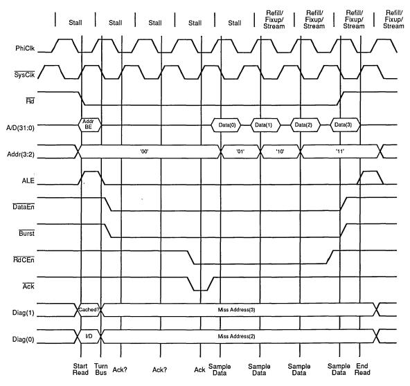
Figure 7. IDT R3051 Family Burst Read Operation (Two Bus Wait Cycles)
