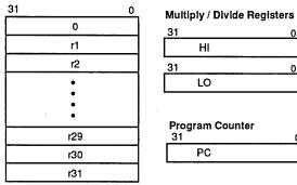
Figure 2. IDT79R3000 CPU Registers
