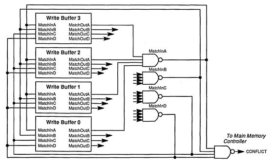
Figure 7. Write Buffer MatchOut/Matchin Logic
