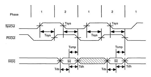
Figure 18. Interrupt Timing
