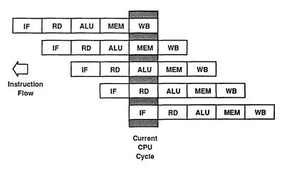
Figure 3. Instruction Execution in IDT79R3001 Pipeline
