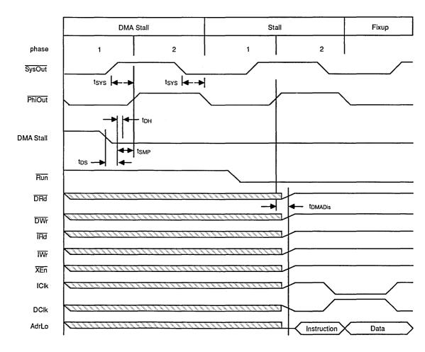
Figure 24. Entering DMA Stall
