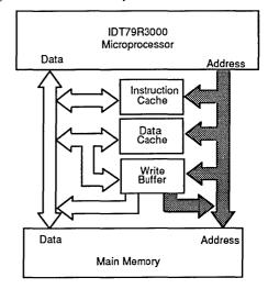
Figure 10. An IDT79R3000 System with a High-Performance Memory System
