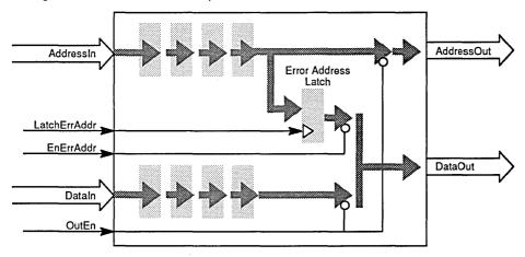
Figure 8. The Write Buffer Error Address Latch
