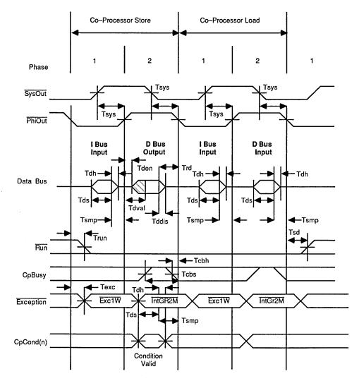
Figure 17. Co-Processor Load/Store Timing
