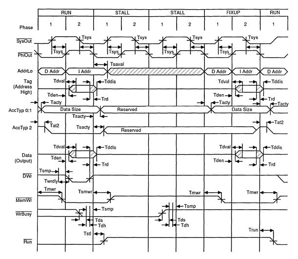
Figure 15. Memory Write Timing
