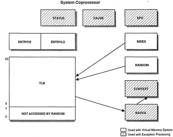
Figure 4. The System Coprocessor Registers
