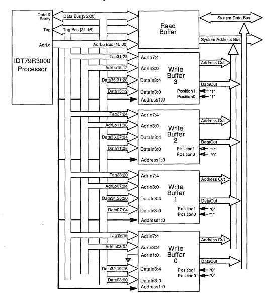
Figure 3. Write Buffer Data and Address Line Connections
