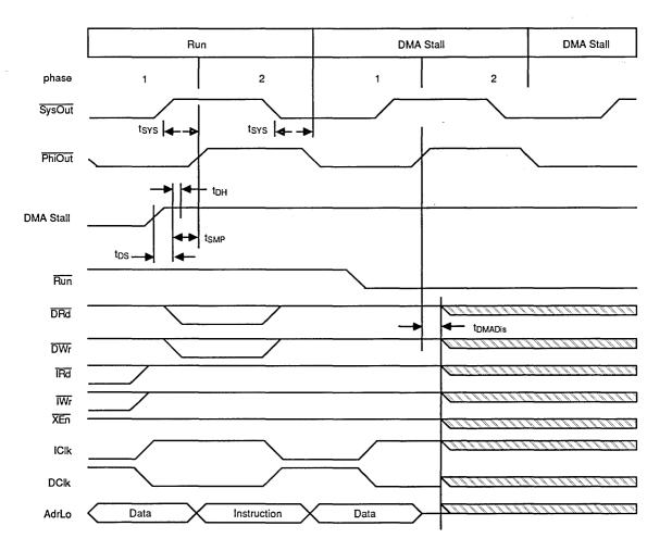
Figure 25. Completing DMA Stall
