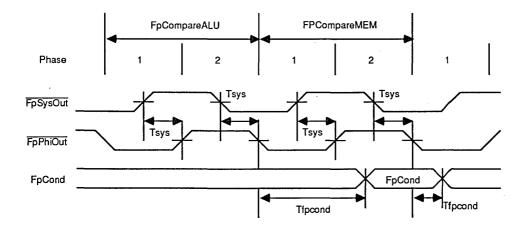
Figure 11. Floating Point Condition Timing
