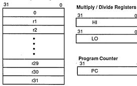
Figure 2. IDT79R3000A CPU Registers
