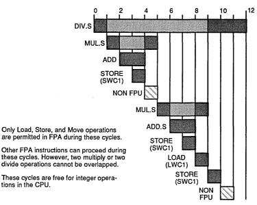
Figure 3. Examples of Overlapping Floating Point Operation
