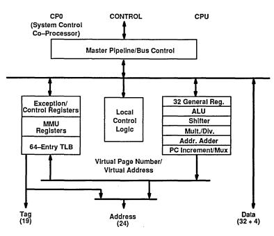
Figure 1. IDT79R3001 Block Diagram
