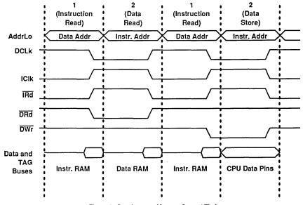
Figure 4. Synchronous Memory Control Timing
