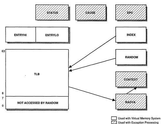
Figure 4. The System Coprocessor Registers
