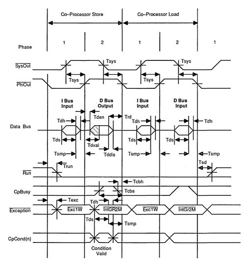
Figure 17. Co-Processor Load/Store Timing
