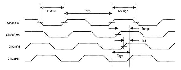
Figure 6. Input "2x" Clock Timing
