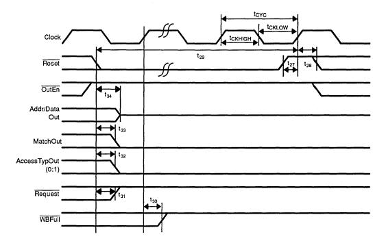
Figure 14. Reset Timing
