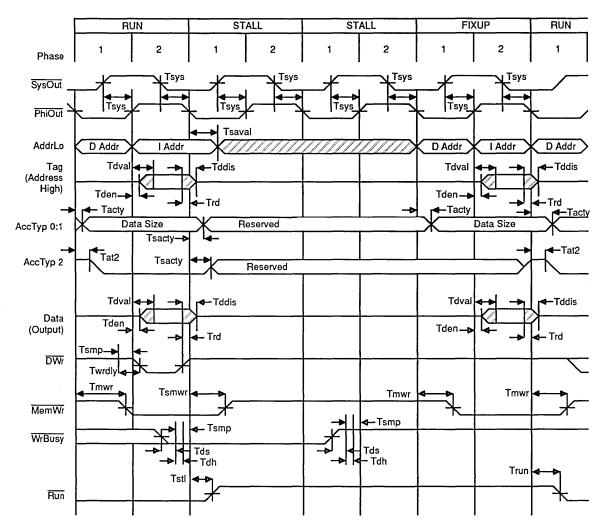
Figure 15. Memory Write Timing
