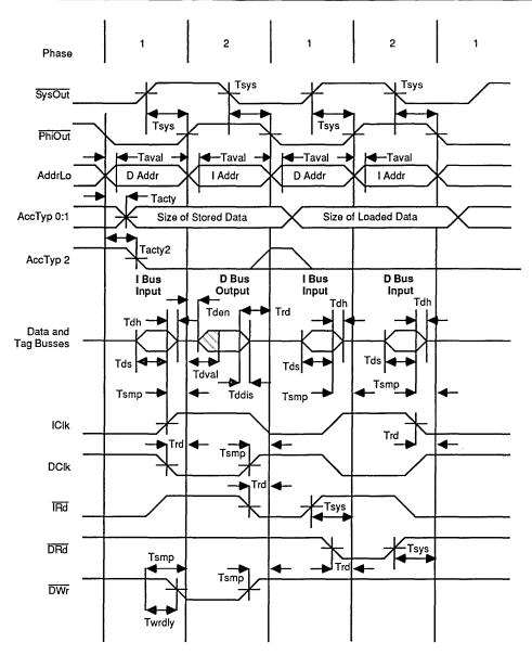
Figure 14. Synchronous Memory (Cache) Timing
