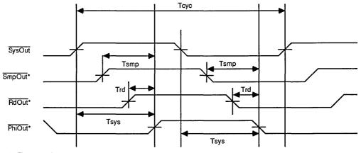
These signals are not actually output from the processor. They are drawn to provide a reference for other timing diagrams.
