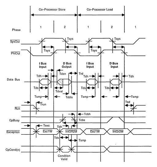
Figure 21. Co-Processor Load/Store Timing
