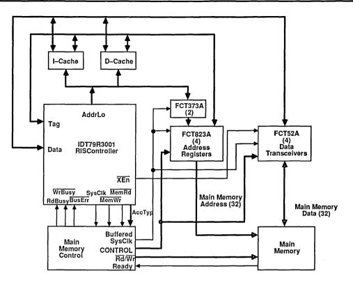
Figure 7. IDT79R3001 Asynchronous Interface
