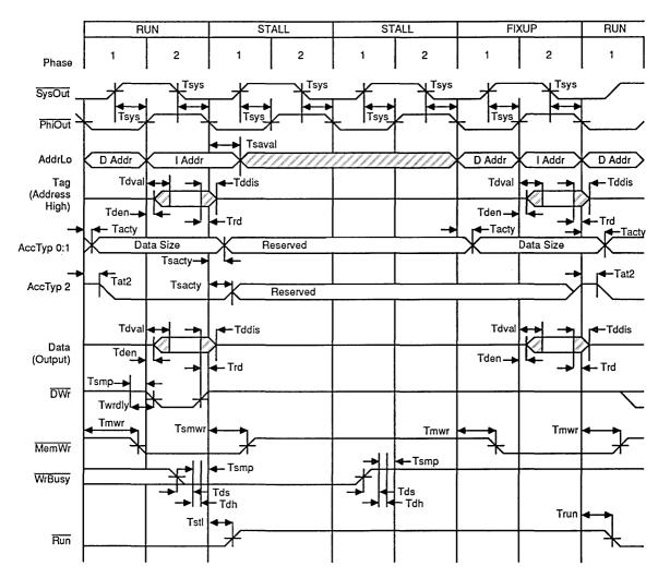
Figure 19. Memory Write Timing
