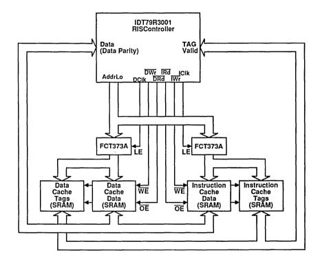
Figure 5. IDT79R3001 Synchronous Interface
