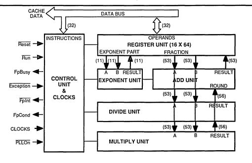
Figure 1. IDT79R3010 Functional Block Diagram
