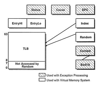
Figure 12. System Control Co-processor (CP0) Registers
