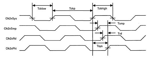
Figure 12. Input Clock Timing
