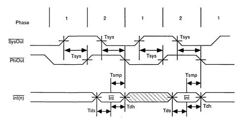
Figure 22. Interrupt Timing
