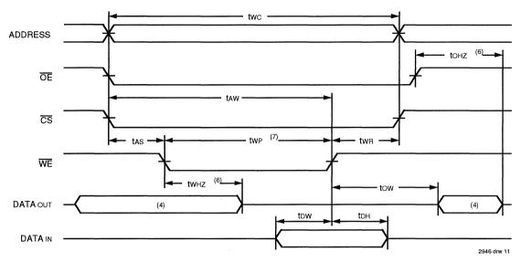
TIMING WAVEFORM OF WRITE CYCLE NO. 2 (CS CONTROLLED TIMING)<sup>(1, 2, 3, 5)</sup>
