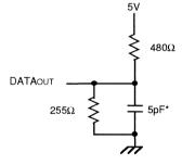
Figure 2. AC Test Load (for toLz, tcLz, toHz, twHz, tcHz & tow)
