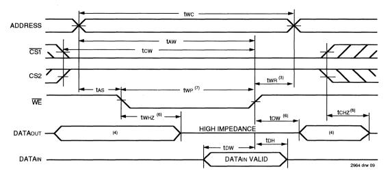
TIMING WAVEFORM OF WRITE CYCLE NO. 2 (CS1 AND CS2 CONTROLLED TIMING)<sup>(1, 2, 5)</sup>
