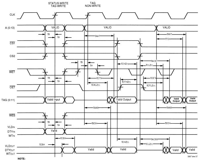
1. Transition is measured ±200mV from steady state.
