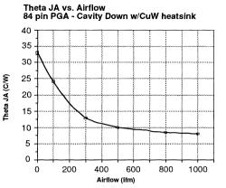
Measurements were done using Temp09 Delco Thermal Die (.250sq.)
