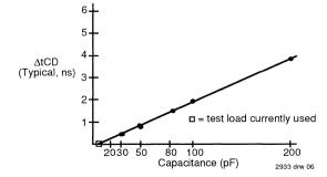
Figure 3. Lumped Capacitive Load, Typical Derating
