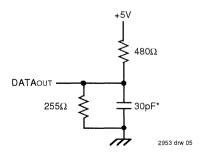
Figure 2. AC Test Load
