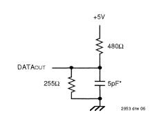
Figure 3. AC Test Load (for toLz, toHz, twHz, tow)
