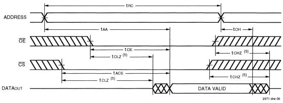
TIMING WAVEFORM OF READ CYCLE NO. 2<sup>(1,2,4)</sup>
