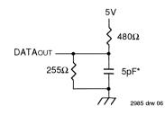
Figure 2. AC Test Load (for tCLZ1, 2, tOLZ, tCHZ1, 2, tOHZ, tow and tWHZ)
