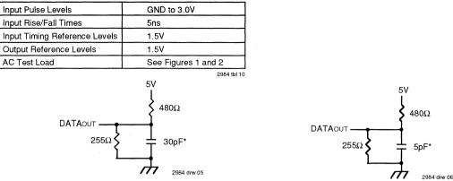
Figure 1. AC Test Load
