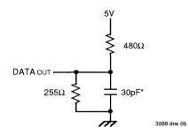
Figure 1. AC Test Load
