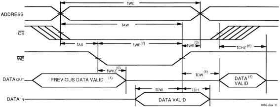
TIMING WAVEFORM OF WRITE CYCLE NO. 2, (CS CONTROLLED TIMING) (1, 2, 3, 5, 7)
