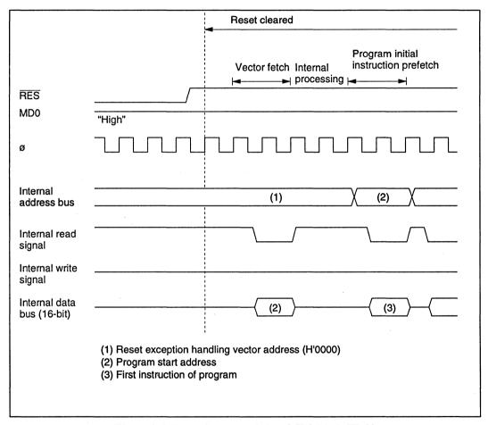
Figure 3-1 Reset Sequence (when MD0 Pin is High)
