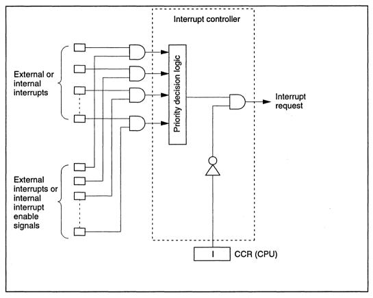
Figure 3-3 Block Diagram of Interrupt Controller
