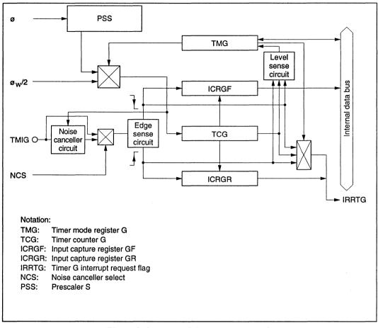
Figure 9-6-1 Block Diagram of Timer G
