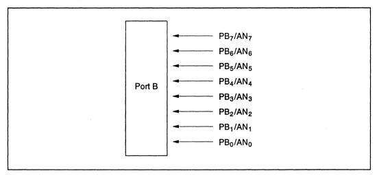
Figure 8-11 Port B Pin Configuration
