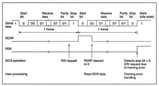
Figure 10-4-9 Typical Receive Operation in Asynchronous Mode (8-Bit Data, Parity Bit Added, and 1 Stop Bit)
