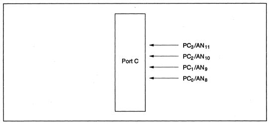
Figure 8-12 Port C Pin Configuration
