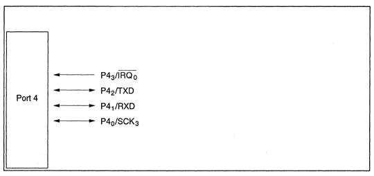
Figure 8-4 Port 4 Pin Configuration
