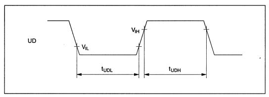
Figure 14-4 Minimum UD High and Low Width
