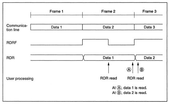
Figure 10-4-22 Relationship between Data and RDR Read Timing
