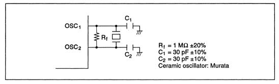
Figure 4-4 Typical Connection to Ceramic Oscillator
