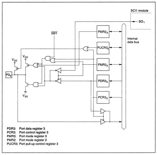
Figure C-3 (f) Port 3 Block Diagram (Pin P3<sub>2</sub>)
