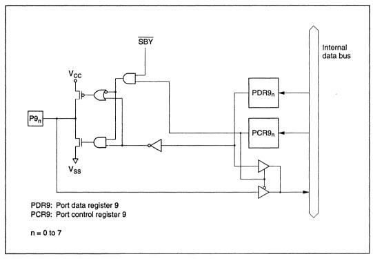
Figure C-9 Port 9 Block Diagram
