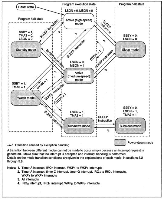
Figure 5-1 Operation Mode Transition Diagram
