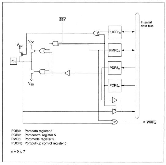
Figure C-5 Port 5 Block Diagram
