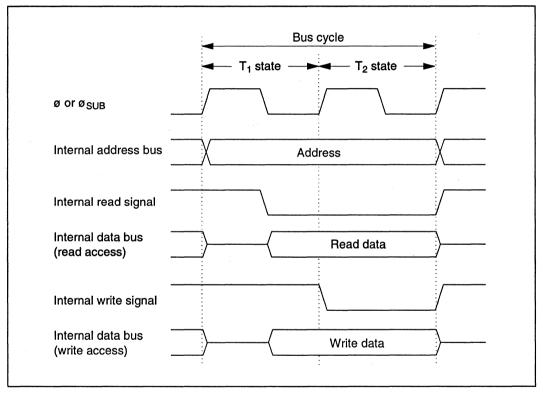
Figure 2-11 On-Chip Memory Access Cycle
