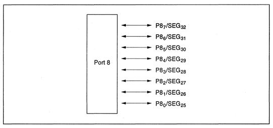
Figure 8-8 Port 8 Pin Configuration
