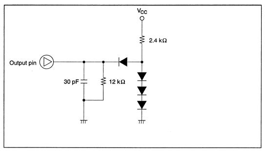
Figure 14-10 Output Load Condition
