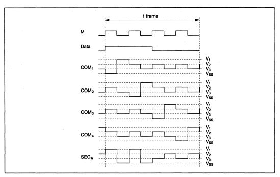
Figure 13-13 (a) Waveforms at 1/4 Duty
