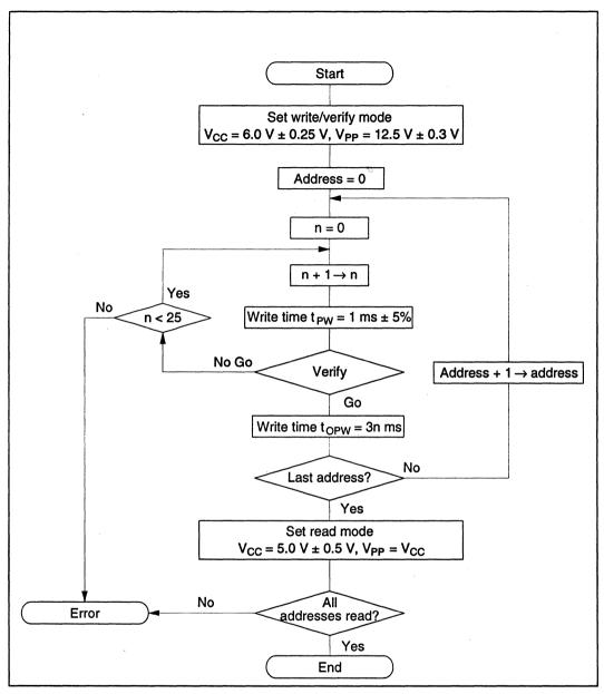
Figure 6-4 High-Performance Programming Flowchart
