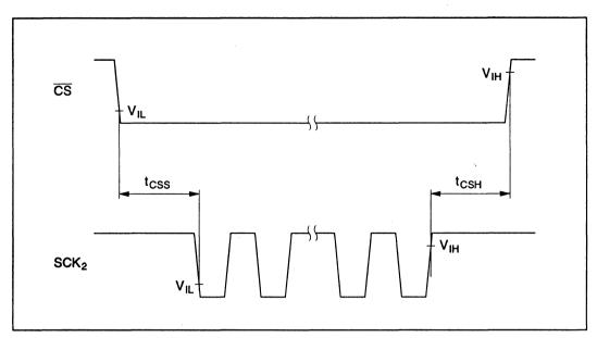
Figure 14-6 Serial Interface 2 Chip Select Timing
