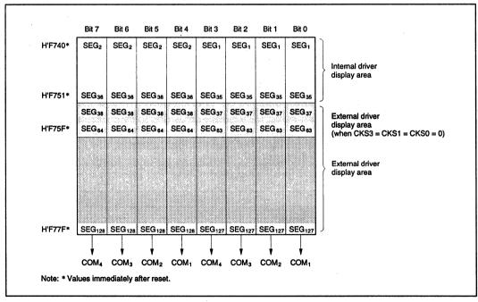
Figure 13-7 LCD RAM Map 1: External Segment Expansion (1/4 Duty)
