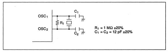
Figure 4-2 Typical Connection to Crystal Oscillator
