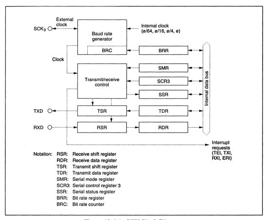
Figure 10-4-1 SCI3 Block Diagram
