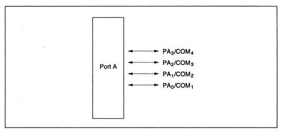
Figure 8-10 Port A Pin Configuration
