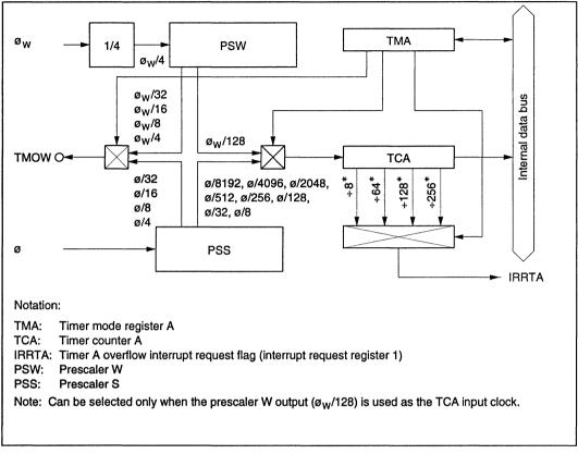
Figure 9-2-1 Block Diagram of Timer A
