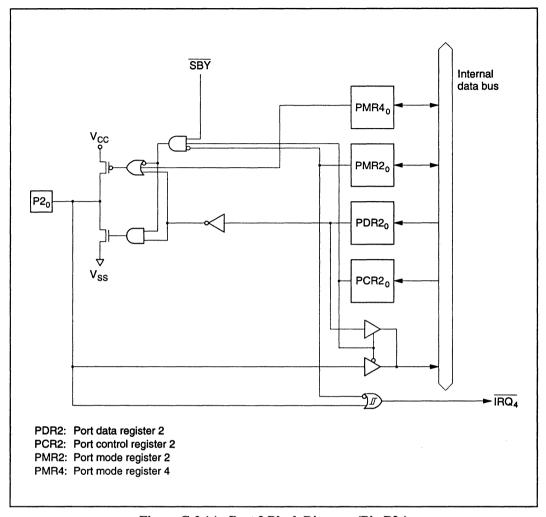
Figure C-2 (c) Port 2 Block Diagram (Pin  $P2_0$ )
