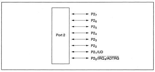
Figure 8-2 Port 2 Pin Configuration
