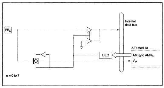
Figure C-11 Port B Block Diagram
