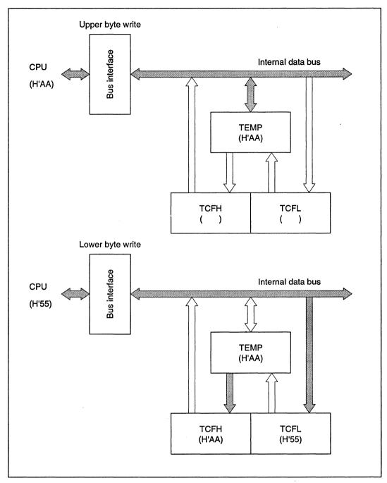
Figure 9-5-2 TCF Write Operation (CPU  $\rightarrow$  TCF)
