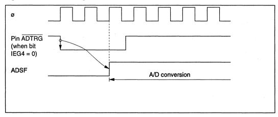
Figure 12-2 External Trigger Input Timing
