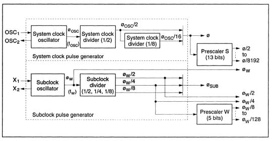
Figure 4-1 Block Diagram of Clock Pulse Generators
