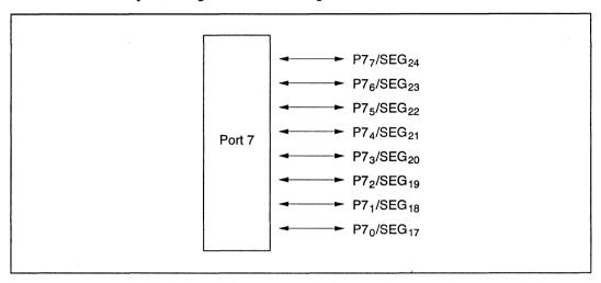
Figure 8-7 Port 7 Pin Configuration
