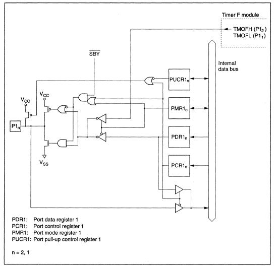
Figure C-1 (d) Port 1 Block Diagram (Pins P1<sub>2</sub> and P1<sub>1</sub>)
