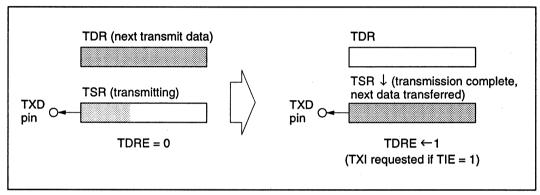
Figure 10-4-2 (b) TDRE Setting and TXI Interrupt
