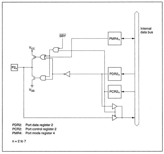
Figure C-2 (a) Port 2 Block Diagram (Pins P2<sub>7</sub> to P2<sub>2</sub>)
