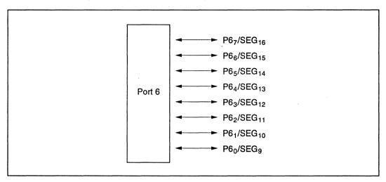
Figure 8-6 Port 6 Pin Configuration
