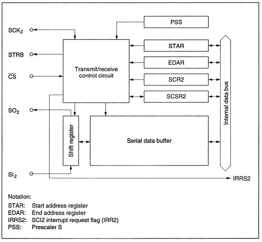
Figure 10-3-1 SCI2 Block Diagram
