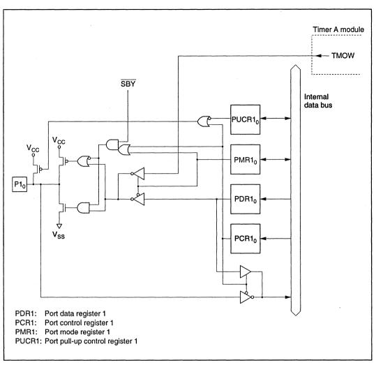
Figure C-1 (e) Port 1 Block Diagram (Pin P1<sub>0</sub>)
