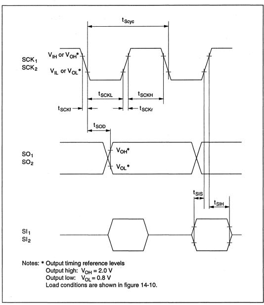
Figure 14-5 Serial Interface 1 and 2 Input/Output Timing
