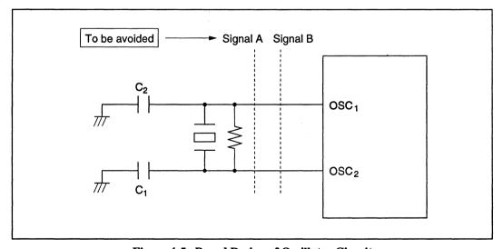
Figure 4-5 Board Design of Oscillator Circuit
