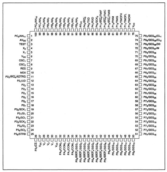
Figure 1-2 Pin Arrangement (FP-100B: Top View)
