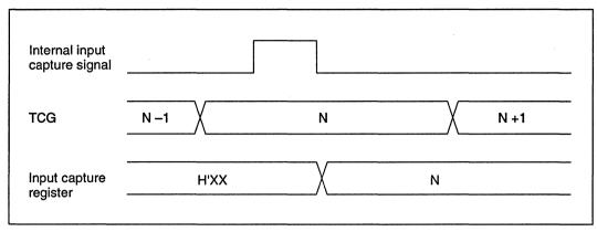
Figure 9-6-6 Input Capture Timing
