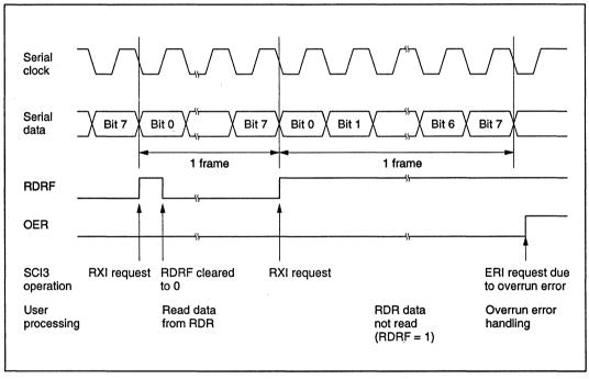
Figure 10-4-14 Typical Receive Operation in Synchronous Mode
