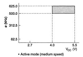
3. Analog power supply voltage vs. A/D converter operating range
