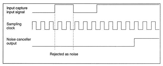
Figure 9-6-3 Noise Canceller Circuit Timing (Example)
