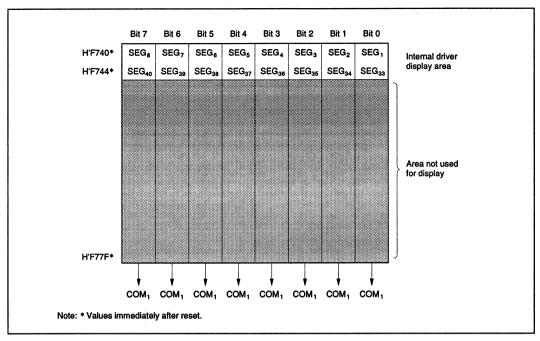
Figure 13-6 LCD RAM Map 4: No External Segment Expansion (Static Duty)
