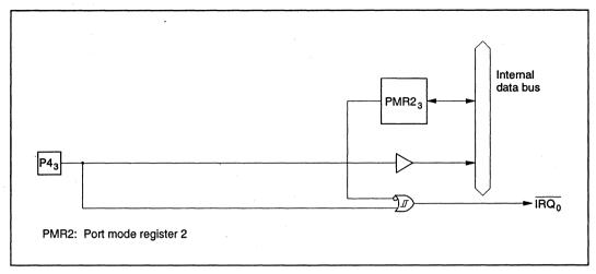
Figure C-4 (a) Port 4 Block Diagram (Pin P43)
