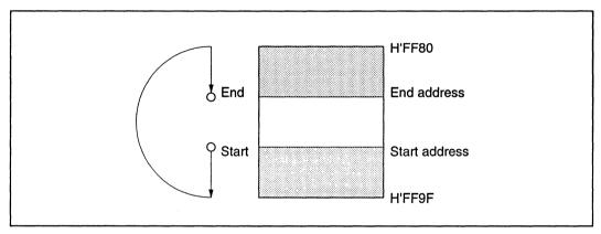
Figure 10-3-4 Operation When End Address is Smaller than Start Address
