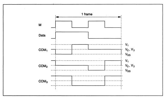
Figure 13-13 (c) Waveforms at 1/2 Duty
