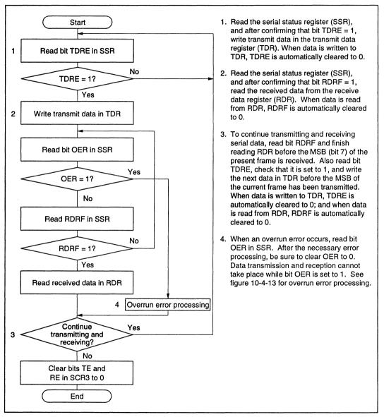
Figure 10-4-15 Simultaneous Transmit/Receive Flow Chart in Synchronous Mode
