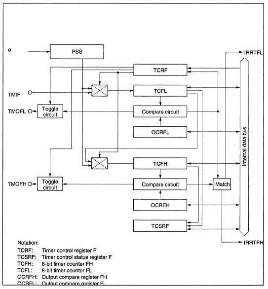
Figure 9-5-1 Block Diagram of Timer F
