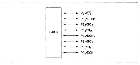
Figure 8-3 Port 3 Pin Configuration
