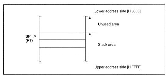
Figure 2-2 Stack Pointer
