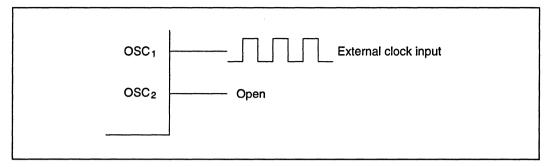
Figure 4-6 External Clock Input (Example)
