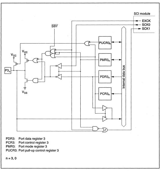
Figure C-3 (e) Port 3 Block Diagram (Pins P3<sub>3</sub> and P3<sub>0</sub>)
