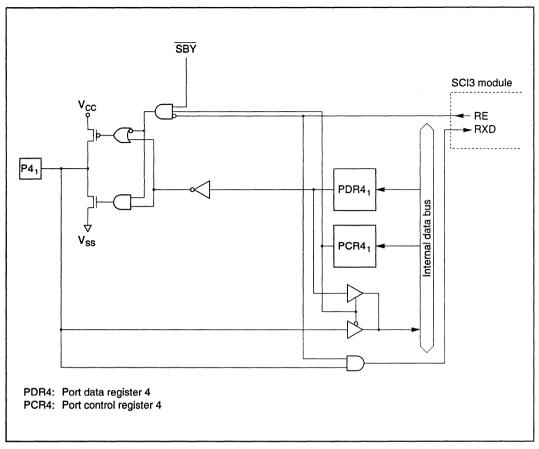
Figure C-4 (c) Port 4 Block Diagram (Pin P4<sub>1</sub>)
