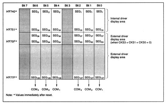
Figure 13-8 LCD RAM Map 2: External Segment Expansion (1/3 Duty)
