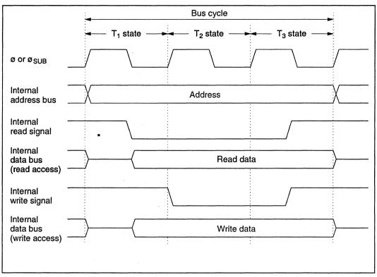
Figure 2-13 On-Chip Peripheral Module Access Cycle (3-State Access)
