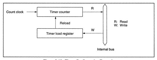
Figure 2-18 Timer Configuration Example
