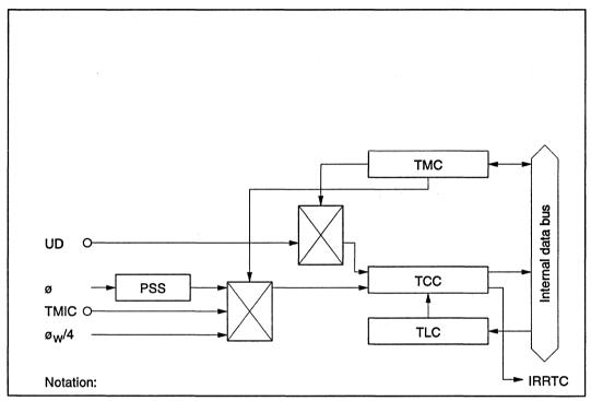
Figure 9-4-1 Block Diagram of Timer C
