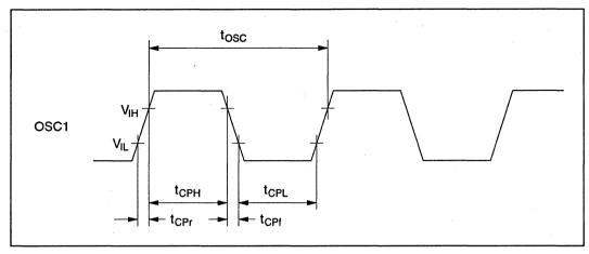
Figure 14-1 System Clock Input Timing
