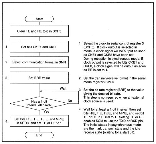
Figure 10-4-5 Typical Flow Chart when SCI3 Is Initialized
