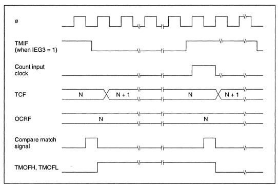
Figure 9-5-4 TMOFH, TMOFL Output Timing
