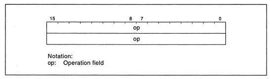
Figure 2-10 Block Data Transfer Instruction Code
