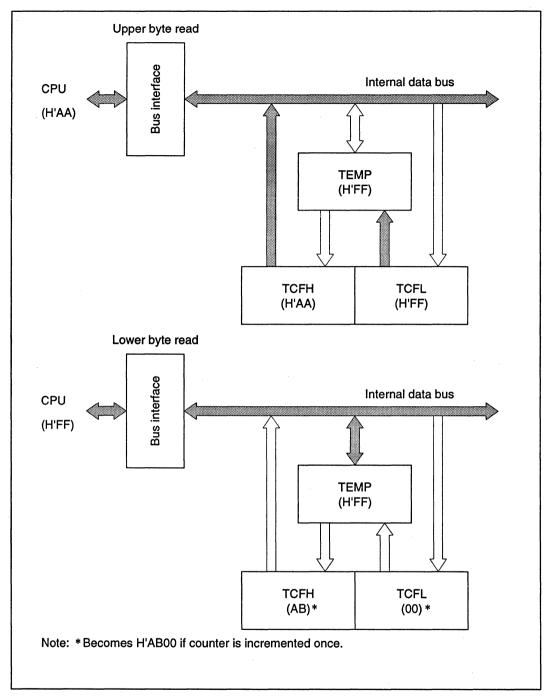
Figure 9-5-3 TCF Read Operation (TCF  $\rightarrow$  CPU)
