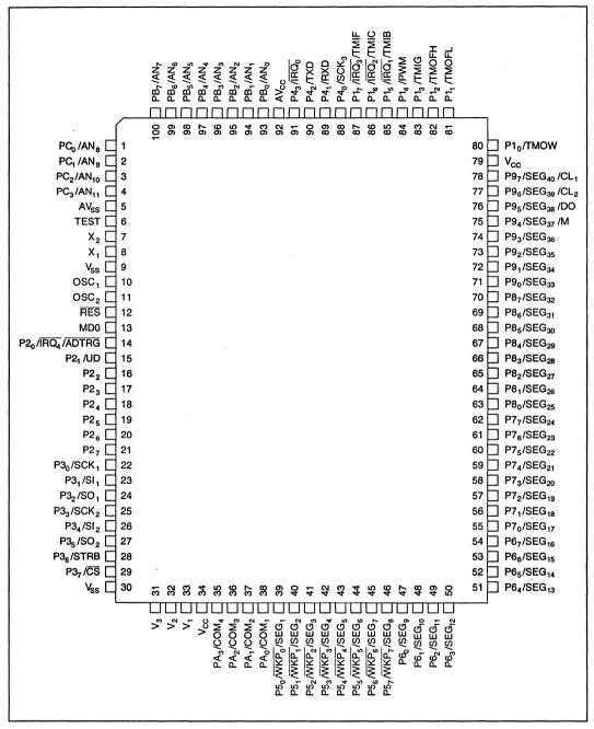
Figure 1-3 Pin Arrangement (FP-100A: Top View)
