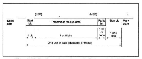
Figure 10-4-3 Data Format in Asynchronous Serial Communication Mode
