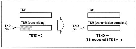
Figure 10-4-2 (c) TEND Setting and TEI Interrupt
