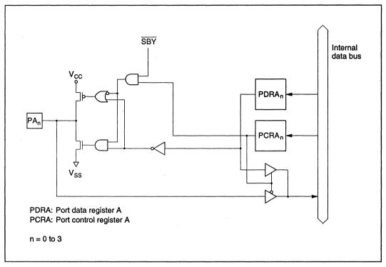
Figure C-10 Port A Block Diagram
