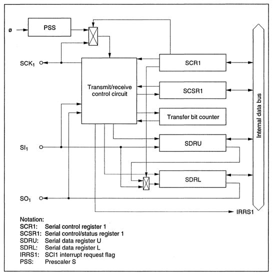
Figure 10-2-1 SCI1 Block Diagram
