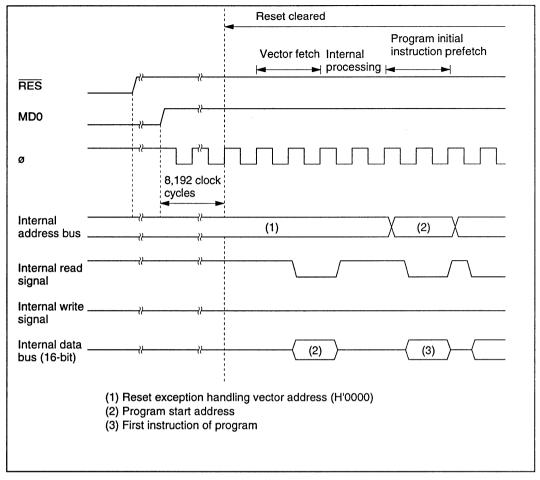
Figure 3-2 Reset Sequence (when MD0 Pin is Low)
