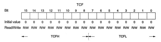
TCF is a 16-bit read/write up-counter consisting of two cascaded 8-bit timer counters, TCFH and TCFL. TCF can be used as a 16-bit counter, with TCFH as the upper 8 bits and TCFL as the lower 8 bits of the counter, or TCFH and TCFL can be used as independent 8-bit counters.
