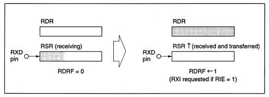
Figure 10-4-2 (a) RDRF Setting and RXI Interrupt
