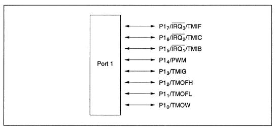
Figure 8-1 Port 1 Pin Configuration
