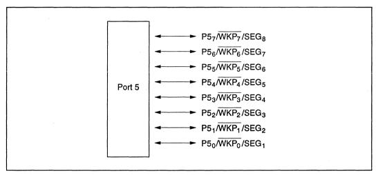
Figure 8-5 Port 5 Pin Configuration
