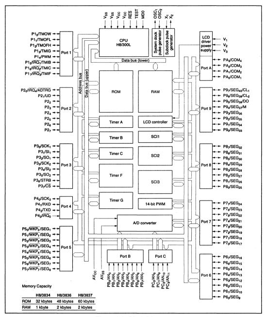
Figure 1-1 Block Diagram
