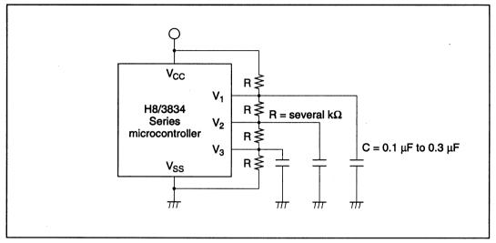
Figure 13-14 Connecting an External Resistive Voltage Divider
