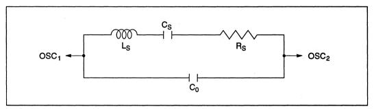
Figure 4-3 Equivalent Circuit of Crystal Oscillator
