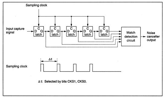
Figure 9-6-2 Block Diagram of Noise Canceller Circuit
