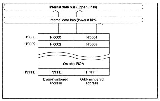
Figure 6-1 ROM Block Diagram (H8/3834)
