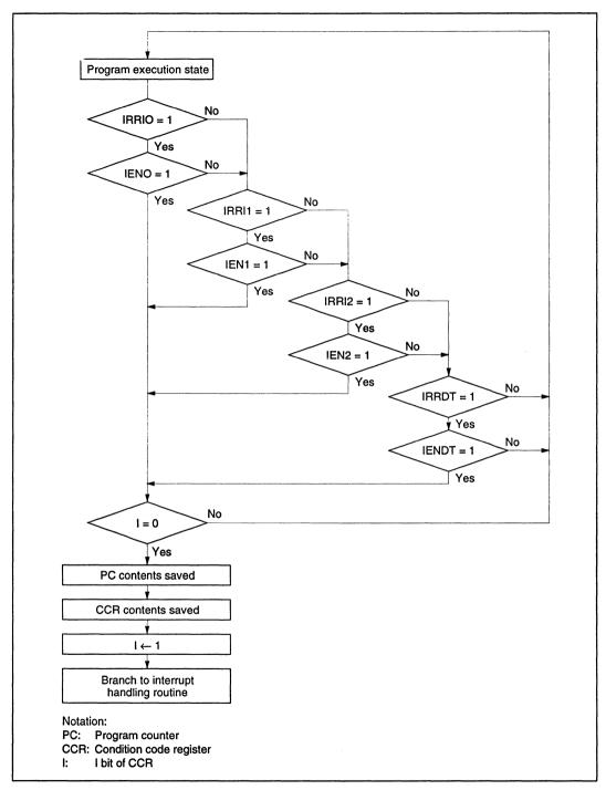
Figure 3-4 Flow up to Interrupt Acceptance
