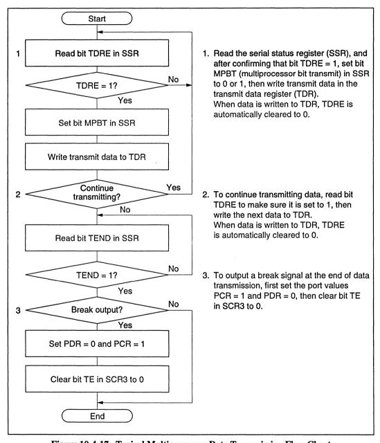
Figure 10-4-17 Typical Multiprocessor Data Transmission Flow Chart
