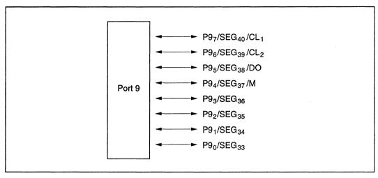
Figure 8-9 Port 9 Pin Configuration
