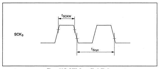
Figure 14-7 SCK<sub>3</sub> Input Clock Timing
