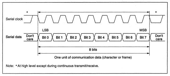
Figure 10-4-10 Data Format in Synchronous Communication Mode
