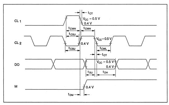
Figure 14-9 Segment Expansion Signal Timing
