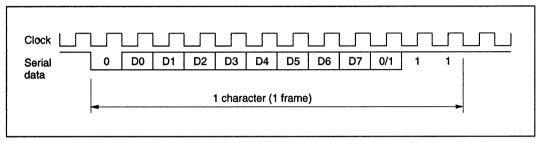
Figure 10-4-4 Phase Relation of Output Clock and Communication Data in Asynchronous Mode (8-Bit Data, Parity Bit Added, and 2 Stop Bits)
