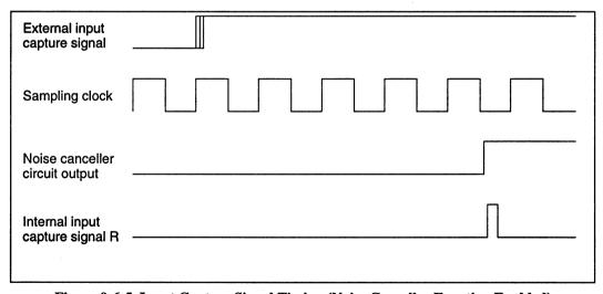
Figure 9-6-5 Input Capture Signal Timing (Noise Canceller Function Enabled)
