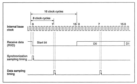
Figure 10-4-21 Receive Data Sampling Timing in Asynchronous Mode
