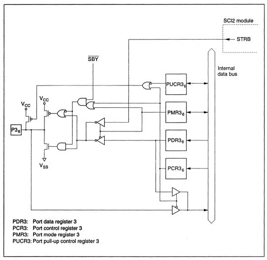
Figure C-3 (b) Port 3 Block Diagram (Pin P3<sub>6</sub>)
