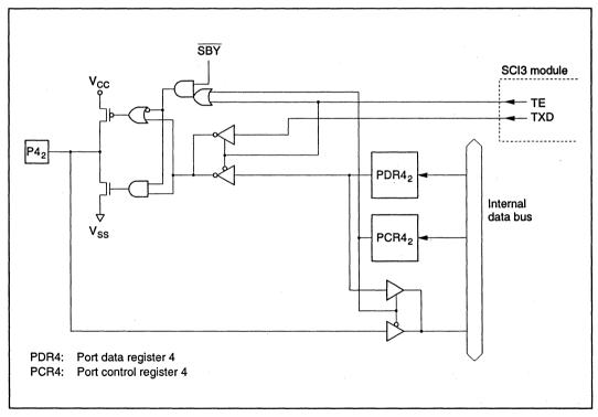
Figure C-4 (b) Port 4 Block Diagram (Pin P42)
