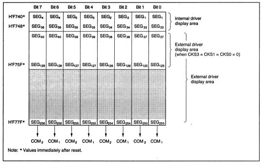
Figure 13-9 LCD RAM Map 3: External Segment Expansion (1/2 Duty)
