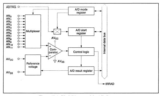
Figure 12-1 Block Diagram of the A/D Converter
