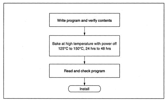
Figure 6-10 Recommended Screening Procedure
