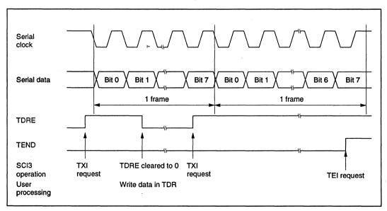
Figure 10-4-12 Typical SCI3 Transmit Operation in Synchronous Mode
