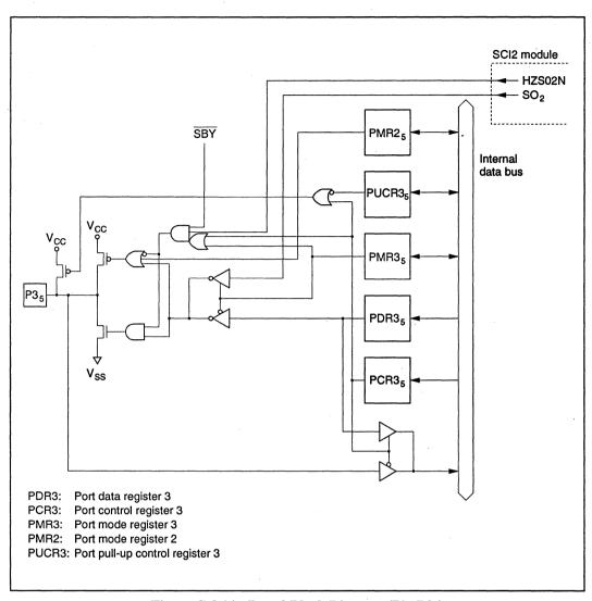
Figure C-3 (c) Port 3 Block Diagram (Pin  $P3_5$ )
