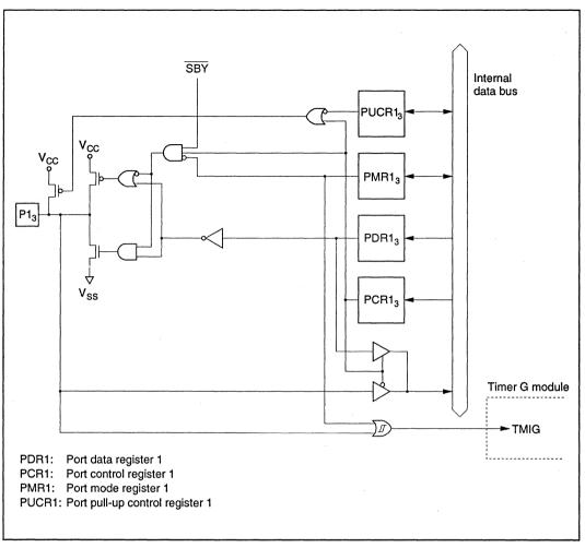
Figure C-1 (c) Port 1 Block Diagram (Pin P1<sub>3</sub>)
