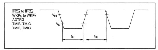
Figure 14-3 Input Timing
