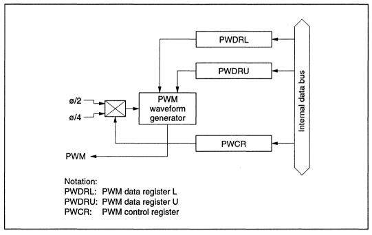
Figure 11-1 Block Diagram of the 14 bit PWM
