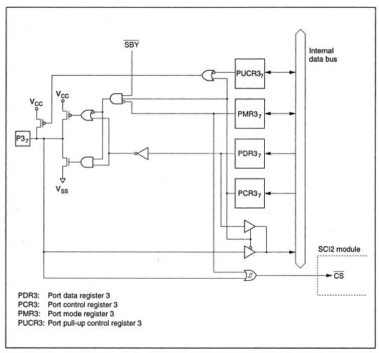
Figure C-3 (a) Port 3 Block Diagram (Pin P37)
