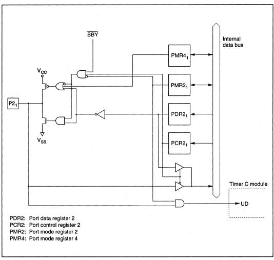
Figure C-2 (b) Port 2 Block Diagram (Pin P2<sub>1</sub>)
