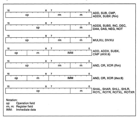
Figure 2-6 Arithmetic, Logic, and Shift Instruction Codes
