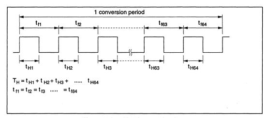
Figure 11-2 PWM Output Waveform
