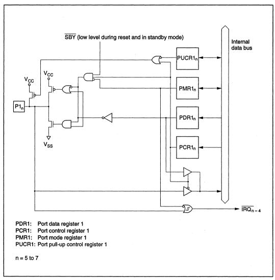
Figure C-1 (a) Port 1 Block Diagram (Pins P1<sub>7</sub> to P1<sub>5</sub>)
