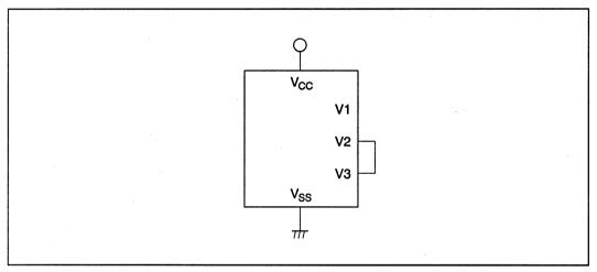
Figure 13-2 LCD Driver Power Supply Processing at 1/2 Duty
