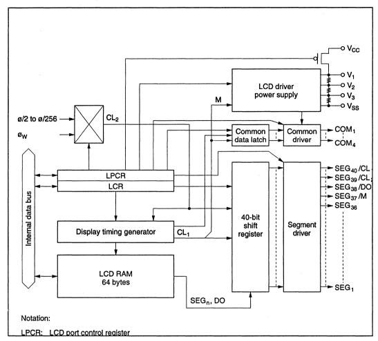
Figure 13-1 LCD Controller/Driver Block Diagram
