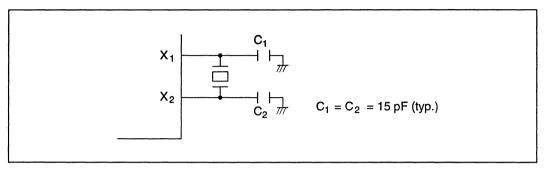
Figure 4-7 Typical Connection to 32.768-kHz Crystal Oscillator (Subclock)
