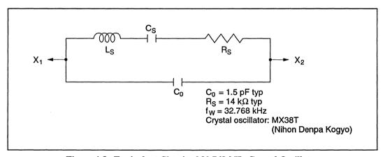
Figure 4-8 Equivalent Circuit of 32.768-kHz Crystal Oscillator
