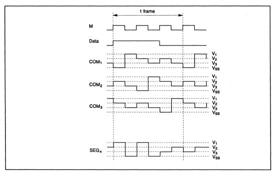
Figure 13-13 (b) Waveforms at 1/3 Duty
