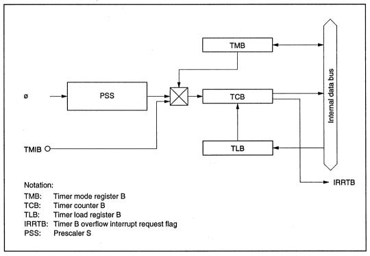
Figure 9-3-1 Block Diagram of Timer B
