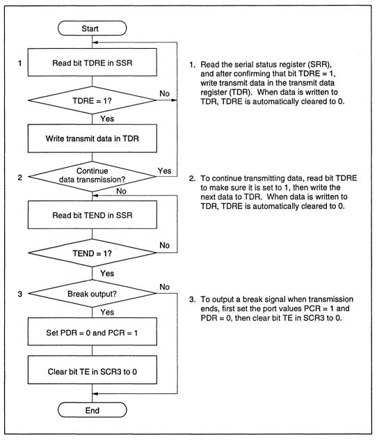
Figure 10-4-6 Typical Data Transmission Flow Chart (Asynchronous Mode)
