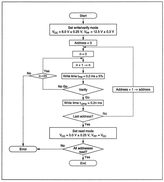
Figure 6-8 High-Speed, High-Reliability Programming Flow Chart
