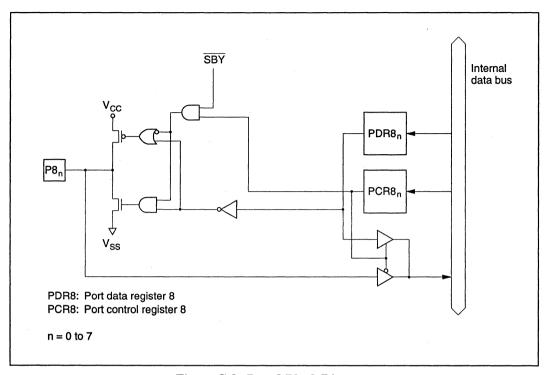
Figure C-8 Port 8 Block Diagram
