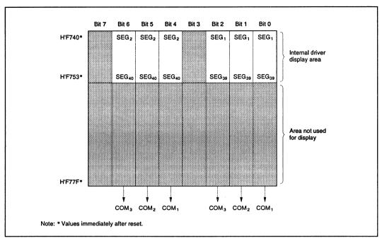
Figure 13-4 LCD RAM Map 2: No External Segment Expansion (1/3 Duty)
