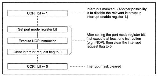
Figure 3-8 Port Mode Register Setting and Interrupt Request Flag Clearing Procedure
