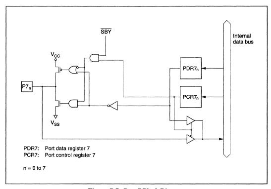
Figure C-7 Port 7 Block Diagram
