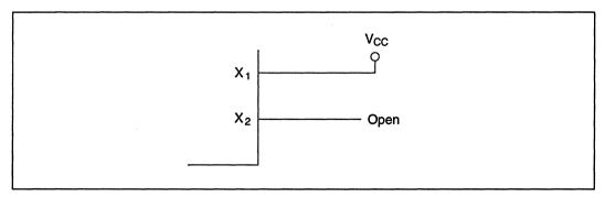
Figure 4-9 Pin Connection when not Using Subclock
