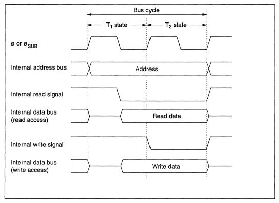
Figure 2-12 On-Chip Peripheral Module Access Cycle (2-State Access)
