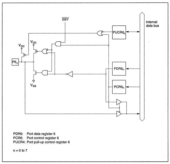
Figure C-6 Port 6 Block Diagram
