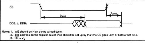
Figure 17-20. Dual-Port RAM Read Timing
