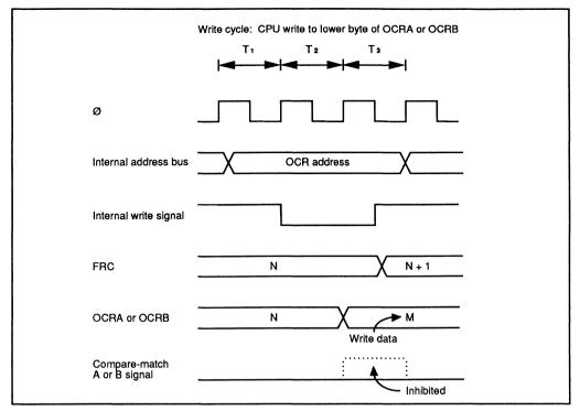
Figure 6-23. Contention between OCR Write and Compare-Match
