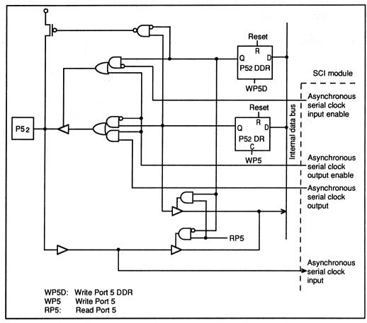
Figure 5-8. Port 5 Schematic Diagram (Pin P52)
