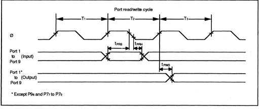
Figure 17-19. I/O Port Input/Output Timing
