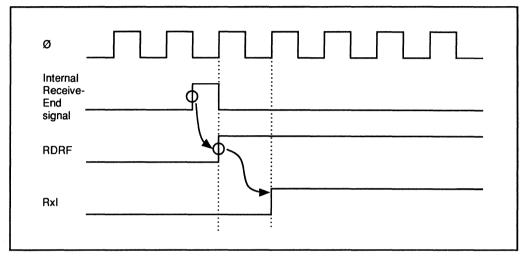
Figure 9-5. Timing of Interrupt Signal
