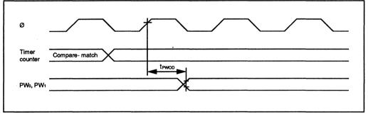
Figure 17-16. PWM Timer Output Timing
