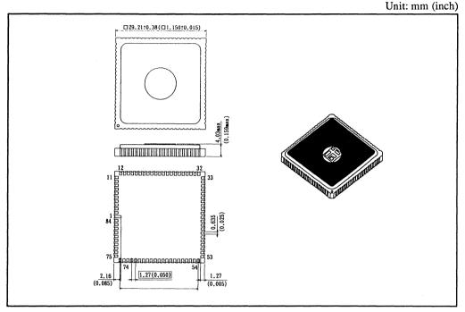
Figure D-1. Package Dimensions (CG-84)
