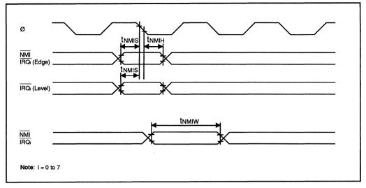
Figure 17-8. Interrupt Input Timing
