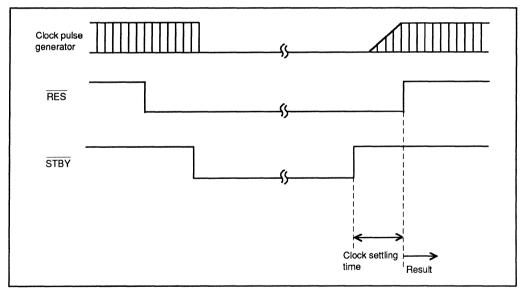
Figure 14-2. Hardware Standby Mode Timing
