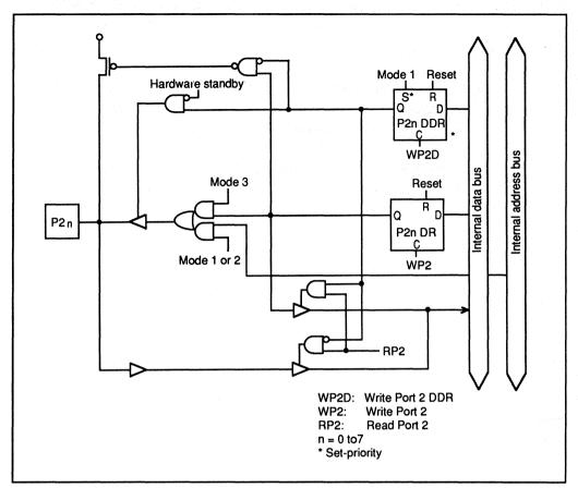
Figure 5-2. Port 2 Schematic Diagram
