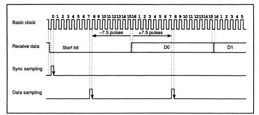
Figure 9-6. Sampling Timing (Asynchronous Mode)
