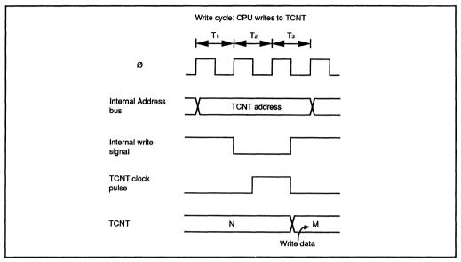
Figure 7-14. TCNT Write-Increment Contention
