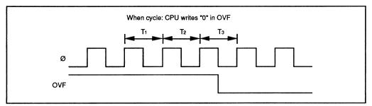
Figure 7-11. Clearing of Overflow Flag
