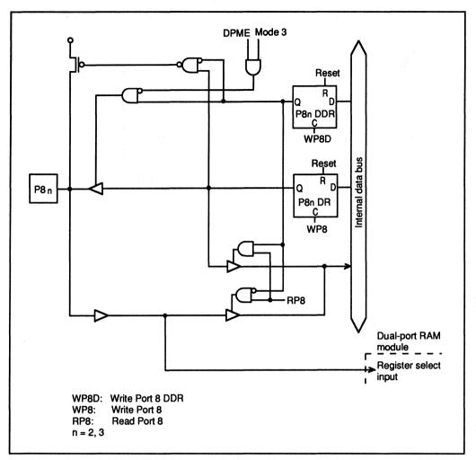
Figure 5-16. Port 8 Schematic Diagram (Pins P82 and P83)
