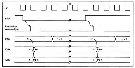
Figure 6-15. Buffered Input Capture with Both Edges Selected
