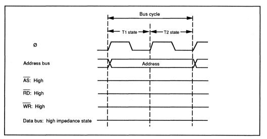
Figure 3-14. Pin States during On-Chip Memory Access Cycle
