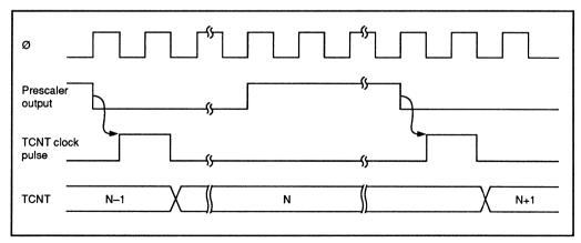
Figure 8-2. TCNT Increment Timing
