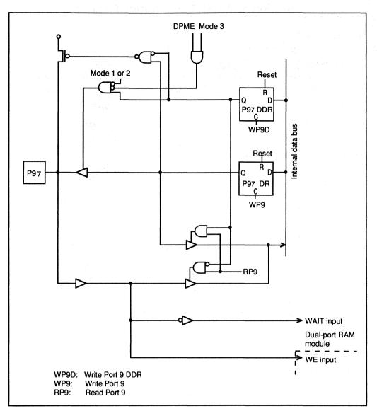
Figure 5-25. Port 9 Schematic Diagram (Pin P97)
