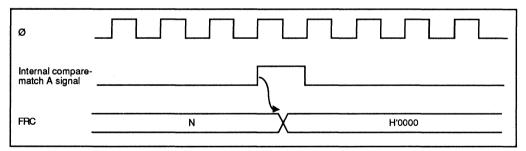
Figure 6-11. Clearing of FRC by Compare-Match A
