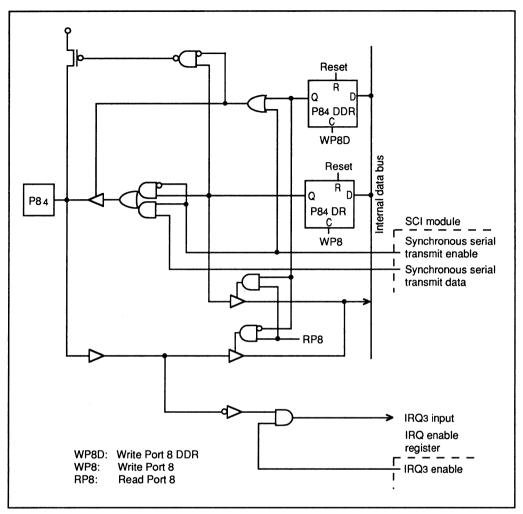
Figure 5-17. Port 8 Schematic Diagram (Pin P84)
