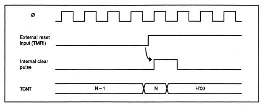
Figure 7-9. Timing of External Reset
