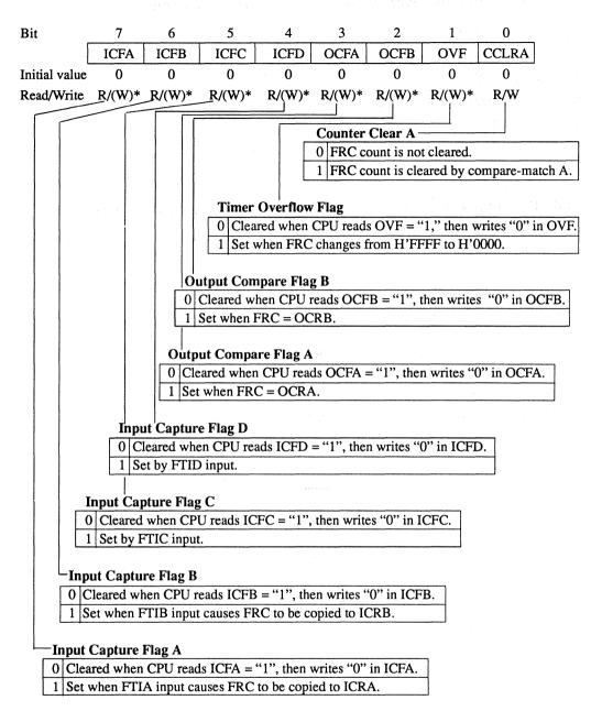
\* Software can write a "0" in bits 7 to 1 to clear the flags, but cannot write a "1" in these bits
