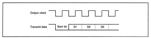
Figure 9-3. Phase Relationship Between Clock Output and Transmit Data
