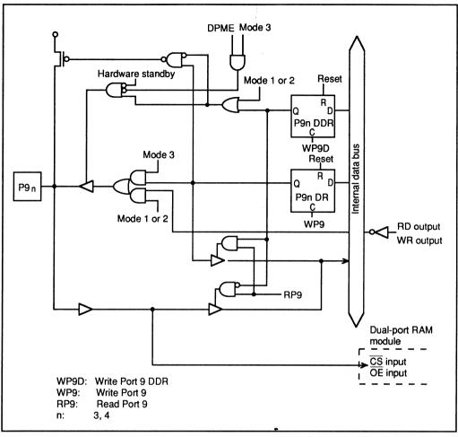
Figure 5-22. Port 9 Schematic Diagram (Pins P93 and P94)
