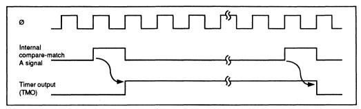
Figure 7-7. Timing of Timer Output
