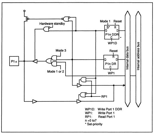
Figure 5-1. Port 1 Schematic Diagram
