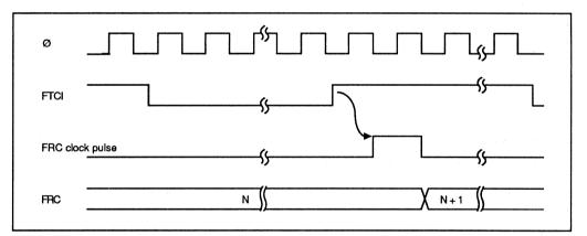
Figure 6-6. Increment Timing for External Clock Source
