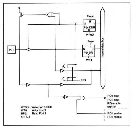
Figure 5-21. Port 9 Schematic Diagram (Pins P91 to P92)
