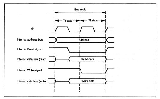
Figure 3-13. On-Chip Memory Access Cycle
