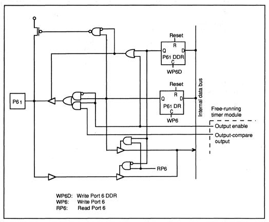
Figure 5-10. Port 6 Schematic Diagram (Pin P61)
