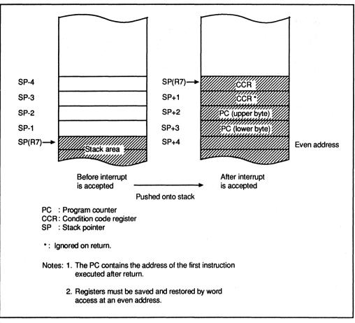
Figure 4-6. Usage of Stack in Interrupt Handling
