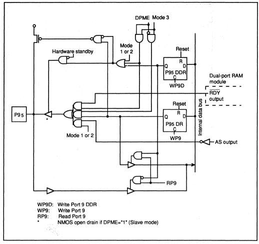
Figure 5-23. Port 9 Schematic Diagram (Pin P95)
