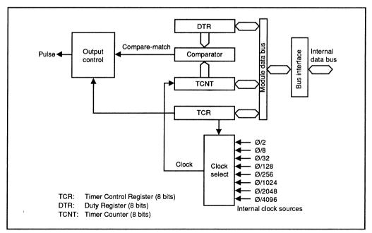
Figure 8-1. Block Diagram of PWM Timer
