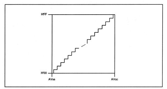
Figure 10-2. The Response of the A/D Converter
