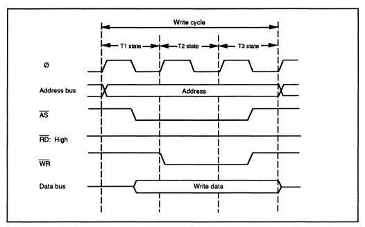
Figure 3-17 (b). External Device Access Timing (write)
