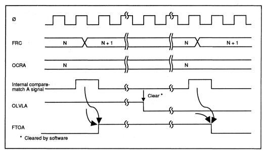
Figure 6-10. Timing of Output Compare A
