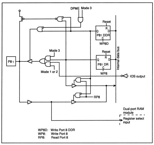
Figure 5-15. Port 8 Schematic Diagram (Pin P81)
