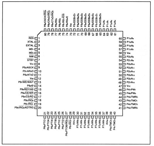
Figure 1-2. Pin Arrangement (FP-80A, Top View)
