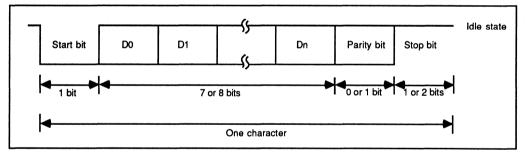
Figure 9-2. Data Format in Asynchronous Mode
