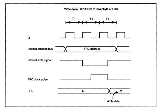
Figure 6-22. FRC Write-Increment Contention
