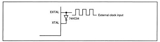
Figure 16-5. External Clock Input (Example)
