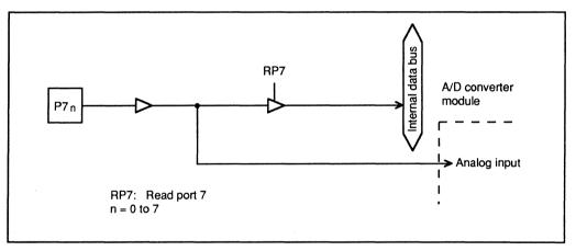
Figure 5-13. Port 7 Schematic Diagram
