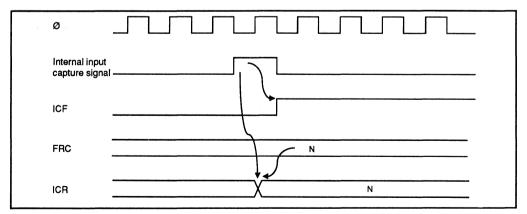
Figure 6-16. Setting of Input Capture Flag
