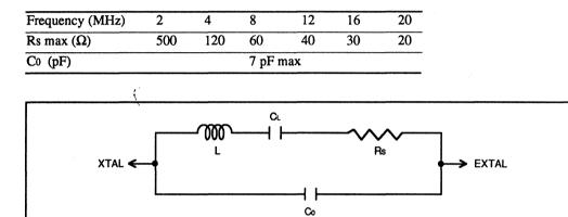
Figure 16-3. Equivalent Circuit of External Crystal
