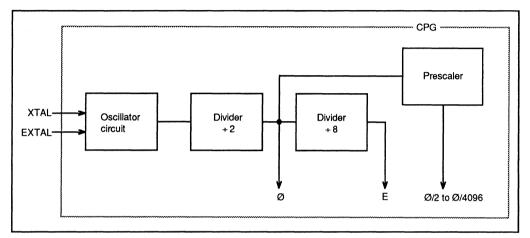
Figure 16-1. Block Diagram of Clock Pulse Generator
