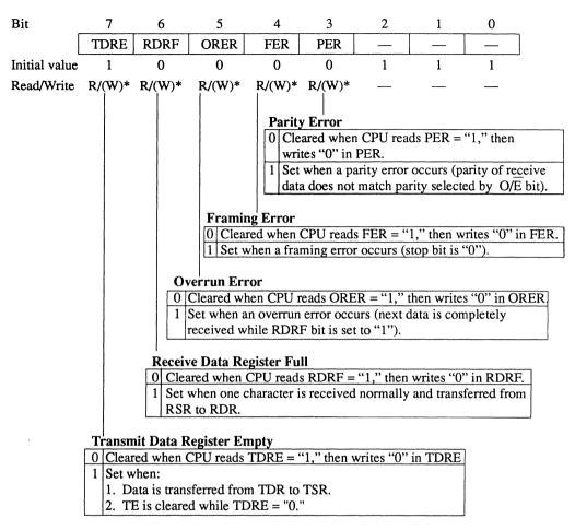
\* Software can write a "0" in bits 7 to 3 to clear the flags, but cannot write a "1" in these bits.
