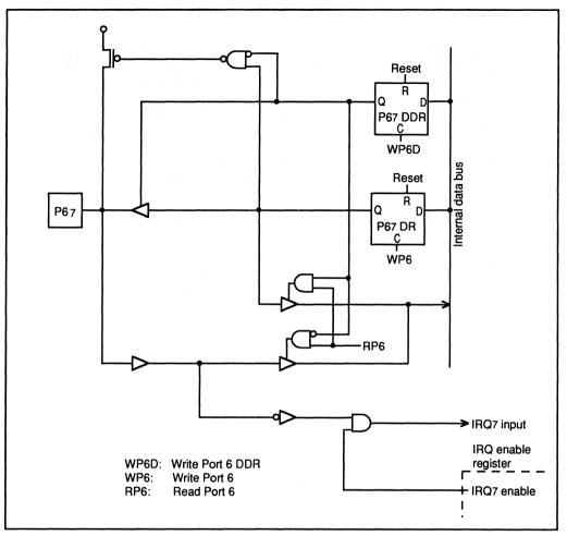
Figure 5-12. Port 6 Schematic Diagram (Pin P67)
