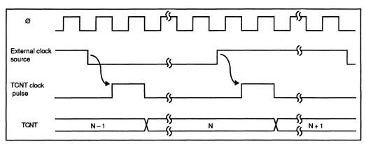
Figure 7-3. Count Timing for External Clock Input
