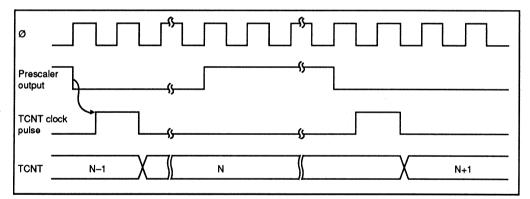
Figure 7-2. Count Timing for Internal Clock Input
