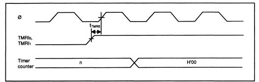
Figure 17-15. 8-Bit Timer Reset Input Timing
