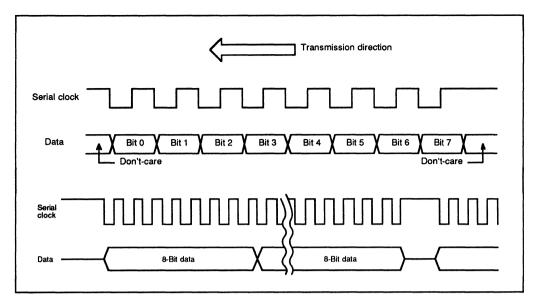
Figure 9-4. Data Format in Synchronous Mode
