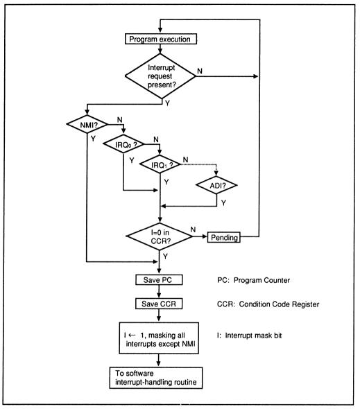
Figure 4-4. Hardware Interrupt-Handling Sequence
