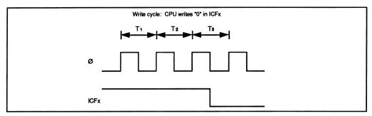
Figure 6-17. Clearing of Input Capture Flag
