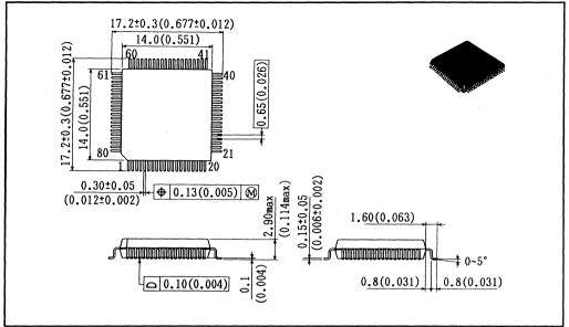
Figure D-3. Package Dimensions (FP-80A)
