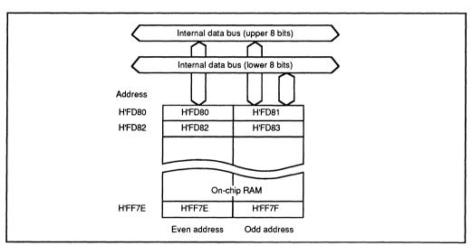
Figure 12-1 is a block diagram of the on-chip RAM.
