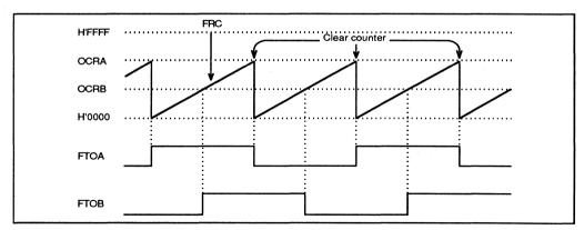
Figure 6-20. Square-Wave Output (Example)
