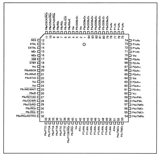
Figure 1-3. Pin Arrangement (CP-84, Top View)
