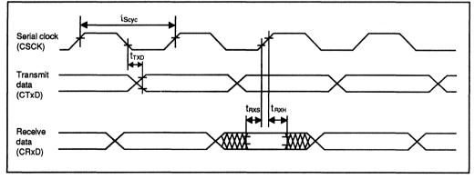
Figure 17-17. SCI Input/Output Timing (Synchronous Mode)
