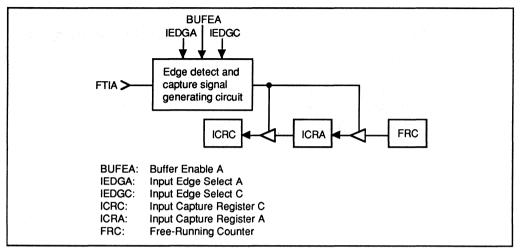
Figure 6-2. Input Capture Buffering
