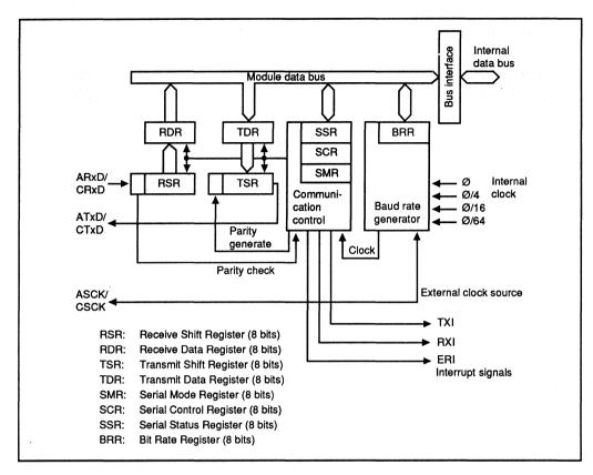
Figure 9-1. Block Diagram of Serial Communication Interface
