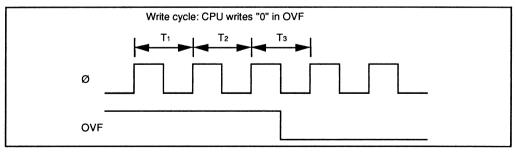
Figure 6-19. Clearing of Overflow Flag
