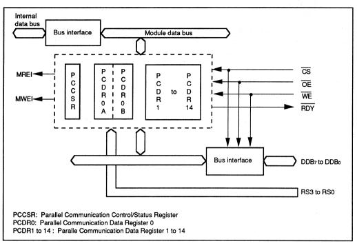
Figure 11-1 shows a block diagram of the dual-port RAM.
