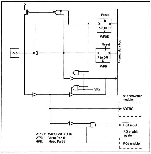
Figure 5-20. Port 9 Schematic Diagram (Pin P90)
