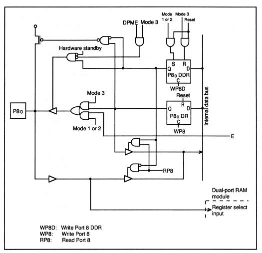
Figure 5-14. Port 8 Schematic Diagram (Pin P80)
