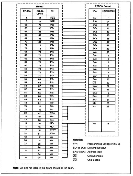
Figure 13-2. Socket Adapter Pin Assignments
