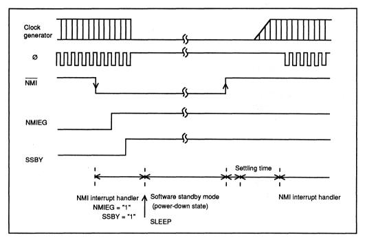
Figure 14-1. Software Standby Mode (when) NMI Timing
