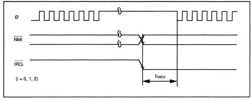
Figure 17-10. Clock Settling Timing for Recovery from Software Standby Mode
