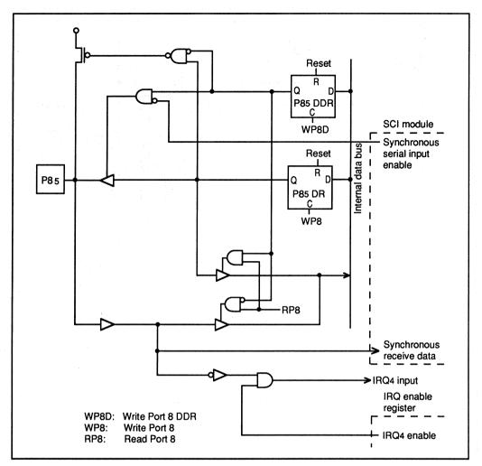
Figure 5-18. Port 8 Schematic Diagram (Pin P8s)
