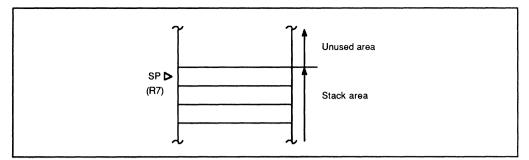
Figure 3-2. Stack Pointer
