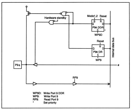
Figure 5-24. Port 9 Schematic Diagram (Pin P96)
