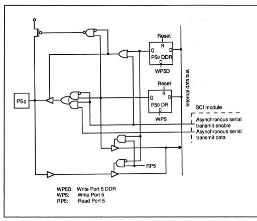
Figure 5-6. Port 5 Schematic Diagram (Pin P50)
