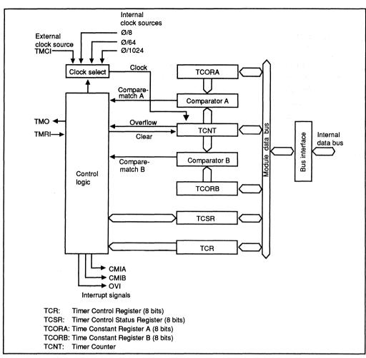
Figure 7-1. Block Diagram of 8-Bit Timer
