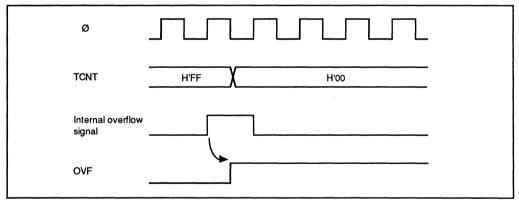
Figure 7-10. Setting of Overflow Flag (OVF)
