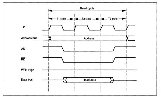
Figure 3-17 (a). External Device Access Timing (read)
