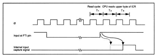
Figure 6-13. Input Capture Timing (1-State Delay)
