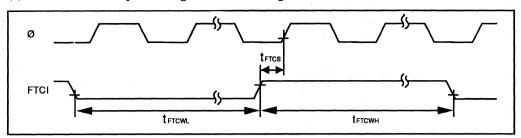
Figure 17-12. External Clock Input Timing for Free-Running Timer
