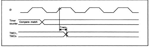
Figure 17-13. 8-Bit Timer Output Timing
