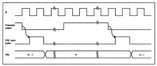
Figure 6-5. Increment Timing for Internal Clock Source
