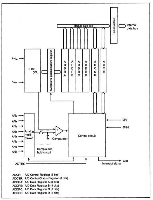
Figure 10-1. Block Diagram of A/D Converter
