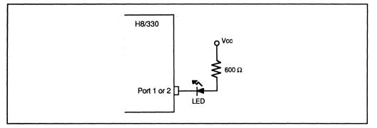
Figure 17-2. Example of Circuit for Driving a LED
