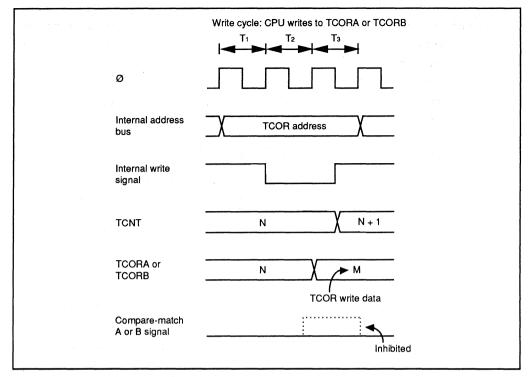
Figure 7-15. Contention between TCOR Write and Compare-Match
