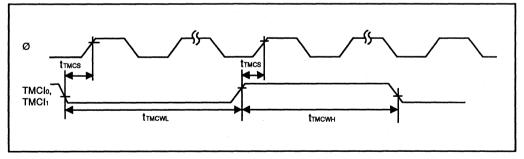
Figure 17-14. 8-Bit Timer Clock Input Timing
