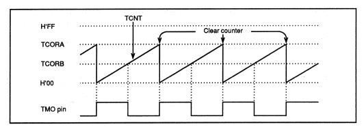
Figure 7-12. Example of Pulse Output
