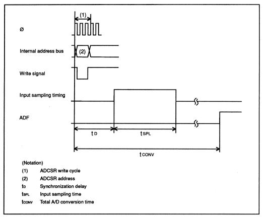
Figure 10-5. A/D Conversion Timing
