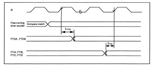
Figure 17-11. Free-Running Timer Input/Output Timing
