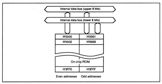
Figure 13-1. Block Diagram of On-Chip ROM
