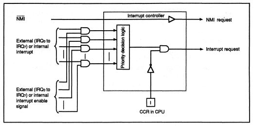
Figure 4-3. Block Diagram of Interrupt Controller
