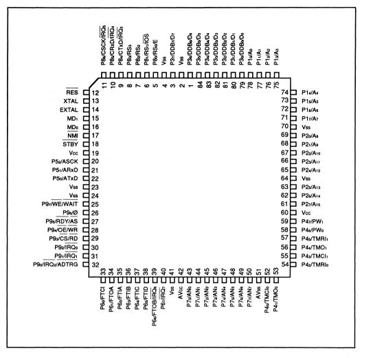
Figure 1-4. Pin Arrangement (CG-84, Top View)
