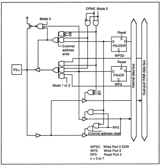
Figure 5-3. Port 3 Schematic Diagram
