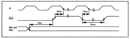
Figure 17-7. Reset Input Timing
