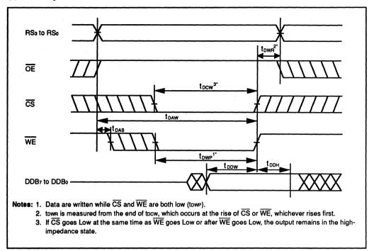
Figure 17-21. Dual-Port RAM Write Timing
