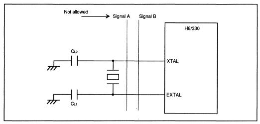
Figure 16-4. Notes on Board Design around External Crystal
