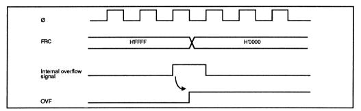
Figure 6-18. Setting of Overflow Flag (OVF)
