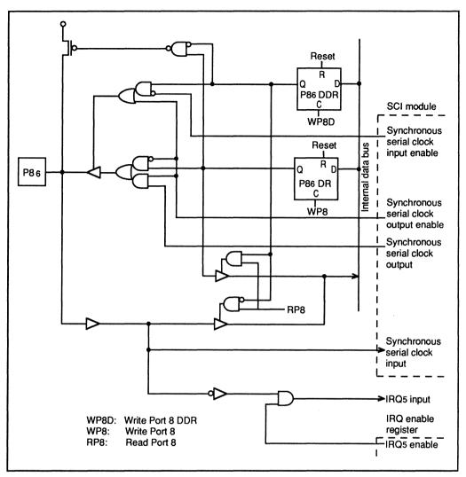
Figure 5-19. Port 8 Schematic Diagram (Pin P86)
