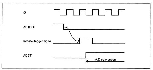
Figure 10-6. External Trigger Input Timing
