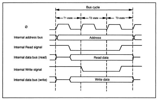
Figure 3-15. On-Chip Register Field Access Cycle
