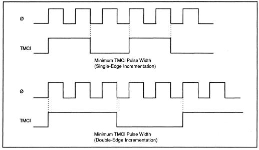
Figure 7-4. Minimum External Clock Pulse Widths (Example)
