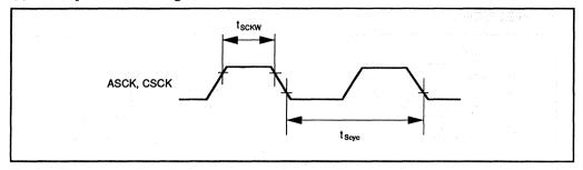
Figure 17-18. SCI Input Clock Timing
