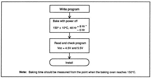
Figure 13-6. Recommended Screening Procedure
