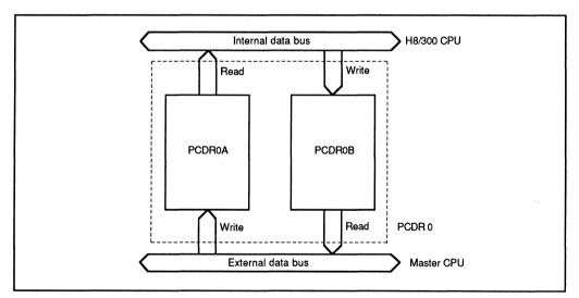
Figure 11-2. Parallel Communication Data Register 0
