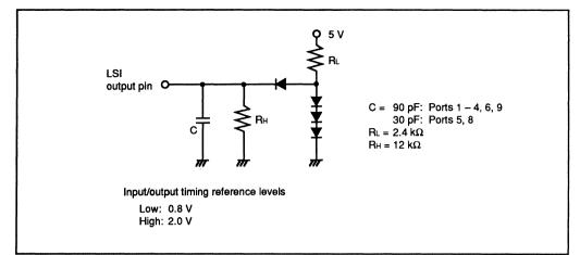
Figure 17-3. Output Load Circuit
