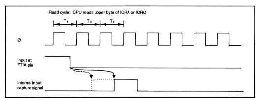
Figure 6-14. Input Capture Timing (1-State Delay, Buffer Mode)
