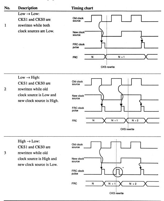
\* The switching of clock sources is regarded as a falling edge that increments the FRC.
