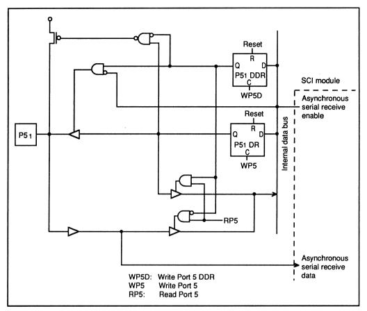
Figure 5-7. Port 5 Schematic Diagram (Pin P51)
