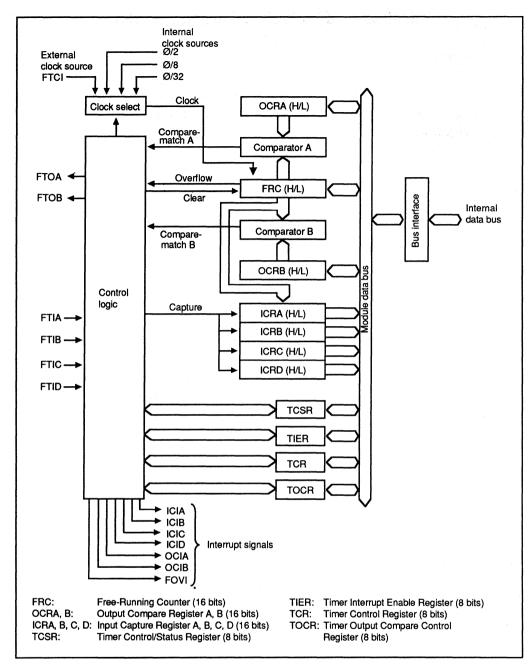
Figure 6-1. Block Diagram of 16-Bit Free-Running Timer
