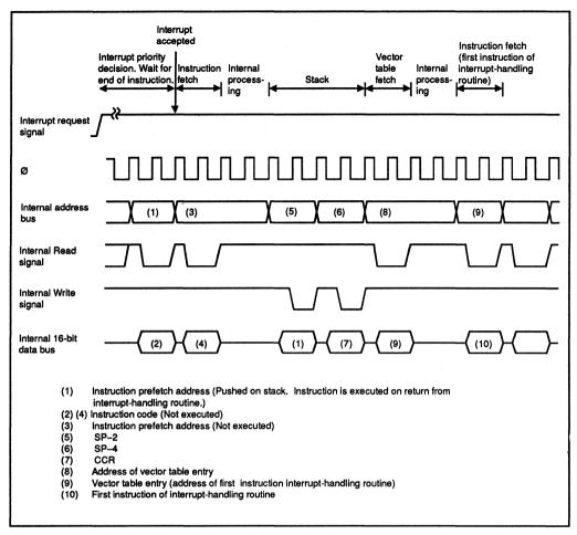
Figure 4-5. Timing of Interrupt Sequence
