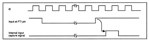
Figure 6-12. Input Capture Timing (Usual Case)
