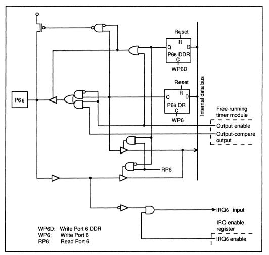
Figure 5-11. Port 6 Schematic Diagram (Pin P66)
