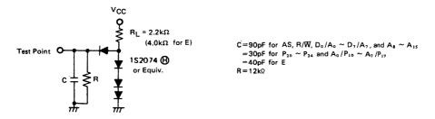
Figure 7 Bus Timing Test Loads (TTL Load)
