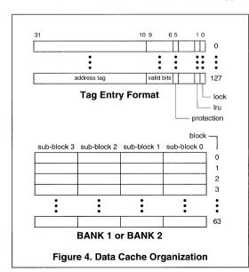
priate cache. This feature gives the flexibility, for example, to assure deterministic response for certain critical interrupt routines by locking the routine's code into the cache. Entries can also be locked where it is desirable to give performance priority to certain often used routines which might otherwise be removed from cache. The 2-way set-associativity allows the cache to perform effectively even with some locked entries.
