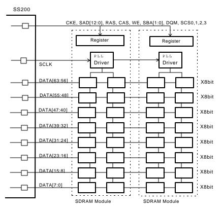
Figure 5-6 Connect with SDRAM DIMM Data
