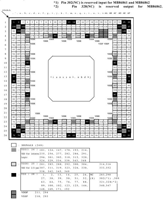
Figure 1.3 Package Pin Assignments
