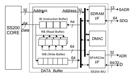
Figure 1.1 SS200 BIU Block Diagram
