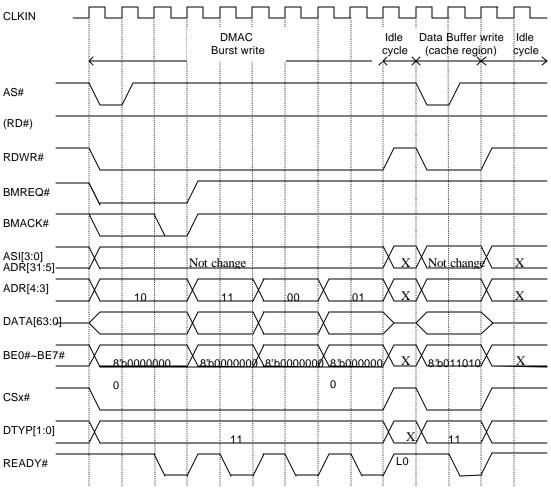
Figure 5-3 SPARClite Bus Burst WRITE Operation (DMA transfer)
