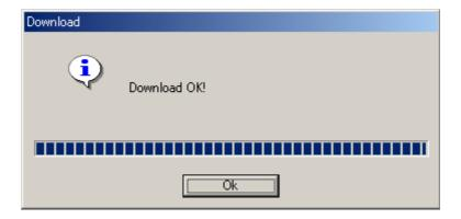
When the [OK] button is clicked to close the dialog window, the [Erase], [Blank Check], [Program & Verify], [Read & Compare] and [Copy] buttons are enabled.
