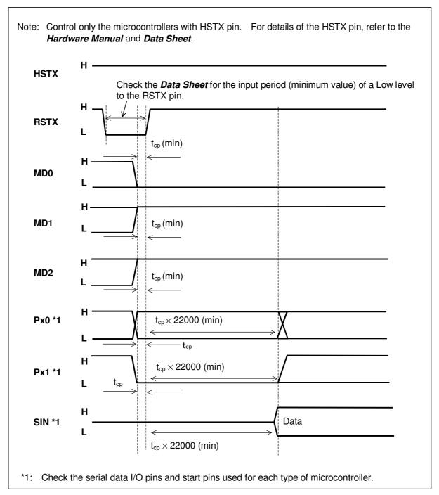
Minimum values of setup and hold times of each signal on rising edge of RSTX
