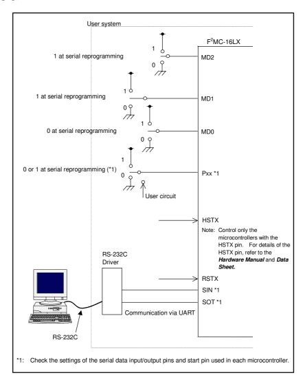
The MD2, MD1, MD0 pins, and Pxx pins cannot be controlled by the PC and should be set in the user system. During serial programming, set the HSTX pin to "High" (only for microcontrollers with the HSTX pin).
