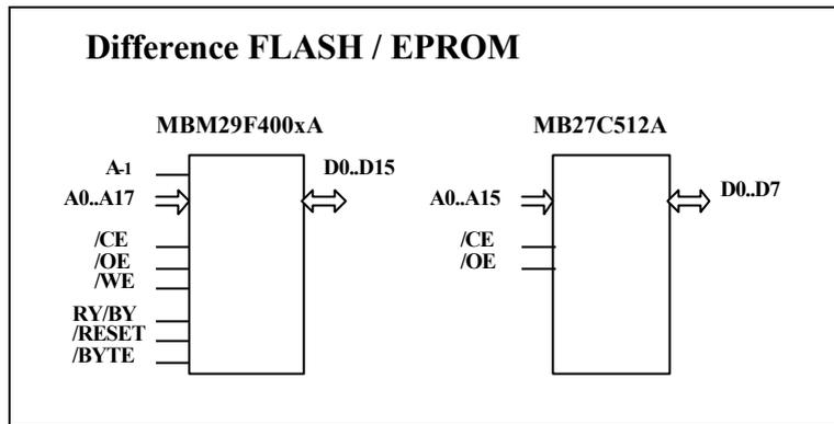
The /BYTE input is used to configure the device to operate in either 8-bit or 16-bit wide mode. If it is configured as an 8-bit memory, the additional address line “A<sub>-1</sub>” is needed to address the complete memory area. As mentioned above, for this application note we assume the 16-bit mode, so “A<sub>-1</sub>” is not used.
