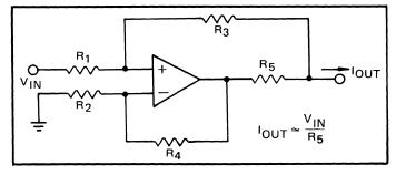
Figure 14. A Voltage-Controlled Current Source Circuit Which Does Not Require External Active Devices.
