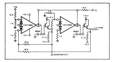
Figure 14. Voltage Controlled State Variable Filter
