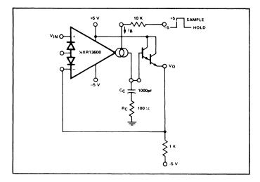
Figure 24. Sample-Hold Circuit
