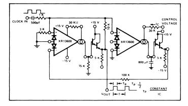
Figure 30. Pulse Width Modulator
