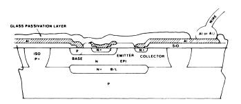
**Typical Bipolar Chip Cross Section**
