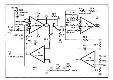
Figure 27. True RMS Converter Circuit
