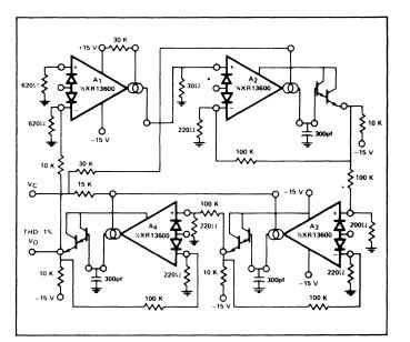
Figure 17. Sinusoidal VCO using two XR-13600 Circuits
