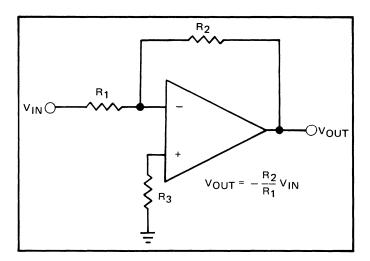
Figure 1. Inverting Amplifier
