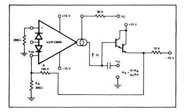
Figure 8. Voltage Controlled Resistor, Single-Ended
