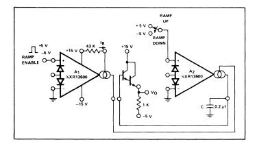
Figure 26. Ramp and Hold Circuit
