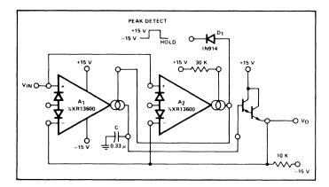
Figure 25. Peak Detector and Hold Circuit
