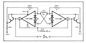
Figure 10. Floating Voltage Controlled Resistor
