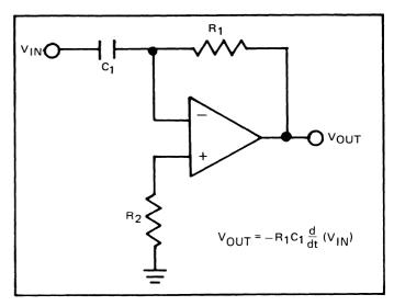
Figure 6. Basic Differentiator Connection
