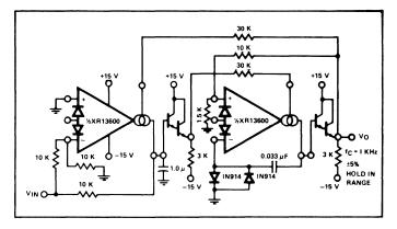
Figure 21. Phase-Locked Loop
