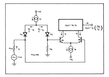
Figure 3. Equivalent VCA Input Circuit
