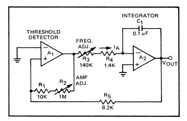
Figure 15. A Simple Triangle Wave Oscillator.
