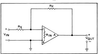
Figure 2. Basic Feedback Configuration Using an Operational Amplifier With Finite Input Impedance and Gain.
