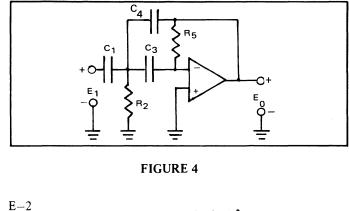
$$\frac{E_0}{E_1}(s) = \frac{-(C_1/C_4)s^2}{s^2 + s(1/R_5)(C_1/C_3C_4 + 1/C_4 + 1/C_3) + 1/R_2R_5C_3C_4}$$
