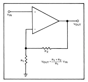
Figure 2. Non-Inverting Amplifier
