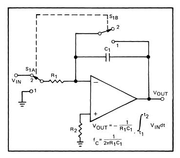
Figure 8. The Integrator Circuit
