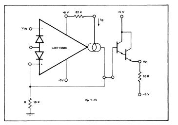
Figure 22. Schmitt Trigger
