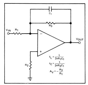
Figure 9. A Simple Low-Pass Filter Circuit
