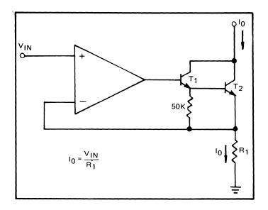
Figure 12. Voltage-Controlled Current-Sink Circuit
