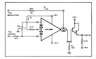
Figure 5. Amplitude Modulator
