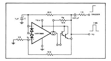
Figure 19. Timer With Zero Stand-By Power
