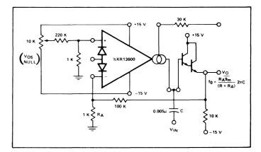
Figure 12. Voltage Controlled High-Pass Filter
