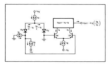
Figure 1. Linearizing Diodes
