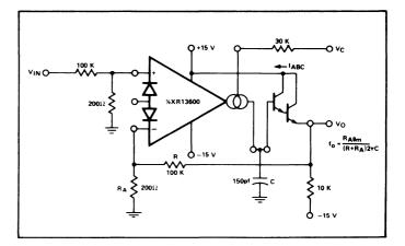
Figure 11. Voltage Controlled Low-Pass Filter
