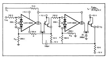
Figure 13. Voltage Controlled 2-Pole Butterworth Low-Pass Filter
