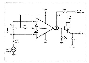
Figure 2. Voltage Controlled Amplifier (VCA) Circuit
