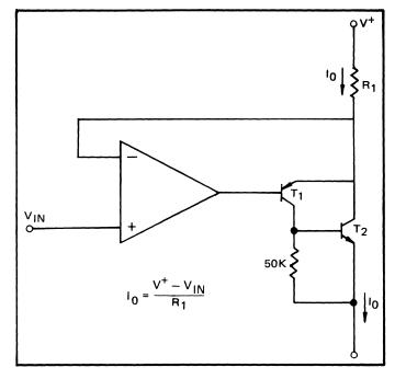
Figure 13. Voltage-Controlled Current-Source Circuit
