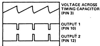
Figure 8. Waveforms for Self-Triggered Operation
