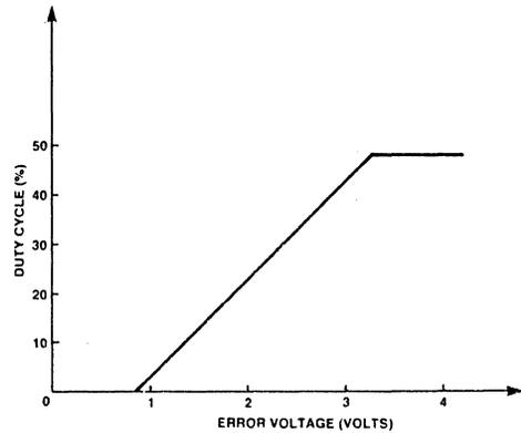
Figure 6. Output Duty Cycle vs Error Voltage
