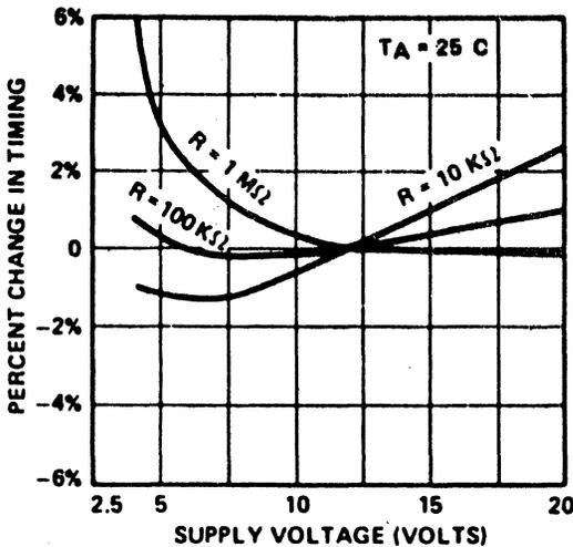
Figure 10. Change in Timing vs. Supply Voltage
