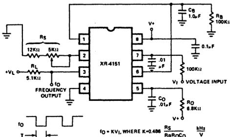
Figure 3. Voltage-to-Frequency Converter
