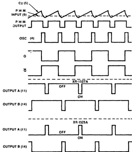
**Figure 1: Typical Waveforms—XR-1525A/1527A**
