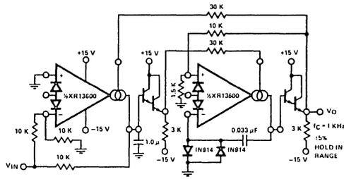
Figure 21. Phase-Locked Loop
