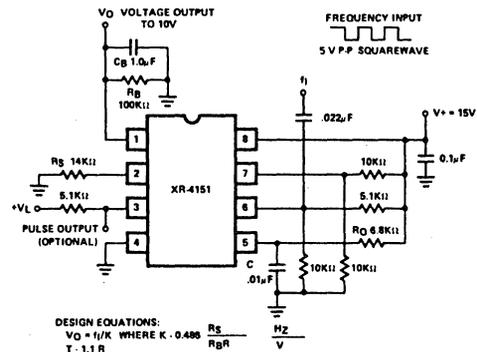
Figure 5. Frequency-to-Voltage Converter
