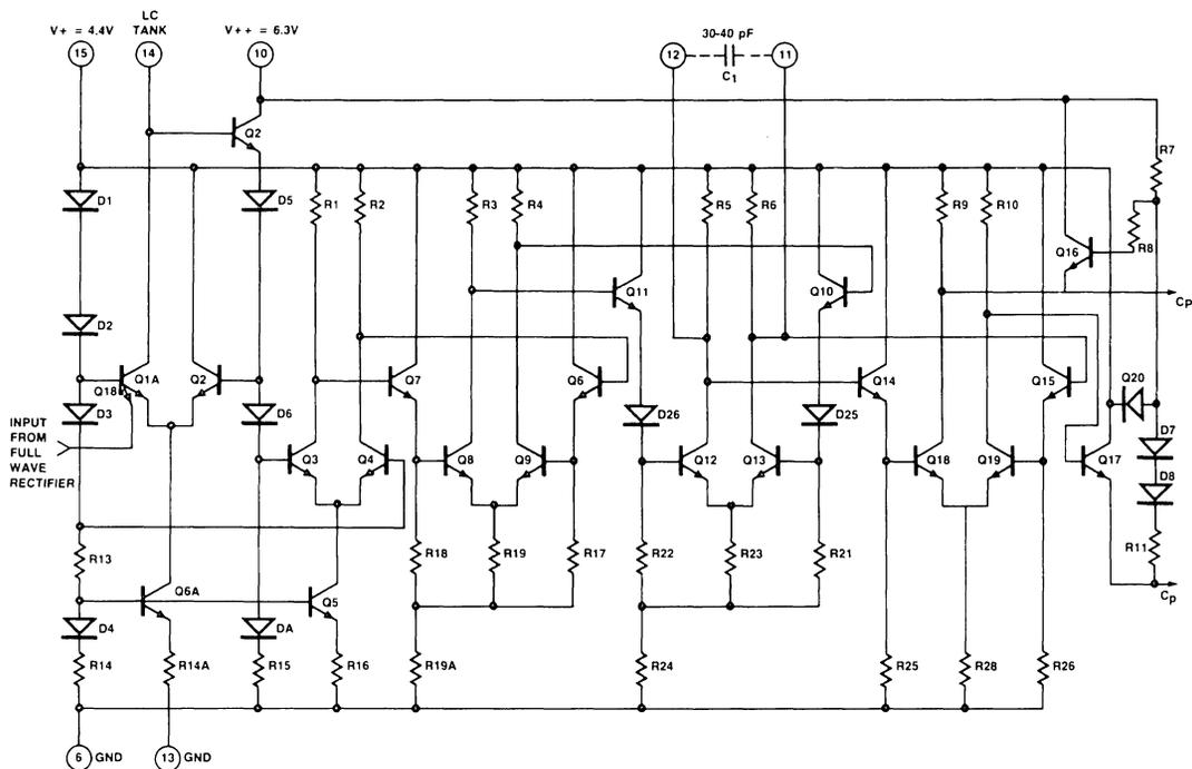
Figure 10. Circuit Diagram of Clock Extractor Section
