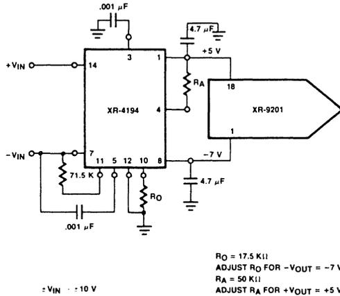
Figure 15. Digital-to-Analog Conversion — Bipolar Operation
