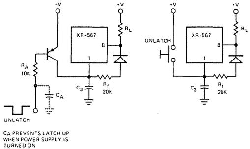
Figure 17. Output Latching
