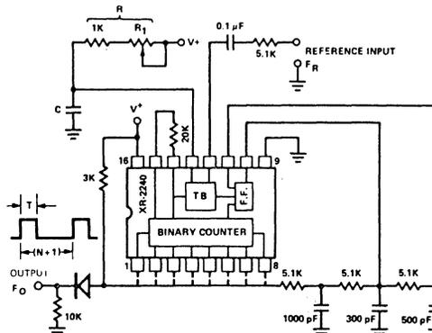
Figure 25. Frequency Synthesis by harmonic Locking to a External Reference
