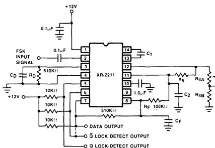
Figure 4: The XR-2211 FSK Demodulator with Carrier Detect
