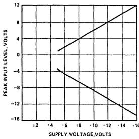
Figure 10. Multiplier Input Dynamic Range vs Power Supply
