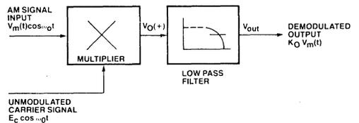
Figure 1 Block Diagram of a Synchronous AM Detector.
