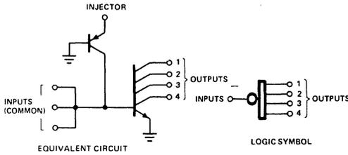
Figure 7. Four-Output I<sup>2</sup>L Gate
