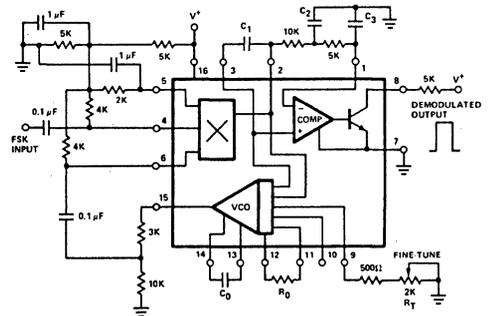
Figure 3. Circuit Connection for FSK Demodulation (Single Supply)
