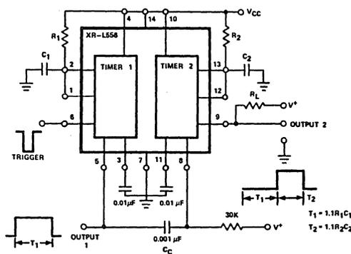
Figure 16. Sequential Timing
