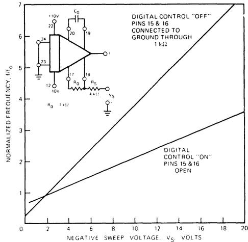
Figure 14. Voltage Sweep Characteristics
