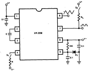
Figure 1. Test Circuit for Split Supply Operation ( $D_1 = 1N4148$  or Equivalent)
