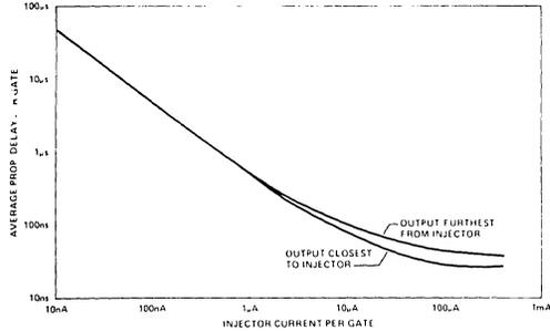
Figure 8. Propagation Delay Characteristics of I<sup>2</sup>L Gates as a Function of Injector Current.
