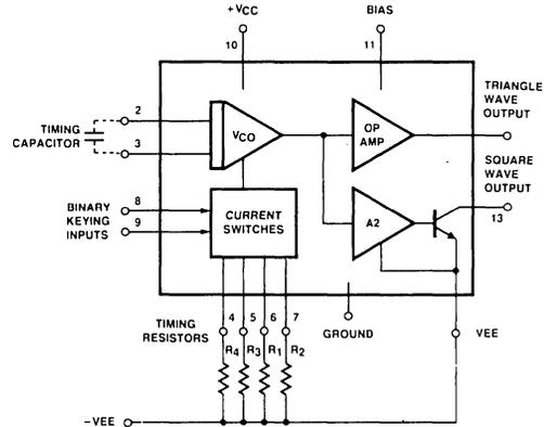
Figure 3. Functional Diagram of XR-2207 Monolithic FSK Generator.
