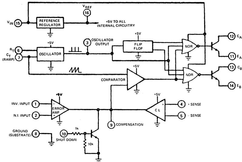
Figure 1. Detailed System Block Diagram of XR-1524
