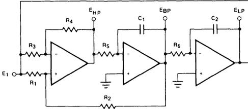
Figure 5. Typical State-Variable Configuration.
