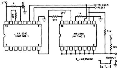
Figure 19. Cascaded Operation for Long Delay Generation
