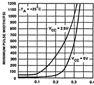
Figure 4. Minimum Pulse-Width Required for Triggering
