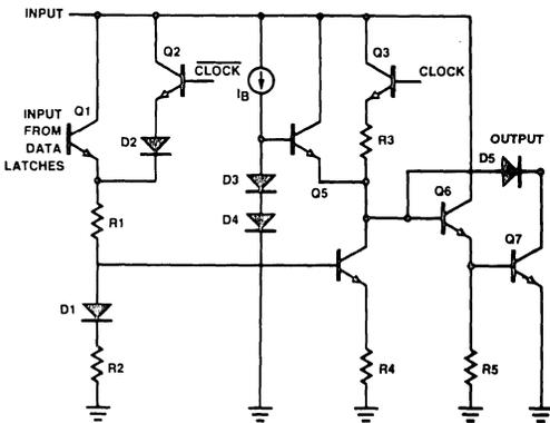
Figure 12. Circuit Configuration for the Output Drivers.
