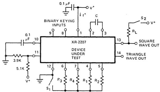
**Figure 1. Test Circuit For Split Supply Operation**
