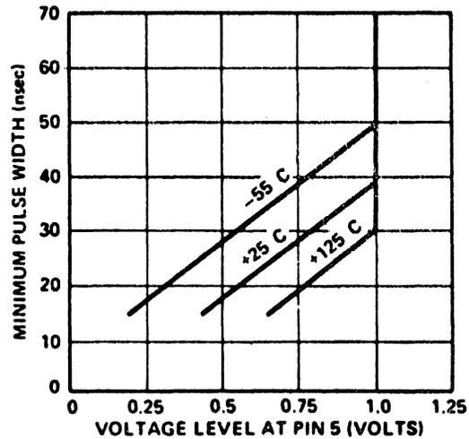
Figure 11. Minimum Pulse Width for Triggering at Pin 5
