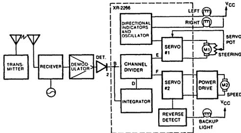
Figure 2. Radio Controlled System Block Diagram
