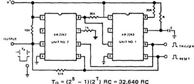
Figure 13. Cascaded Operation of Two XR-2242 Timer Circuits
