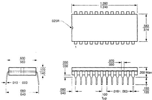
24 PIN CERAMIC CAVITY DIP
