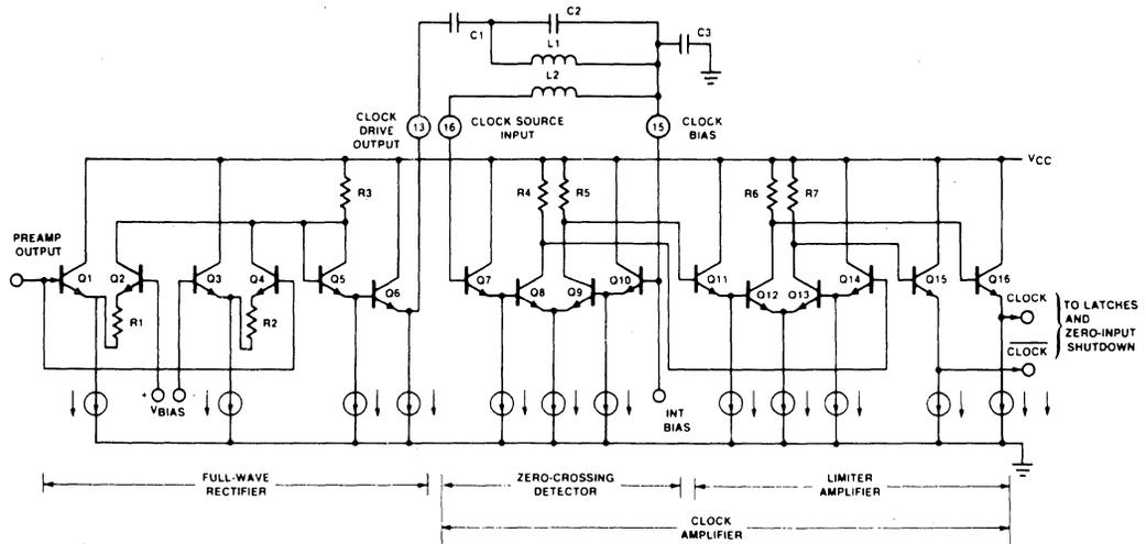
Figure 10. Circuit Diagram of the Clock Recovery Section.
