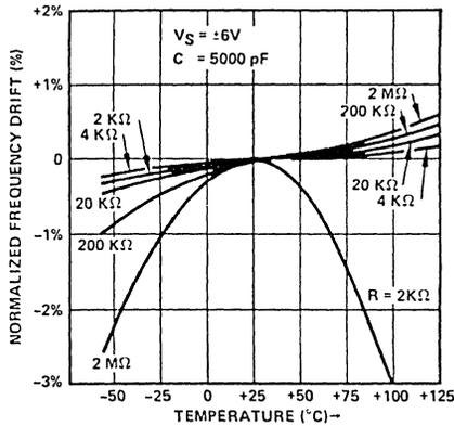
Figure 7. Normalized Frequency Drift With Temperature
