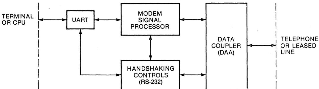
Figure 2. Modem Architecture
