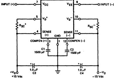
C1 and C2 should be located as close to the device as possible. A  $0.1 \text{ }\mu\text{F}$  ceramic capacitor may be required on the input lines if the device is located an appreciable distance from the rectifier filter capacitors.
