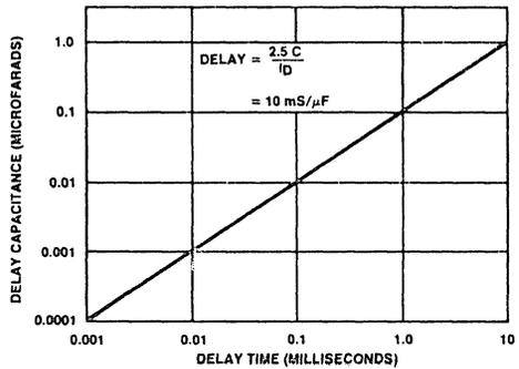
Figure 5. Comparator Activation Delay vs. Capacitor Value
