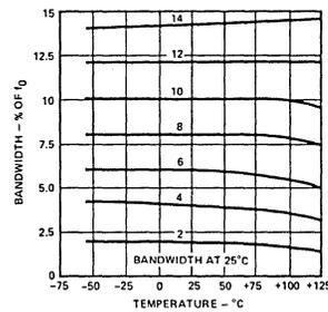
Figure 13. Bandwidth Variation With Temperature
