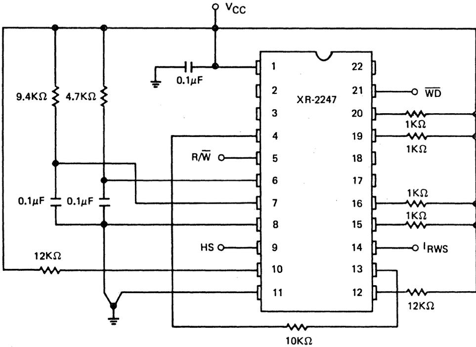
Figure 4. Test Circuit for AC Switching Characteristics
