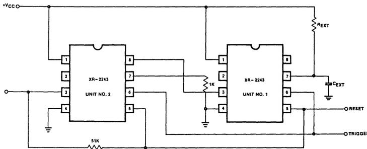
Figure 4. Cascaded Operation of Two XR-2243 Timer Circuits
