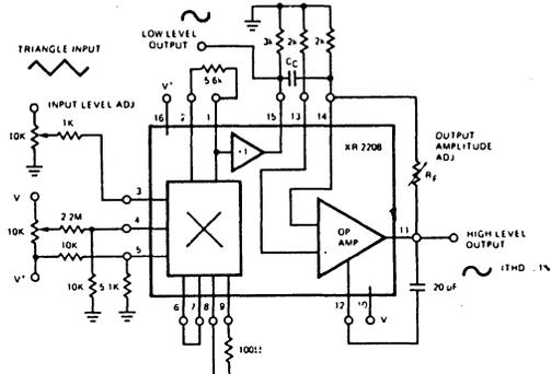
Figure 19. Triangle-to-Sine Converter
