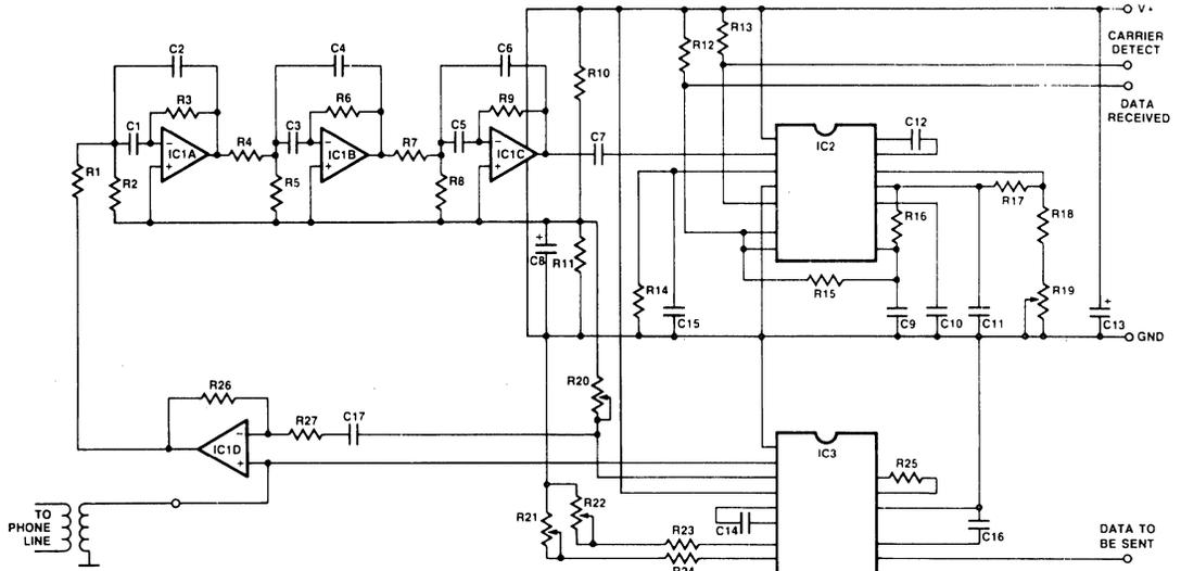
Figure 2. Complete FSK Modem Using XR-2211 and XR-2206.
