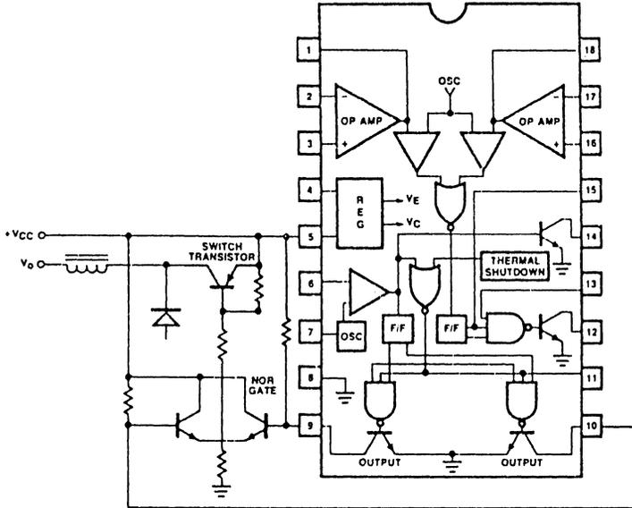
Figure 9. Outputs Nor'd for up to 90% Duty Cycle's
