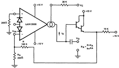
Figure 8. Voltage Controlled Resistor, Single-Ended
