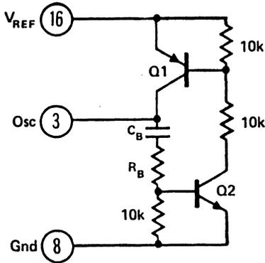
**Figure 12. Recommended External Circuitry for Long Duration Blanking Pulse Generation (Method 3 of Deadband Control).** Note: For 5  $\mu$ sec blanking, choose  $C_B = 200$  pF,  $R_B = 10$  K $\Omega$
