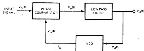
Figure 12. Block Diagram of a Phase-Locked Loop
