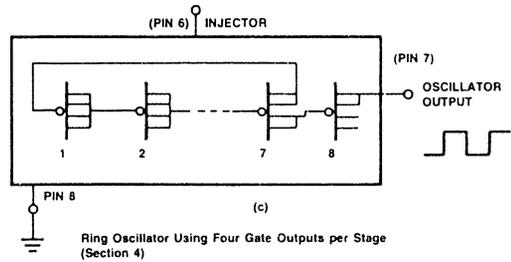
Ring Oscillator Using Four Gate Outputs per Stage (Section 4)
