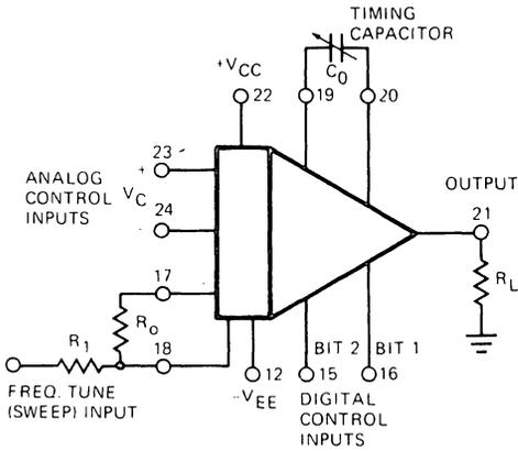
Figure 11. XR-S200 Oscillator Section
