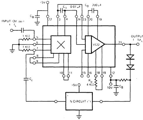
Figure 19. Frequency Synthesizer
