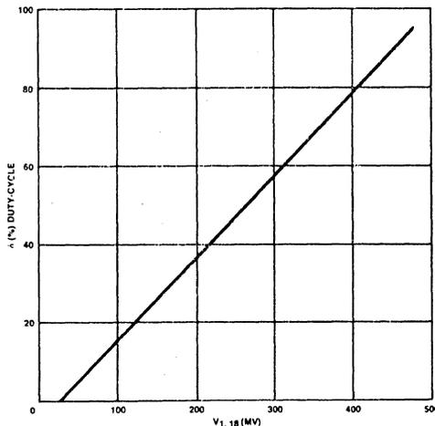
Figure 2. Modulation Duty Cycle vs Error Voltage
