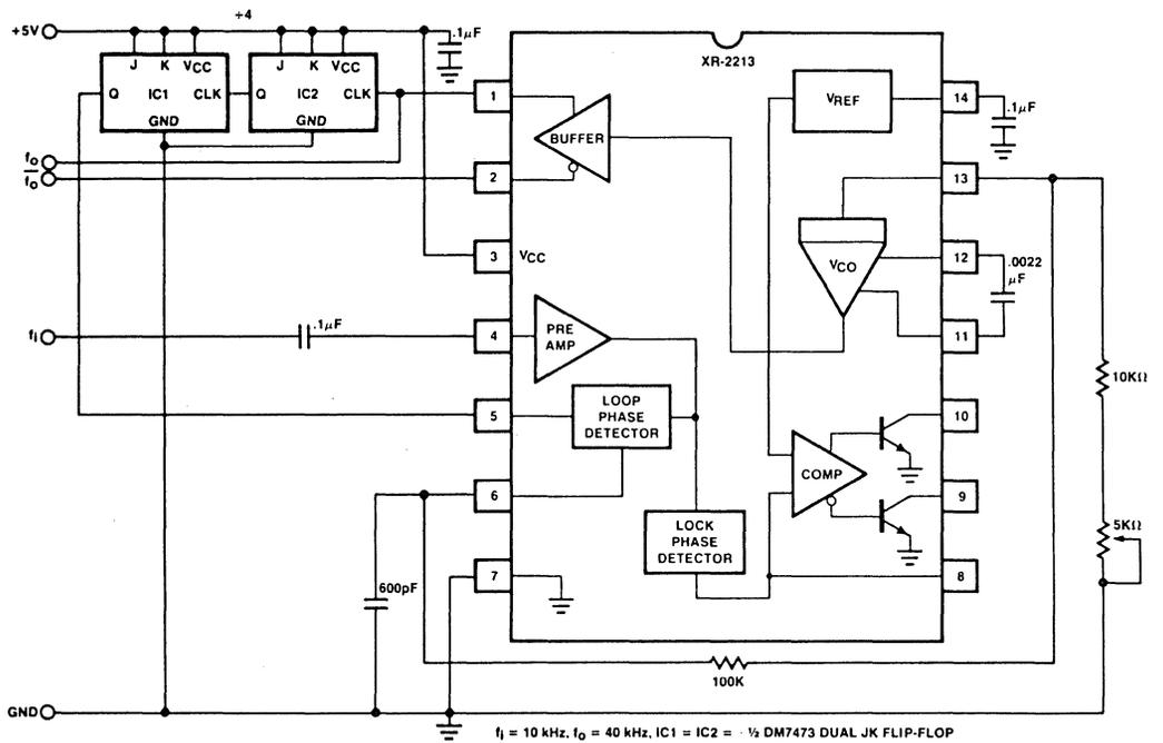
Figure 5. Frequency Synthesizer
