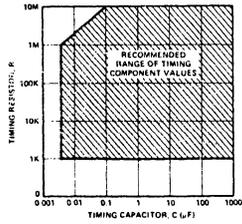
Figure 5. Recommended Range of Timing Component Values
