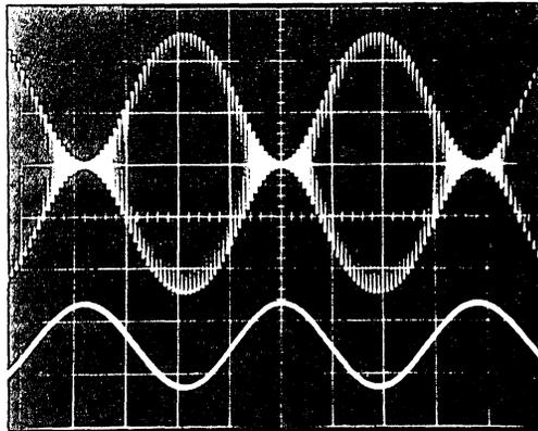
Figure 7-1. AM Modulation, 95% AM,  $f_c = 50$  kHz,  $f_m = 1$  kHz
