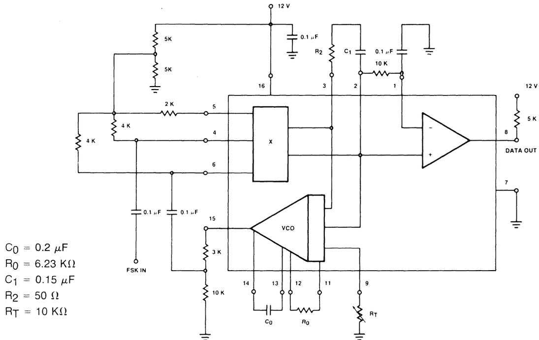
Figure 11. XR-210 FSK Demodulation.
