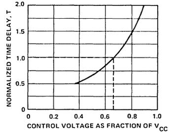
Figure 8. Normalized Time Delay as a Function of Control Voltage
