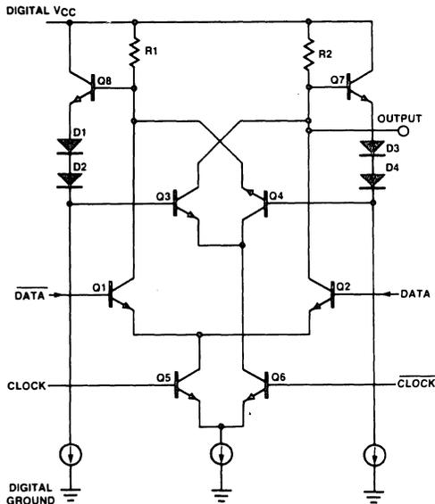
Figure 8. Circuit Configuration for Tracking Data Latches.
