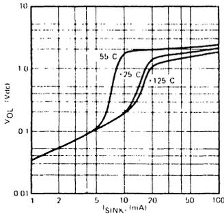
Figure 9. Low Output Voltage
