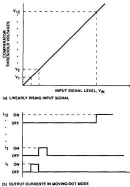
Figure 3. Typical Output Waveforms in Moving-Dot Display Mode
