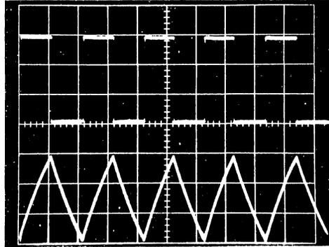
Figure 22. Oscillator Output Waveform Available From CCO Section.
