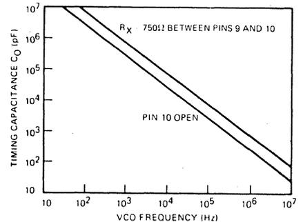
Figure 7. VCO Free Running Frequency vs Timing Capacitor
