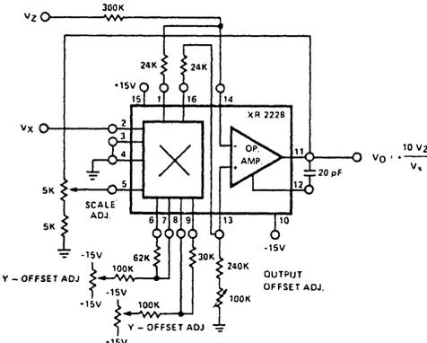
Figure 15. Dividing Circuit
