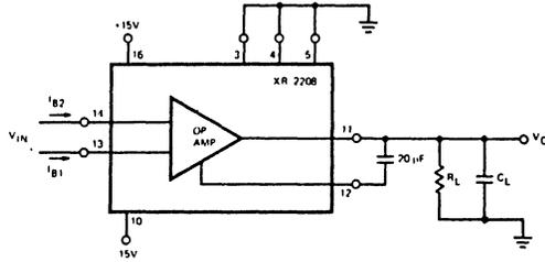
Figure 5. Test Circuit for Op Amp DC Parameters
