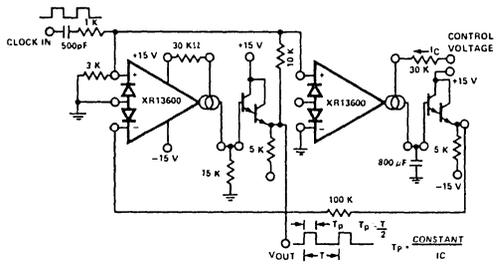
Figure 30. Pulse Width Modulator
