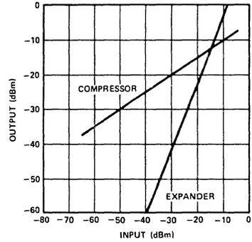
Figure 2. Transfer Characteristics of Compressor and Expander Circuits
