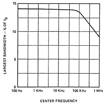
Figure 5. Largest Detection Bandwidth Versus Operating Frequency
