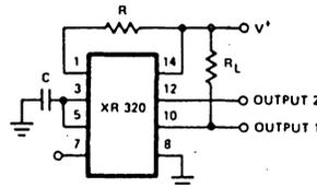
Figure 7. Free-Running Operation
