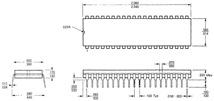
40 PIN CERAMIC CAVITY DIP
