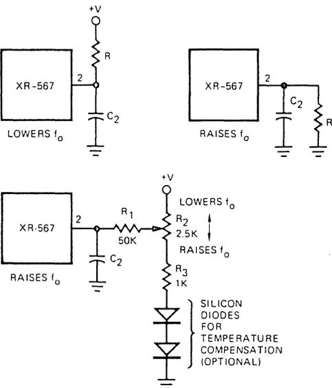
Figure 16. Connections to Reposition Detection Band
