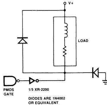
Figure 4. Circuit Connection for Driving Inductive Loads.
