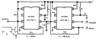
Figure 14. Sequential Timing Using Two XR-2242 Timer Circuits
