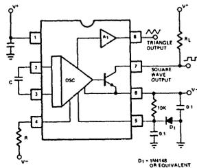
Figure 10. Generalized Circuit Connection for Split Supply Operation
