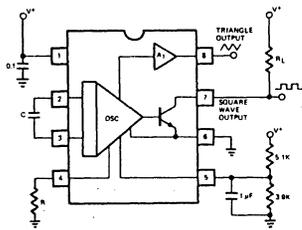
Figure 9. Circuit Connection for Single Supply Operation
