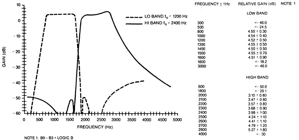
Figure 6. High and Low Band Amplitude Response
