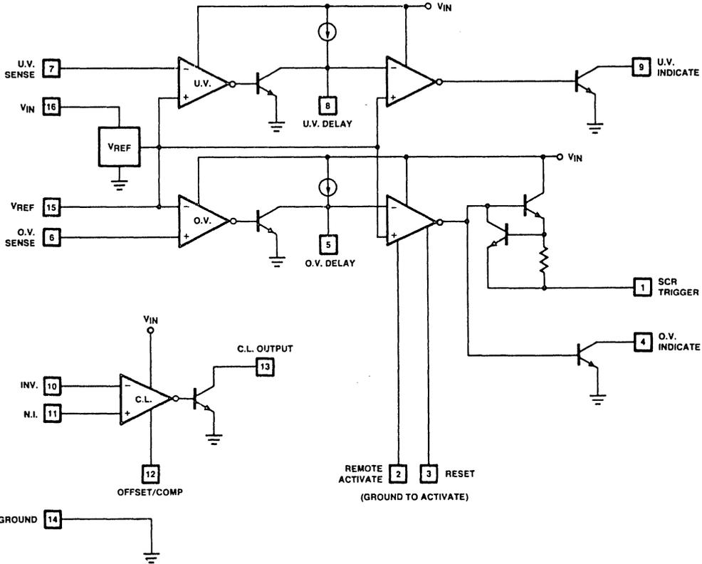
Figure 7. XR-1543 Block Diagram
