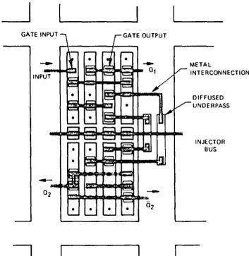
**SAMPLE LAYOUT OF 8 GATE CELL AFTER CUSTOMIZING WITH N<sup>+</sup> COLLECTOR DIFFUSION, CONTACT MASK AND METAL INTERCONNECTION PATTERN**
