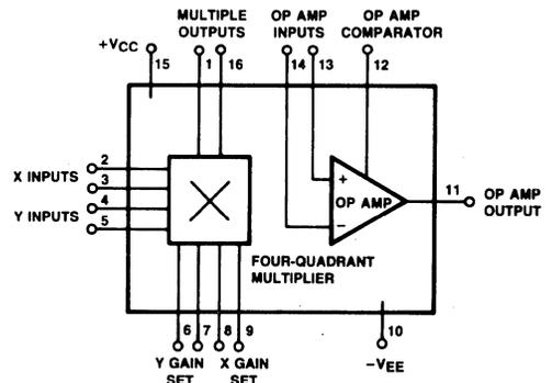
Figure 5. Functional Block Diagram of XR-2228 Multiplier/Detector.
