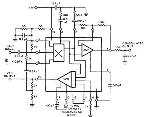
Figure 27. Typical Circuit Connection For Crystal-Controlled FM Detection
