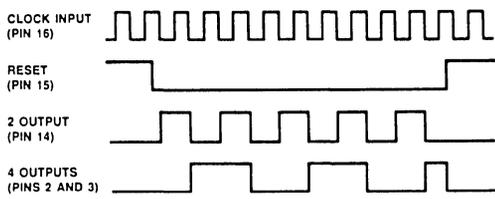
**TIMING DIAGRAM FOR FREQUENCY DIVIDER SECTION**
