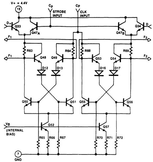
Figure 12. Output-Driver Section
