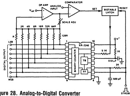
Figure 28. Analog-to-Digital Converter
