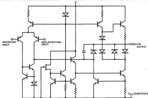
EQUIVALENT SCHEMATIC DIAGRAM
