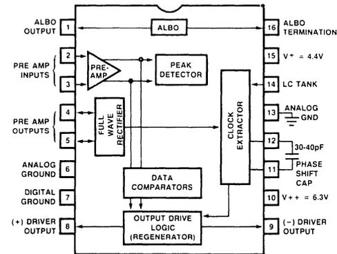
**Figure 3. Package Diagram of XR-C277 Monolithic PCM Repeater**
