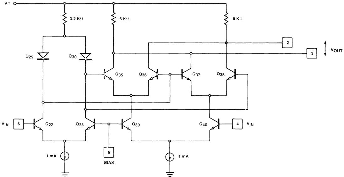
Figure 2. XR-210/XR-215 Phase Comparator.
