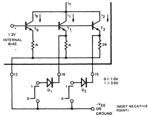
Figure 15. Explanation of VCO Digital Controls
