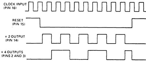
Figure 3. Timing Diagram for Frequency Divider Section.
