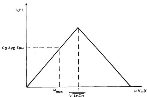
Figure 11. Differentiator Response with  $R_D$ ,  $C_D$ , and  $L$
