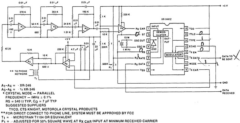
Figure 4. Complete 300 Baud, Answer Mode, FSK Modem
