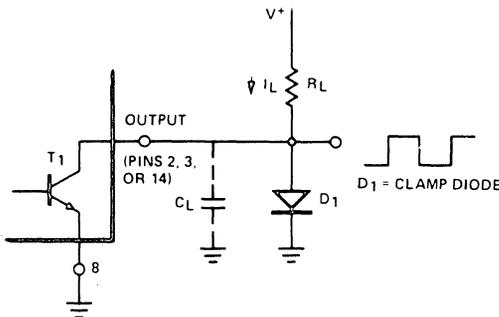
Figure 5. Recommended External Connections to Measure Output Waveforms.
