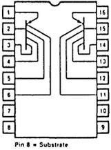
XR-C507 contains two four-collector lateral PNP transistors. These devices are equivalent to the PNP transistors available in the linear section of the XR-400 Master-Chip.
