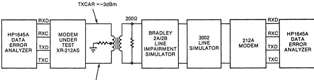
CONDITIONS: RXCAR = -40 dBm, NOISE LEVEL = -52 dBm (S/N = 12 dB), HIGH SPEED MODE (1200 BPS)
