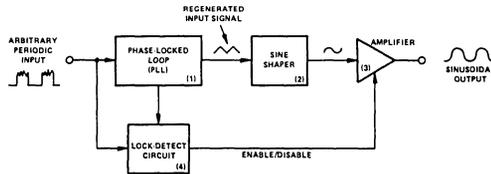
Figure 1. Basic Concept of a Regenerative Sinewave Converter.
