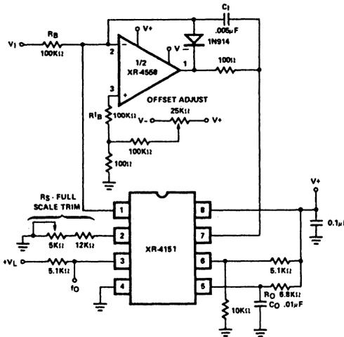
Figure 4. Precision Voltage-to-Frequency Converter
