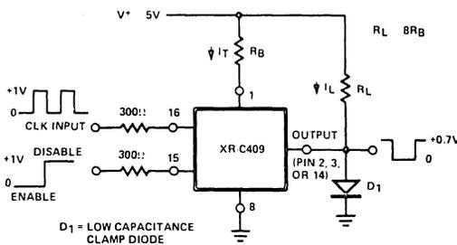
Figure 4. Test Circuit for Frequency Divider Section.
