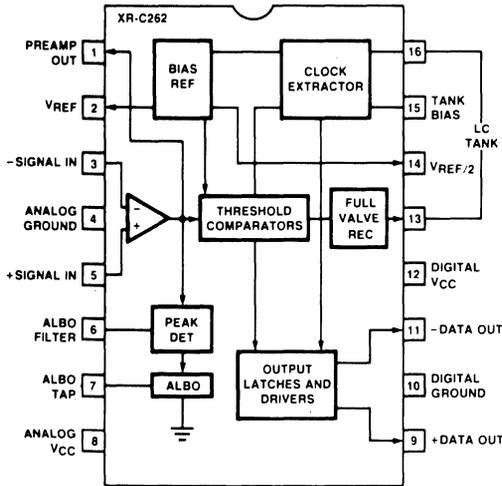
Figure 2. Package Diagram of XR-C262 Monolithic PCM Repeater.
