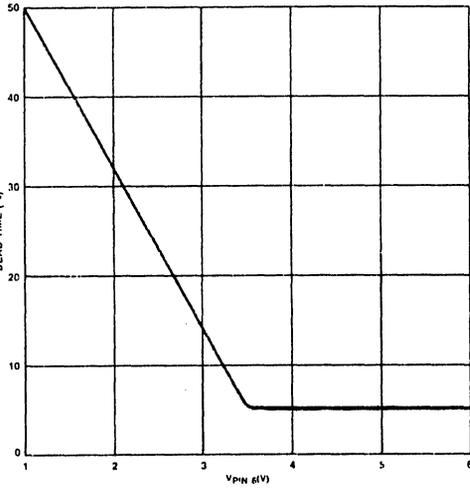
Figure 4. Dead Time vs Dead Time Adjustment Voltage
