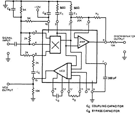
Figure 24. Circuit Connection For Tracking Filter Applications
