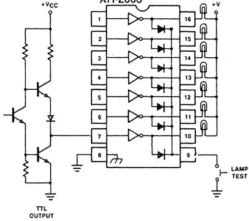
Figure 7. TTL to Load
