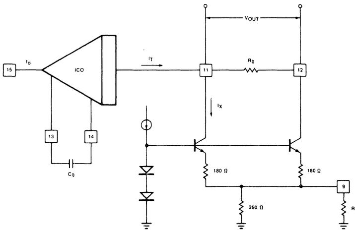
Figure 6. XR-210 Current Controlled Oscillator.
