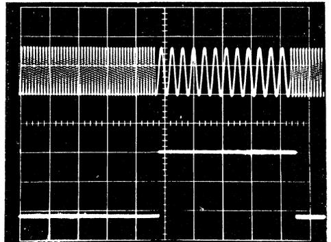
Figure 26. Input and Output Waveforms for FSK Decoding
