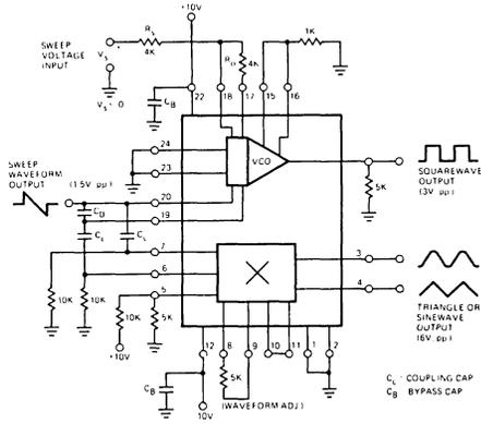
Figure 21. Waveform Generator Typical Circuit Connection Diagram
