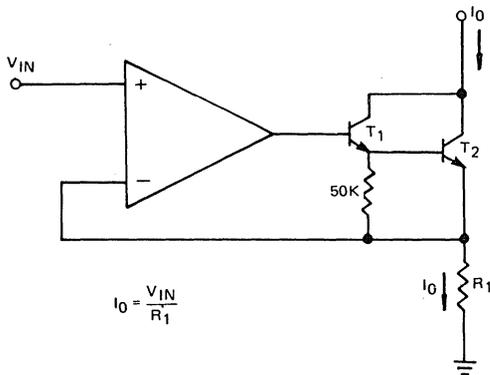
Figure 12. Voltage-Controlled Current-Sink Circuit
