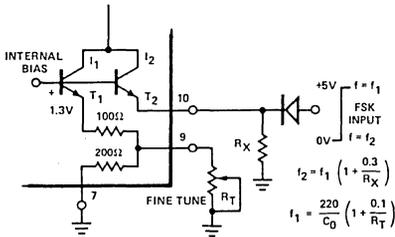
Figure 6. VCO Fine-Tune (Pin 9) and Frequency-Keying (Pin 10) Controls
