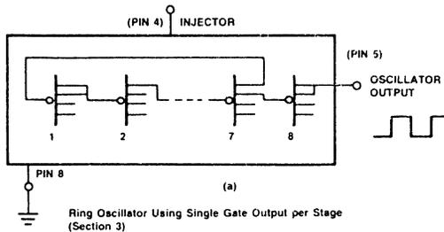
Ring Oscillator Using Single Gate Output per Stage (Section 3)
