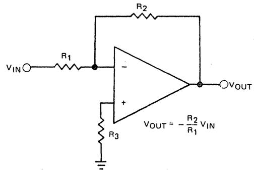
Figure 1. Inverting Amplifier
