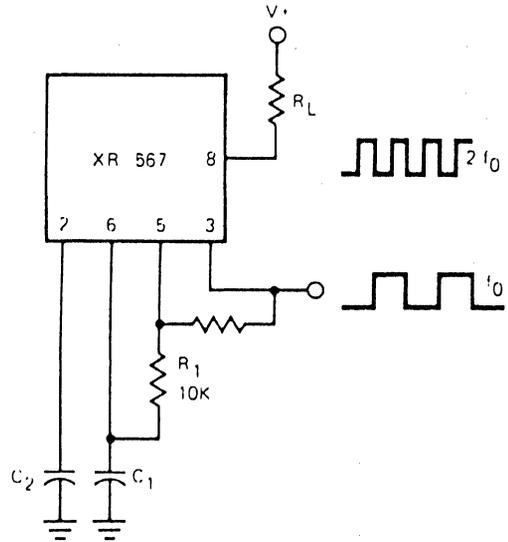
Figure 25. Oscillator with Double Frequency Output
