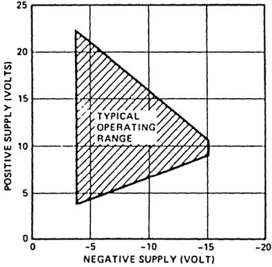
Figure 3. Typical Operating Range For Split Supply Voltage
