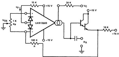
Figure 9. Voltage Controlled Resistor with Linearizing Diodes
