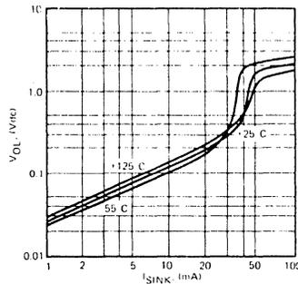
Figure 10. Low Output Voltage
