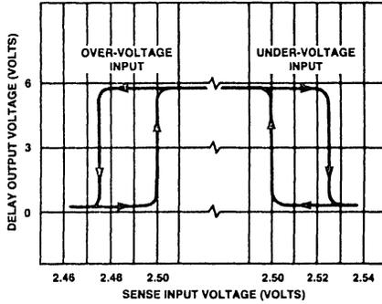
Figure 4. Over-Voltage and Under-Voltage Comparator Hysteresis
