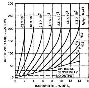
Figure 10. Bandwidth vs. Input Signal Amplitude ( $C_2$  in  $\mu\text{F}$ )
