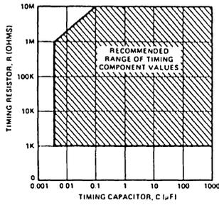
Figure 8. Recommended Range of Timing Component Values.
