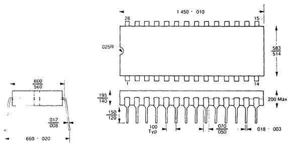
28 PIN CERAMIC CAVITY DIP
