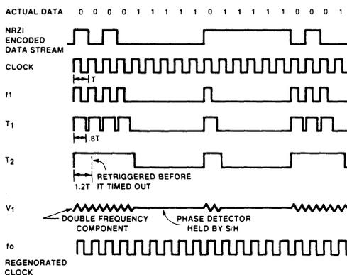
Figure 1. System Timing Diagram.
