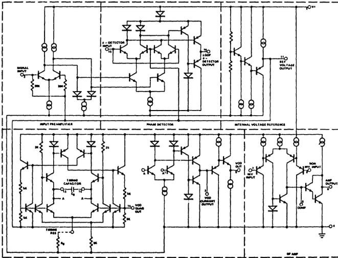
Figure 3. Simplified Circuit Schematic of XR-2212
