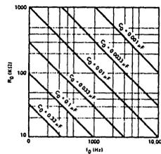
Figure 6. VCO Frequency vs Timing Capacitor
