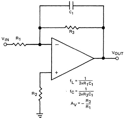
Figure 9. A Simple Low-Pass Filter Circuit
