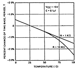
Figure 14. Temperature Drift of Time-Base Period, T
