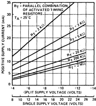
Figure 18. Positive Supply Current, I<sup>+</sup> (Measured at Pin 1) vs. Supply Voltage\*
