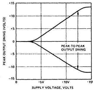
Figure 11. Op Amp Output Swing vs Power Supply
