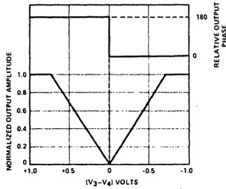
Figure 5. Modular Section Phase and Amplitude Transfer Characteristics
