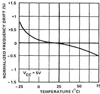
Figure 10. Typical Frequency Stability as a Function of Temperature
