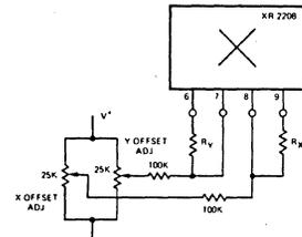
Figure 13. Offset Adjustment
