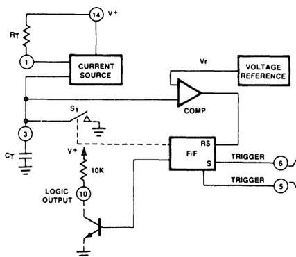
Figure 5. XR-320 Internal Blocks with External Components.
