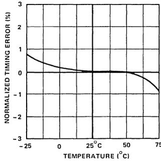
Figure 7. Typical Timing Accuracy as a Function of Temperature
