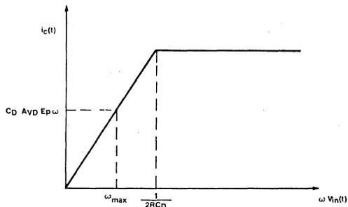
Figure 10. Differentiator Response for  $C_D$  and  $R$
