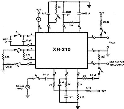
Figure 1. Test Circuits for Single Supply Operation
