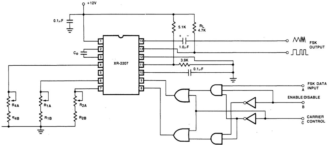
Figure 4. Three-State FSK Transmitter Using the XR-2207.
