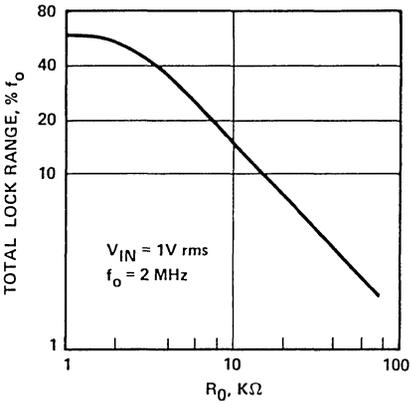
Figure 7. Total Lock Range,  $\pm \Delta f_L$ , versus VCO Gain Control Resistor,  $R_0$
