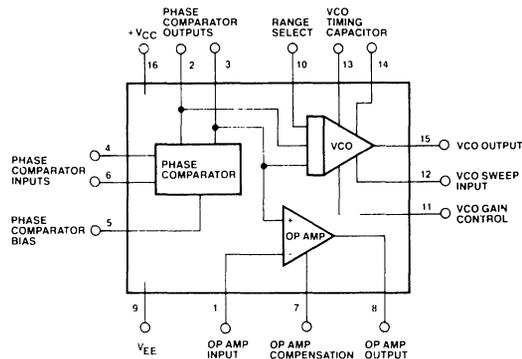
Figure 5. Functional Diagram of XR-215 High-Frequency Phase-Locked Loop.
