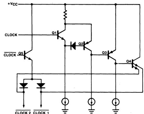
Figure 11. Zero-Input Shutdown Circuit for Output Protection.
