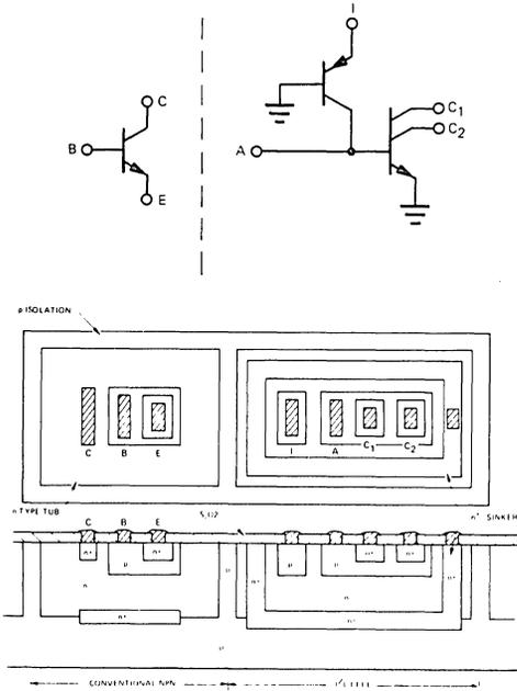
Figure 3. Basic Device Structure for Bipolar Compatible I<sup>2</sup>L.
