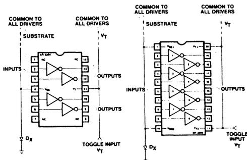
Figure 4. Generalized Connection Diagram XR-2284 and XR-2288.
