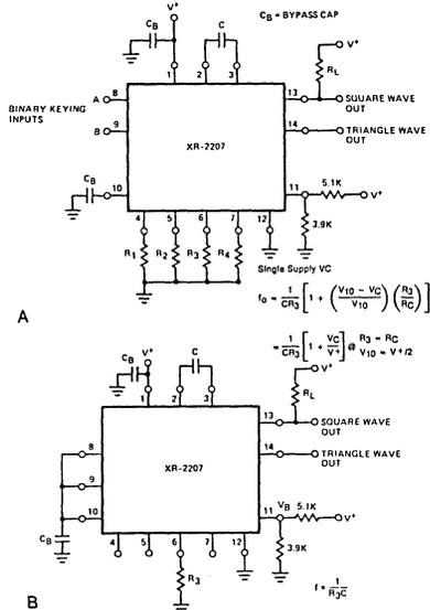
Figure 11. Single Supply Operation:
