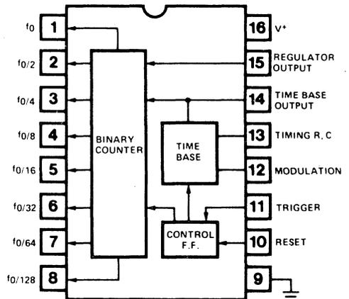
Figure 2. Functional Block Diagram of XR-2240 Counter/Timer.
