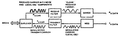
Figure 10. Transmit/Receive Filtering
