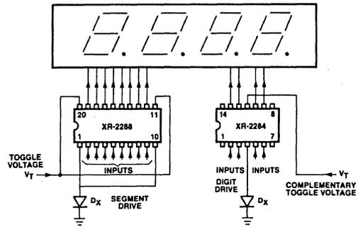
NOTE: EXTERNAL DIODE,  $D_x$  (IN4002 OR EQUIVALENT) SHOULD BE SEPARATE FOR DIGIT AND SEGMENT SIDES
