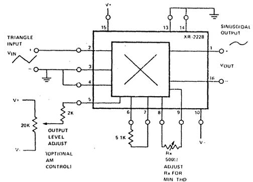
Figure 19. Triangle-to-Sinewave Converter
