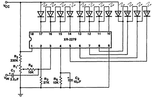
\* $R_1 = 500\Omega =$  CALIBRATION POTENTIOMETER.
