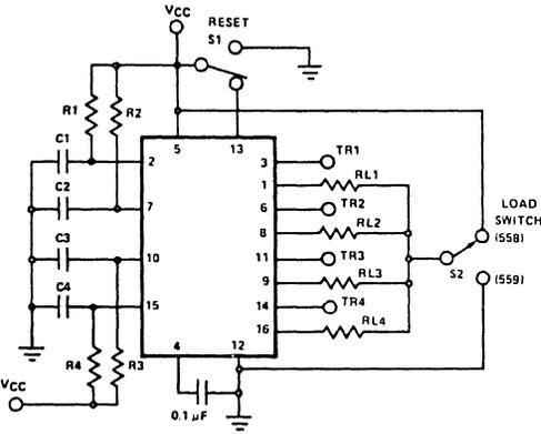
Figure 1. Generalized Test and Evaluation Circuit for XR-558/ XR-559 Quad Timer Circuits
