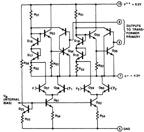
Figure 12. Output Driver Section.
