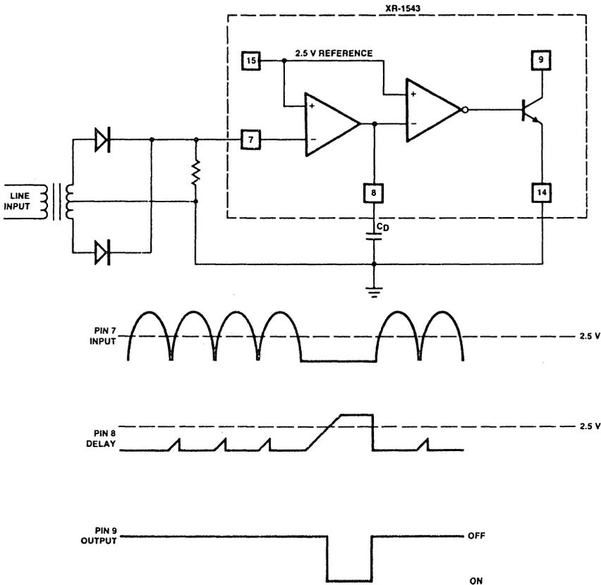
Figure 10. XR-1543—Input Line Monitor Circuit
