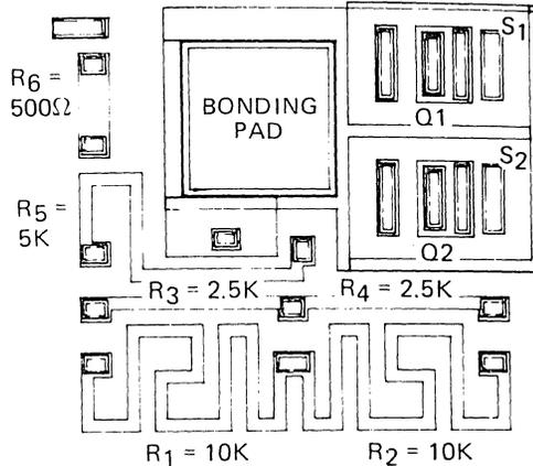
Figure 11. A Typical Schottky-Bipolar Input/Output Interface Cell.
