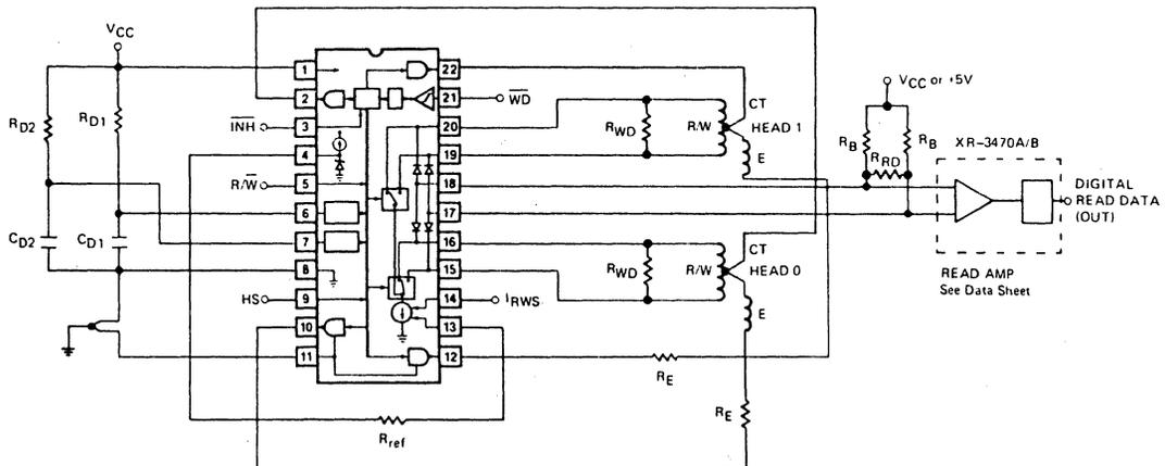
Figure 5. Typical Dual Head Floppy Disk System
