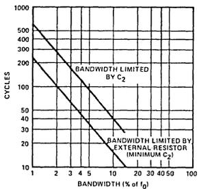
Figure 11. Greatest Number of Cycles Before Output
