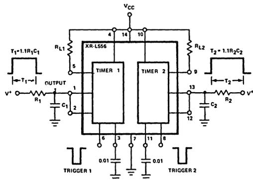
Figure 15. Generation of Two Independent Time Delays
