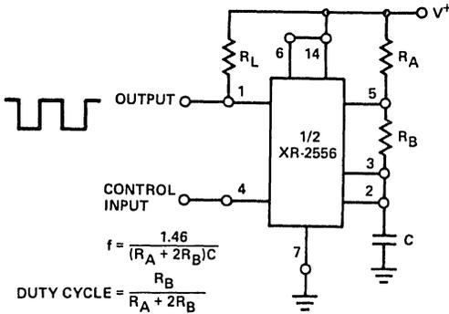
Figure 15. Astable (Free-Running) Circuit
