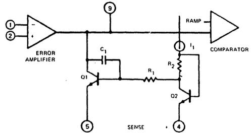
Figure 7. Current Limiting Circuitry of the XR-1524
