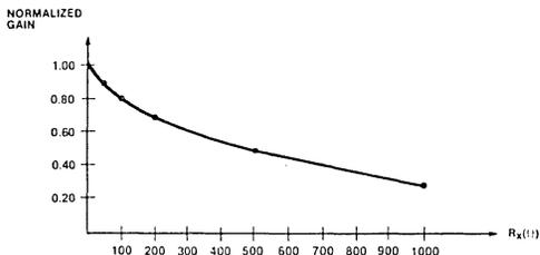
Figure 8. Normalized Gain vs  $R_x$  for Amplifier Stage
