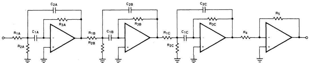
Figure 8. Modem Filter.
