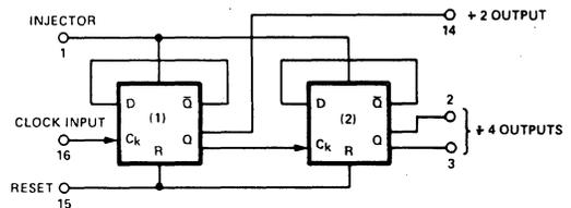
Figure 2. Block Diagram of Frequency Divider Section.
