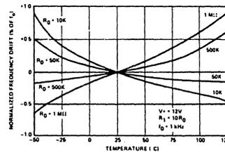
Figure 8. Typical Center Frequency Drift vs Temperature
