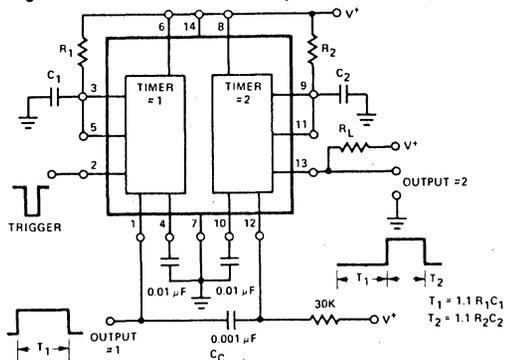
Figure 21. Sequential Timing
