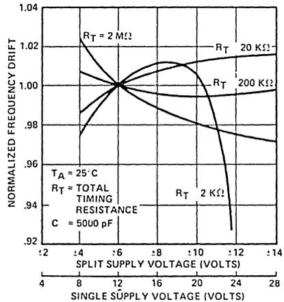
Figure 6. Frequency Drift vs. Supply Voltage
