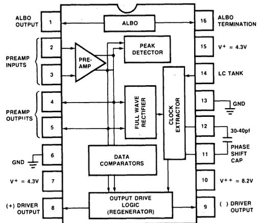
Figure 3. Package Diagram of XR-C240 Monolithic PCM Repeater.
