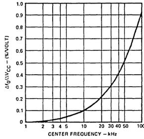
Figure 6. Power Supply Dependence of Center Frequency
