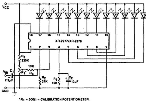
\*  $R_1 = 500\Omega$  = CALIBRATION POTENTIOMETER.
