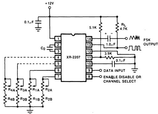
Figure 2. The XR-2207 FSK Modulator Single-Supply Operation.
