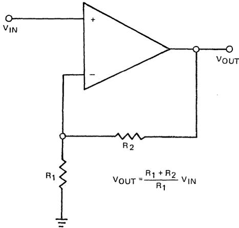
Figure 2. Non-Inverting Amplifier
