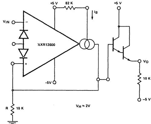
Figure 22. Schmitt Trigger
