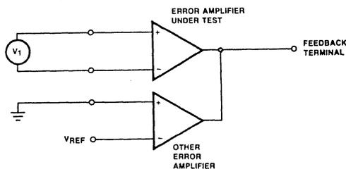
Figure 3. Error-Amplifier Characteristics
