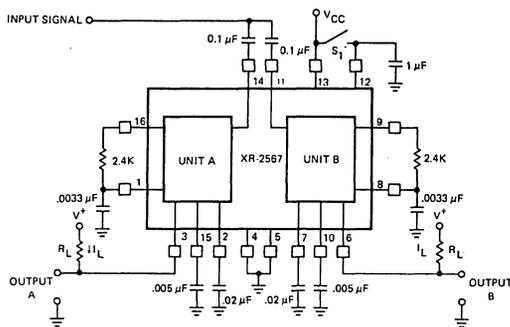
Figure 2. Test Circuit
