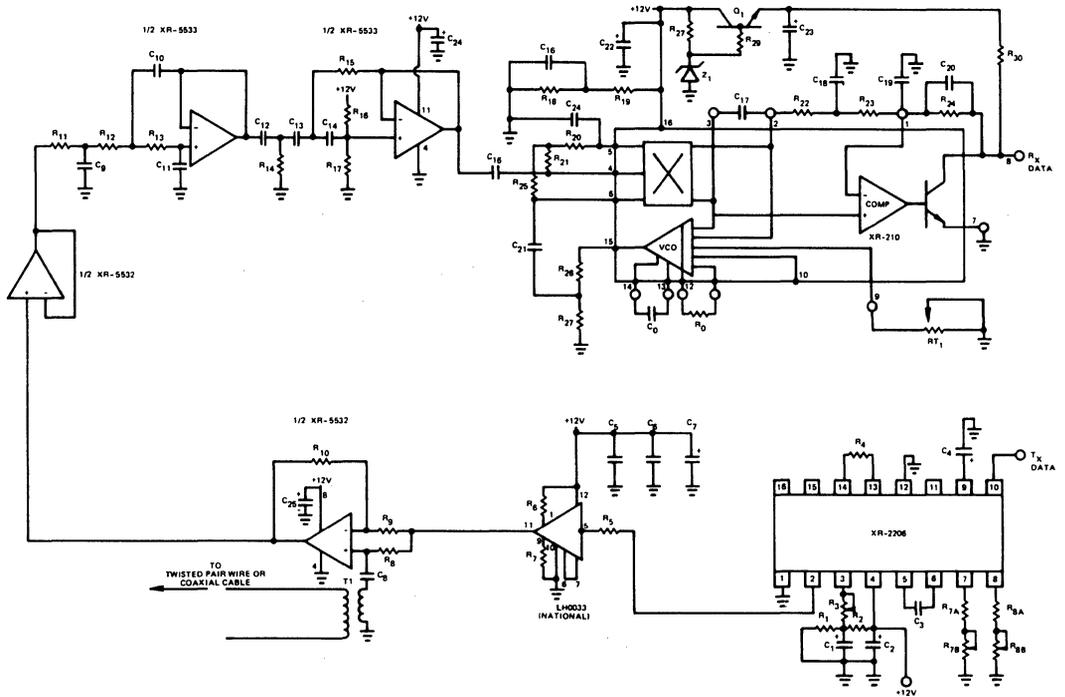
Figure 6. Complete Schematic for 100 Kilobaud FSK Modem
