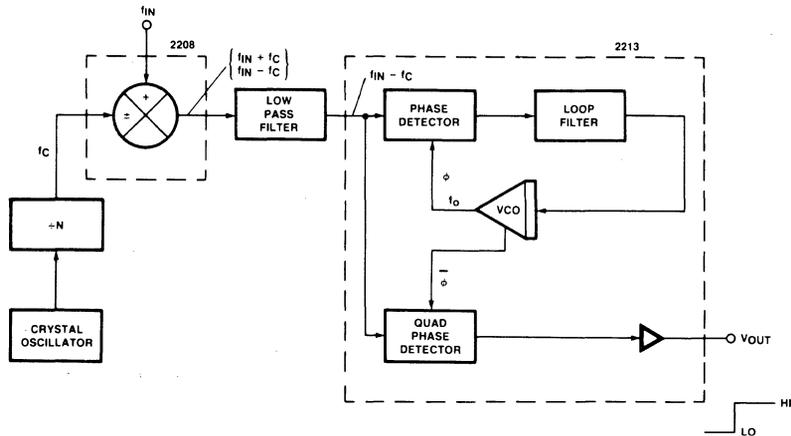
Figure 1. Functional Diagram of Narrow Band Tone Decoder.
