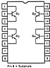
XR-C506 contains four small signal NPN transistors. These are equivalent to the transistors available in the linear section of the XR-400 Master-Chip.
