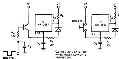
Figure 20. Output Latching
