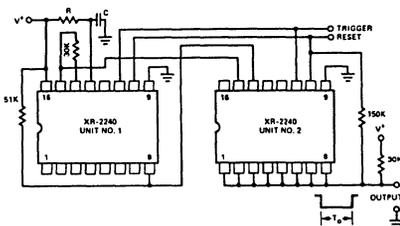
Figure 20. Low-Power Operation of Cascaded Timers
