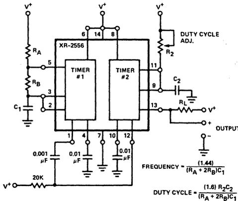
**Figure 26. Fixed Frequency Oscillator With Variable Duty Cycle**
