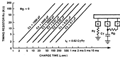
**Figure 2: Oscillator Charge Time vs  $R_T$  and  $C_T$**
