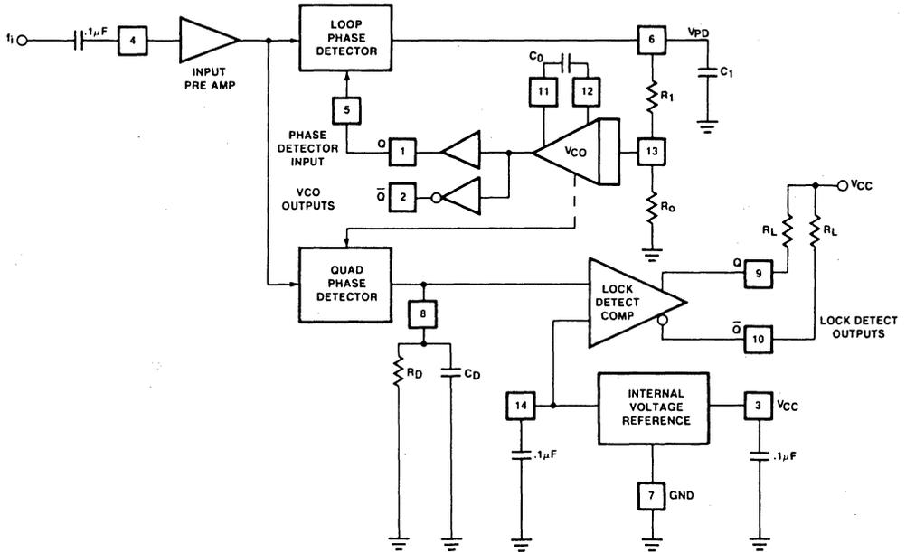
Figure 2. Generalized Circuit Connection for Tone Detection
