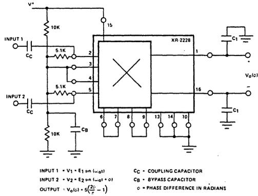
Figure 16. Phase-Detector Circuit
