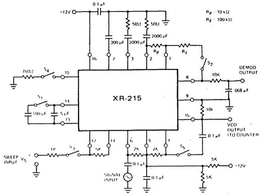
Figure 2. Test Circuit For Single Supply Operation
