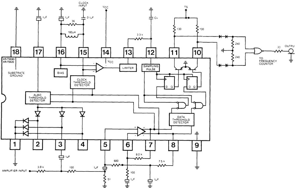
Figure 4. Sampling Pulse Test Circuit
