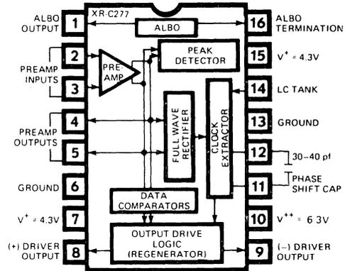
ating at 1.544 M bit/s. It can operate on either pulp or plastic insulated twisted pair cables. Although the cable gauge may vary the total cable loss should not exceed 36 dB at 772 kHz. For a 22 gauge pulp insulated cable and a bit error rate (BER) of less than  $10^{-6}$  the max allowable repeater to repeater spacing is about 6300 feet.
