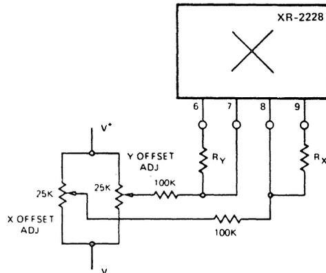
Figure 13. Offset Adjustment
