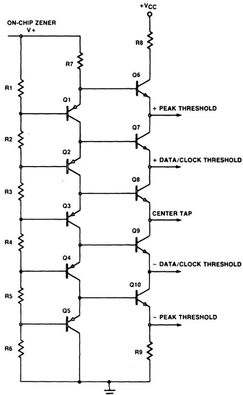
Figure 9. Internal Voltage-Divider Network for Comparator Threshold Setting.
