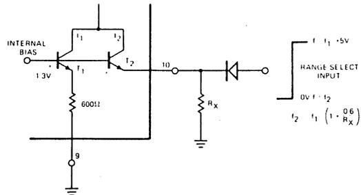
Figure 11. Explanation of VCO Range-Select Controls
