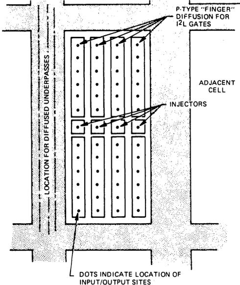
Figure 5. Basic 8-Gate Cell Before Customization.
