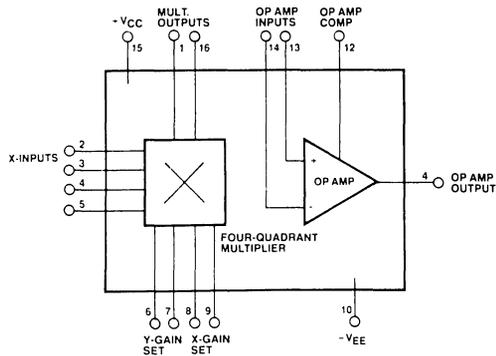
Figure 4. Functional Block Diagram of XR-2228 Multiplier/Detector IC.
