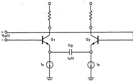
Figure 9. Simplified Active Differentiator Section
