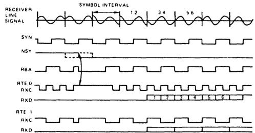
Figure 2. Timing Diagram of the Receiver
