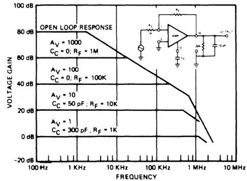
Figure 10. Amplifier Section Frequency Response
