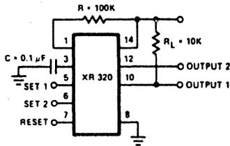
Figure 1. Test Circuit
