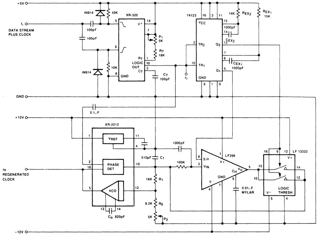
$P_1 =$  ADJUST SO POSITIVE PORTION OF  $f_i$  IS EQUAL TO  $\frac{1}{2}$  OF THE CLOCK PERIOD
