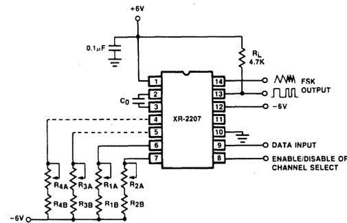
Figure 3. The XR-2207 FSK Modulator Split-Supply Operation.
