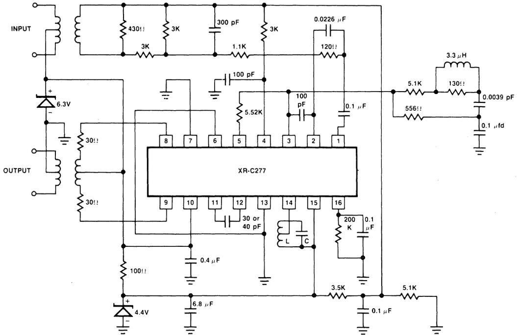
Figure 6. Typical Circuit Connection of XR-C277 in 1.544 MHz T-1 Repeater System. (Note: Set L and C to Form a High Q Tank Resonant at 1.544 MHz. It is Recommended that  $Q \geq 100$ , and  $C \approx \text{pF}$  for most applications).
