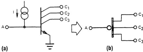
Figure 2. Equivalent Circuit (a), and a Recommended Symbol (b) for an I<sup>2</sup>L Gate.
