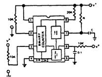
Figure 12. Free-running Operation Self-Triggered When Power Supply is Turned On
