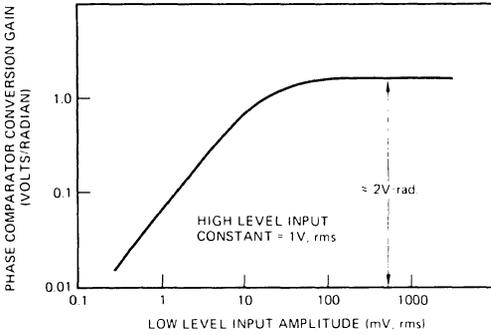
Figure 5. Phase Comparator Conversion Gain Versus Input Amplitude
