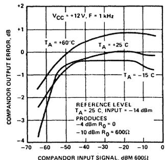
Figure 7. XR-2216 Compressor Tracking Error vs. Input Signal
