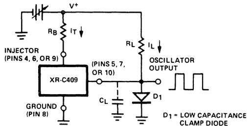
Figure 9. Recommended Test Circuit for Evaluating Power-Delay Characteristics of I<sup>2</sup>L Gates Using Ring Oscillator Sections of XR-C409.
