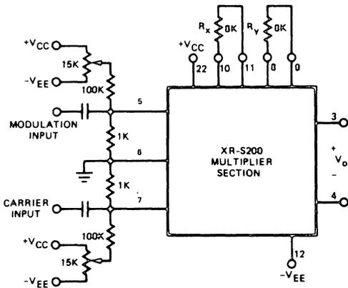
Figure 6. Suppressed Carrier Modulation Using XR-S200 Multiplier Section
