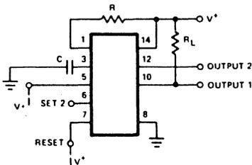
Figure 3. Monostable Operation, Positive Trigger
