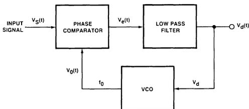
Figure 1. Block Diagram of a Phase-Locked Loop.
