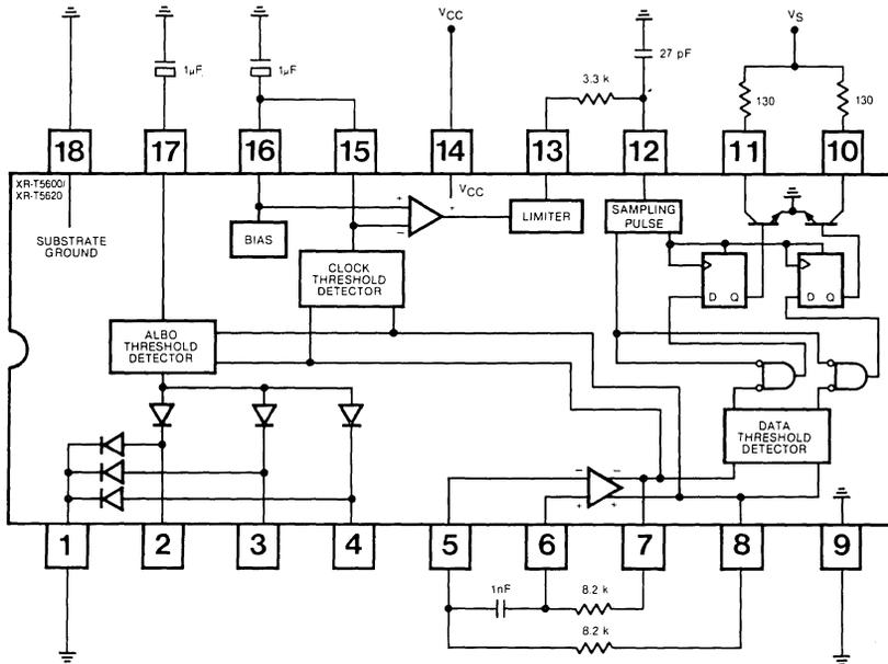
Figure 2. D.C. Parameter Test Circuit
