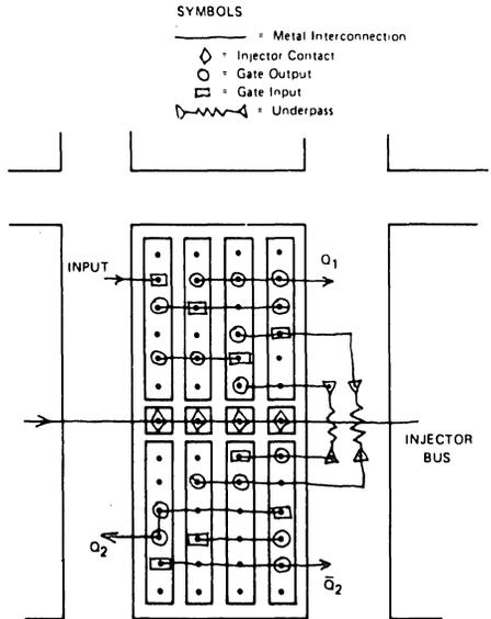
Figure 6. Sample Pencil Layout on a Logic Cell.
