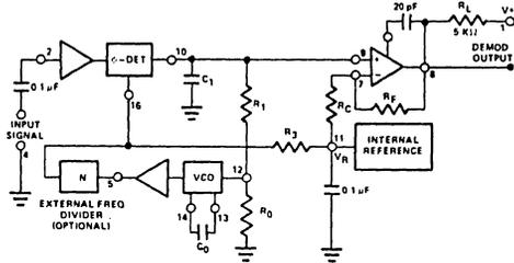
Figure 2. Generalized Circuit Connection for FM Detection, Signal Tracking or Frequency Synthesis
