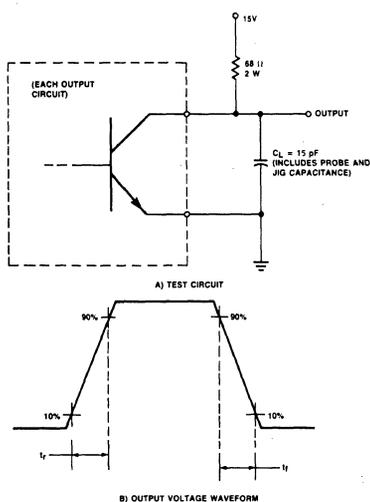
Figure 1. Common-Emitter Configuration
