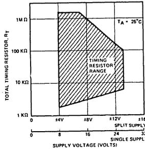
Figure 4. Recommended Timing Resistor Value vs. Power supply Voltage\*
