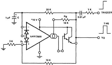
Figure 19. Timer With Zero Stand-By Power
