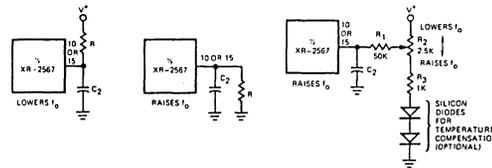
Figure 19. Connections to Reposition Detection Band
