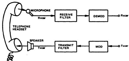
**Figure 14. Acoustical Coupling**
