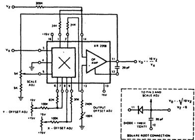
Figure 16. Dividing Circuit
