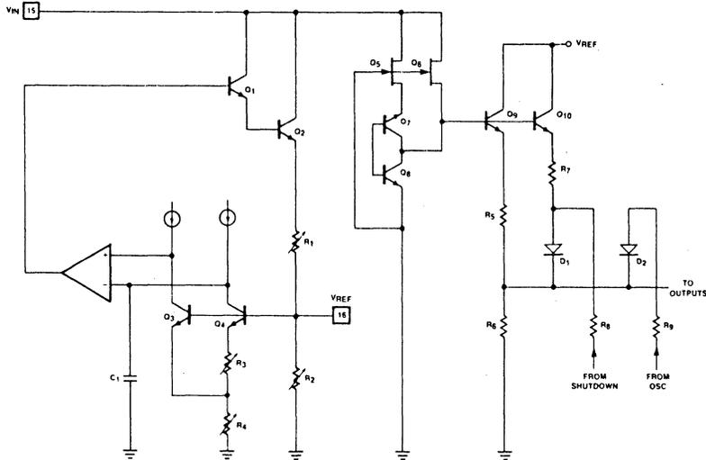
Figure 7. Equivalent Schematic of Voltage Reference Section
