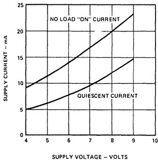
Figure 4. Supply Current Versus Supply Voltage
