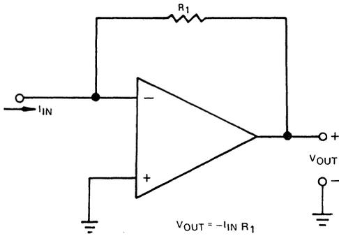
Figure 11. Operational Amplifier as a Current-to-Voltage Converter
