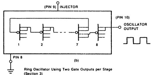
Ring Oscillator Using Two Gate Outputs per Stage (Section 3)
