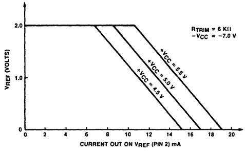
Figure 5. V<sub>REF</sub> vs. Current Output
