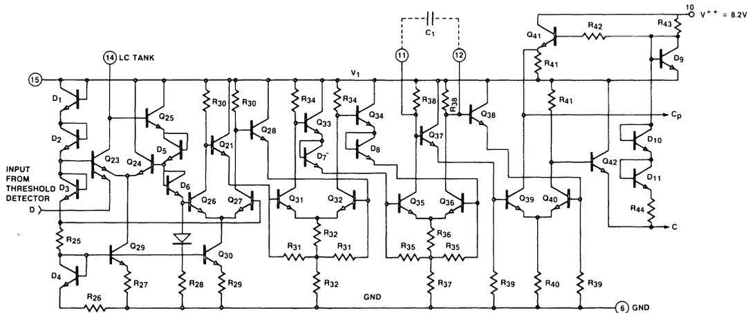
Figure 10. Circuit Diagram of Clock Extractor Section.
