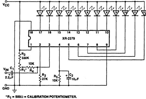
\* $R_1 = 500\Omega =$  CALIBRATION POTENTIOMETER.
