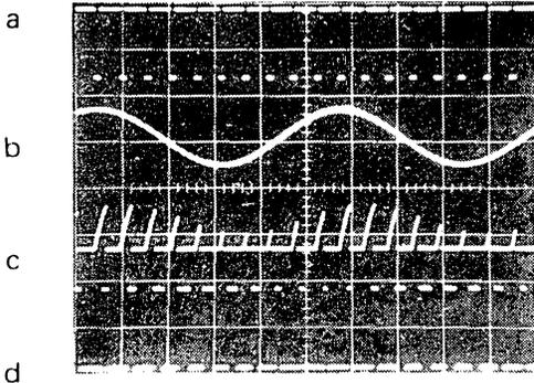
Figure 28. Pulse-Width Modulation Waveforms
