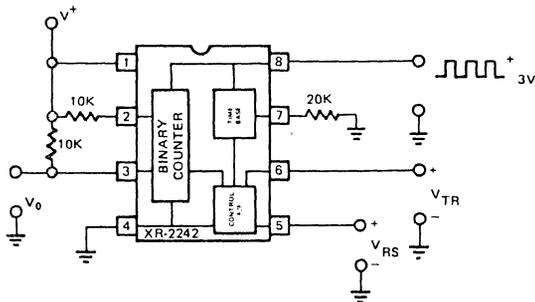
Figure 3. Generalized Test Circuit
