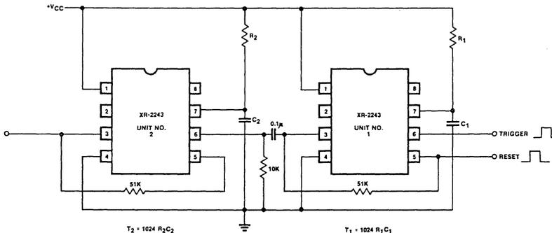
Figure 5. Sequential Timing Using XR-2243 Timer Circuits
