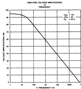
Figure 6. Amplifier Voltage Amplification vs Frequency
