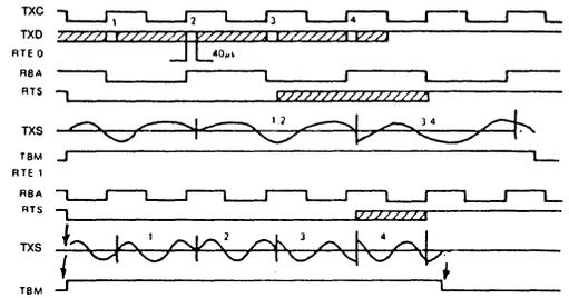
Figure 1. Timing Diagram of the Transmitter
