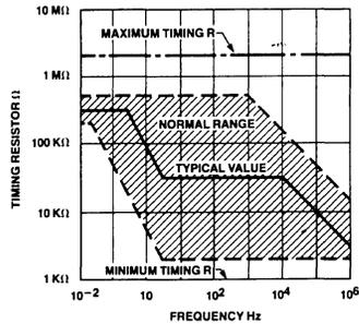
Figure 4. R versus Oscillation Frequency.
