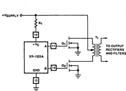
Figure 13. Push-Pull Outputs with XR-1525A
