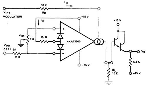
Figure 5. Amplitude Modulator
