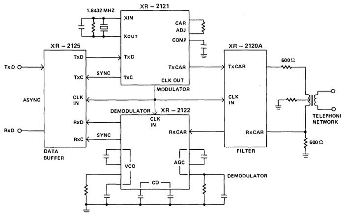
Figure 2. Complete 1200/300 BPS Modem Signal Processor
