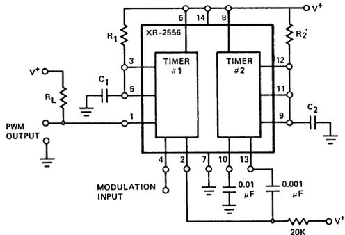
Figure 29. Pulse-Width Modulation With Internal Clock
