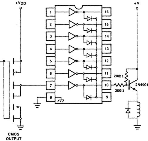
Figure 8. Buffer for Higher Current Loads
