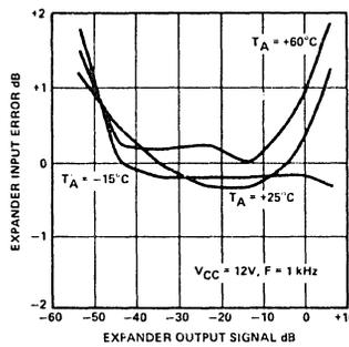
Figure 6. EX-2216 Expander Input Error vs. Output Signal Amplitude
