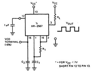
Figure 27. Precision Oscillator with High Current Output Capability
