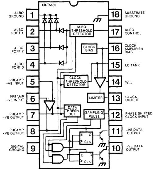
Bipolar PCM signal is attenuated and dispersed in time as it travels along the transmission cable, characteristics of which vary with length, frequency, temperature and humidity. The PCM signal when received is amplified, equalized for amplitude characteristics and reconstructed by the preamplifier, automatic line build out (ALBO), clock and data threshold circuits. Amplitude equalization is achieved through shaping the frequency spectrum with the help of variable impedance ALBO ports.
