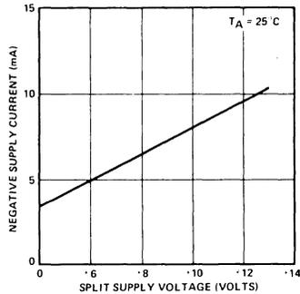
Figure 19. Negative Supply Current, I<sup>-</sup> (Measured at Pin 12) vs. Supply Voltage
