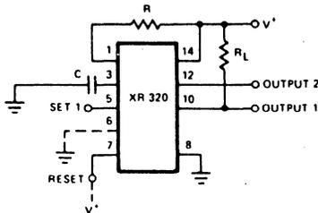
Figure 2. Monostable Operation, Negative Trigger
