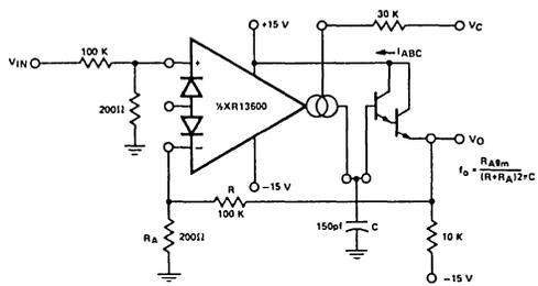
Figure 11. Voltage Controlled Low-Pass Filter
