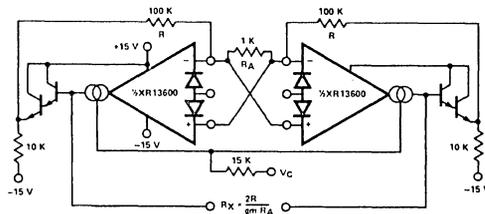
Figure 10. Floating Voltage Controlled Resistor
