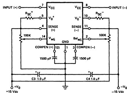
Figure 2. Voltage Adjust and Balance Adjust Circuit
