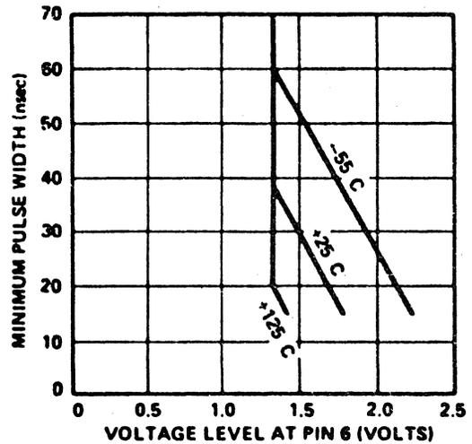
Figure 12. Minimum Pulse Width for Triggering at Pin 6
