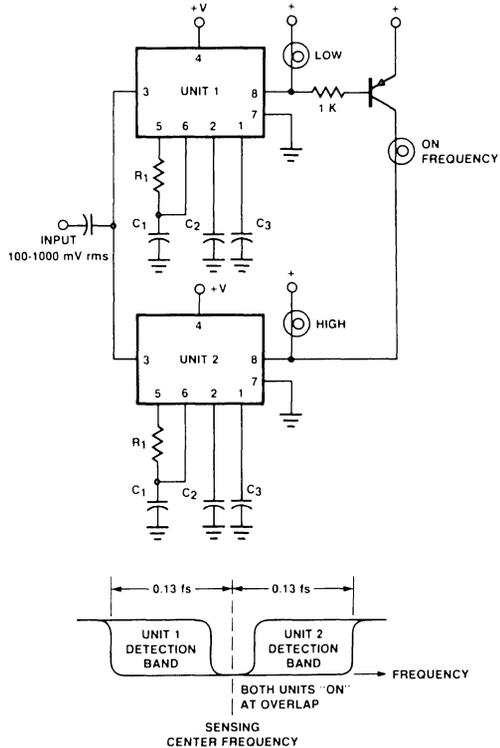
Figure 3. Frequency Meter with Low-Cost Lamp Readout
