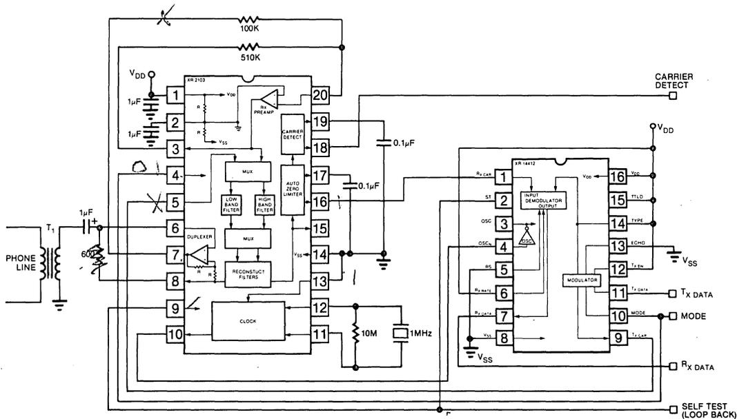
Figure 4. Bell 103 Compatible Modem
