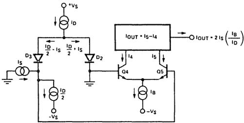
Figure 1. Linearizing Diodes
