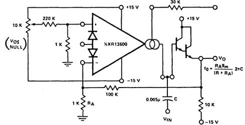
Figure 12. Voltage Controlled High-Pass Filter
