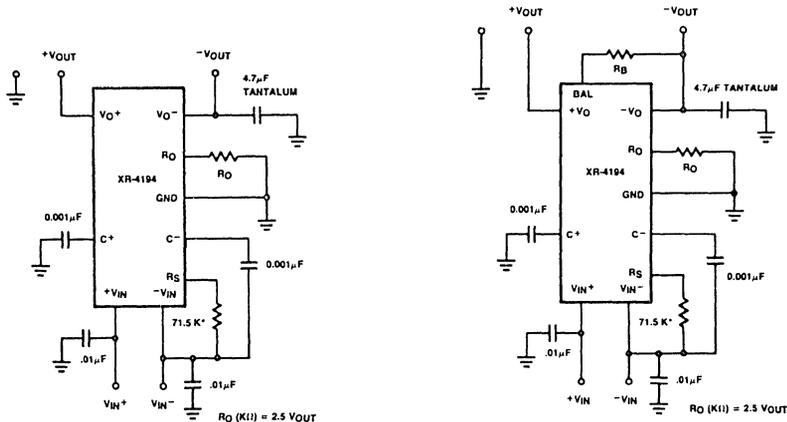
\* For Best Tracking Temperature Coefficient of  $R_O$  Should Be Same As For  $R_S$
