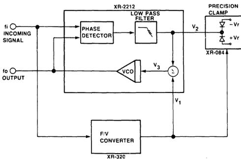
Figure 1. Tracking PLL Block Diagram.
