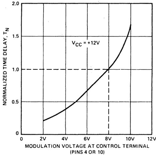
Figure 19. Normalized Time Delay vs. Modulation Voltage
