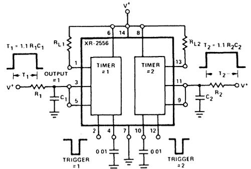
Figure 20. Generation of Two Independent Time Delays
