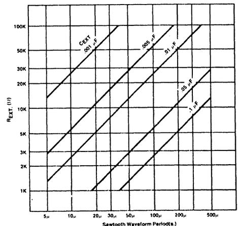
Figure 3. Oscillation Period vs R<sub>EXT</sub> and C<sub>EXT</sub>
