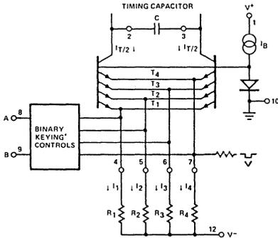
**Figure 9. Simplified Schematic of Frequency Control Mechanism**
