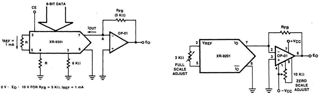
FOR OPERATION WITH NEGATIVE LOGIC D/A CONVERSION, I.E. ZERO FULL SCALE (0000 0000) CORRESPONDING TO FULL SCALE OUTPUT, CONNECT THE INVERTING INPUT OF OP AMP TO  $I_Q$  (PIN 6) AND CONNECT  $I_Q$  (PIN 7) TO GROUND.
