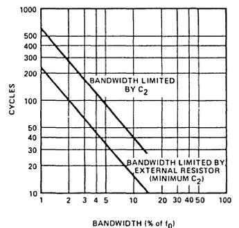
Figure 12. Greatest Number of Cycles Before Output
