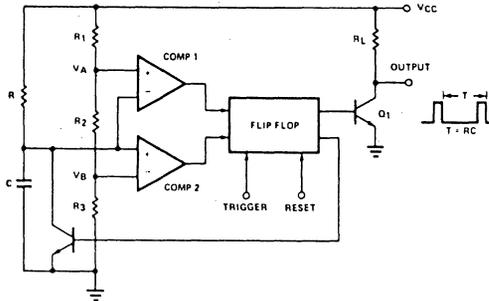
Figure 4. Simplified Schematic of a Time-Base Oscillator Circuit
