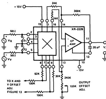
Figure 3. Test Circuit for Feedthrough Measurement. X-Input Feedthrough =  $V_Z$  with  $S_1$ , open  $S_2$  closed. Y-Input Feedthrough =  $V_Z$  with  $S_1$  closed,  $S_2$  open.
