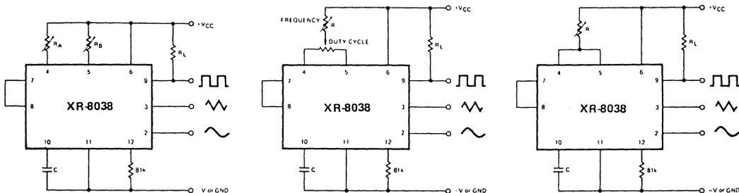
Figure 2. Possible Connections for the External Timing Resistors.
