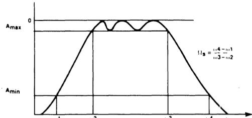
Figure 2. Ratio of  $A_{min}$  Bandwidth to  $A_{max}$  Bandwidth.
