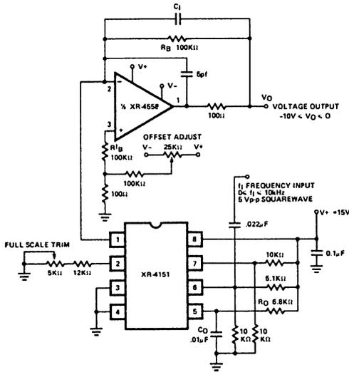
Figure 6. Precision Frequency-to-Voltage Converter
