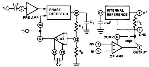
Figure 2. XR-2212 Internal Blocks with External Components.
