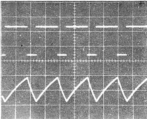
Figure 16. Astable Waveforms
