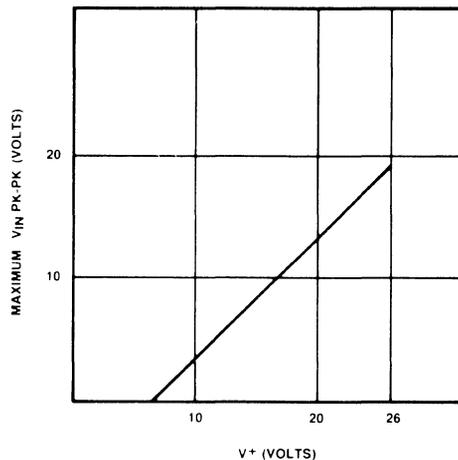
Figure 10. Maximum Input Voltage vs. Supply Voltage.
