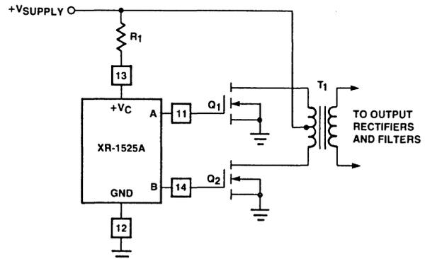
Figure 14. Power FET Push-Pull Outputs with XR-1525A
