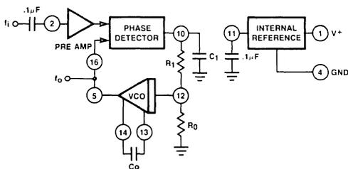
Figure 3. XR-2212 Internal Blocks with External Components.
