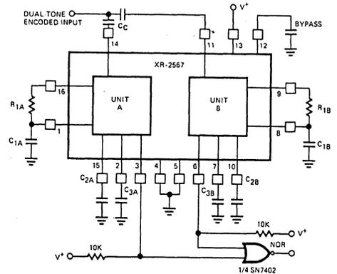
Figure 23. Connection for Decoding Dual-Tone Encoded Input Signals
