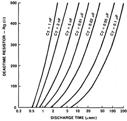
Figure 3. Oscillator Discharge Time vs  $R_D$  and  $C_T$
