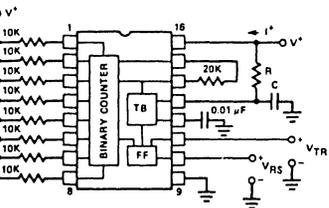
Figure 2. Generalized Test Circuit
