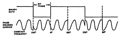
Figure 4. PSK Encoding
