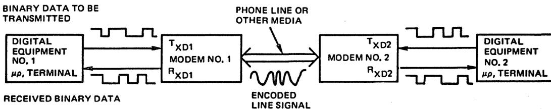
Figure 1. Modem System Block Diagram
