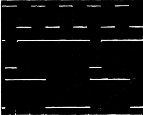
**Figure 25. Frequency Divider and Pulse-Shaper Waveforms**
