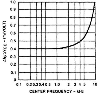
Figure 14. Power Supply Dependence of Center Frequency
