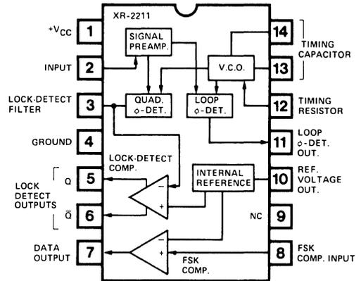
Figure 3. Package Diagram of XR-2211 PLL Circuit.
