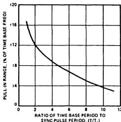
Figure 17. Typical Pull-In Range for Harmonic Synchronization
