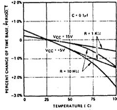
Figure 6. Temperature Drift of Time-Base Period, T
