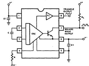
Figure 11. Simplified Circuit Connection for Split Supply Operation With  $V_{GG} = V_{EE} \pm 7V$  (Note: Triangle wave output has  $+0.6V$  offset with respect to ground.)
