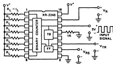
Figure 4. Test Circuit for Counter Section
