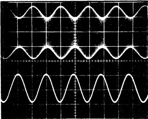
Figure 9-1. Synchronous AM Demodulation
