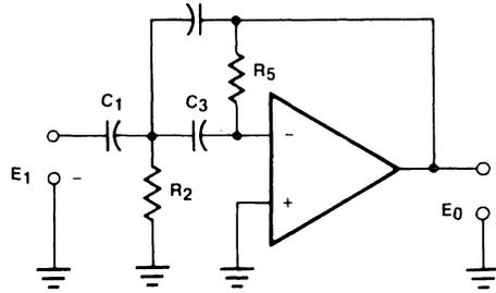
Figure 4. Network Function for the High-Pass Filter.
