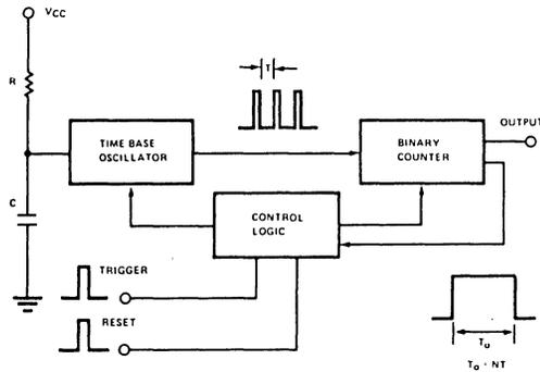
Figure 3. Simplified Block Diagram of a Timer/Counter
