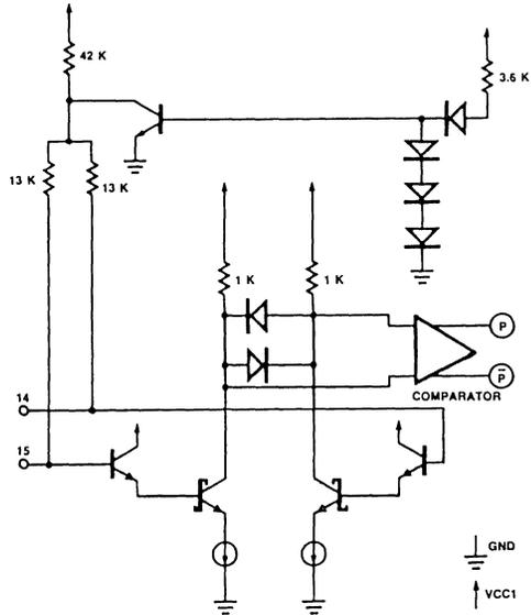
Figure 3. Active Differentiator and Zero Crossing Detector
