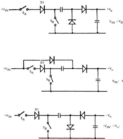
**Figure 9. Capacitor-Diode Coupled Voltage Multiplier Output Stages.** (Note: Diode D1 is Necessary to Prevent Reverse Emitter-Base Breakdown of Transistor Switch S<sub>A</sub>)
