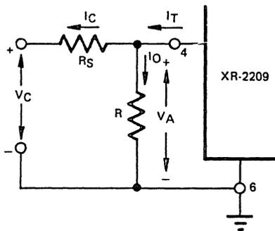
Figure 12. Frequency Sweep Operation
