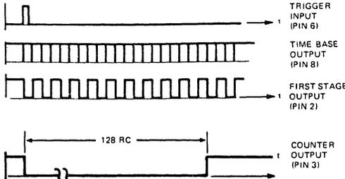
Figure 7. Timing Diagram of Output Waveforms
