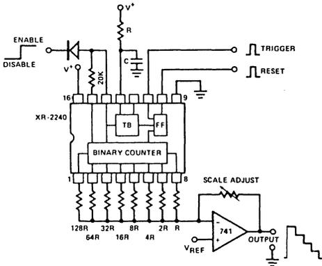
Figure 26. Staircase Generator
