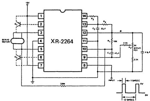
\*NOTE: XR-2264 Q<sub>1</sub> and Q<sub>2</sub> optional; only needed for Servos requiring 500mA drive current.
