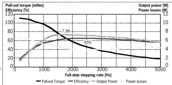
Figure 7. Performance curves for a 25ohm bipolar 42mm square hybrid stepper driven by PBL3770A constant-current driver (Chopper voltage 40V, winding current 280mA).
