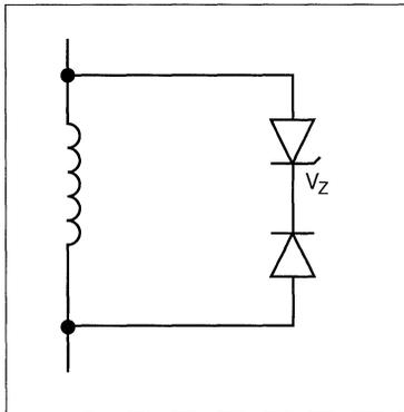
Figure 23. Zener diode turn-off circuit.
