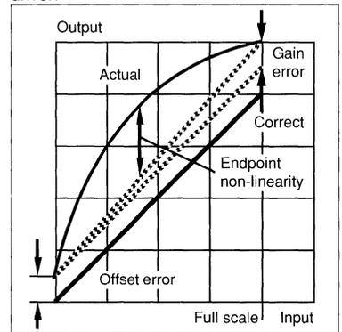
Figure 7. Errors in D/A conversion. Non-linearity, gain and offset errors.
