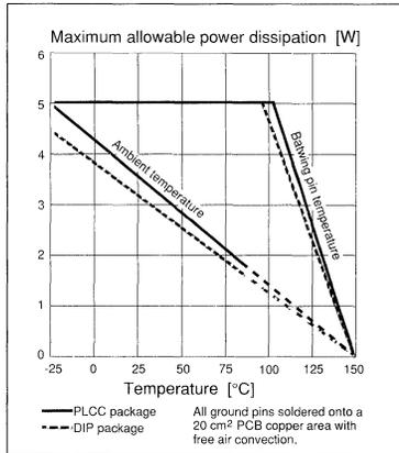
Figure 10. Maximum allowable power dissipation vs. temperature.
