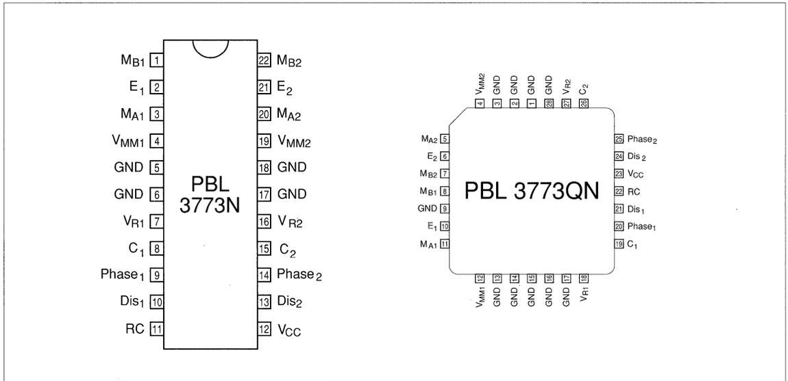
Figure 4. Pin configuration.
