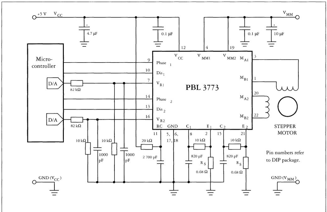
Figure 6. Microstepping system where a microcontroller including DACs provides analog current control voltages as well as digital signals to the PBL 3773.
