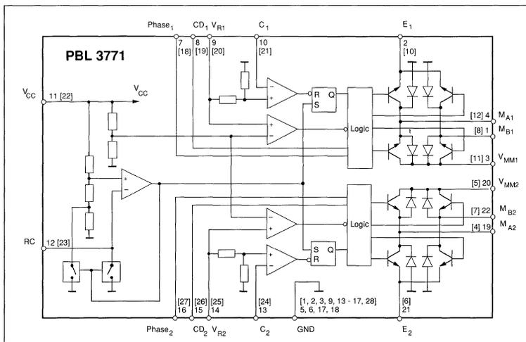
Figure 1. Block diagram.
