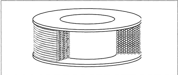
Figure 1. Winding of a typical Permanent Magnet stepper motor.
