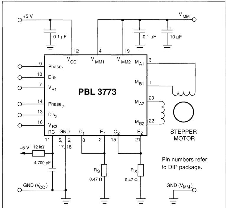
Figure 6. Typical stepper motor driver application with PBL 3773.
