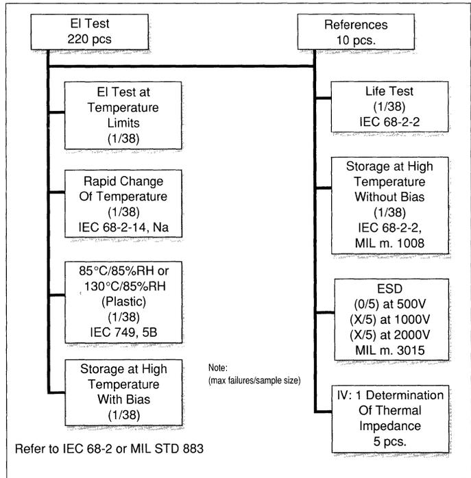
Figure 3. Flow chart, qualification of new chip design. Wafer process and assembly already qualified (all tests are in accordance with MIL-STD883 and IEC 68-2).
