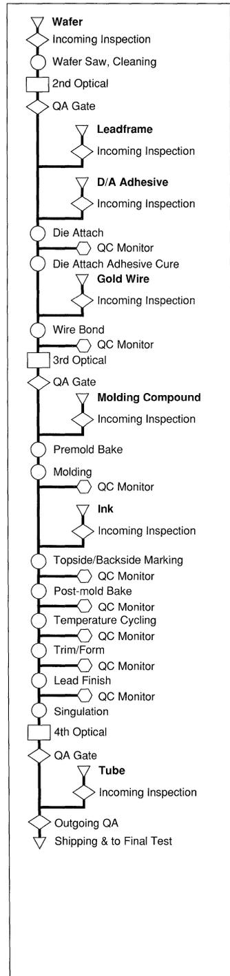
Figure 6. Plastic package QA flow.
