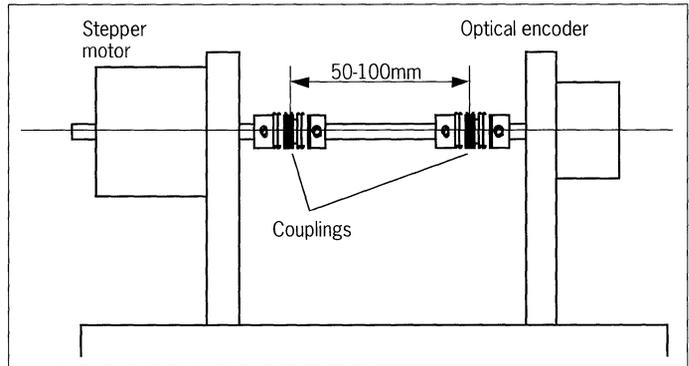
Figure 10. Suggested set-up for measuring microstepping position ripple.
