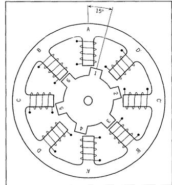
Figure 1. Cross-section of a variable-reluctance (VR) motor.
