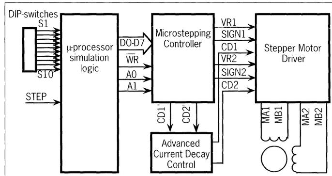
Figure 1. TB370I block diagram.
