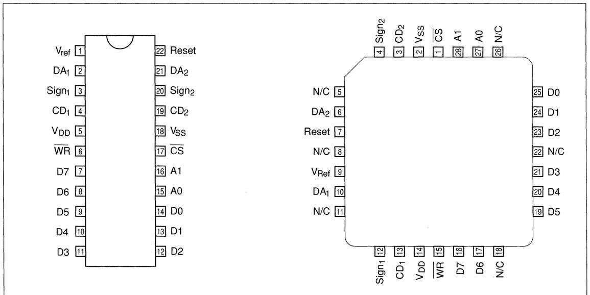
Figure 4. Pin configuration.
