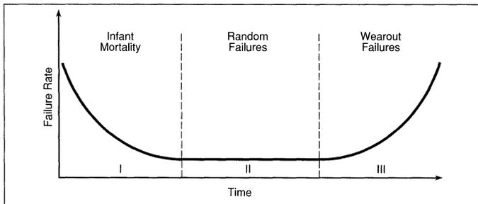
Figure 9. Failure rate distribution, "bathtub" curve.
