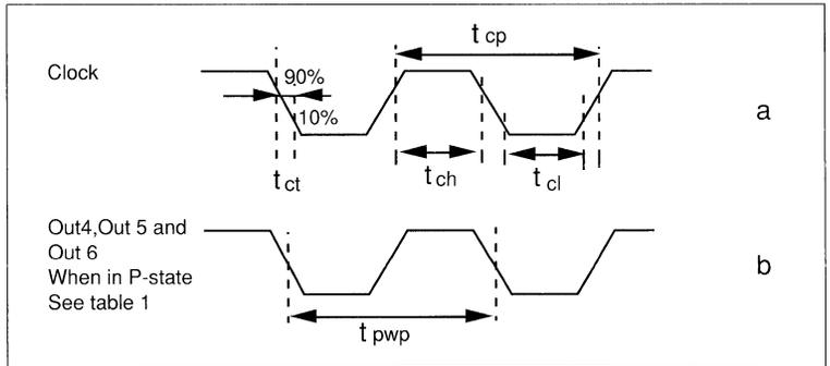
Figure 3. Timing diagram.
