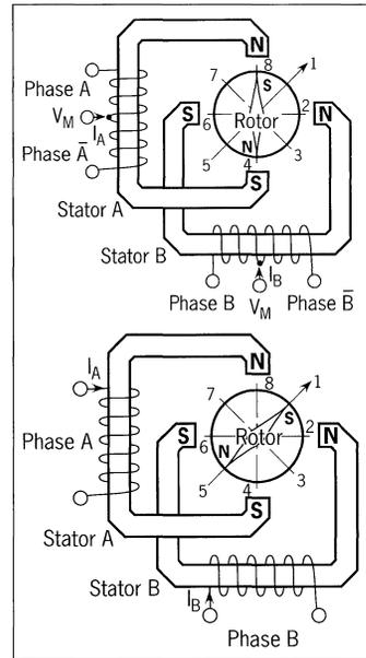
Unipolar and bipolar wound stepper motors.
