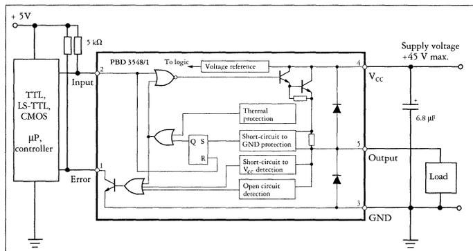
Figure 10. Block diagram and typical application of the PBD 3548/1 Source Driver.
