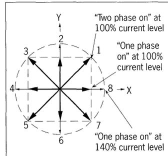
Figure 2. Direction and amplitude of the magnetic field.
