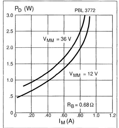
Figure 9. Power dissipation vs. motor current, both channels on.  $T_a = 25^\circ C$ .
