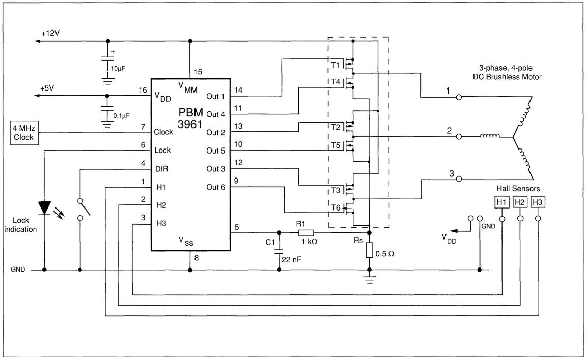
Figure 6. Typical application, T1 — T6 are P and N channel power MOS FETs.
