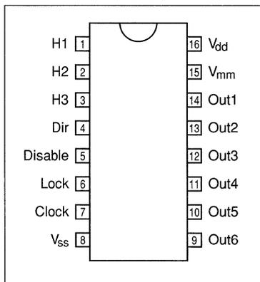
Figure 4. Pin configuration.
