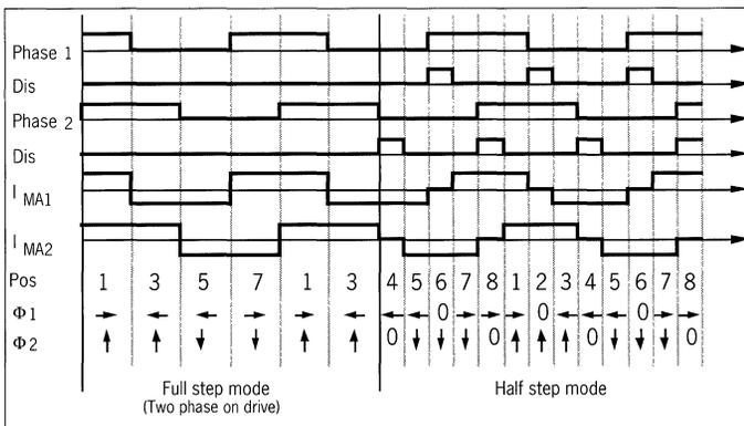
Figure 3. Input signals, output current and magnetic field direction for the different rotor positions in figure 1.
