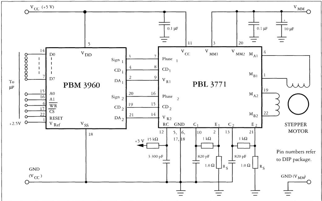
Figure 5. Typical microstepping application in a microprocessor based system.
