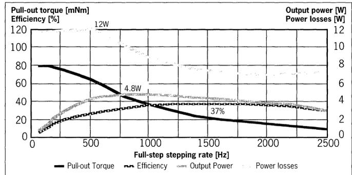
Figure 6. Performance curves for a 3.75ohm bipolar 57mm PM-motor driven by PBL3770A constant-current driver. Power losses in motor and driver are also shown (Chopper voltage 20V, winding current 960mA).
