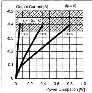
Figure 11. Typical  $P_{Dl}$  vs.  $I_r$  Power dissipation in the bilevel pulse when raising to the  $I_l$  value. One active output.
