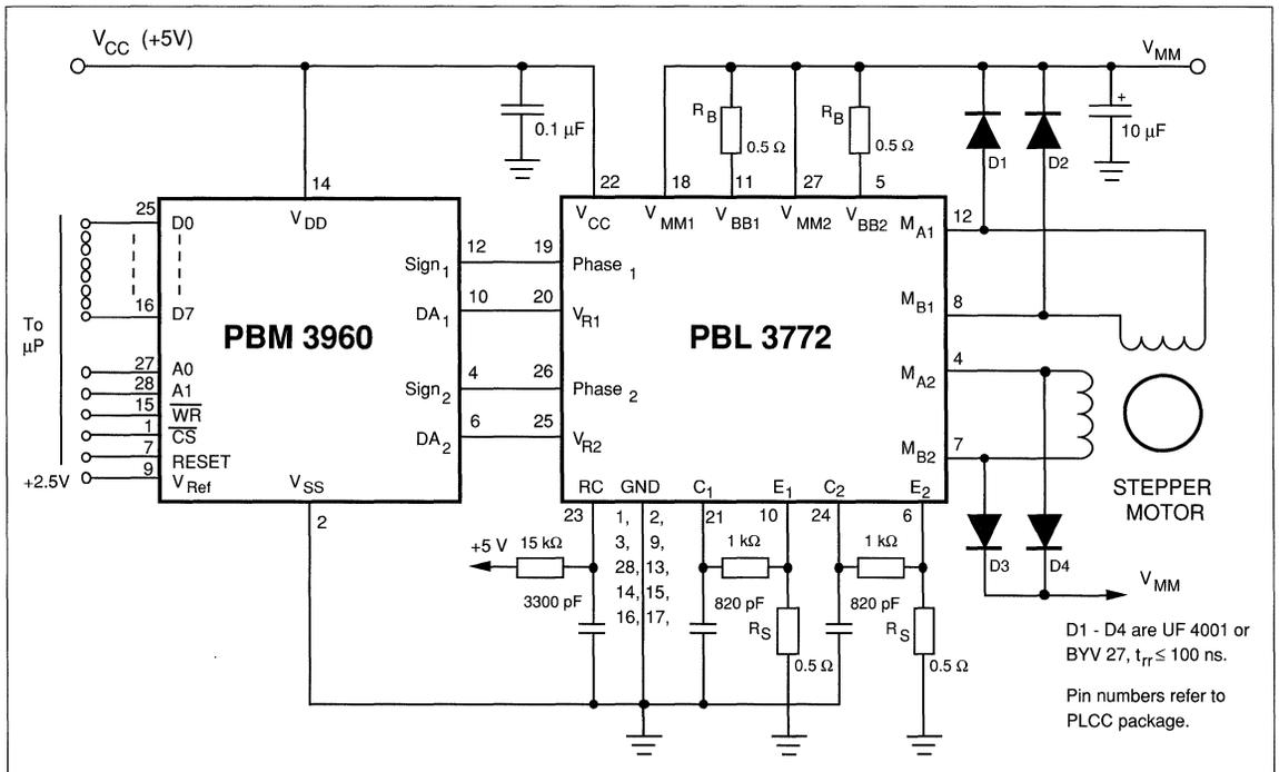
Figure 7. Microstepping system with PBM 3960 and PBL 3772.
