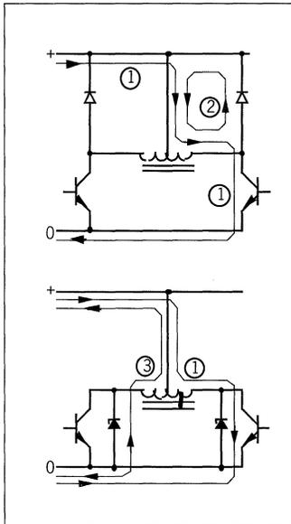
Figure 10. Current paths in the unipolar driver.
