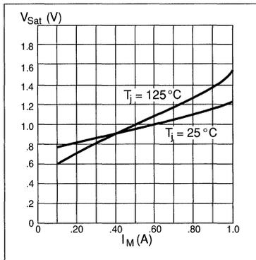
Figure 9. Typical source saturation vs. output current.
