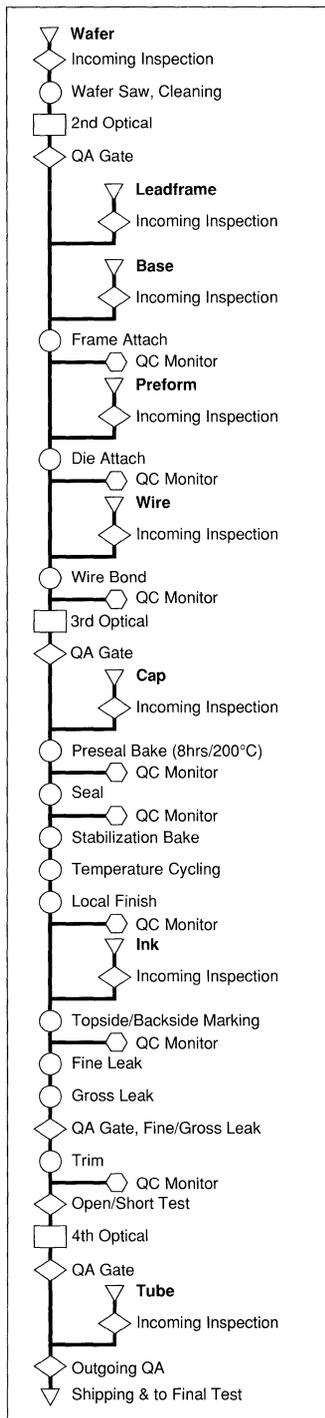
Figure 7. Ceramic package QA flow.
