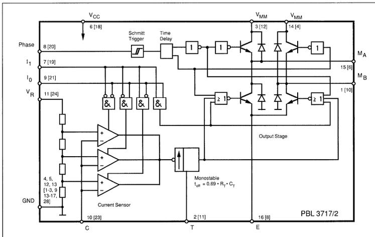
Figure 1. Block diagram
