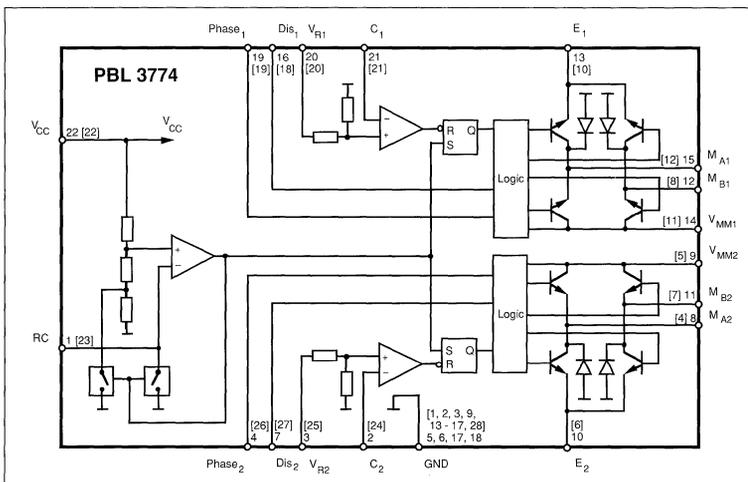
Figure 1. Block diagram.
