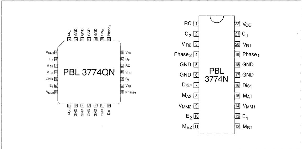
Figure 4. Pin configuration.
