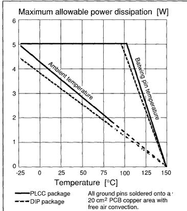
Figure 9. Maximum allowable continuous power dissipation vs. temperature.
