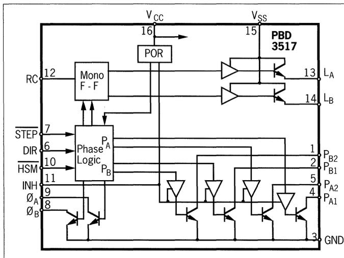
Figure 12. PBD 3517 block diagram.
