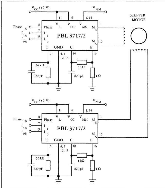
Figure 2. Typical stepper motor driver application with PBL 3717/2.
