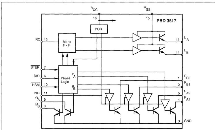
Figure 1. Block diagram.
