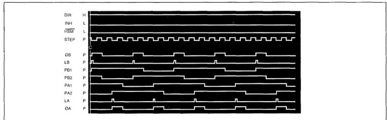
Figure 18. Half-step mode, forward. 8-step sequence.
