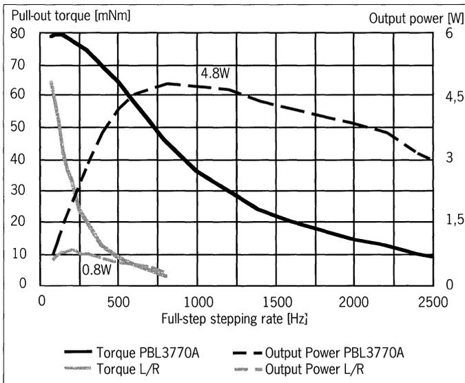
Figure 1. Pull-out torque and output power for a 57mm PM stepper driven by a unipolar L/R-driver and a PBL3770A bipolar constant current driver.
