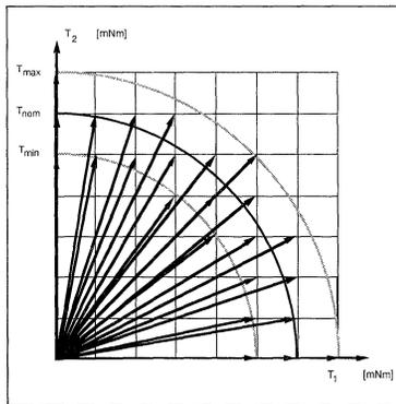
Figure 8b. An example of accessible positions with a given torque deviation/fullstep. Note that 1:st µstep sets highest resolution. Data points are exaggerated for illustration purpose. TNom = code 127.
