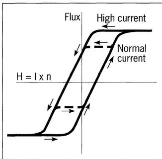
Figure 9. Flux as function of flux history and H-value when two different current levels are applied to the winding.
