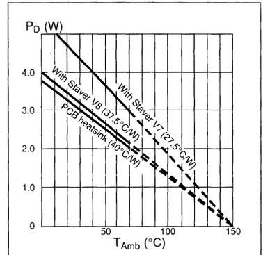
Figure 14. Allowable power dissipation vs. ambient temperature.
