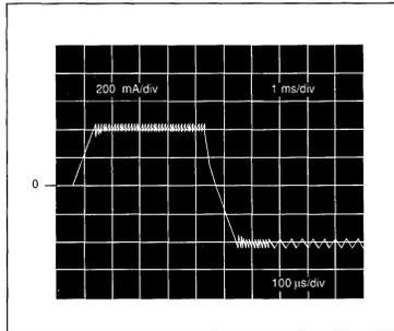
Figure 5. Motor current ( $I_M$ ), Vertical : 200 mA/div, Horizontal: 1 ms/div, expanded part 100 µs/div.
