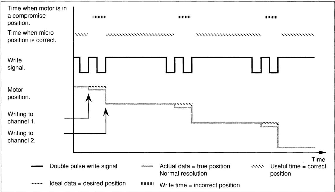
Figure 11. Double pulse programming, in- and output signals.
