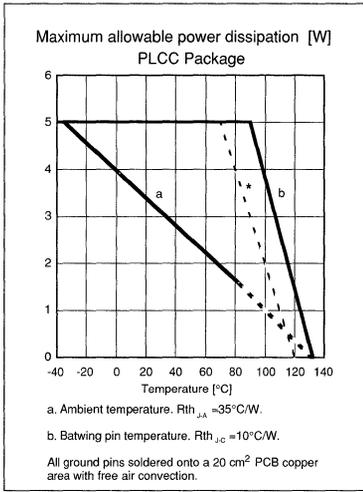
Figure 20. Maximum allowable power dissipation. PLCC package.
