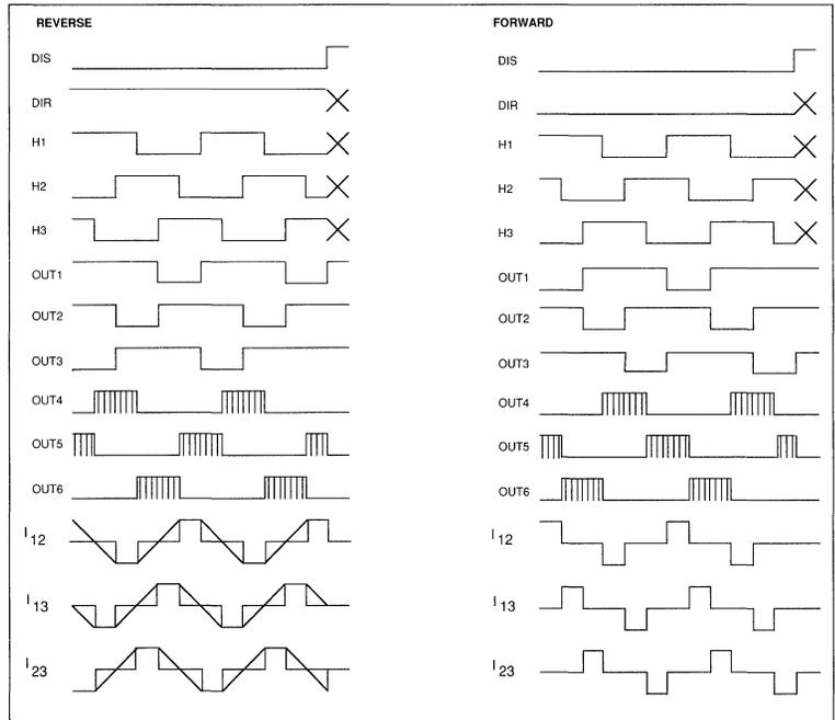
Figure 5. Voltage and current waveforms.
