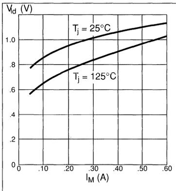
Figure 9. Typical lower diode voltage drop vs. recirculating current.
