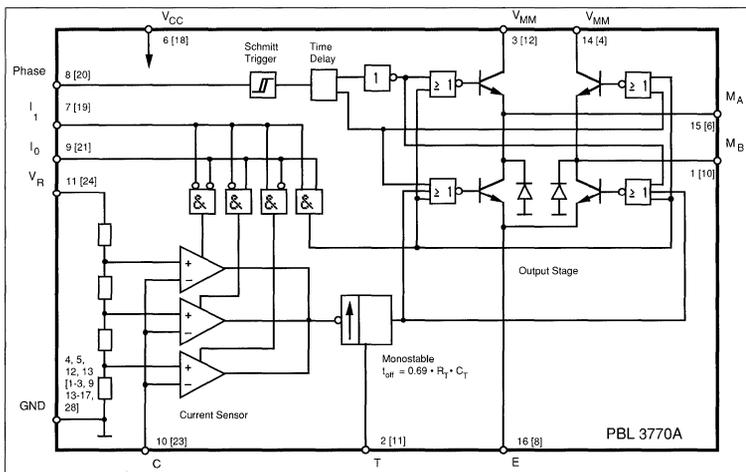
Figure 1. Block diagram.
