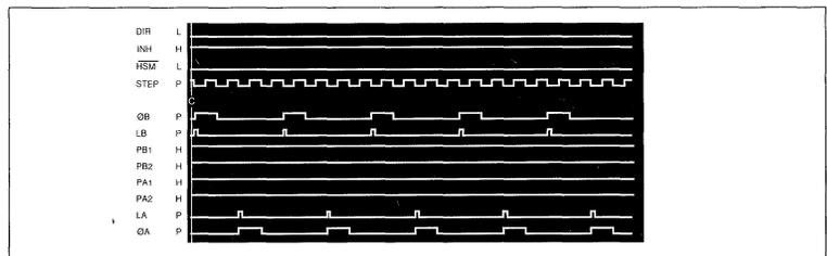
Figure 20. Half-step mode, inhibit.
