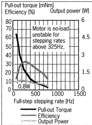
Figure 2. Performance curves for a 100ohm unipolar 57mm PM-motor driven by a 20V L/R constant voltage driver.
