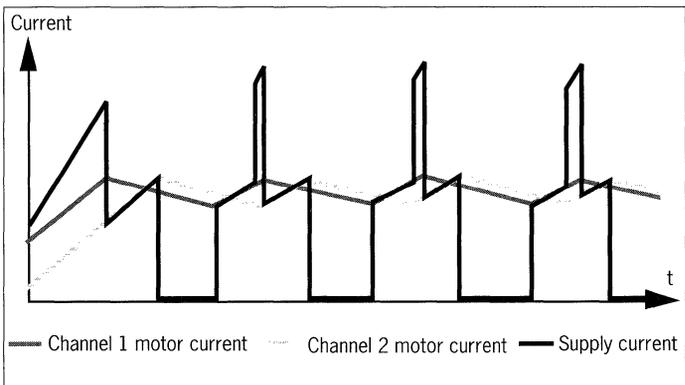
Figure 2. Typical supply current with two channels free-running.
