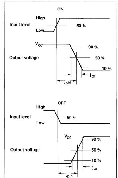
Figure 3. Timing diagram, input vs. output.  $V_{CC} = 24\text{V}$ .
