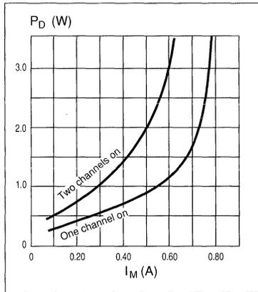
Figure 8. Typical power dissipation vs. motor current. T<sub>a</sub> = 25°C.
