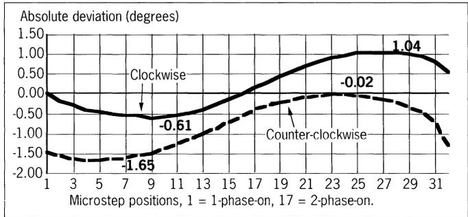
Figure 6. Microstepping position ripple for a 57mm 7.5 degree PM stepper. CW ripple = 1.04 - (-0.61) = 1.65 degrees = 22%.
