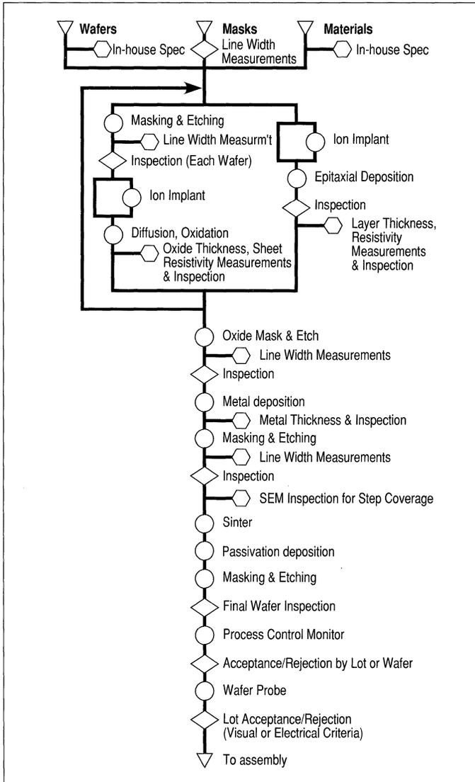
Figure 8. Bipolar production flow.
