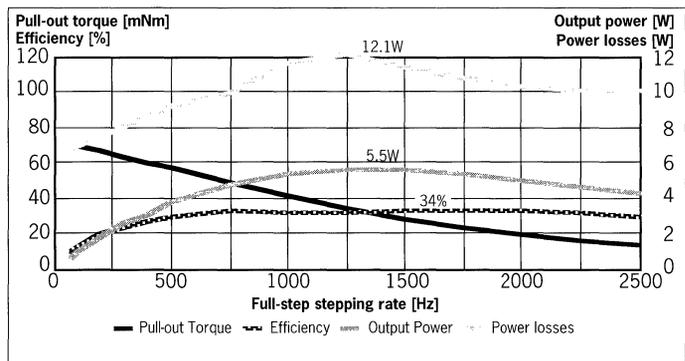
Figure 11. Performance curves for a 3.75ohm bipolar 57mm PM-motor driven by PBL3770A constant-current driver. (Chopper voltage 25V, winding current 600mA).
