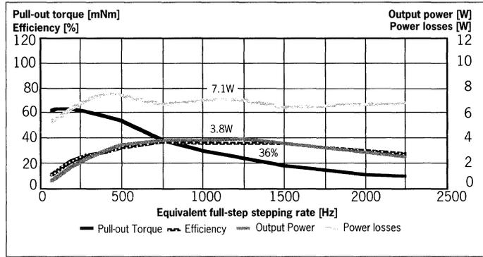
Figure 12. Performance curves for a 3.75ohm bipolar 57mm PM-motor driven by PBL3770A constant-current driver. (Half-step mode fast current decay, Chopper voltage 20V, 2-phase-on current 480mA).
