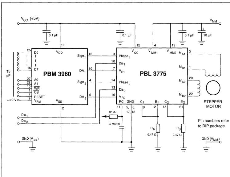
Figure 7. Microstepping system where a microcontroller including DACs provides analog current control voltages as well as digital signals to the PBL 3775.
