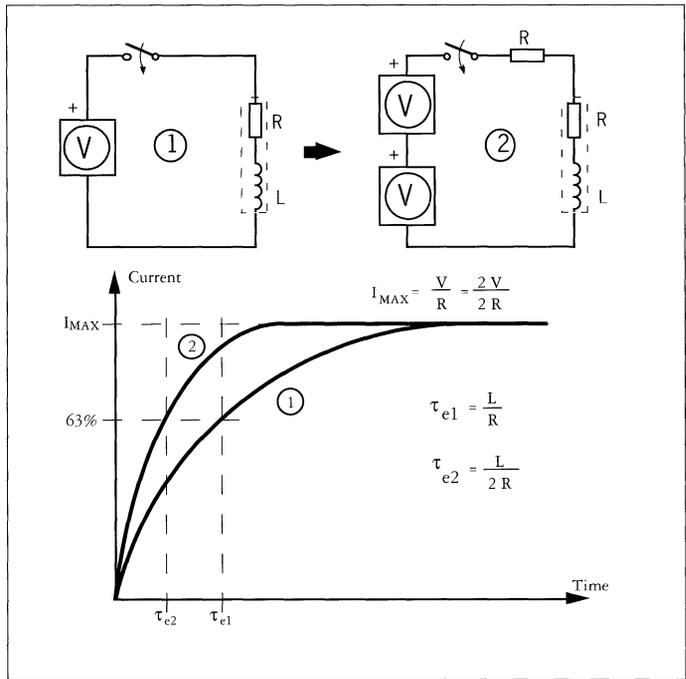
Figure 6. Resistance limitation of the current.
