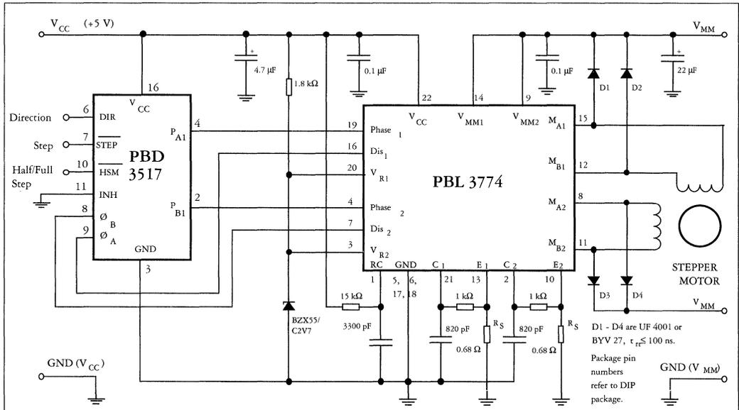
Figure 7. Typical stepper motor driver application with PBL 3774.
