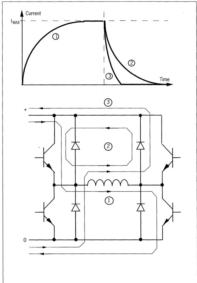
Figure 9. Current paths in the bipolar driver.
