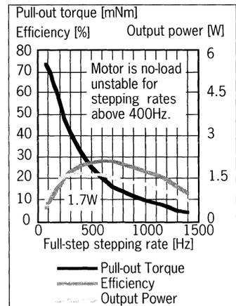
Figure 3. Performance curves for a 100ohm unipolar 57mm PM-motor driven by a 40V L/2R constant-voltage driver ( $2 \times 100\text{ohm}$  external series resistors).
