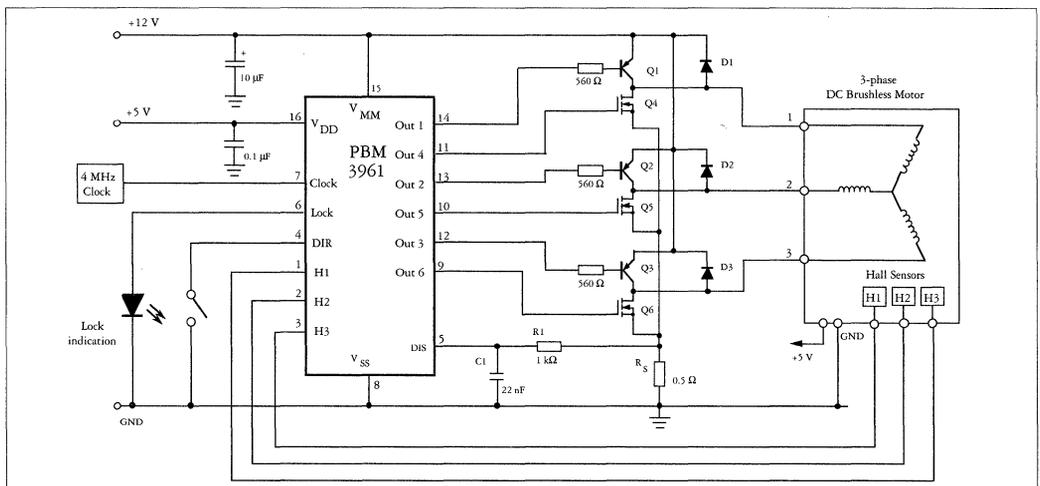
Figure 8. Typical application. Q1-Q3 are PNP power transistors and Q4-Q6 are N-channel power MOSFETs.
