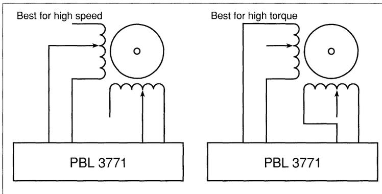
Figure 11. Connection of unipolar motors.
