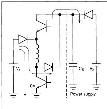
Figure 25. Power return turn-off circuit for bilevel.
