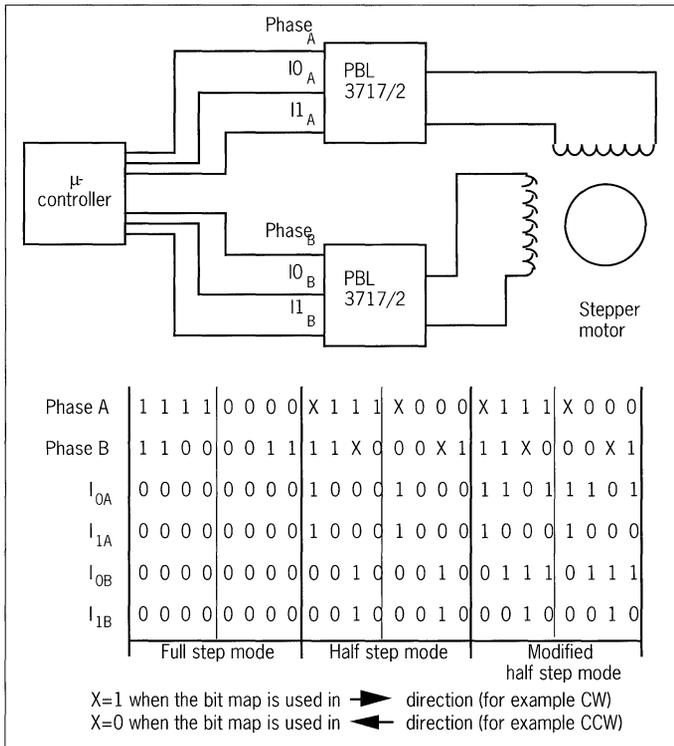
Figure 8. Two PBL 3717/2 controlled by a microprocessor and an output bit map. Note, the change in the digital sequence when changing direction; the figure will generate fast current decay; reverse X-polarity to get slow current decay.
