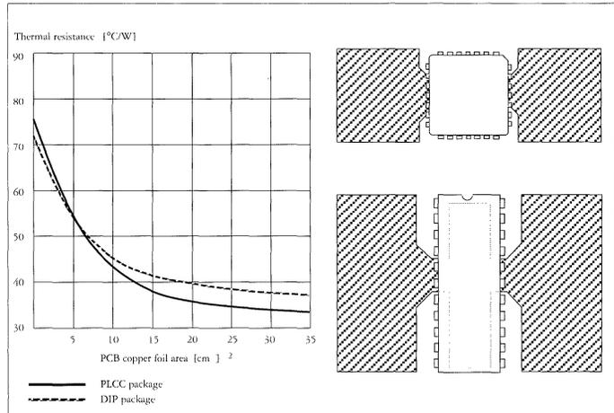
Figure 1. Typical thermal resistance vs. PC Board copper area and suggested layout.
