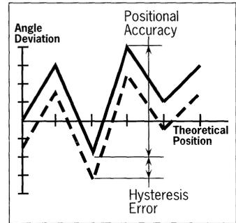
Figure 6. Positional accuracy of a stepper motor.
