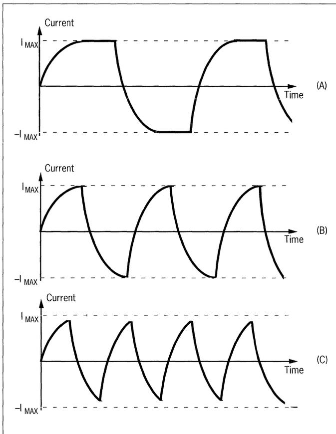
Figure 4. Current wave form in an inductive-resistive circuit.
