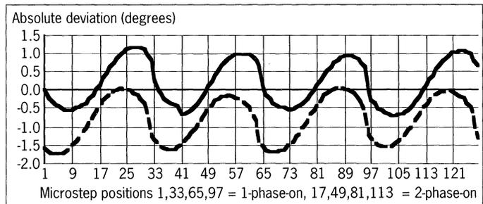
Figure 11. Microstepping position ripple for 4 full-step cycles for a 57mm 7.5 degree PM stepper.
