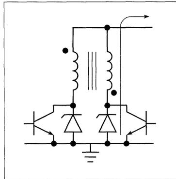
Figure 24. Power return turn-off circuit.
