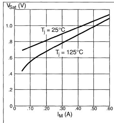
Figure 10. Typical sink saturation voltage vs. output current.
