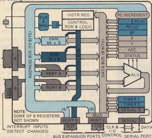
**HARDWARE SUPPORT:** Special 64-pin device for prototyping. 660X's ROM can carry "KIM" or "TIM" monitors, so users can develop stand-alone prototyping stations. Besides 650X parallel-bus support chips, 660X will have serial-bus peripheral devices.
