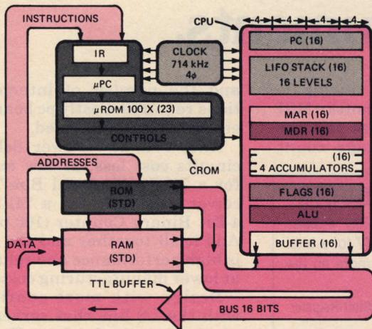
Slice approach plus microprogramming gives customers freedom to reconfigure hardware and software. (I/O not shown.)
