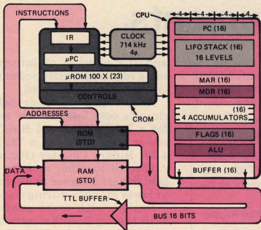
Slice approach plus microprogramming gives customers freedom to reconfigure hardware and software. (I/O not shown.)
