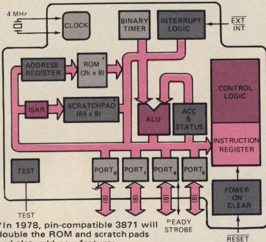
\*In 1978, pin-compatible 3871 will double the ROM and scratch pads and also add new features.
