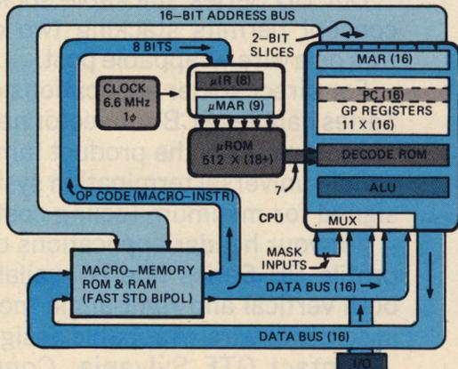
Diagram shows 16-bit minicomputer constructed from 3000-Series parts. Although slices are only two bits wide, they include a large number of parallel paths for high processing throughput.
