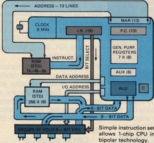
Simple instruction set allows 1-chip CPU in bipolar technology.
