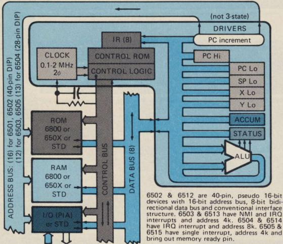
6502 & 6512 are 40-pin, pseudo 16-bit devices with 16-bit address bus, 8-bit bidirectional data bus and conventional interface structure. 6503 & 6513 have NMI and IRQ interrupts and address 4k. 6504 & 6514 have IRQ interrupt and address 8k. 6505 & 6515 have single interrupt, address 4k and bring out memory ready pin.
