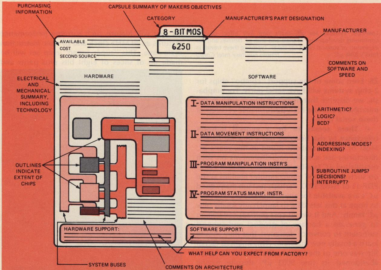
**Legend diagram for EDN's  $\mu$ P files** with the various "information spaces" called out and explained. The information is purposely equally divided into a hardware half and a software half to emphasize the "two-sided" nature of these SP/GP/DC-type products. (SP/GP/DC stands for stored program, general-purpose digital computer.)
