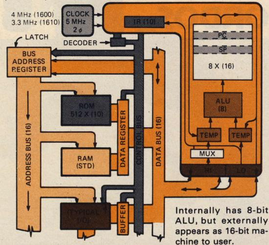
Internally has 8-bit ALU, but externally appears as 16-bit machine to user.
