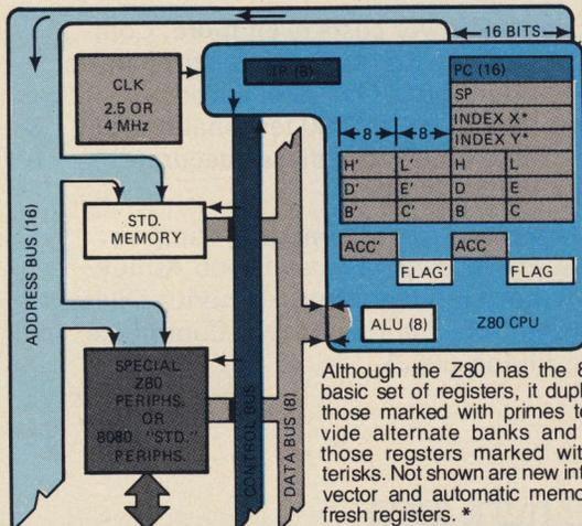
Although the Z80 has the 8080's basic set of registers, it duplicates those marked with primes to provide alternate banks and adds those registers marked with asterisks. Not shown are new interrupt vector and automatic memory refresh registers.\*
