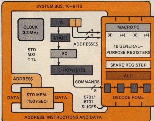
16-bit computers of this architecture using slices are said to equal performance of PDP-11 and Interdata Model-70 minis with much reduced parts counts (50 vs. 200 or better).
