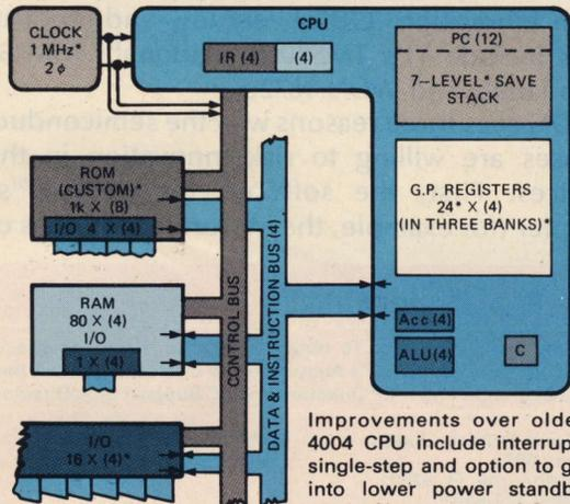
Improvements over older 4004 CPU include interrupt, single-step and option to go into lower power standby mode. New memory, I/O and clock devices.
