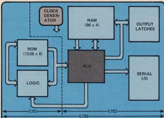
**NOTE:** The 1-chip 5799 is not expandable. However, a 2-chip version (5781 and 5782) provides double the ROM and more RAM and also allows for further memory expansion. Available support chips interface to printers and displays, etc.
