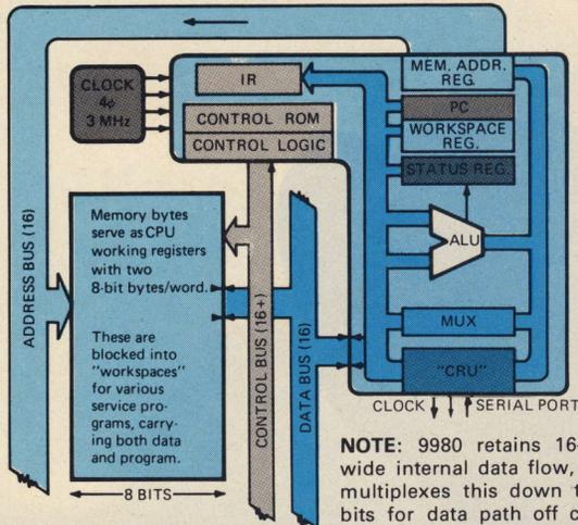
**NOTE:** 9980 retains 16-bit wide internal data flow, but multiplexes this down to 8 bits for data path off chip.
