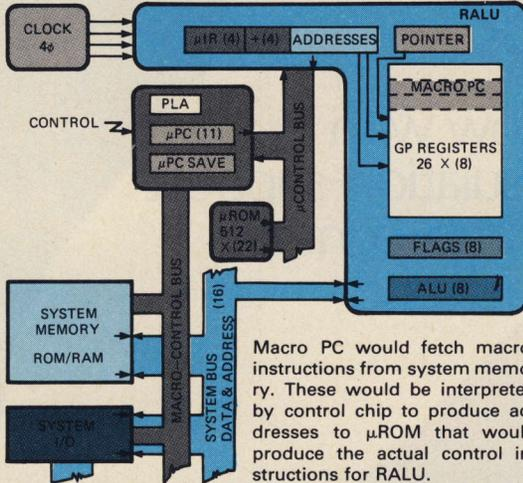
Macro PC would fetch macro-instructions from system memory. These would be interpreted by control chip to produce addresses to  $\mu$ ROM that would produce the actual control instructions for RALU.
