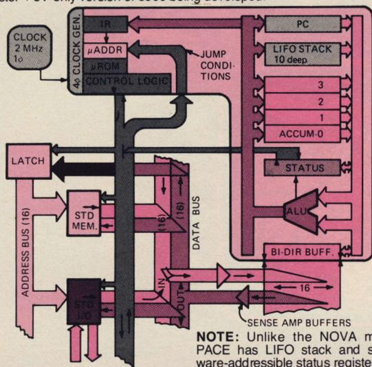
**NOTE:** Unlike the NOVA mini, PACE has LIFO stack and software-addressible status registers.
