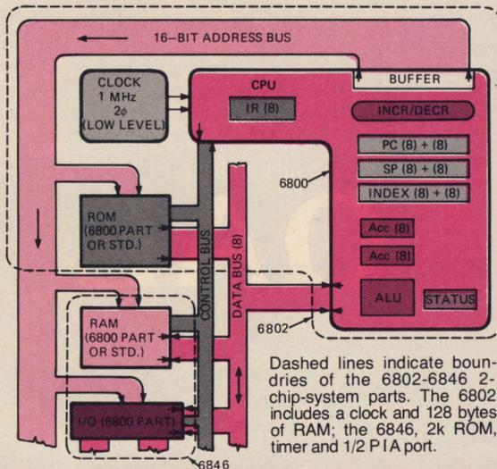
Dashed lines indicate boundaries of the 6802-6846 2-chip-system parts. The 6802 includes a clock and 128 bytes of RAM; the 6846, 2k ROM, timer and 1/2 PIA port.
