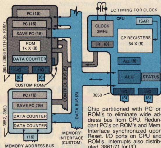
Chip partitioned with PC on ROM's to eliminate wide address bus from CPU. Redundant PC's on ROM's and Mem. Interface synchronized upon Reset. I/O ports on CPU and ROM's. Interrupts also distributed. 3861/71 for I/O.
