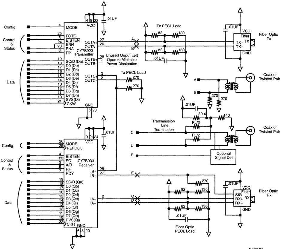
**Figure 6. HOTLink Connection Diagram**
