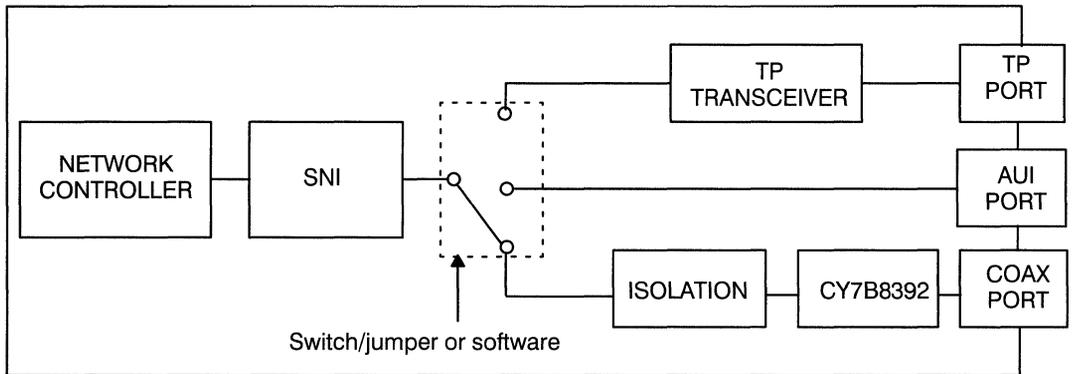
**Figure 10. Typical Network Interface Card**
