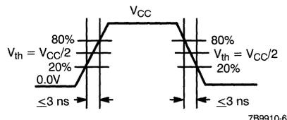
**CMOS Input Test Waveform (CY7B9920)**
