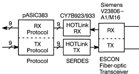
**Figure 5. Design Example Structure**
