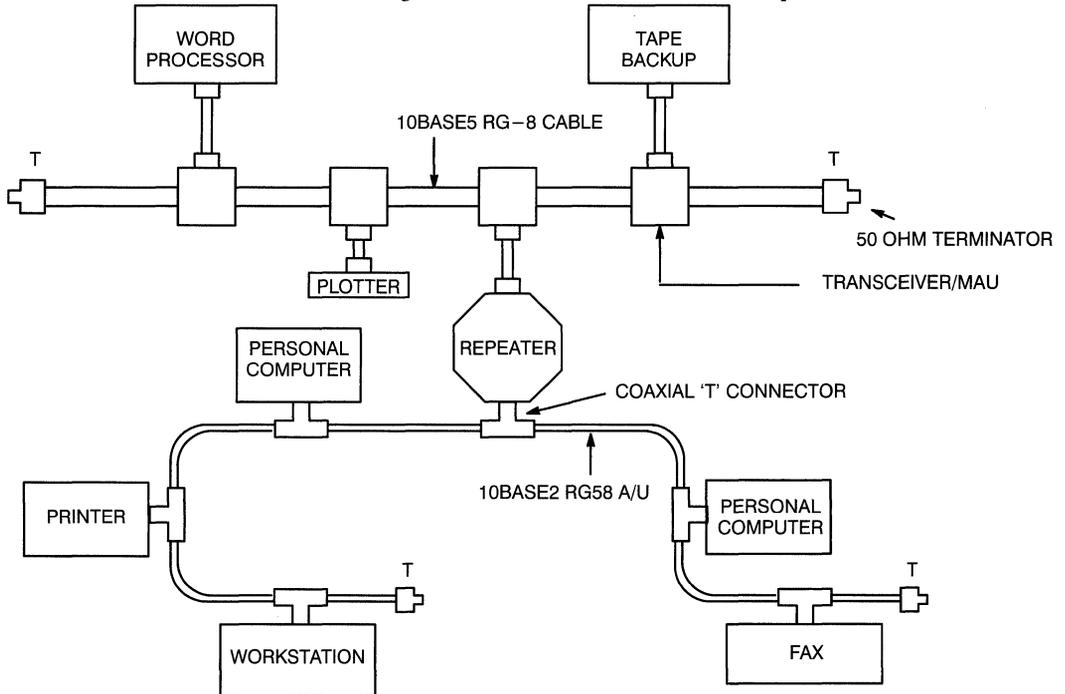
**Figure 5. Combined Ethernet and Cheapernet Network**
