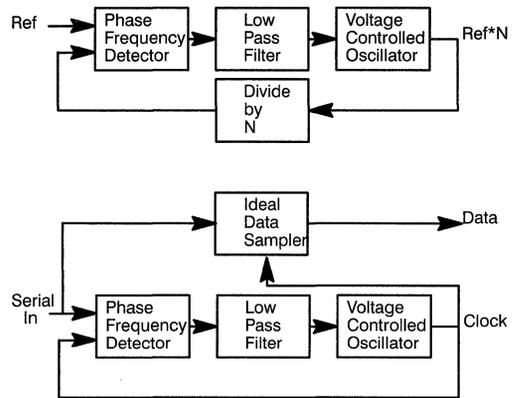
**Figure 8. Multiplication and Clock/Data Recovery PLLs**
