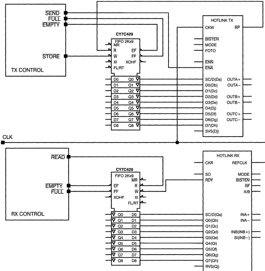
**Figure 12. Asynchronous FIFO Interface**
