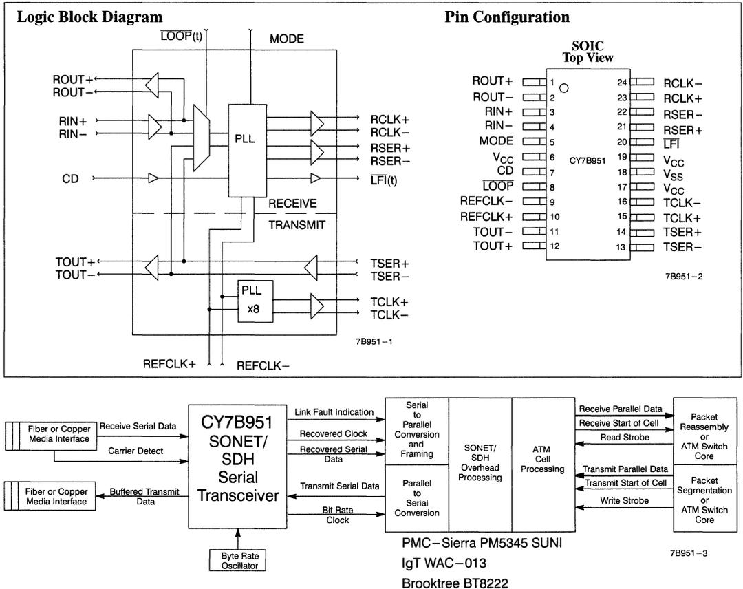
Figure 1. SONET/SDH and ATM Interface
