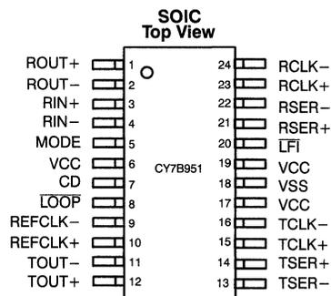
**Figure 2. SST Pinout**
