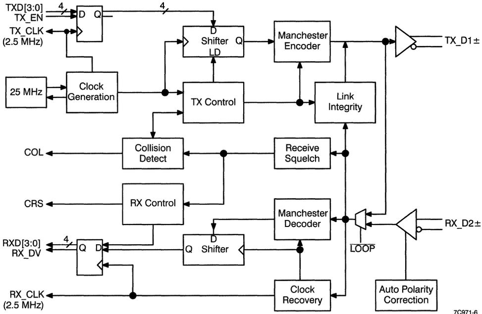
**Figure 4. 10BASE-T Transmitter & Receiver Block Diagram**
