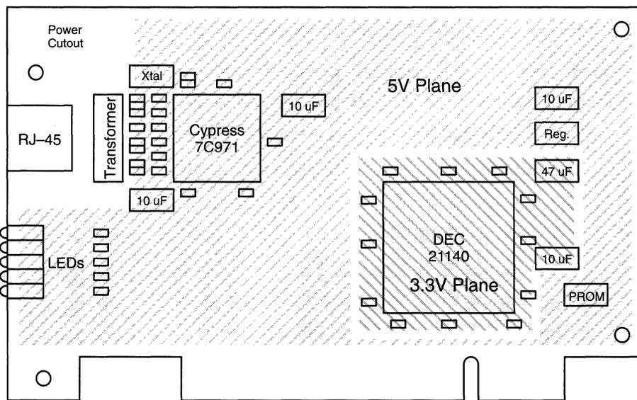
**Figure 7. Power Plane and Component Placement**
