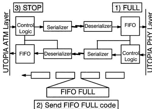
**Figure 13. FIFO State Updating, FIFO Full**
