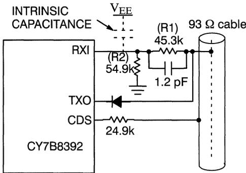
**Figure 9. CY7B8392 application using 93Ω Cable**
