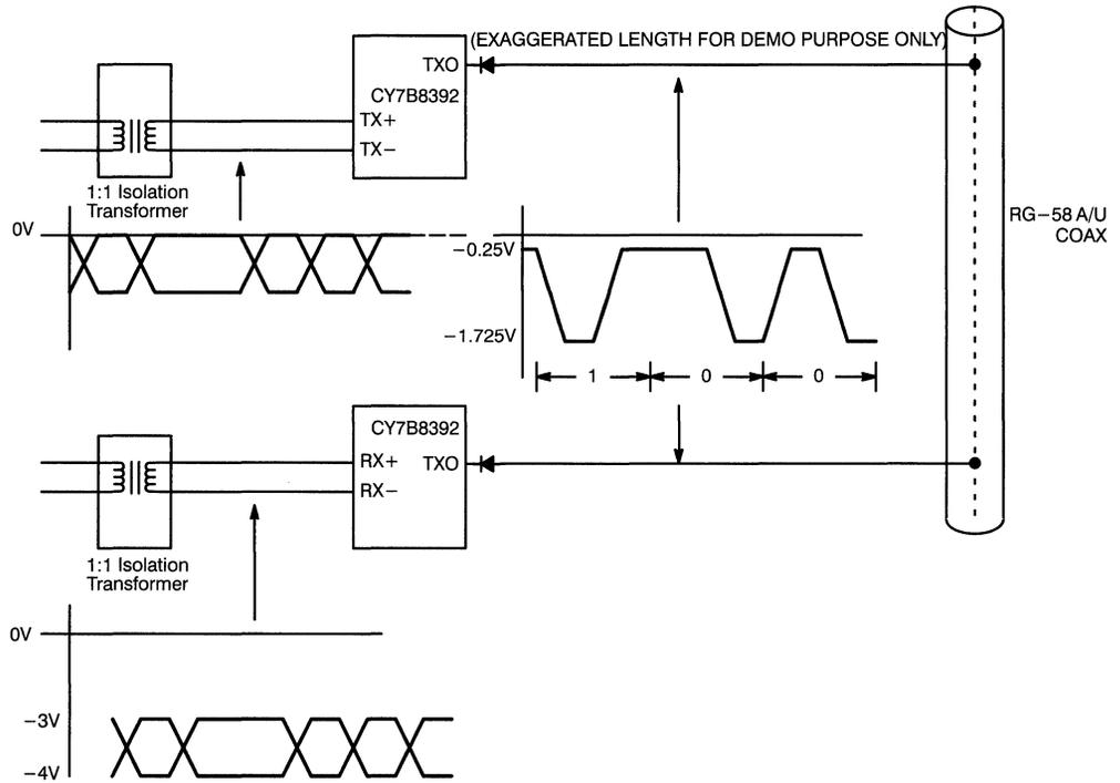
**Figure 6. CY7B8392 Transmission and Reception over the Network**
