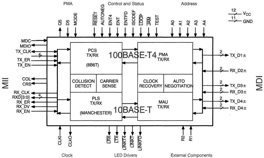
**Figure 3. CY7C971 Block Diagram**
