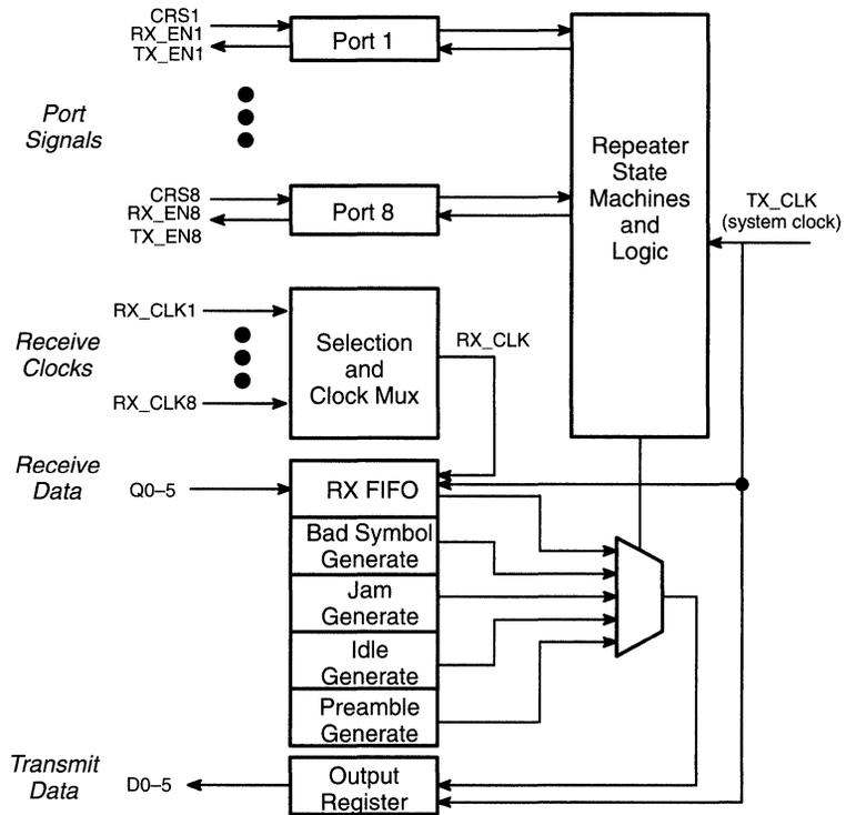
Figure 9. Core Logic
