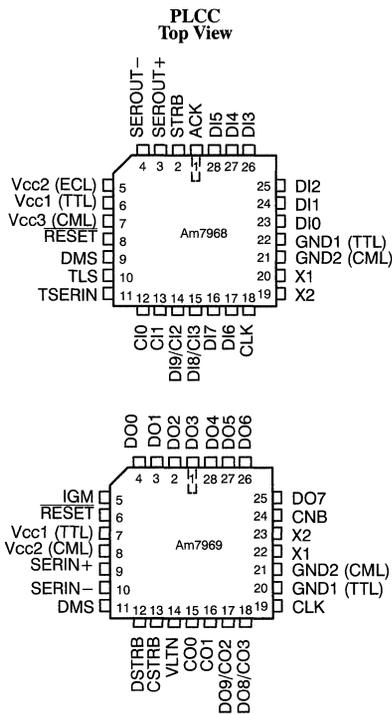
**Figure 7. Am7968 and Am7969 Pin Configurations**
