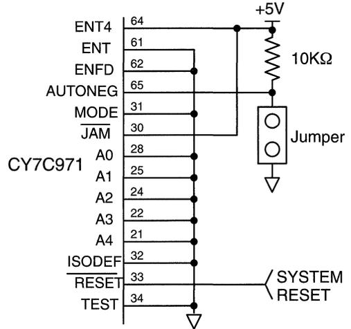
**Figure 7. Configuration Pins**
