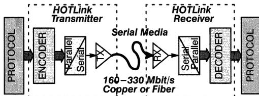
Figure 1. CY7B923 Transmitter Logic Diagram
