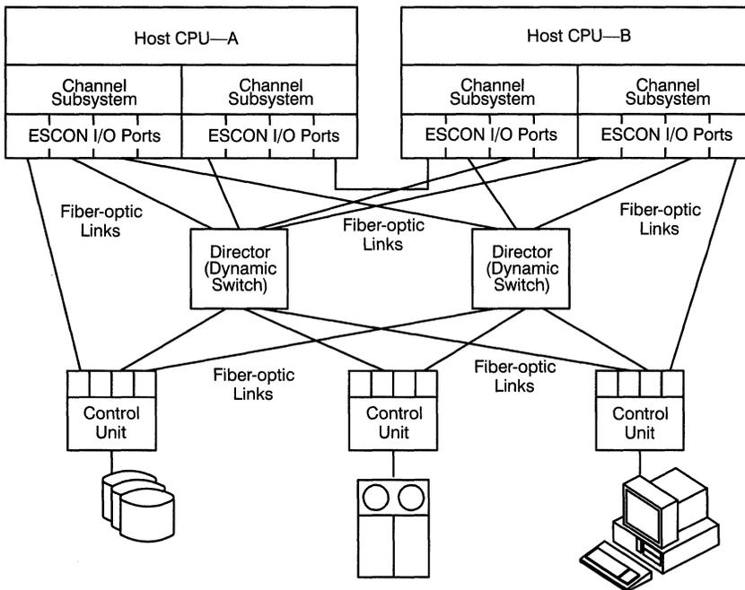
Figure 2. ESCON Channel Subsystem
