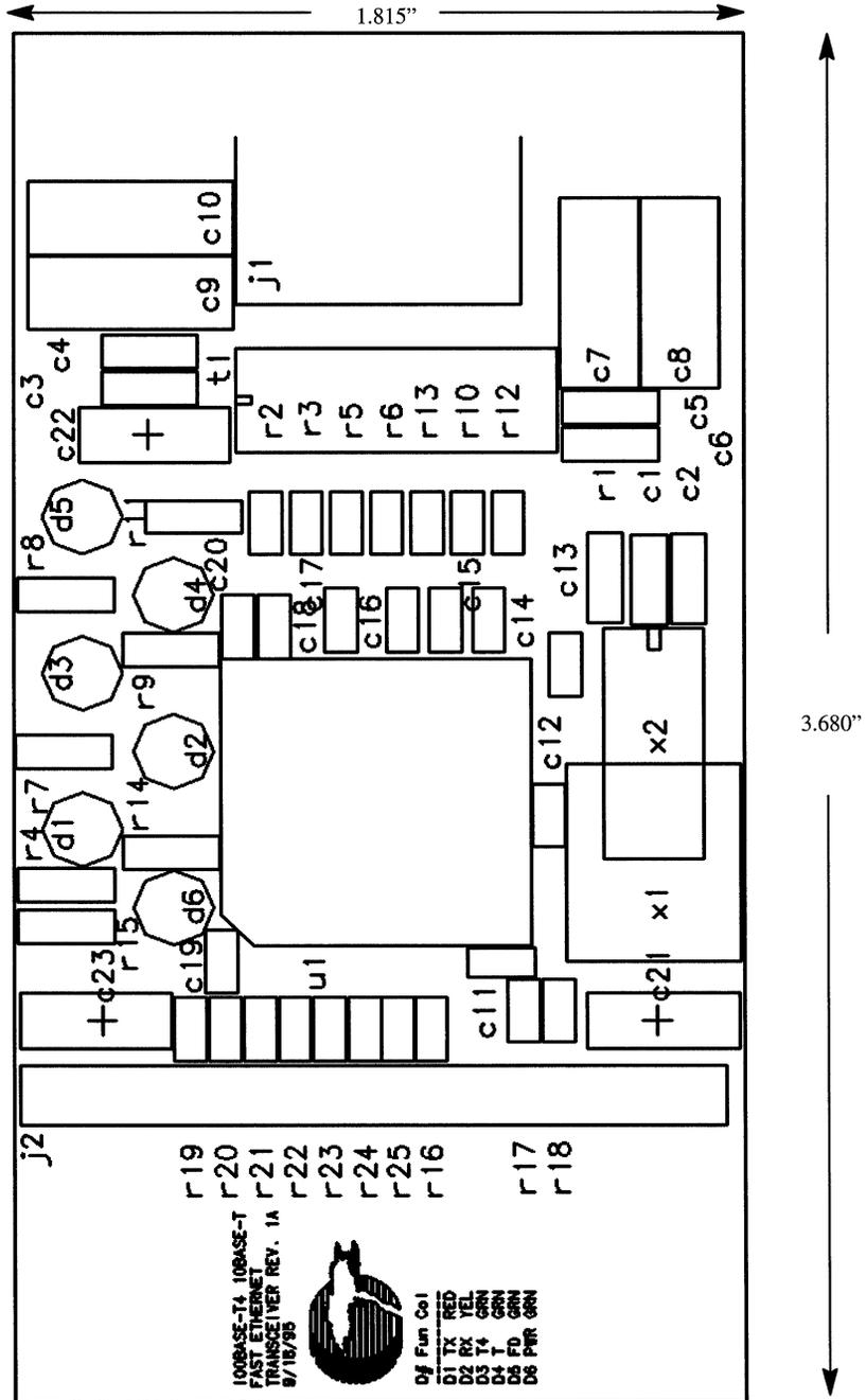
Figure 3. Transceiver Application PCB
