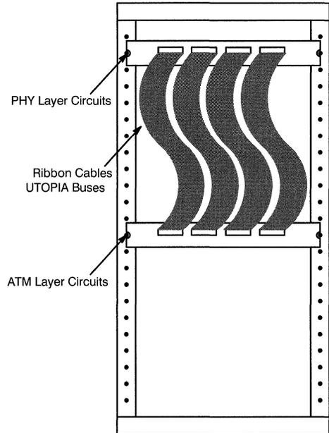
**Figure 5. UTOPIA in a Rack Mount Switch**
