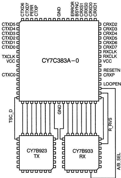
**Figure 12. HOTLink/pASIC Pinout and Interconnect**
