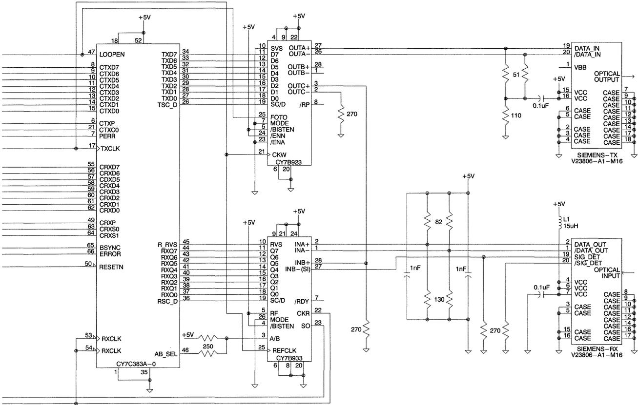
Figure 6. ESCON Physical I/O Interface Schematic
