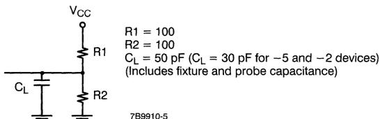
**CMOS AC Test Load (CY7B9920)**
