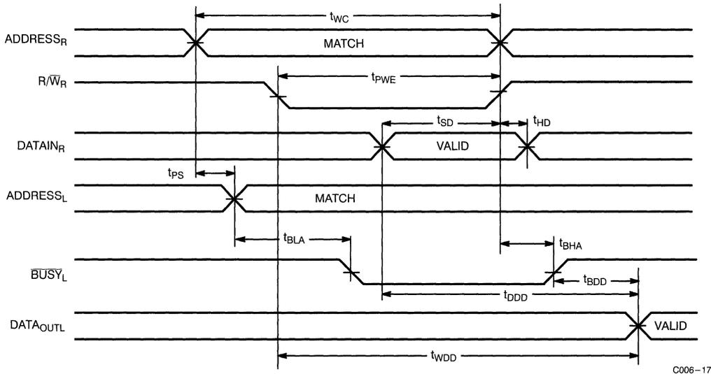
**Write Timing with Busy Input ( $\text{M}/\overline{\text{S}}=\text{LOW}$ )**
