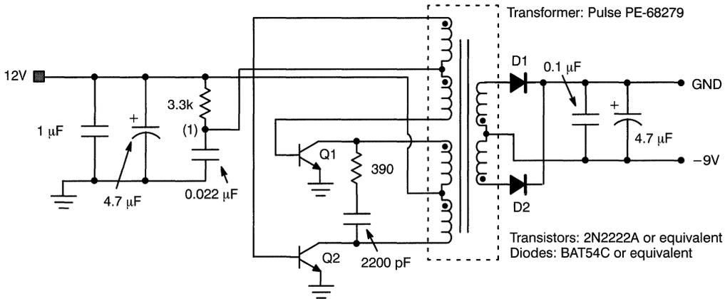
**Figure 12. DC-DC Converter Design**
