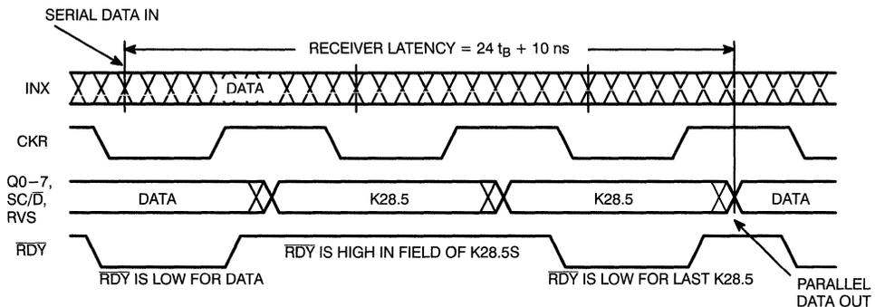
**Figure 3. CY7B933 Receiver Data Pipeline in Encoded Mode**
