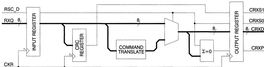
**Figure 10. pASIC Receive Path Block Diagram**
