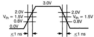
**TTL Input Test Waveform (CY7B991)**
