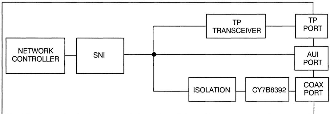
**Figure 11. Advanced Network Interface Card with Auto-AUI Function**
