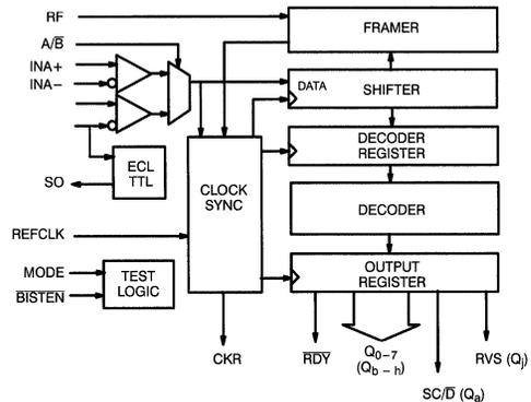
Figure 3. CY7B933 Receiver Logic Diagram
