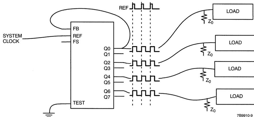
Figure 1. Zero-Skew and/or Zero-Delay Clock Driver
