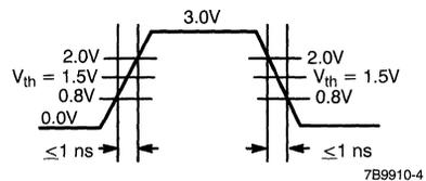
**TTL Input Test Waveform (CY7B9910)**
