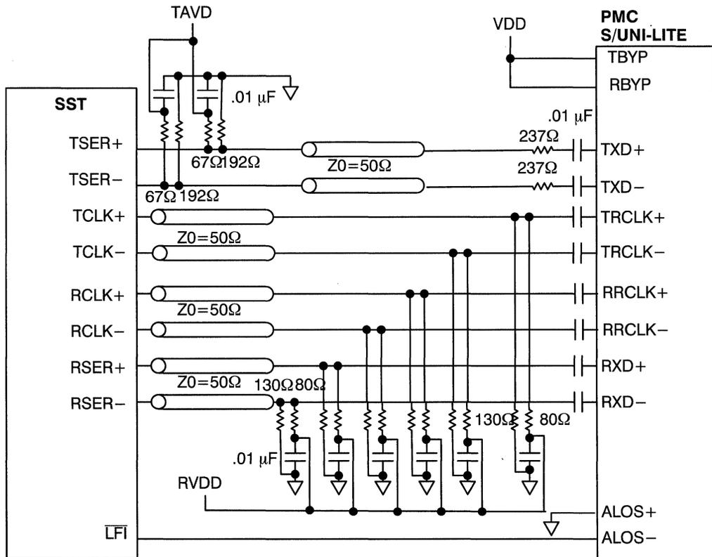
**Figure 6. High Performance SST to PMC S/UNI-LITE Interface**
