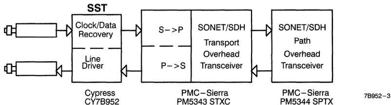
Figure 1. SONET/SDH Overhead Processing Application
