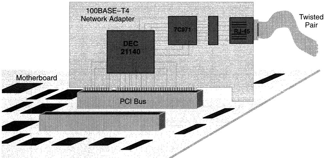
Figure 1. PCI Network Adapter Card
