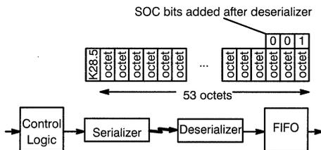
**Figure 12. Transmission Data Flow**
