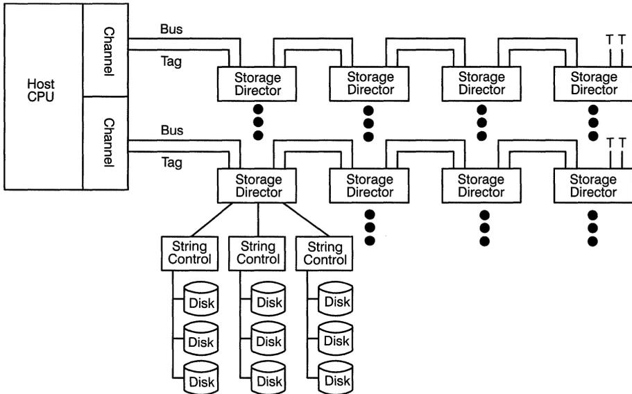
Figure 1. Block-Multiplexer Channel Subsystem
