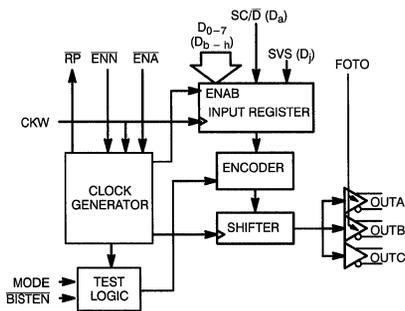
Figure 2. CY7B923 Transmitter Logic Diagram
