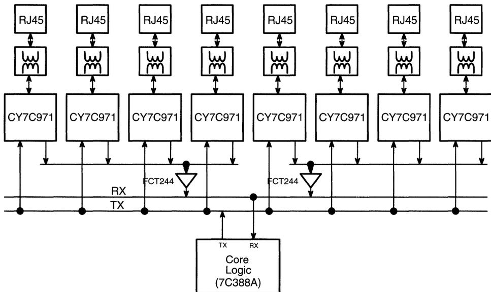
**Figure 2. Repeater Block Diagram**
