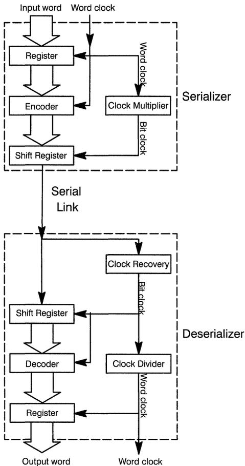
**Figure 7. Architecture of a Serial Link**
