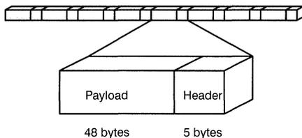
**Figure 2. ATM Cell Format**
