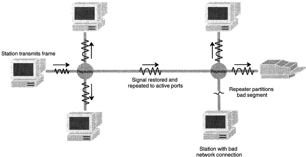
Figure 1. Ethernet Network Built with Repeaters
