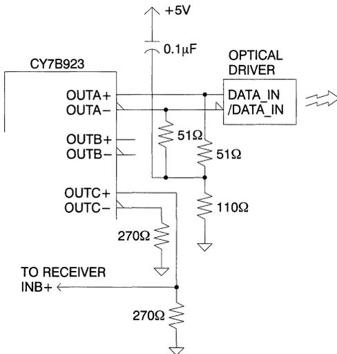
**Figure 7. HOTLink Transmitter-to-Optical Serial Interface**
