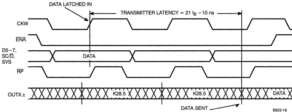
**Figure 2. CY7B923 Transmitter Data Pipeline**
