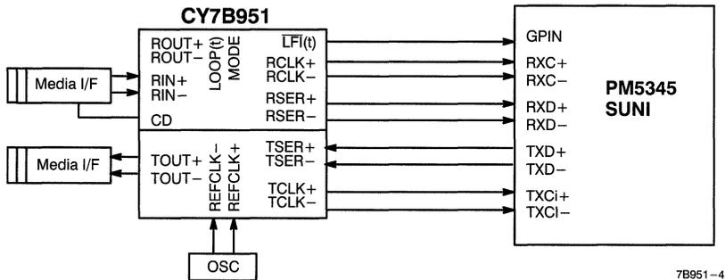
**Figure 2. CY7B951 to PMC-Sierra PM5345 SUNI Connection Diagram**
