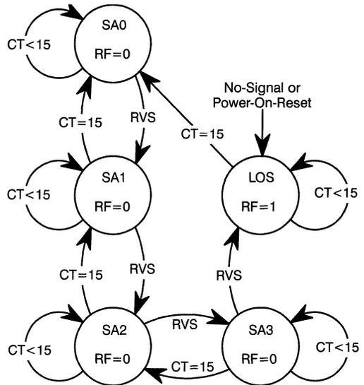
**Figure 3. Synchronization State Machine**
