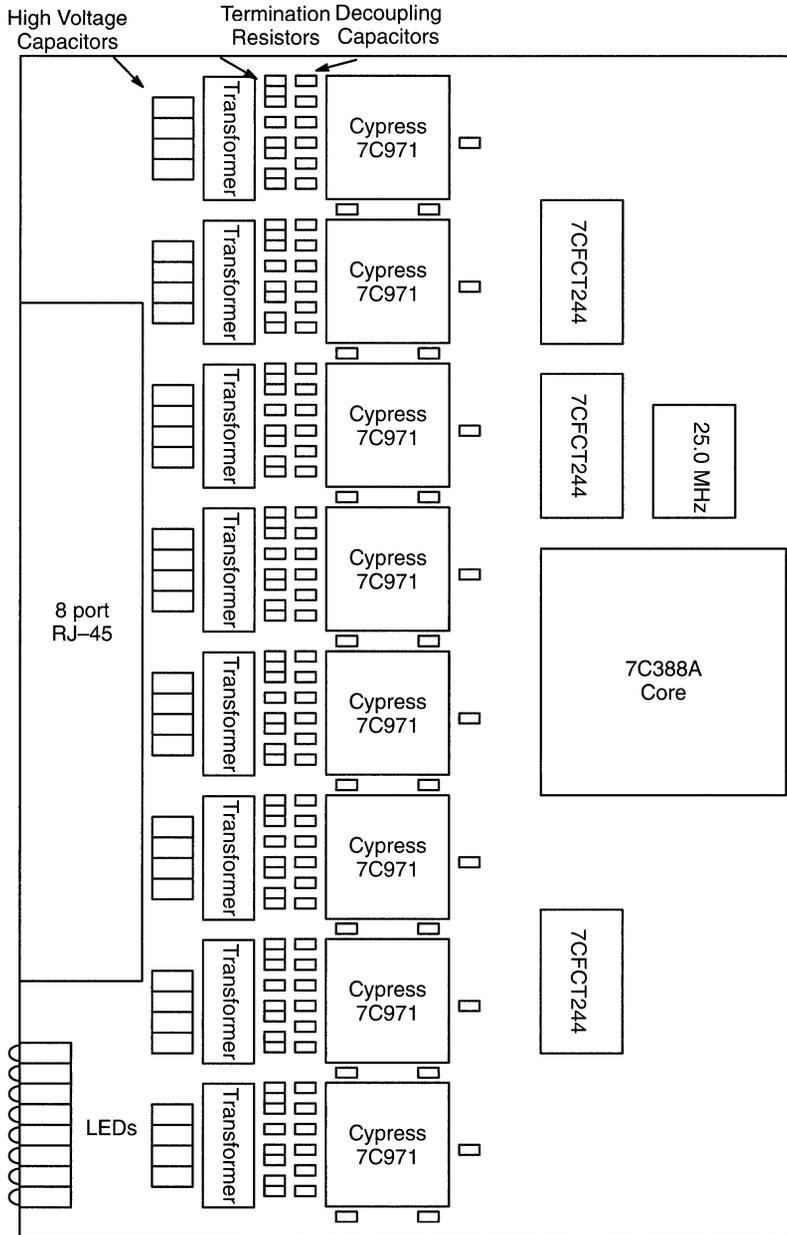
Figure 8. Component Placement
