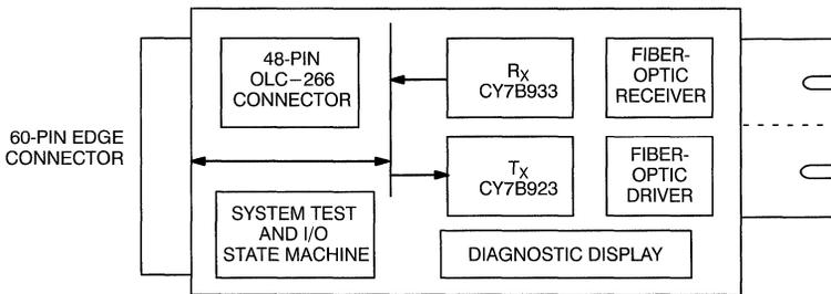
Figure 2. Fiber-Optic Interface Evaluation Board CY9266-F
