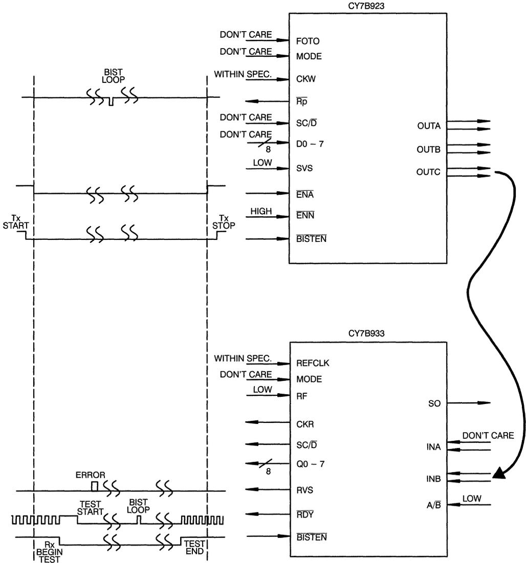
**Figure 11. Built-In Self-Test**
