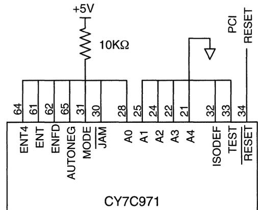
**Figure 6. Configuration Pins**
