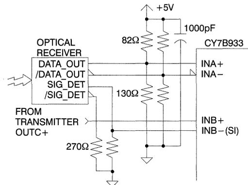
**Figure 8. Optical-to-HOTLink Receiver Serial Interface**
