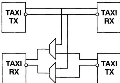
**Figure 9. Loop-Back Testing with Multiplexers**
