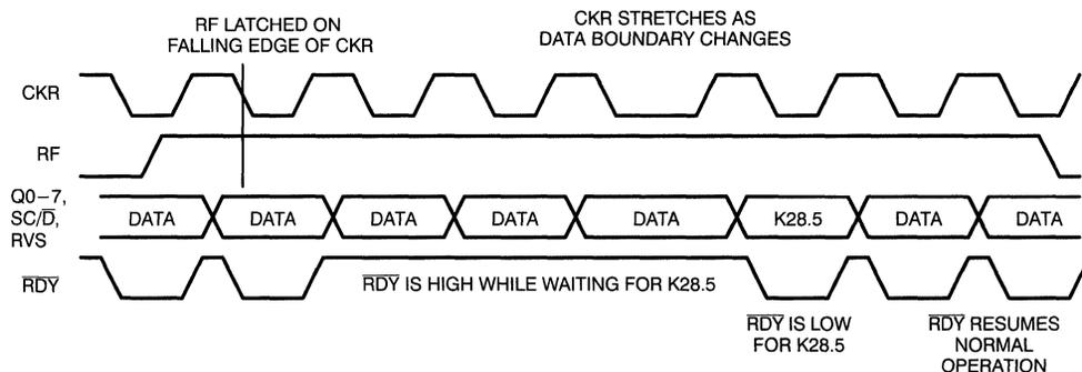
**Figure 4. CY7B933 Framing Operation in Encoded Mode**
