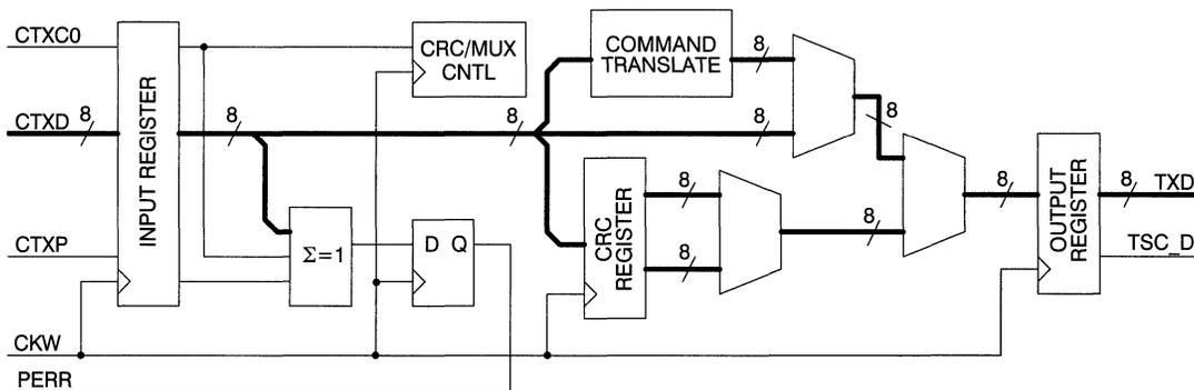
**Figure 9. pASIC Transmit Path Block Diagram**
