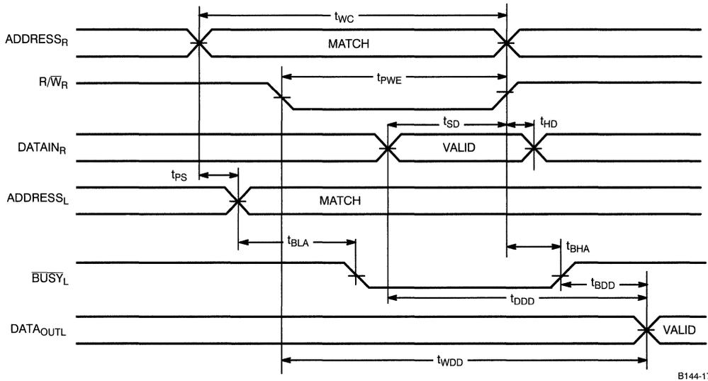
**Write Timing with Busy Input ( $\text{M}/\overline{\text{S}}=\text{LOW}$ )**
