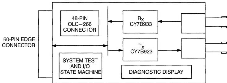
Figure 1. Copper Media Interface Evaluation Board CY9266-C
