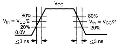
**CMOS Input Test Waveform (CY7B992)**
