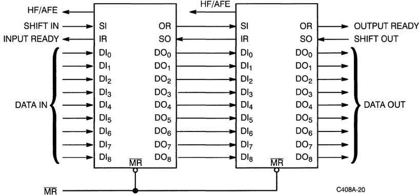
Figure 4. Cascaded Configuration at or below 25 MHz<sup>[22, 23, 24, 25, 26]</sup>
