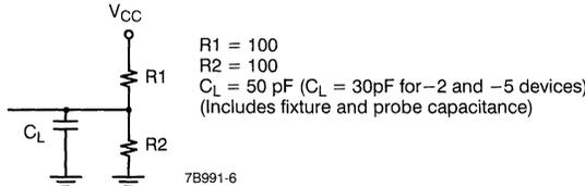
**CMOS AC Test Load (CY7B992)**
