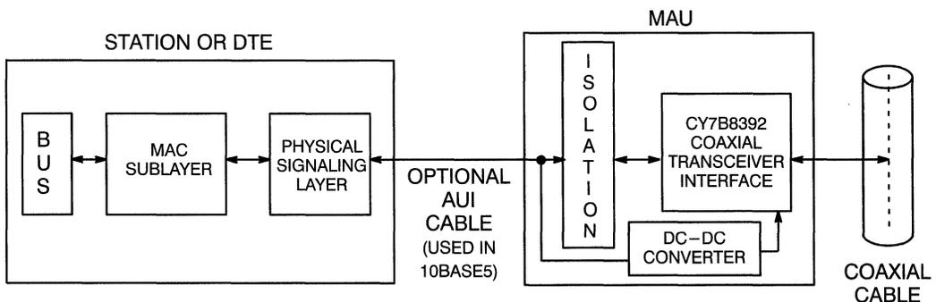
Figure 1. Block Diagram of Single Network Node
