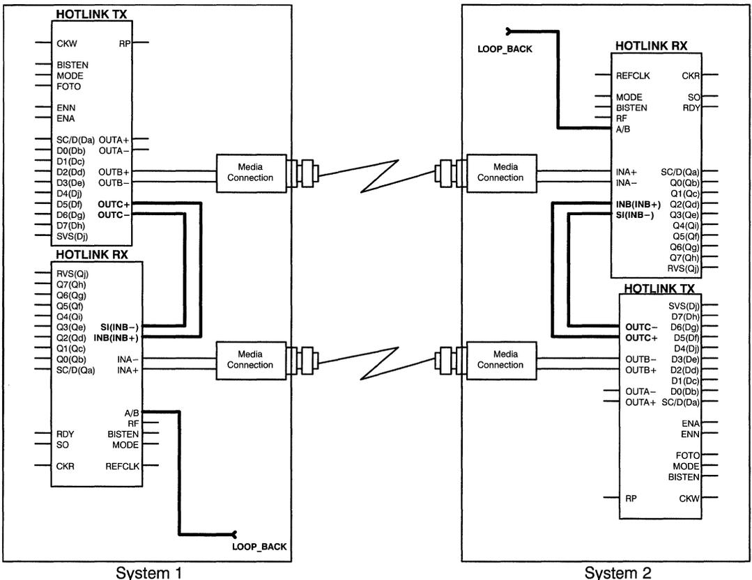
**Figure 8. Example HOTLink Loop-Back System Connection**
