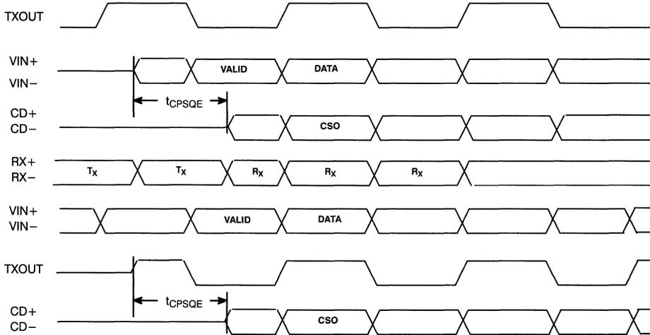
**Figure 4. Collision Timing**
