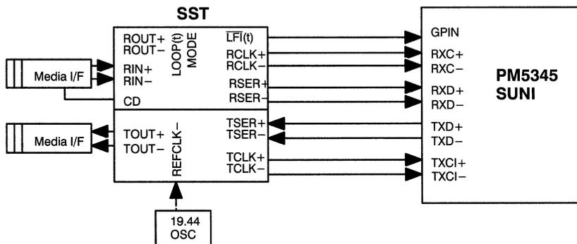
**Figure 4. SST to PMC-Sierra PM5345 SUNI Connection Diagram**
