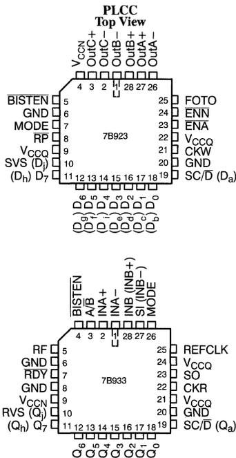
**Figure 4. CY7B923 and CY7B933 Pin Configurations**
