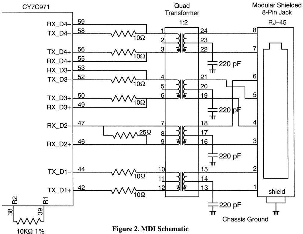
The center taps on the media side of the transformer are connected to the chassis ground through 220-pF (minimum) high-voltage (2 KV) capacitors. These capacitors help absorb common-mode noise that is picked up or generated on the twisted-pair medium. The capacitors must be capable of withstanding the isolation requirements specified in the 100BASE-T4 standard. High-voltage ceramic disc capacitors are economical and work well in this application.
