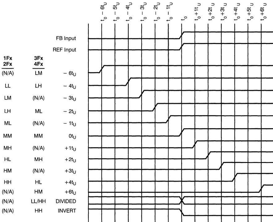
Figure 1. Typical Outputs with FB Connected to a Zero-Skew Output<sup>[4]</sup>
