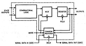
Figure 5. Diagnostic PROM Block Diagram
