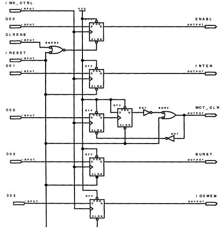
**Figure 4. Control Register Schematic**
