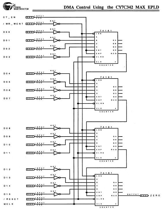
**Figure 6. Word Counter Schematic**
