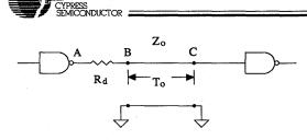
**Figure 14. Series Damping Termination**
