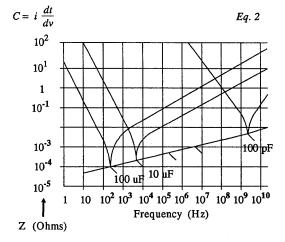
Figure 4. Capacitor Impedance Versus Frequency
