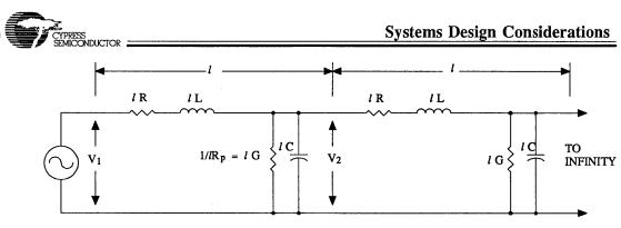
Figure 1. Transmission Line Model
