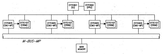
Figure 15. Fully-Extended SPARC Cache
