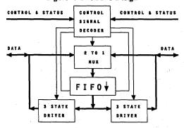
Figure 3. Switch FIFO Design
