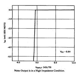
Figure 9. Output V/I Characteristics
