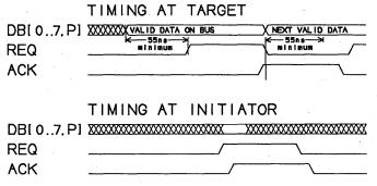
Figure 1. Asynchronous Transfer Timing, Target Transmit
