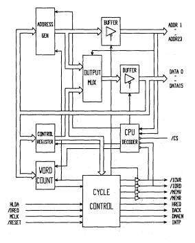
Figure 3. DMAC Block Diagram
