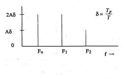
Figure 6. Fourier Transform of Periodic Pulse
