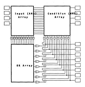
Figure 3. A Simplified FPLS Block Diagram
