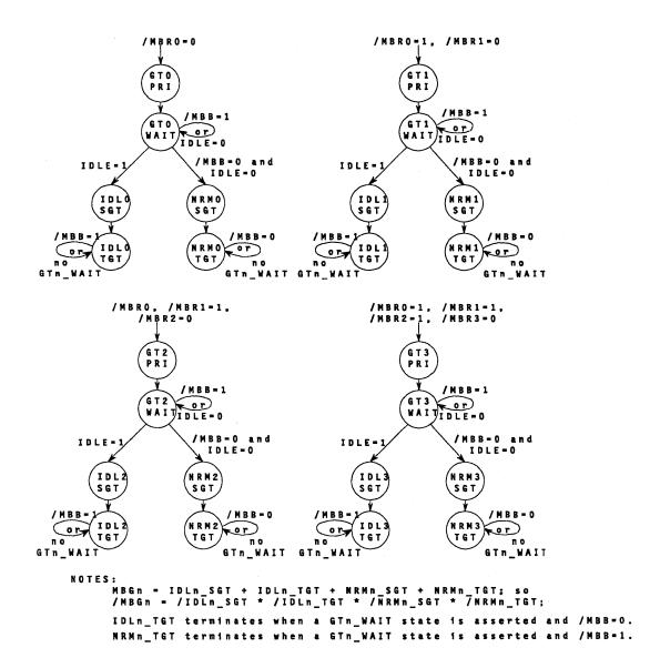
Figure 7. State Diagram of the Mbus Arbiter
