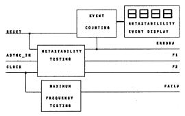
Figure 20. Metastability Test Board Block Diagram
