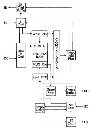
Figure 5. RAM Based FIFO Architechture
