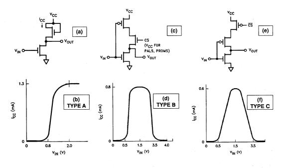
Figure 2. Three Buffer Types
