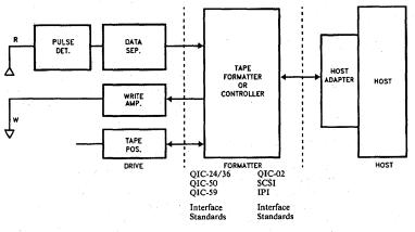
**Figure 1. Typical Tape Drive System**
