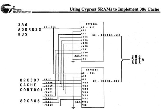
Figure 4. Operation with the 82C307
