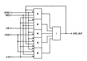
Figure 20. External ACK Gating/Latch
