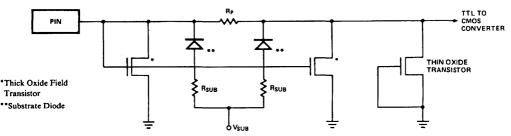
**Figure 5. Input Protection Circuit**
