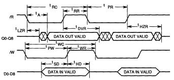
Figure 1. Asynchronous Read and Write Timing
