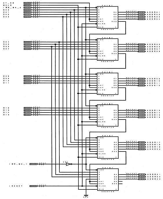
**Figure 5. Address Generator Schematic**
