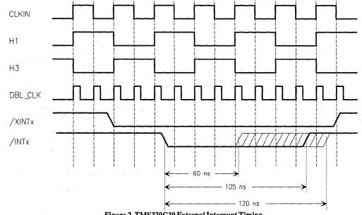
Figure 2. TMS320C30 External Interrupt Timing
