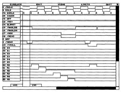
Figure 10. PLD ToolKit Simulator Output (Load)
