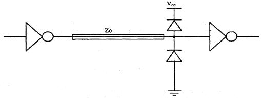
Figure 10. Diode Termination
