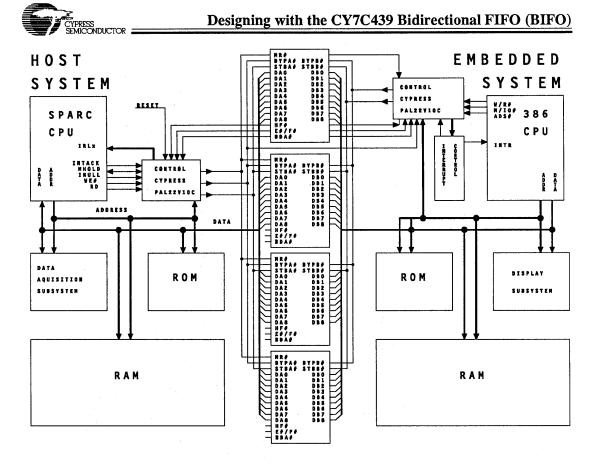
Figure 7. Design Example Block Diagram
