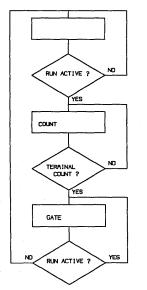
**Figure 7. Reset State Machine Flowchart**
