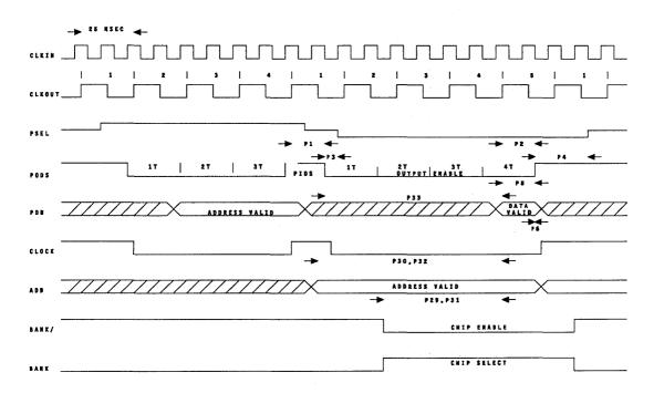
Figure 4. Address Load, Data Read
