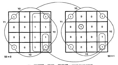
$INV = \underline{Y0} \underline{SOUT} + \underline{Y3} \underline{Y2} + \underline{Y3} \underline{Y1} \underline{Y0} + \underline{Y3} \underline{Y2} \underline{Y1} \underline{Y0} SOUT$ Figure 6. Binary Values Not Listed in *Table 1*
