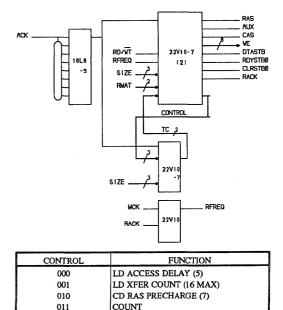
Figure 12. DRAM Control Block Diagram
