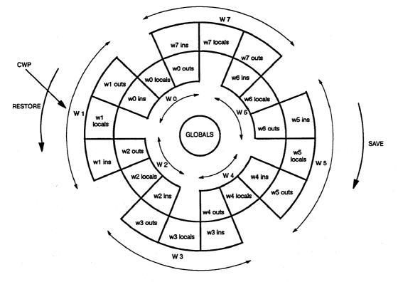
Figure 3. Register Window Concept with Eight Windows
