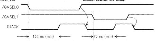
Figure 6. Timing Requirements for DTACK Circuitry
