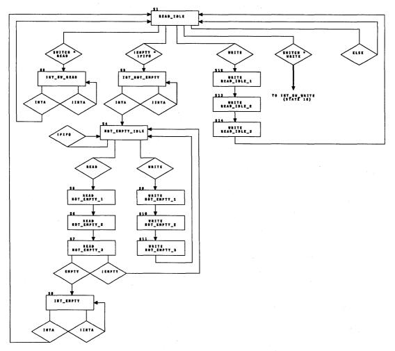
Figure 17. Reading State Diagram of the 80386 Control Logic
