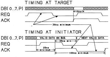
Figure 7. Fast Synchronous Transfer Timing, Initiator Transmit
