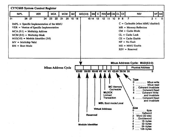
Figure 2. Module Identifier Field
