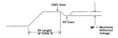
Figure 5. DELTA V Reflected Voltage Measurement
