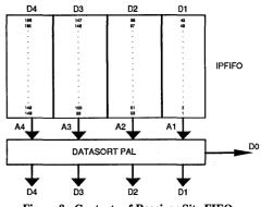
Figure 8. Contents of Receiver Site FIFO
