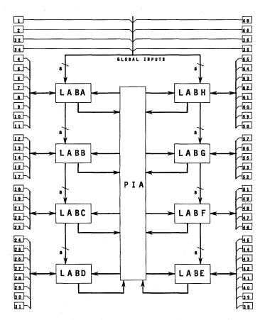
Figure 13. The CY7C342 Block Diagram.
