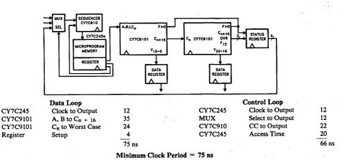
Figure 4. CY7C9101-Based 32-Bit System (Pipelined System, Add without Simultaneous Shift)
