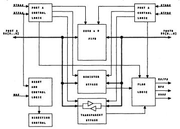
Figure 1. BIFO Block Diagram
