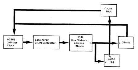
Figure 8. 80386 Cache System Critical Path
