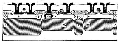
Figure 1. STAR M2 BiCMOS Process, Simplified
