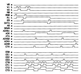
Figure 19. Synchronous Write State Register Timing
