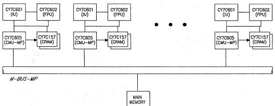
Figure 16. A SPARC Multiprocessing System
