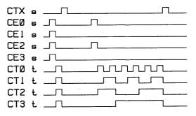
Figure 14. Delay Counter State Register Timing
