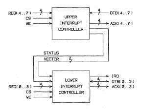
Figure 10. Cascading Interrupt Controllers
