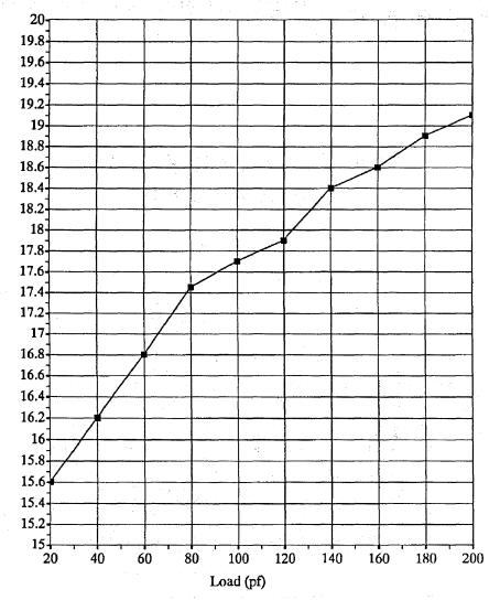
Figure 2. Delay (ns) vs Load (pF) for CY7C601
