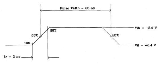
Figure 4. Setup Pulse on Channel B (nothing in the path)
