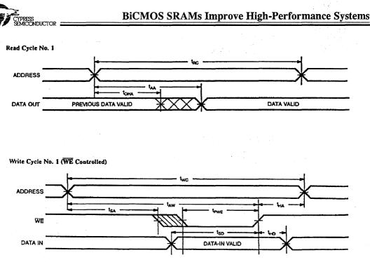
Figure 2. Balanced Read/Write Cycle Timing Diagrams
