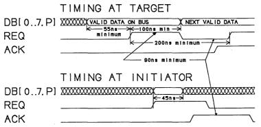
Figure 4. Synchronous Transfer Timing, Target Transmit
