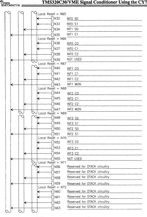
Figure 4. Resource Allocation Chart for 'C30 Interrupt Conditioner Circuit
