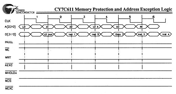
Figure 2. Load Bus Cycle
