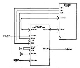
Figure 6. CPU/Pipelined Processor Interface
