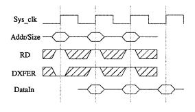
Figure 2. Load/Load Double Timing
