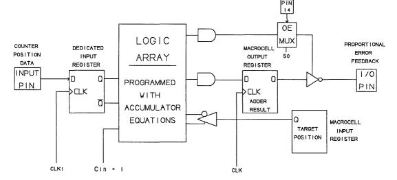
Figure 6. Control Mode Operation Sequence
