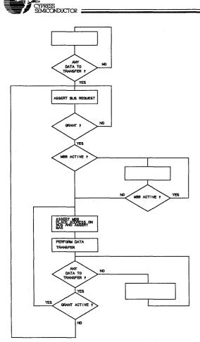
**Figure 4. Bus Arbitration Flowchart**
