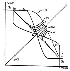
Figure 12. Energy Transfer Curves showing Trigger Paths
