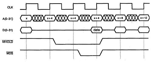
Figure 5. Wait-State Generation using MHOLD with MDS
