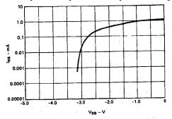
Figure 7. Bias Generator Characteristics
