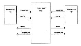
Figure 1. Dual-Processor Communication
