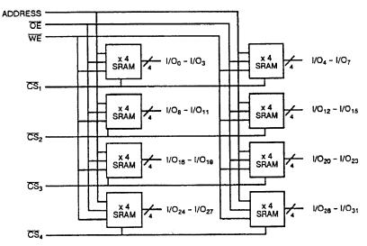
Figure 2. 64-Pin SRAM Module Block Diagram
