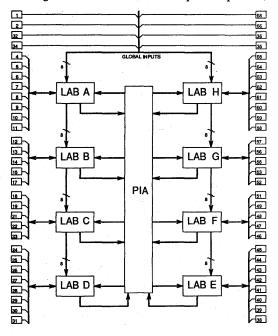
Figure 1. CY7C342 Block Diagram
