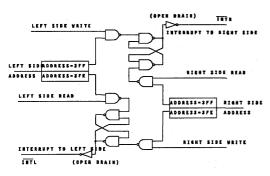
Figure 4. Interrupt Logic
