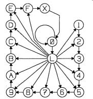
Figure 13. Loadable Delay Counter State Diagram
