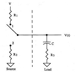
Figure 18. Lumped Load; AC Termination
