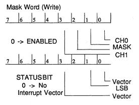
Figure 1. Data Bus Bit Assignments
