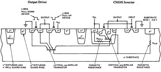
Figure 5. CMOS Cross Section and Parasitic Circuits
