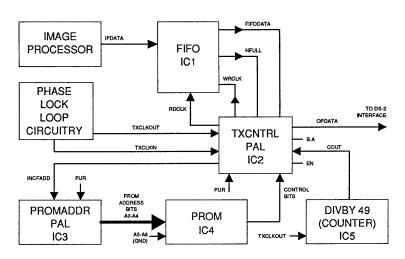
Figure 5. Transmitter Site Circuitry
