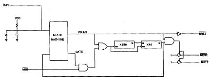
Figure 6. Watchdog Timer Block Diagram
