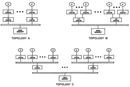
Figure 13. Multiprocessing Topologies with Multilevel Cache Hierarchies
