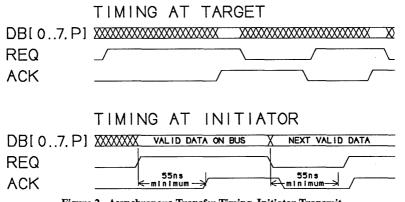
Figure 2. Asynchronous Transfer Timing, Initiator Transmit
