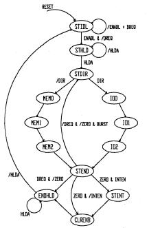
Figure 8. Cycle Controller State Diagram
