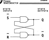
Figure 1. SR Latch, Asynchronous State Machine Example
