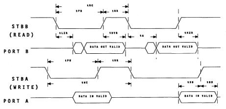
Figure 4. FIFO Read and Write Timing
