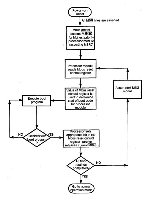
Figure 1. Boot-Up Mechanism
