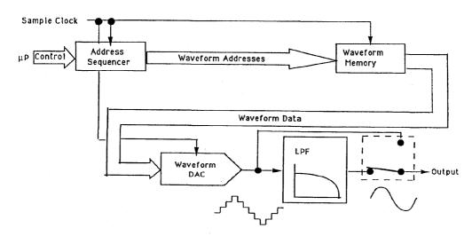
Figure 5. Waveform Synthesis System
