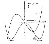
Figure 9. Energy/Force Function of a Bistable System
