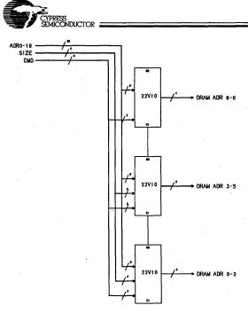
Figure 13. DRAM Address Generation Block Diagram
