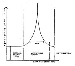
Figure 6. Output Propagation vs. Data Transition
