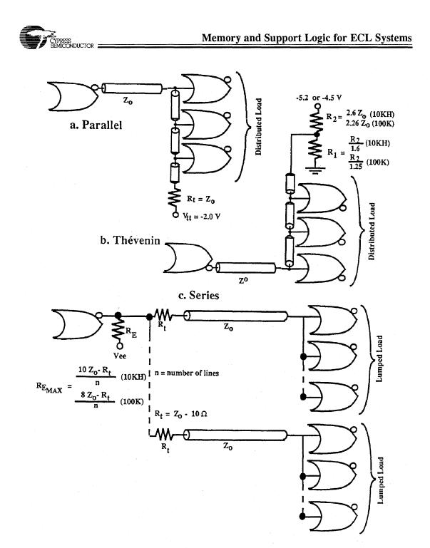
Figure 4. Three Types of Transmission Line Terminations
