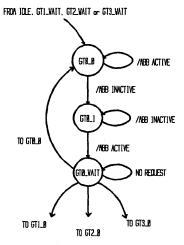
Figure 6. Bus Master 0 State Diagram.
