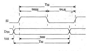
Figure 8. Input Data Timing
