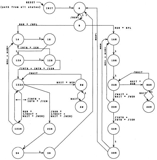
Figure 6. CPU Clock State Machine
