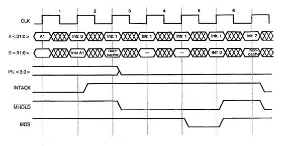
Figure 10. INTACK Frozen Due to MHOLD
