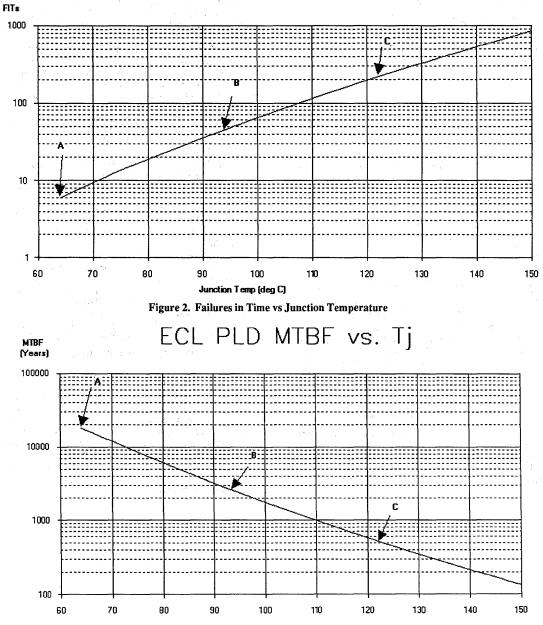
Tj.Junction Temp (deg C) Figure 3. Mean Time Between Failures vs Junction Temp.
