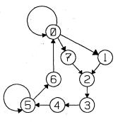
Figure 11. FIFO Read State Diagram
