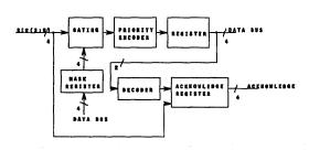
Figure 2. Interrupt Controller Block Diagram
