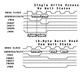
Figure 3. Mbus Data Transfer Waveforms
