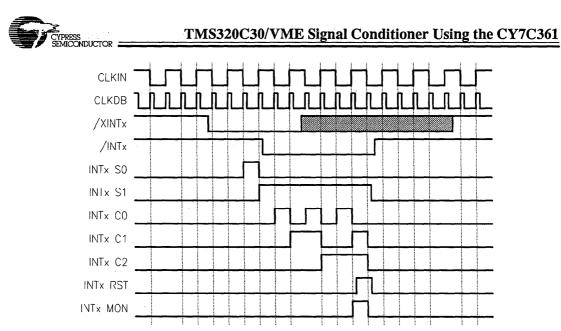
Figure 5. Output Signals for the Interrupt Controller
