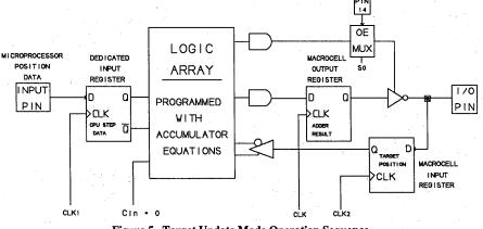
Figure 5. Target Update Mode Operation Sequence
