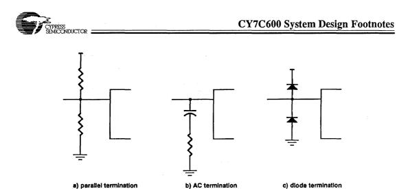
**Figure 3. Signal Termination Examples**
