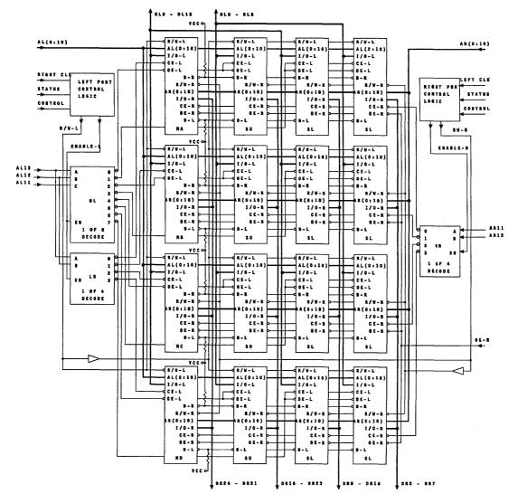
Figure 10. Logic Diagram for Dual-Port Example
