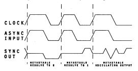
Figure 3. Possible Metastable States of Synchronizer
