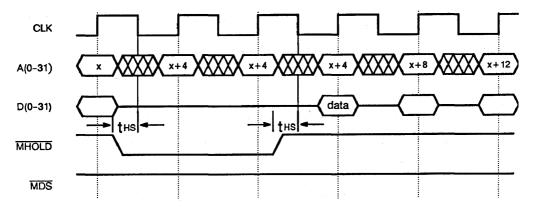
Figure 7. Wait-State Generation using MHOLD without MDS
