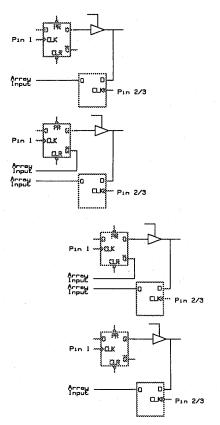
Figure 4. Four CY7C330 I/O Macrocell Configurations
