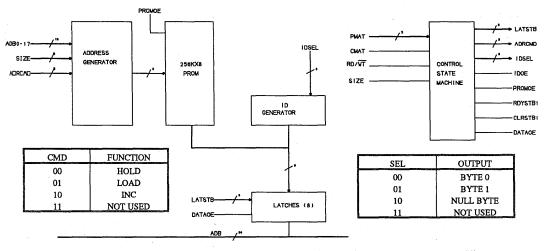
Figure 15. PROM and ID Generation Block Diagram
