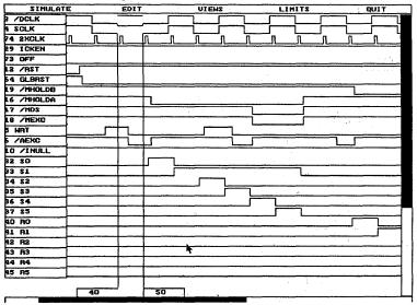
Figure 11. PLD ToolKit Simulator Output (Store)
