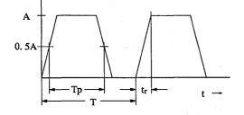
**Figure 5. Periodic Pulse Waveform**
