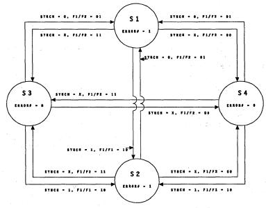
Figure 18. Metastability Testing State Diagram
