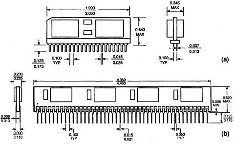
Figure 5. VDIP (a) and HVDIP (b)
