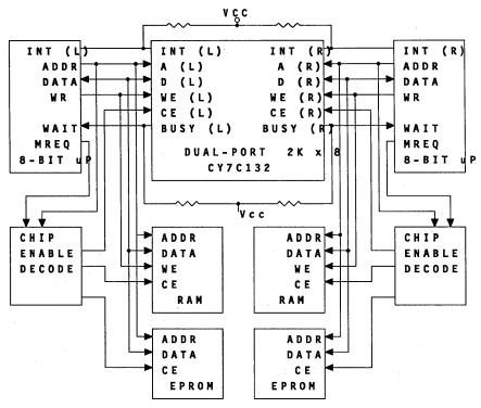
Figure 8. Typical 8-Bit Microprocessor
