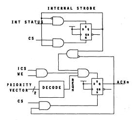
Figure 8. Internal Strobe/Acknowledge Generation
