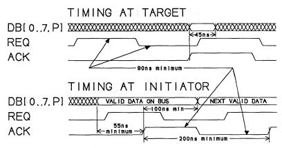
Figure 5. Synchronous Transfer Timing, Initiator Transmit
