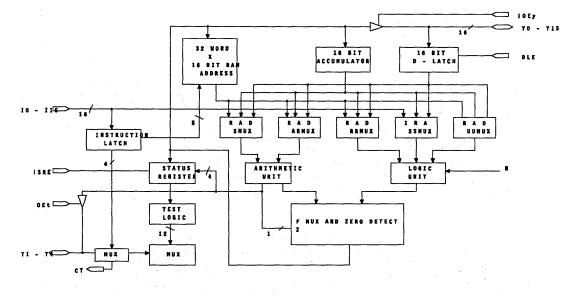
Figure 1. CY7C9116 Block Diagram
