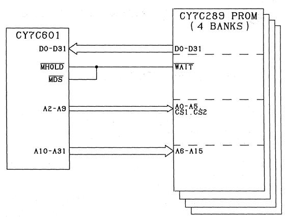
Figure 1. Block Diagram of CY7C601 Memory Design
