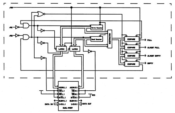
Figure 1. Block Diagram of a FIFO RAM Controller
