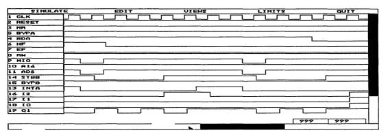
Figure 22. 80386 Control Logic Write Simulation Waveforms
