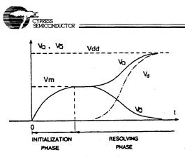
Figure 8. Two Phases of Metastability
