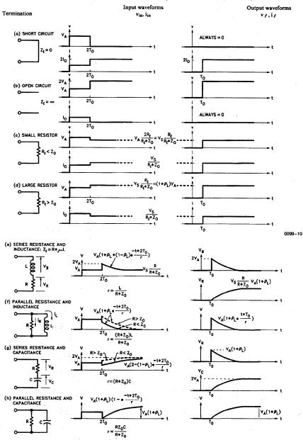
$V_A = V_S/2$ ,  $I_O = V_O/Z_O$ ,  $T_O = \ell \sqrt{LC}$ ,  $\rho L = (R_L - Z_O)/(R_L + Z_O)$
