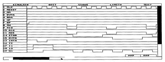
Figure 21. 80386 Control Logic Read Simulation Waveforms
