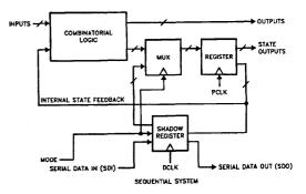
Figure 2. Simple Sequential Machine with Diagnostic Capability
