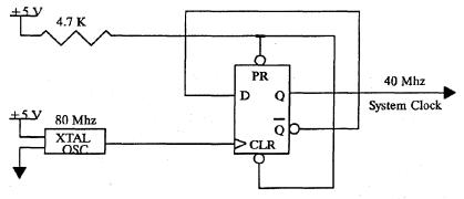
Figure 1. Symmetric-Duty-Cycle Clock Generation
