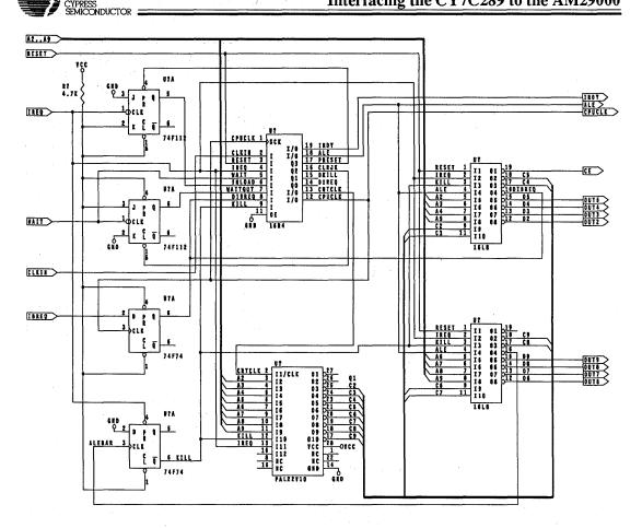
Figure 2. Control Logic for the 29000 Instruction Memory
