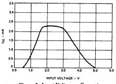
Figure 2. Input Voltage vs Current
