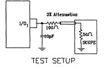
Figure 2. Test Load to Determine Taa vs CL
