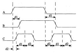
Figure 14b. Digital Frequency Doubler Timing
