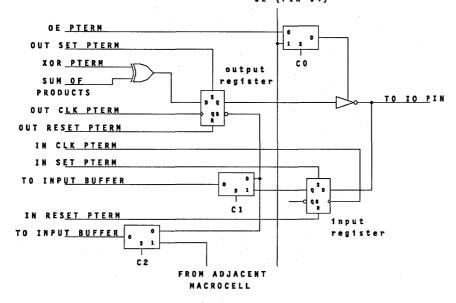
Figure 1. The CY7C331 I/O Macrocell and Shared Input Mux
