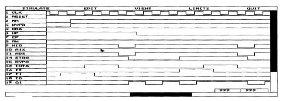
Figure 20. Master Reset Initialization -- 80386 Producer
