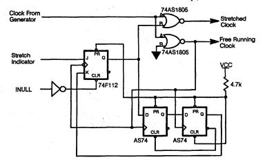
Figure 6. Simple Clock-Stretching Circuit
