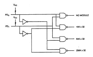
Figure 3. Depth Indicator Circuit
