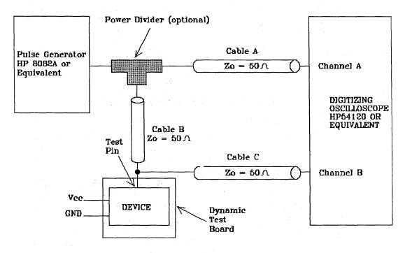
Figure 3. Test Setup for TDR Capacitance Measurement
