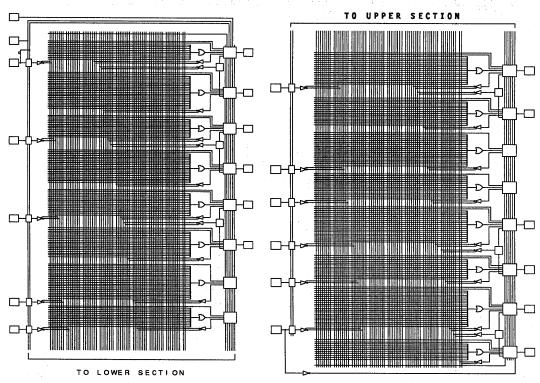
Figure 1. The CY7C330 Block Diagram
