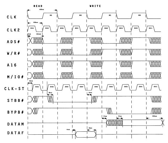
Figure 16. 80386 BIFO Control Logic Timing Diagram
