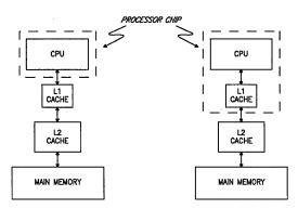
Figure 12. Multilevel Cache Hierarchy for Single-Processor Systems
