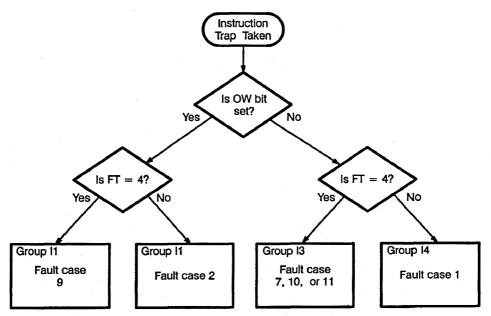
Figure 2. Instruction Access Fault Identification
