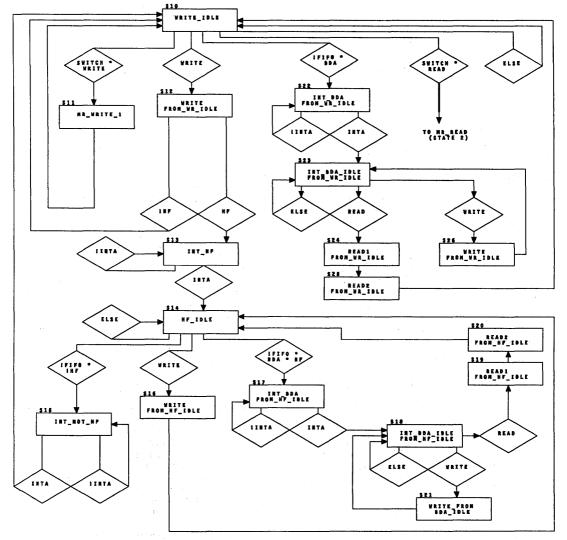
Figure 11. Writing State Diagram of the 7C601 Control Logic
