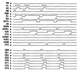
Figure 16. Asynchronous Write State Register Timing
