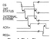
Figure 9. Timing Diagram
