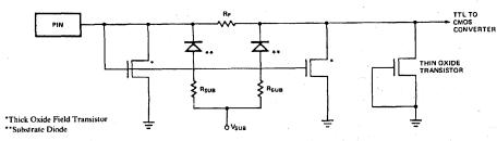
**Figure 4. Input Protection Circuit**
