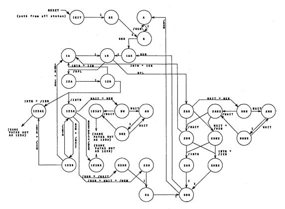
Figure 8. CY7C361 Implementation, CPU Clock State Machine
