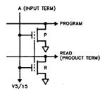
Figure 1. PAL EPROM Cell Schematic
