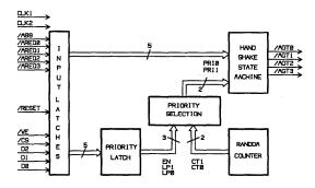
Figure 5. Arbiter Block Diagram
