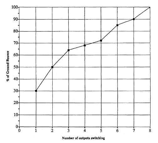
Figure 5. Ground Bounce Magnitude vs Number of Switched Outputs (from Reference 5)
