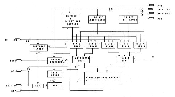
Figure 2. CY7C9117 Block Diagram
