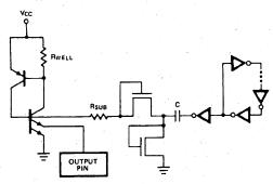
Figure 6. Parasitic SCR and Bias Generator
