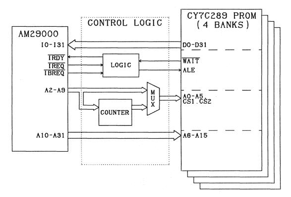
Figure 1. AM29000 Instruction Memory Block Diagram
