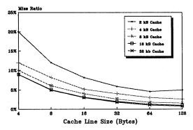
Figure 9. Cache Miss Rate as a Function of Line Size (Transposed from *Reference 10*)
