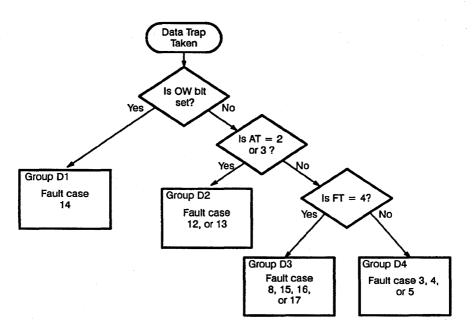
Figure 1. Data Access Fault Identification
