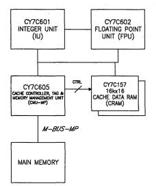
Figure 14. The SPARC Multiprocessing Cluster
