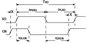
Figure 7. Output Handshaking
