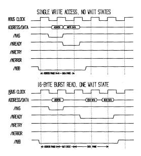
Figure 3. Mbus Data Transfer Waveforms
