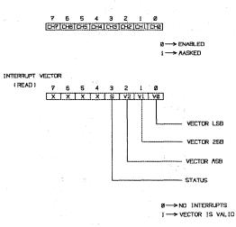
Figure 11. Extended Interrupt Vector
