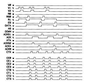
Figure 18. Fast Synchronous Write State Register Timing
