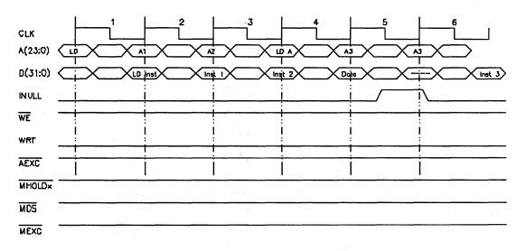
Figure 3. Load Double Bus Cycle
