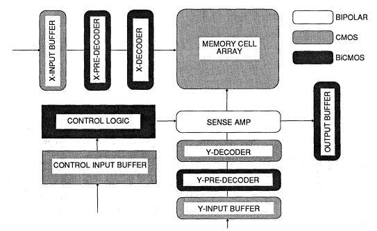
Figure 1. 64K TTL SRAM Circuit Technology
