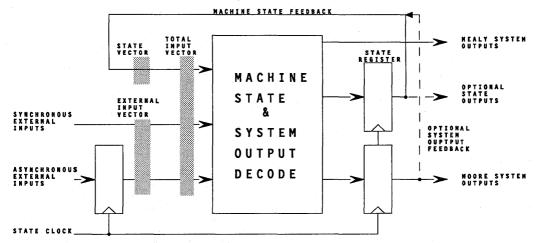
Figure 2. Synchronous State Machine Block Diagram
