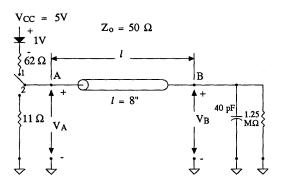
Figure 20. Equivalent Circuit for Cypress PAL Driving
