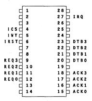
Figure 5. Interrupt Controller Pin Assignments
