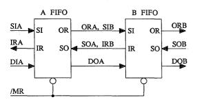
Figure 15a. Cascaded FIFOs: Intrisic Handshaking
