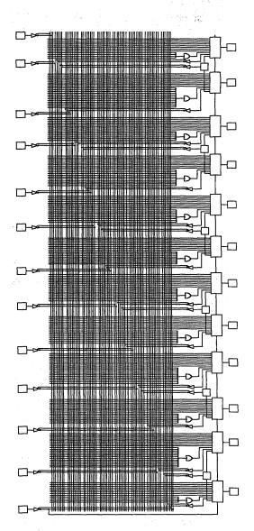
Figure 3. CY7C331 Block Diagram
