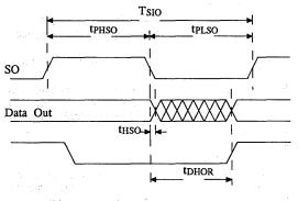
Figure 9. Output Data Timing
