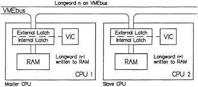
Figure 4. Block Transfer Read Cycle
