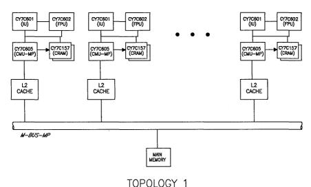
Figure 17. SPARC Single-Level Cache Extension to Multilevel Cache Topology
