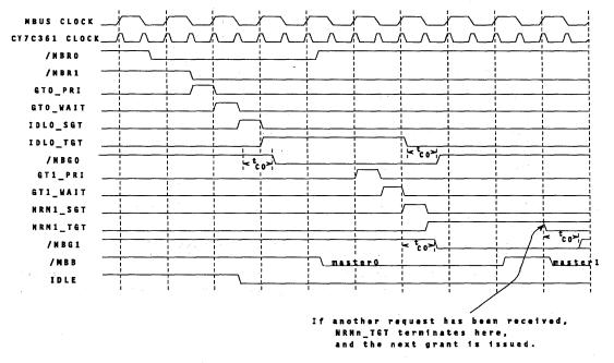
Figure 8. Handshake State Machine Waveforms
