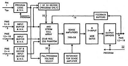
Figure 3. 16L8 Device Simplified Block Diagram
