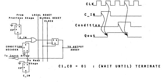
Figure 10. The TERMINATE Macrocell Configuration
