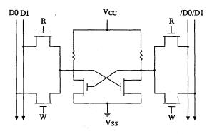
Figure 4. Dual Port RAM Cell Schematic
