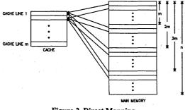
Figure 2. Direct Mapping
