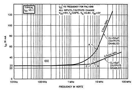
Figure 4. Typical ICC vs f
