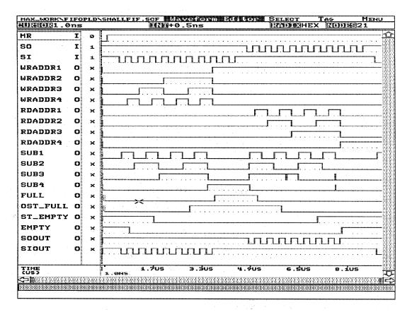
Figure 2. Sample Waveforms for the 8 Word FIFO Example
