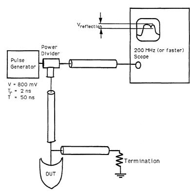
Figure 5. Time Domain Reflectometry Setup
