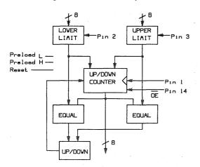
Figure 7. UP/DOWN Counter Block Diagram
