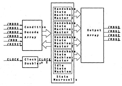
Figure 5. Arbiter Block Diagram
