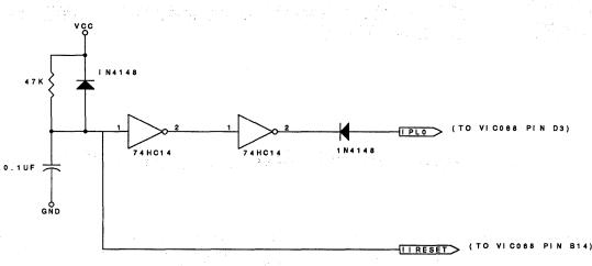
Figure 2. Global Reset Circuit
