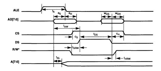
Figure 9-3b. Multiplexed Motorola Register Write Timing
