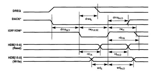
Figure 9–10. Host DMA 8-/16-Bit Interface Timing (Demand Mode)
