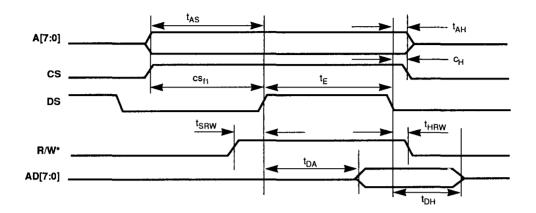
Figure 9-4a. Non-Multiplexed Register Read Timing
