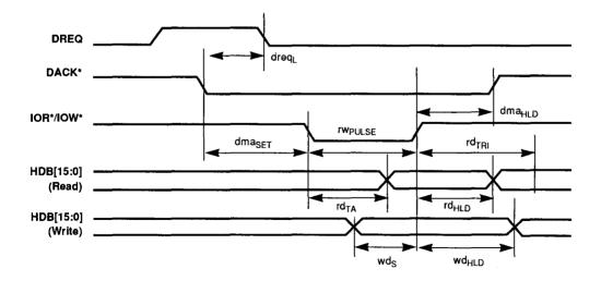
Figure 9–9. Host DMA 8-/16-Bit Interface Timing (Single-Transfer Mode)
