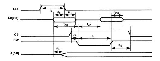
Figure 9-2a. Multiplexed Intel Register Read Timing
