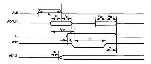
Figure 9-3a. Multiplexed Intel Register Write Timing
