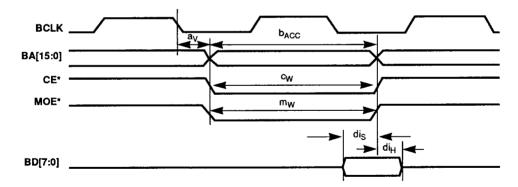
Figures 9-7a. and 9-7b. Buffer Memory Read/Write Timing Parameters
