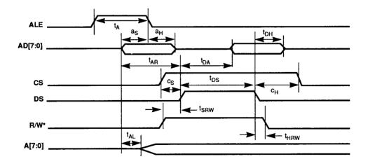
Figure 9-2b. Multiplexed Motorola Register Read Timing
