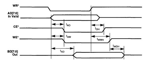
Figures 9-5a. and 9-5b. Register 70H Access Timing Parameters
