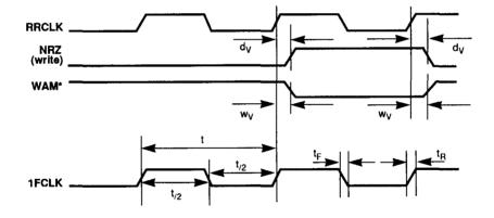
Figures 9-6a. and 9-6b. Disk Read/Write Timing Parameters
