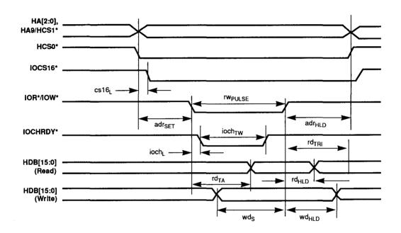
Figure 9-8. Programmed I/O, 8-/16-Bit Host Interface Timing
