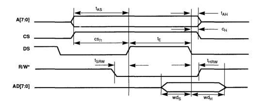
Figure 9-4b. Non-Multiplexed Register Write Timing
