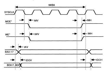
**NOTE:** tWBA is a functional parameter that gives the duration of one RAM data buffer access cycle in SYSCLK periods. The value is programmed in Bits 1-0 of Register 54H. These examples show tWBA = 4t.
