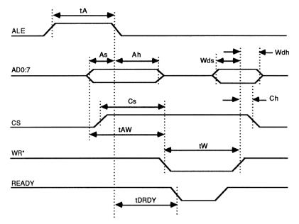
11.3.2.4 Register Write Operation in Motorola Mode
