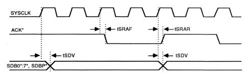
Odd Number of SYSCLK Cycles per SCSI Synchronous Transfer Period
