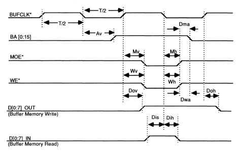
NOTES: (1) When the SCSI WRITE ENABLE or the SCSI READ ENABLE bit (Register 53H, Bits 2,3 respectively) is set, the MOE\* signal (Pin 15) will be asserted low each unused BUFCLK\* cycle until the falling (leading) edge the SCSI ACKNOWLEDGE signal (ACK\* — Pin 70).
