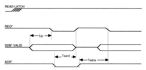
NOTE: The MOE\* signal (Pin 15) will be continuously asserted low every unused BUFCLK\* cycle while waiting for the falling (leading) edge of the SCSI ACKNOWLEDGE signal (ACK\* — Pin 70).
