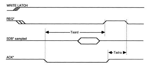
NOTE: The MOE\* signal (Pin 15) and the WE\* signal (Pin 16) will be continuously asserted low every unused BUFCLK\* cycle while waiting for the falling (leading) edge of the SCSI ACKNOWLEDGE signal (ACK\* — Pin 70).
