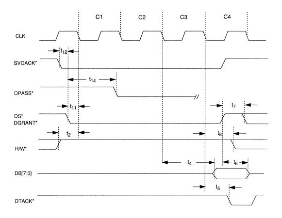
Figure 3–8. Synchronous Service Acknowledge Cycle Timing
