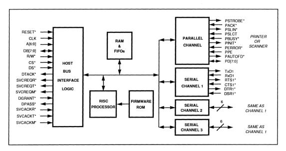
Figure 1–2. Three Serial Ports and One Parallel Port
