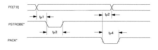
Figure 3–9. Parallel Port Transmit Timing
