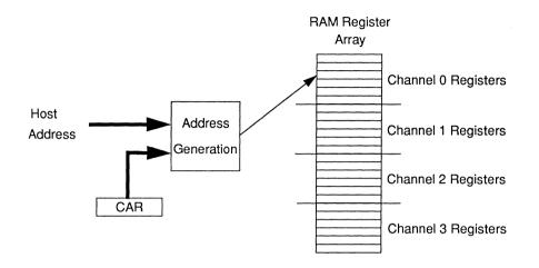
Figure 4–2. Internal Address Generation
