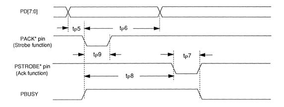
Figure 3–10. Parallel Port Receive Timing
