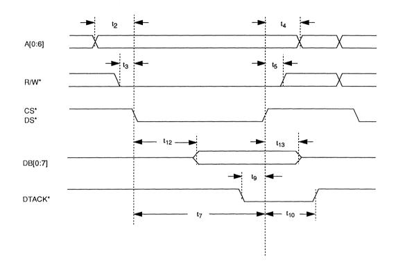
Figure 3-4. Asynchronous Write Cycle Timing
