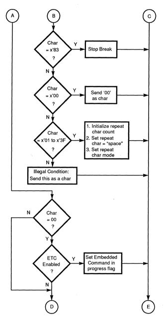
Figure 4-7. CL-CD1400 Transmit Character Processing (cont.)
