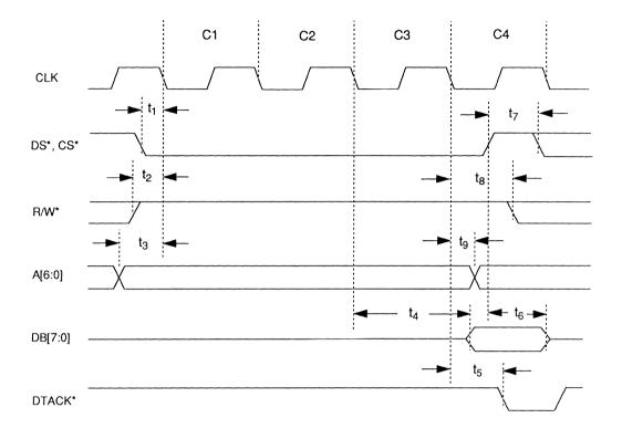
Figure 3–6. Synchronous Read Cycle Timing
