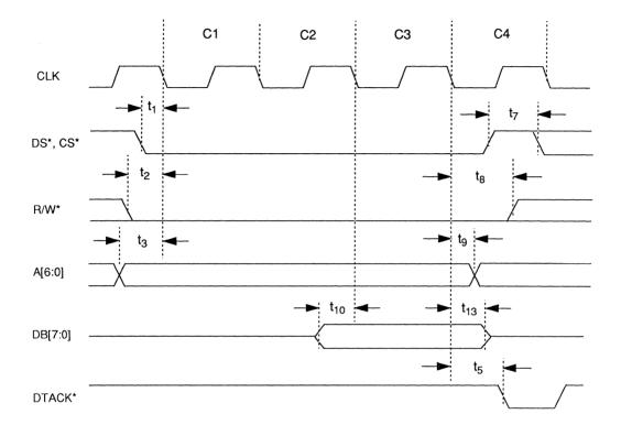
Figure 3–7. Synchronous Write Cycle Timing
