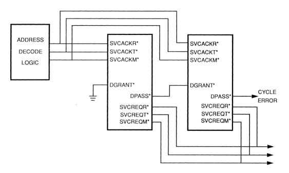
Figure 4-4. CL-CD1400 Daisy-Chain Connections
