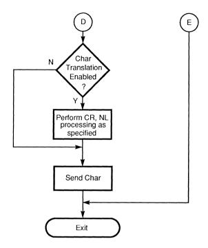
Figure 4-7. CL-CD1400 Transmit Character Processing (cont.)
