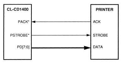
Figure 4–8. CL-CD1400 Parallel Data Transmit Connections
