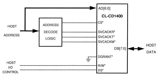
Figure 4–3. Control Signal Generation
