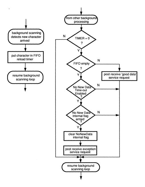
Figure 4–5. FIFO Timer Processing
