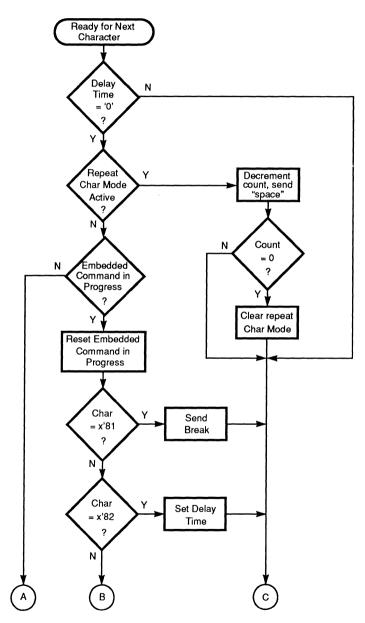
Figure 4–7. CL-CD1400 Transmit Character Processing
