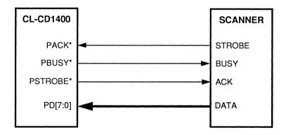
Figure 4–9. CL-CD1400 Parallel Data Receive Connections
