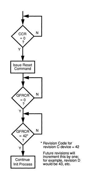
Figure 6–1. Flow Diagram of CL-CD1400 Master Initialization Sequence
