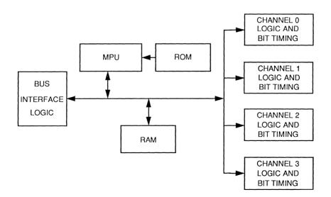
Figure 4–1. CL-CD1400 Functional Block Diagram
