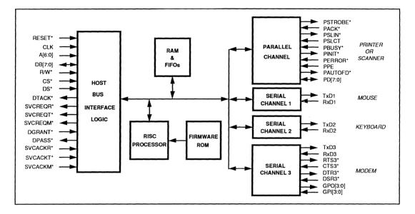
Figure 1–1. Workstation: Printer, Keyboard, Mouse and Modem Ports
