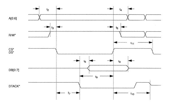
Figure 3–3. Asynchronous Read Cycle Timing
