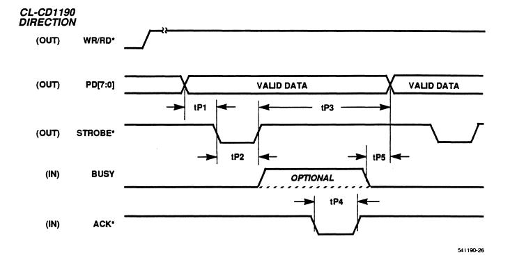
**NOTE:** The CL-CD1190 does not require that the receiver generate a BUSY. If present it will use it as a hand-shake signal; otherwise transfers happen continuously: setup, strobe, hold, setup, strobe, hold, etc.
