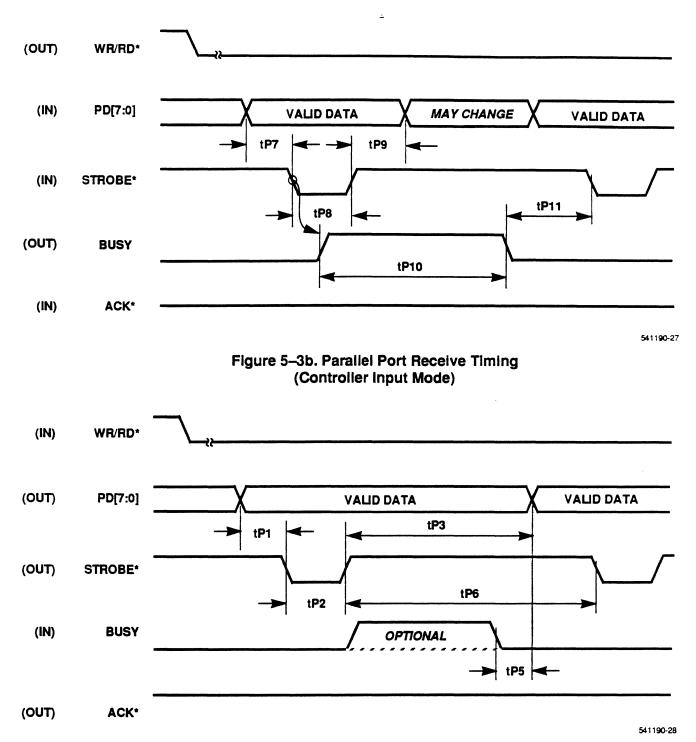
**NOTE:** The CL-CD1190 does not require that the receiver generate a BUSY. If present it will use it as a hand-shake signal; otherwise transfers happen continuously: setup, strobe, hold, setup, strobe, hold, etc.
