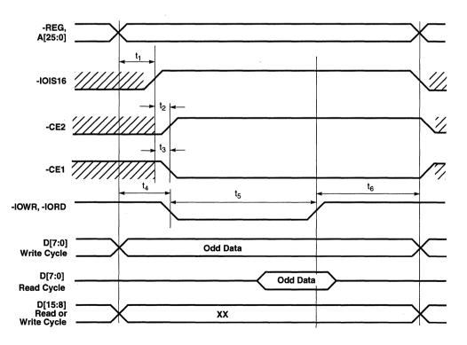
Figure 13–10. 16-Bit System to 8-Bit I/O Card: Odd Byte Timing
