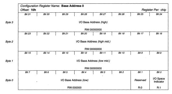
This is the PCI I/O address space base address for the Operation registers.
