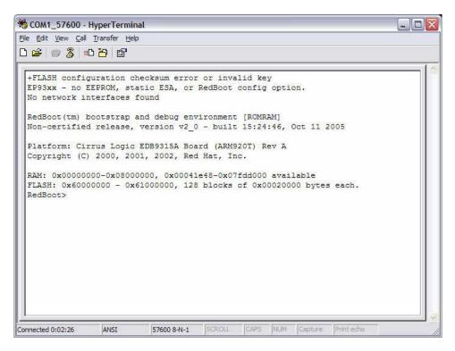
Note: The initial error about configuration checksum error is expected for a brand new board or a board where the Flash device has been completely erased. This happens because the Flash memory has not been initialized for redboot yet.
