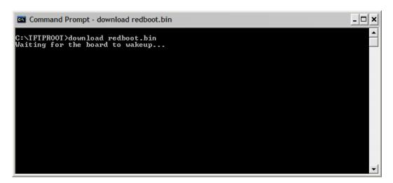
2. At this point, the download program is waiting for the user to press AND hold down pushbutton S2 SERIAL BOOT. While holding down S2, press and release pushbutton S3 /POR. Keep holding down S2 until red LED, D2 (next to the flashing green LED) is no longer illuminated. Afterwards, release S2. You should then see the following in the Command Prompt window.
