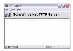
Note: Note: You may get an IP address of 127.0.0.1 because the EDB9315A board does not have the boot loader code programmed yet. This is ok. Simply quit the TFTP server program. Instructions on when to start the program will be given during the board programming section. If an IP address other then the one above appears, the Ethernet port is connected to something and should be removed.
