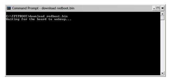
2. At this point, the download program is waiting for the user to press AND hold down pushbutton S1 SERIAL BOOT. While holding down S1, press and release pushbutton S3 /POR. Keep holding down S1 until red LED D2 (next to the flashing green LED) is no longer illuminated. Afterwards, release S1. You should then see the following in the Command Prompt window.
