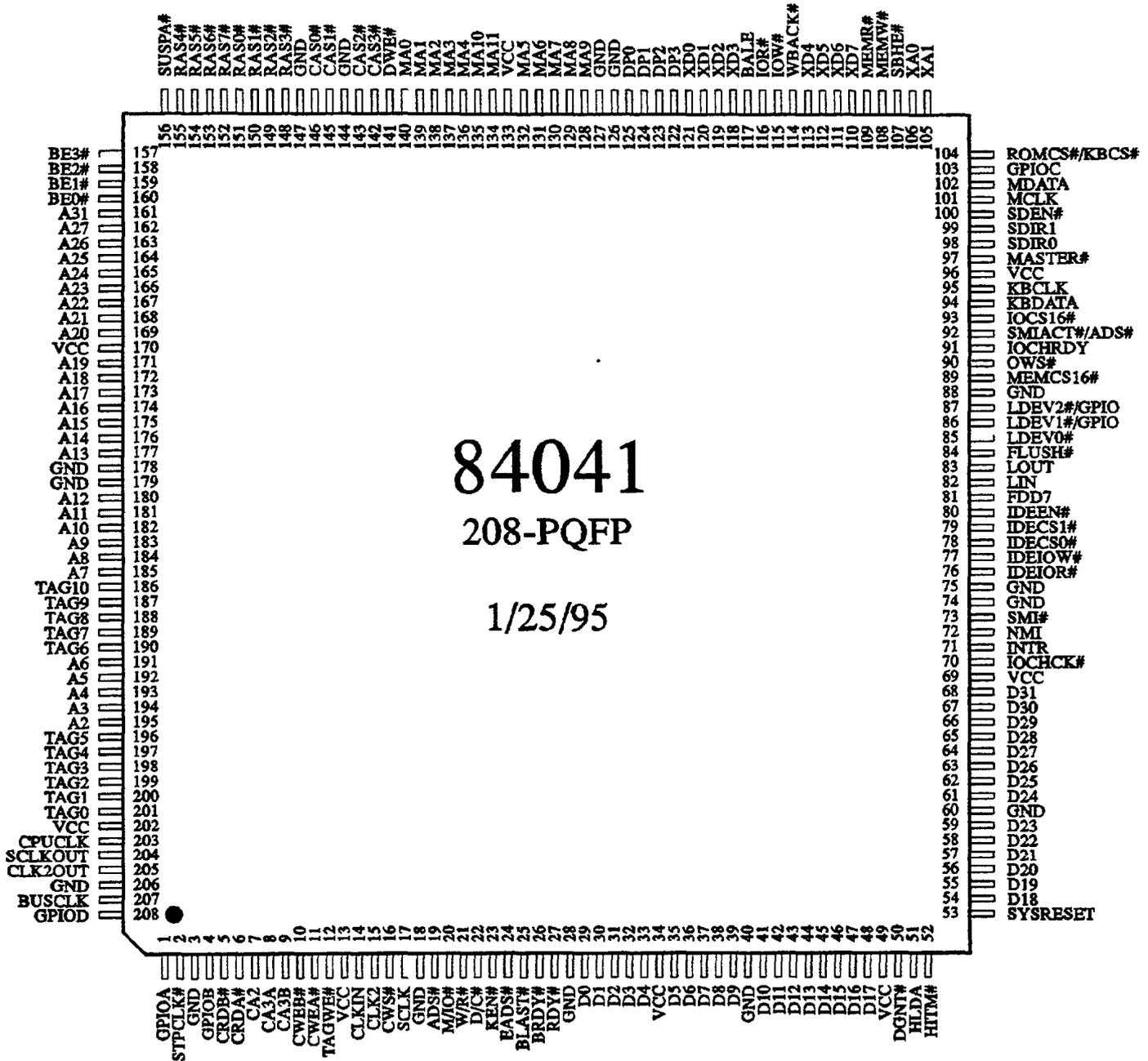
Figure 2.1: 84041 Pinout
