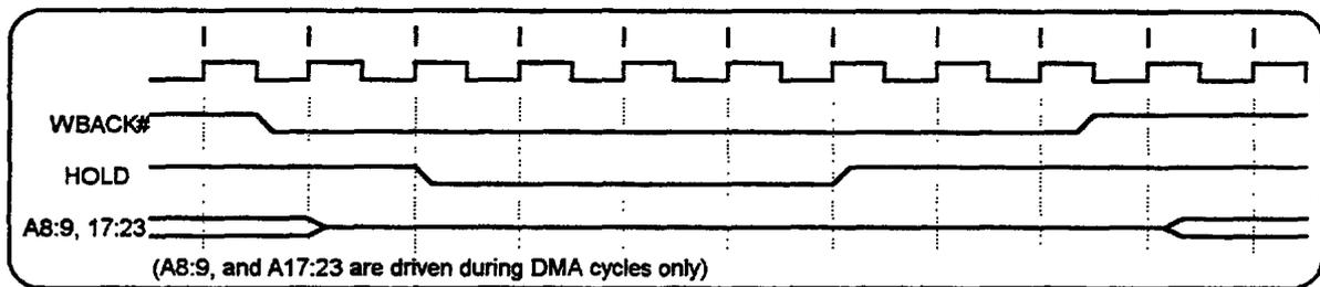
**Figure 6.1 WBACK# Timing**
