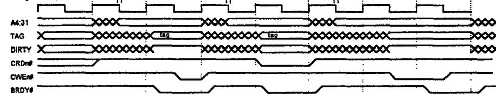
Note: The 1WS option for clean-to-dirty tag write is not currently implemented. It is included for general illustration only. The clean-to-dirty tag write is always 2WS.
