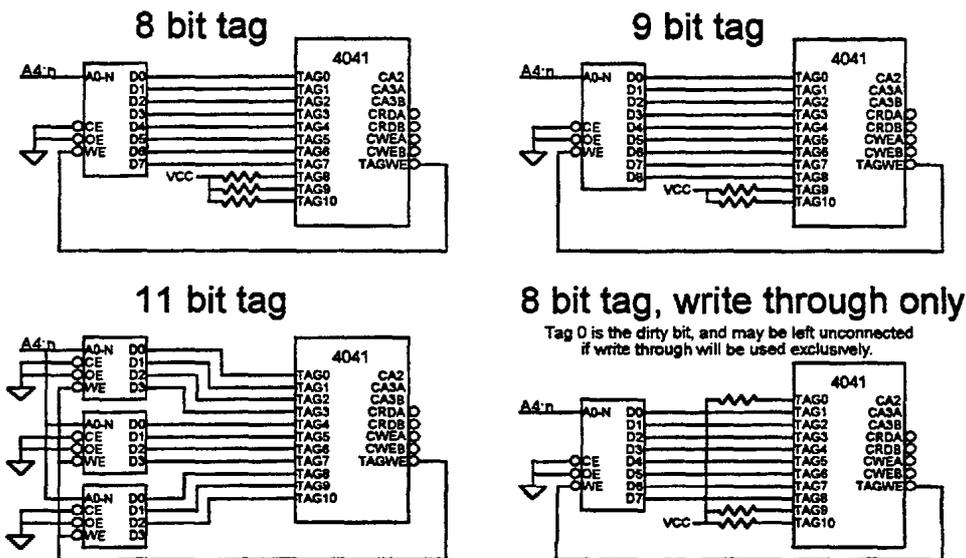
Figure 5.4: Cache Tag RAM Connections
