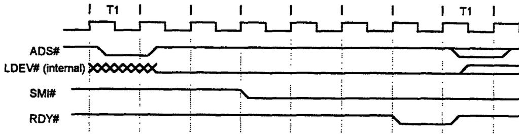
**Figure 5.19: I/O Restart Timing**
