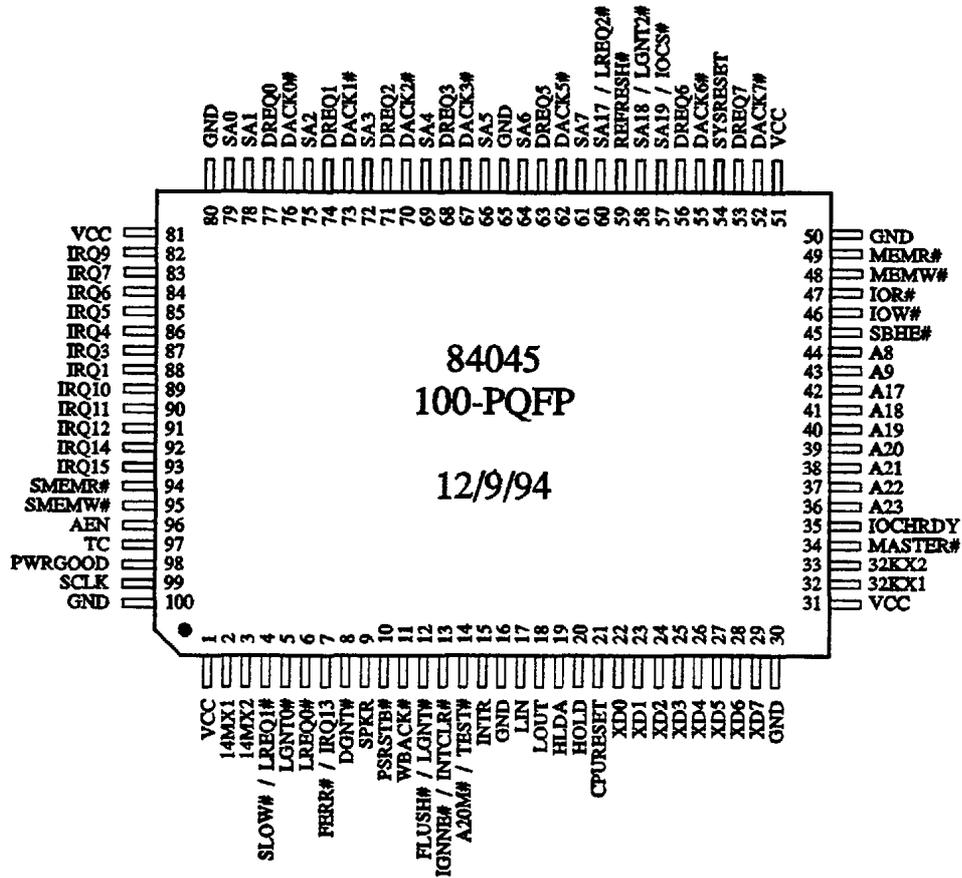
**Figure 2.2: 84045 Pinout**
