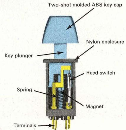
Reed switch key module is available with one or two Form A reed switches.
