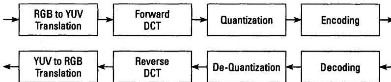
**Figure 1-1 Basic Image Compression Scheme for Coder and Decoder**
