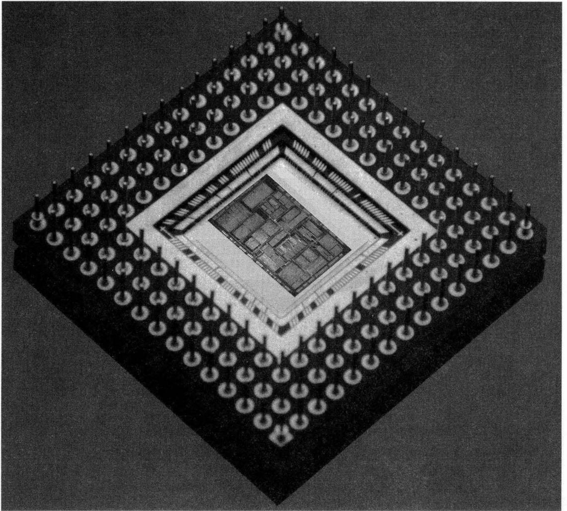
*The CL560 is the successor to the CL550, which was the world's first JPEG processor when it was introduced in 1990. Both products are high-performance single-chip JPEG processors that encode and decode gray-scale and color images at video rates.*
