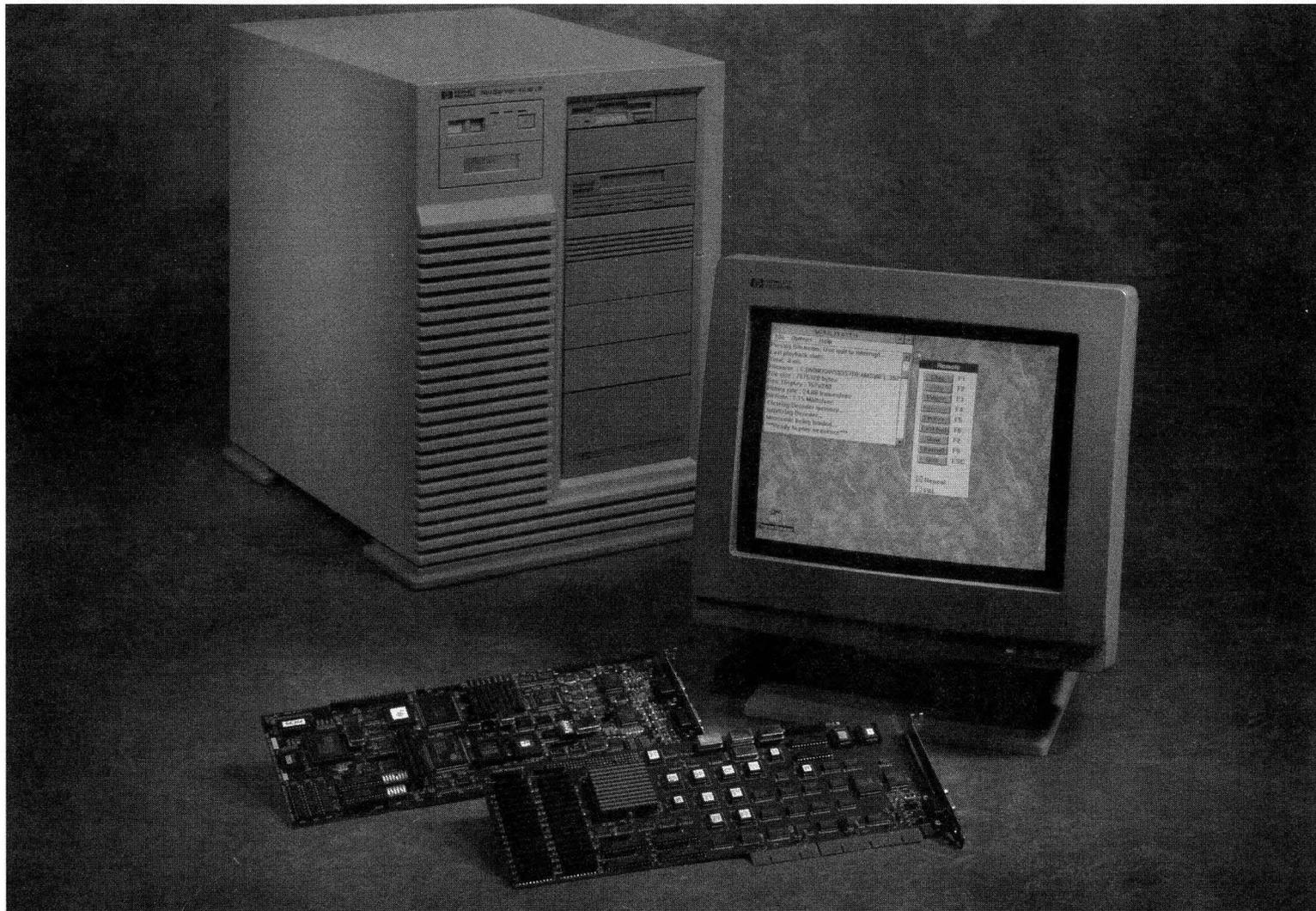
*C-Cube's MPEG Video Lab decodes and previews MPEG bitstreams at up to 8 megabits per second.*
