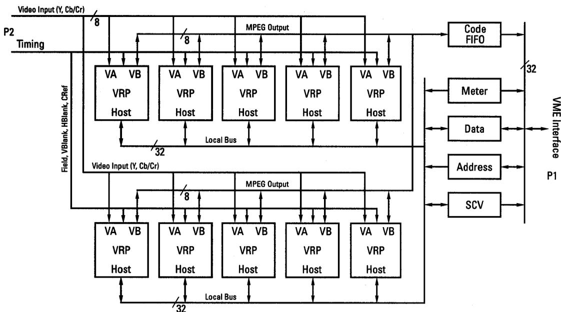
**Figure 6-1 CLM460x-Based Video Encoding System**
