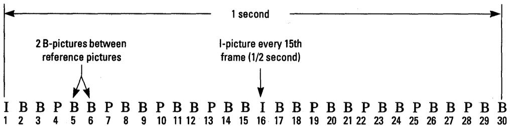
**Figure 2-7 Typical Display Order of Picture Types**
