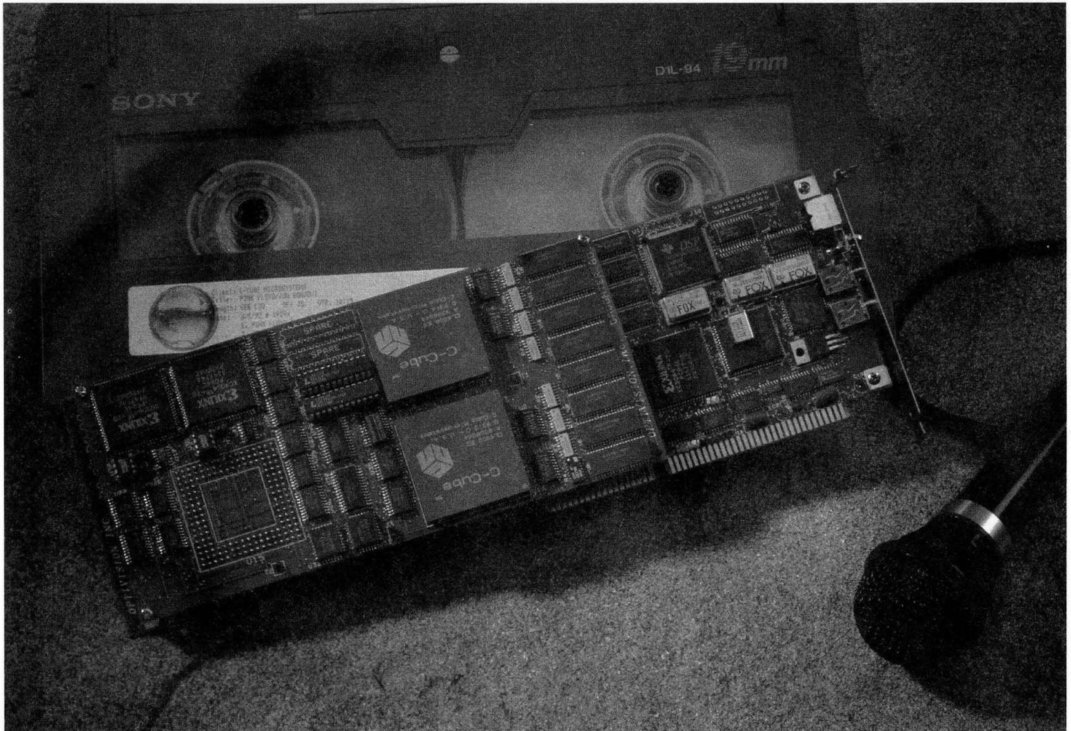
*The CLM4500 uses two VideoRISC Processors to compress digital video into SIF-resolution MPEG bitstreams in real time. The product pictured above is the OPTIVideo™ board from OPTIVISION, Inc.*
