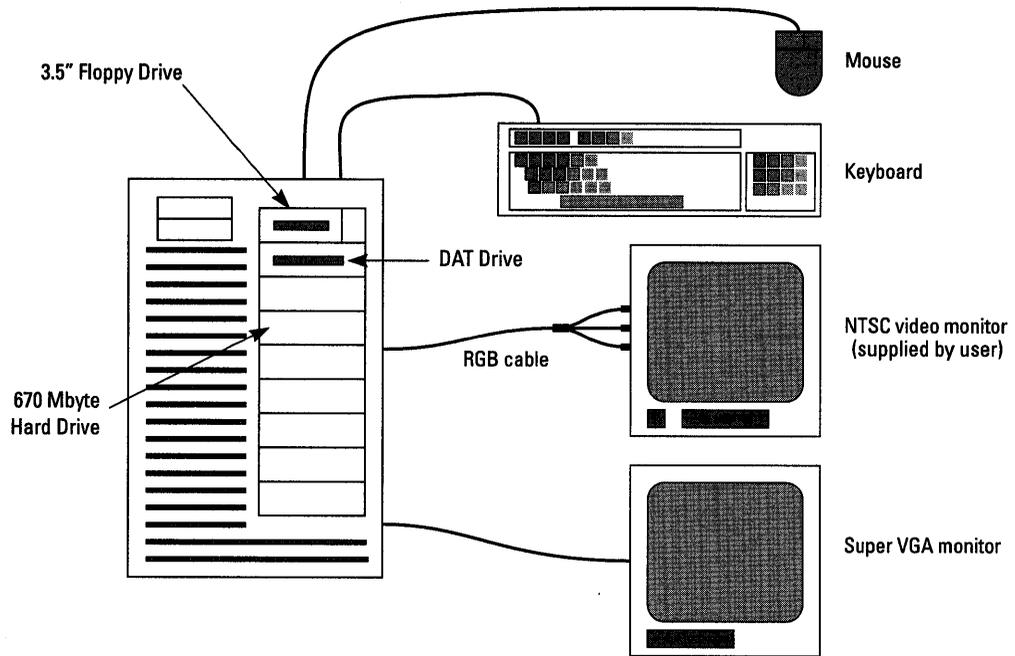
**Figure 10-1 Video Lab Components**
