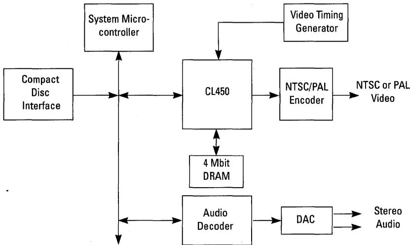
**Figure 8-2 Typical CL450 System Application**
