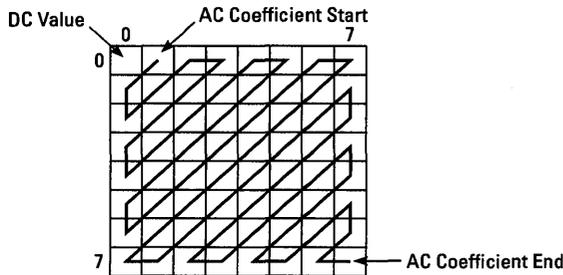
**Figure 1-4 Zigzag Reordering of the 8x8 DCT Coefficients**
