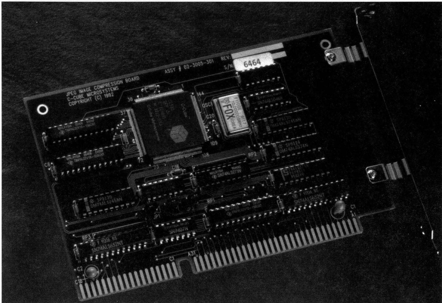
*C-Cube's JPEG Still-Image Board is an ISA-bus card that compresses and decompresses graphic images using the CL550 JPEG Processor.*
