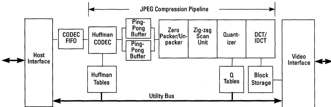
**Figure 3-2 CL560 Block Diagram**
