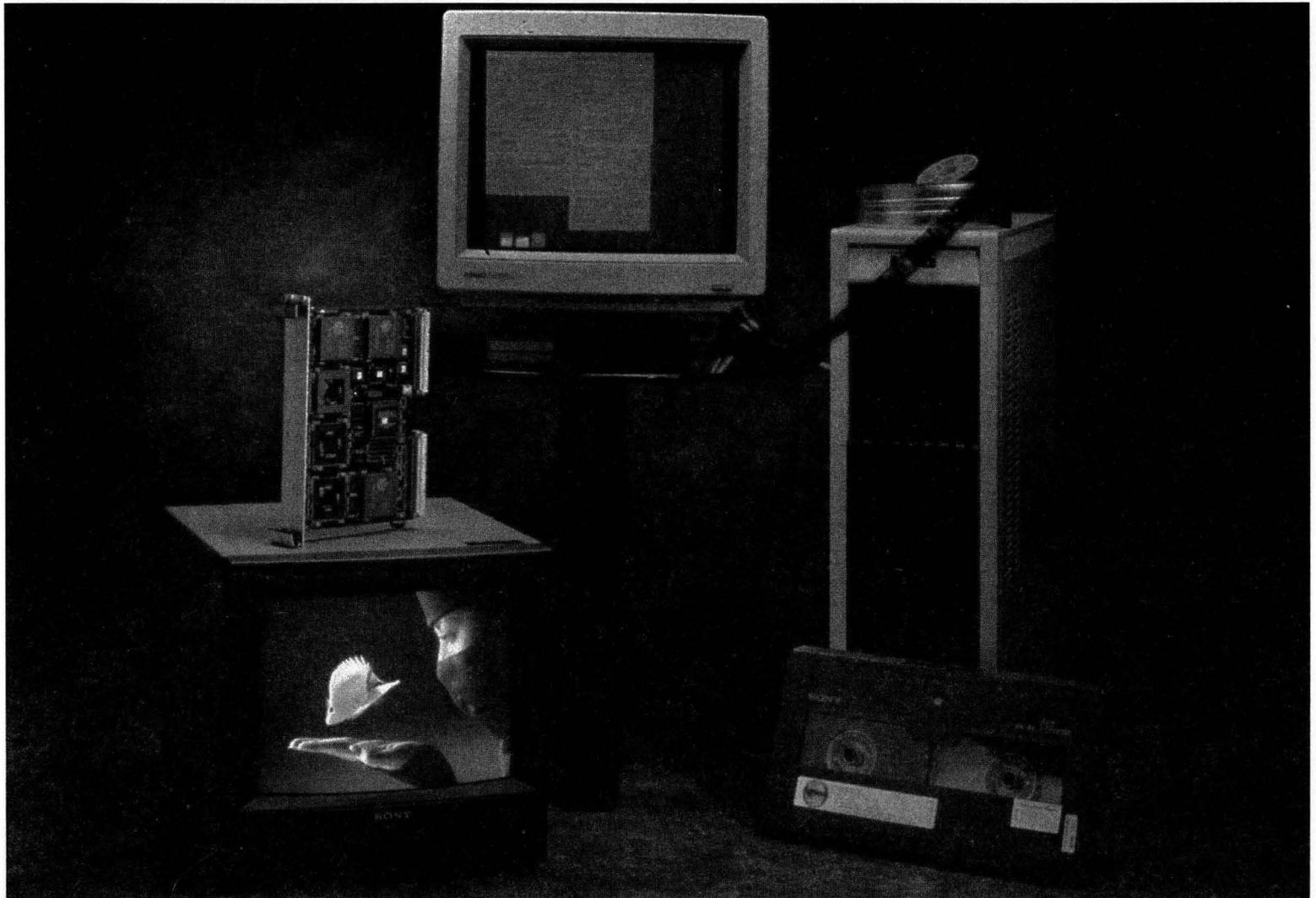
*The MPEG Encoder Development Station uses the CLM4600 to encode video and audio sequences into MPEG 1 syntax in real time.*
