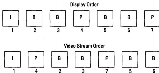
**Figure 2-8 Video Stream versus Display Ordering**
