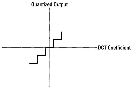
**Figure 1-2 Quantizer Stepping (Uniform Quantization)**
