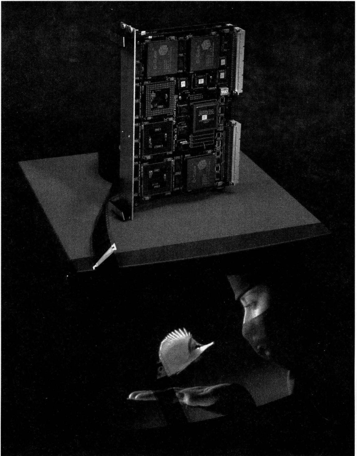
*The CLM4600 compresses digital video into MPEG syntax for broadcast applications.*
