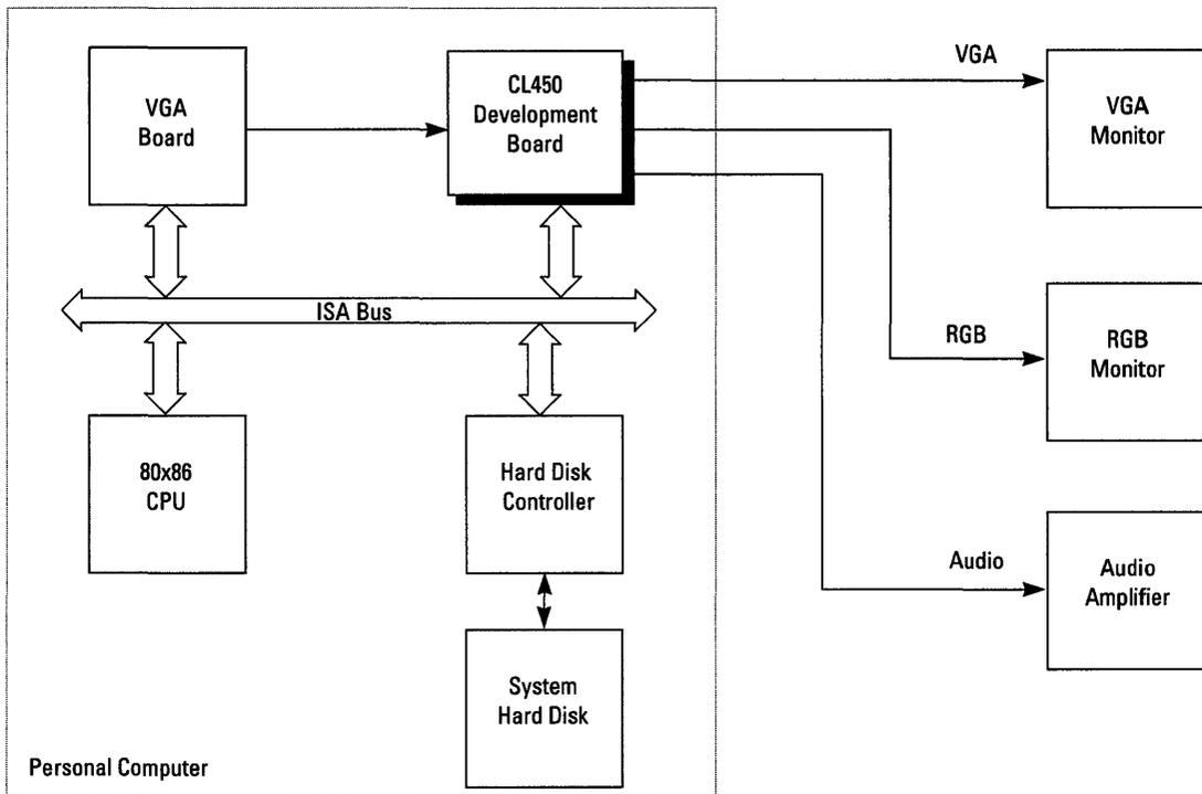
**Figure 9-1 Typical System Application**
