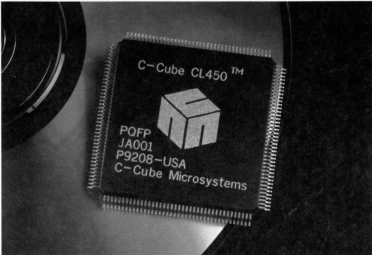
*The CL450 MPEG Video Decoder provides full-motion video capability for cost-sensitive electronics products.*
