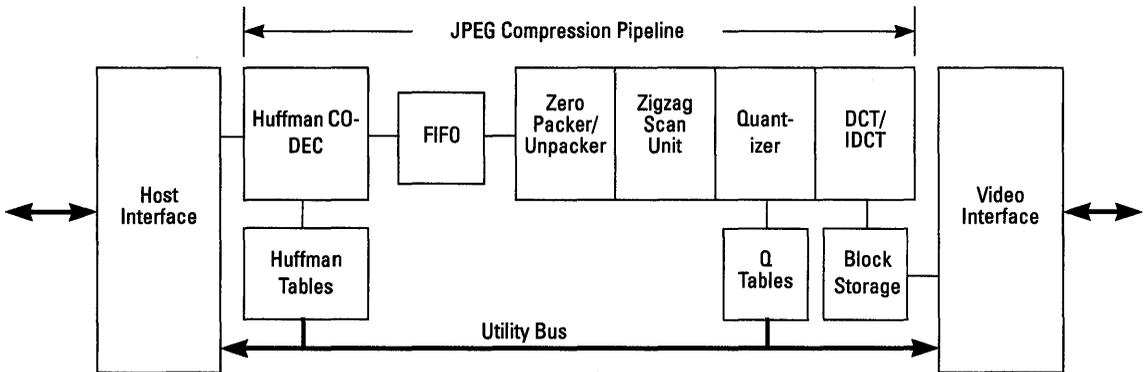
**Figure 3-1 CL550 Block Diagram**
