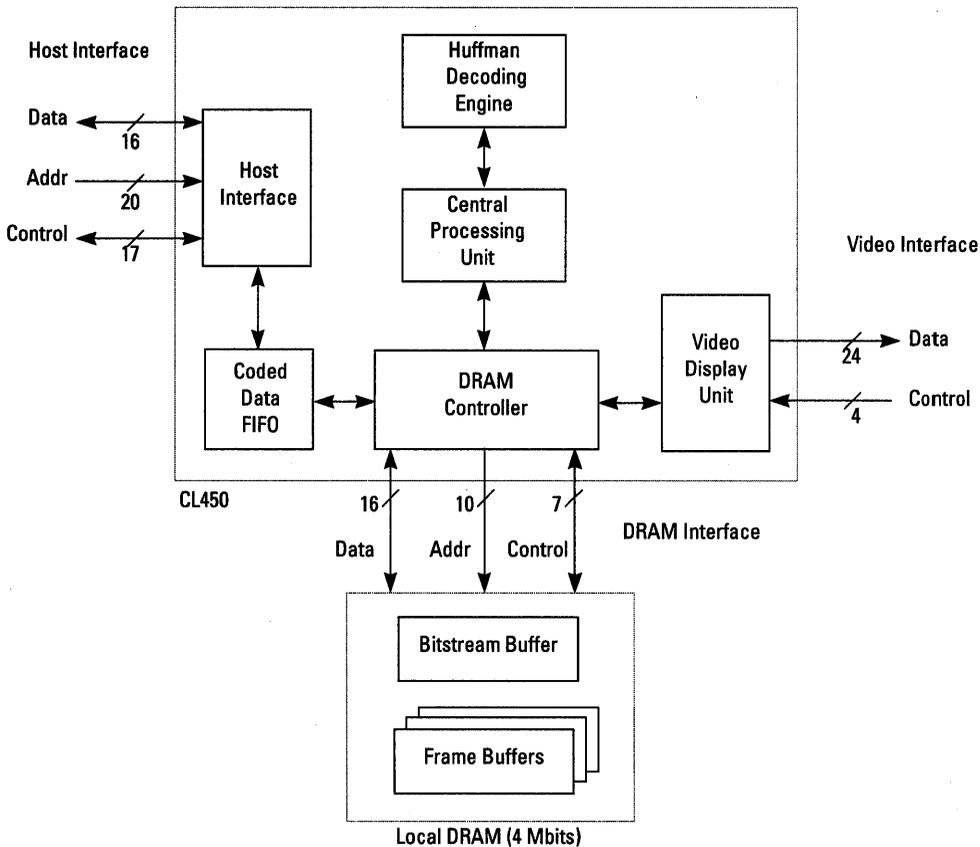
**Figure 8-1 Block Diagram of the CL450**
