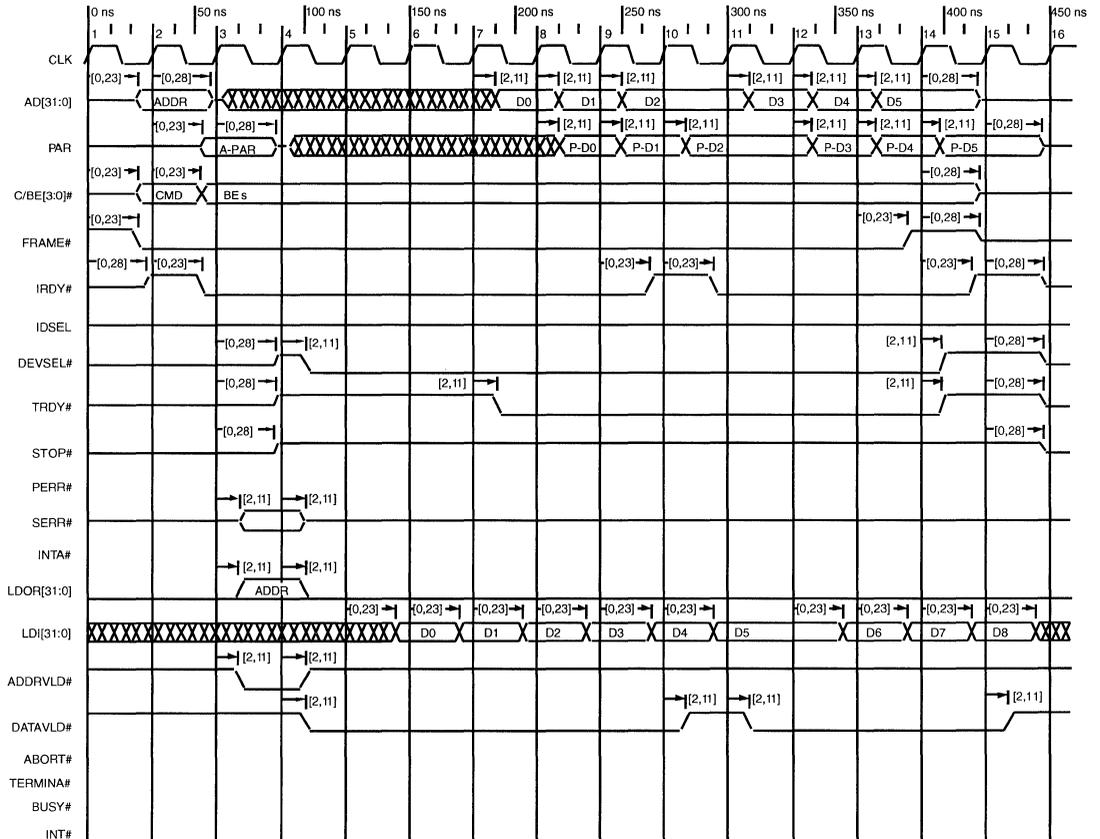
Figure 10. PCI Bus Single-Phase Read with Back-End Signals
