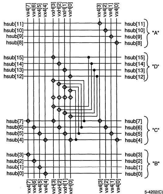
Figure 26. Horizontal Subquad Routing Connectivity (Half Quad)
