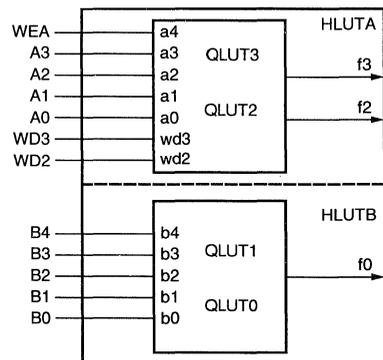
Figure 11. MA/F5 Mode—16 x 2 Memory and One Function of Five Input Variables
