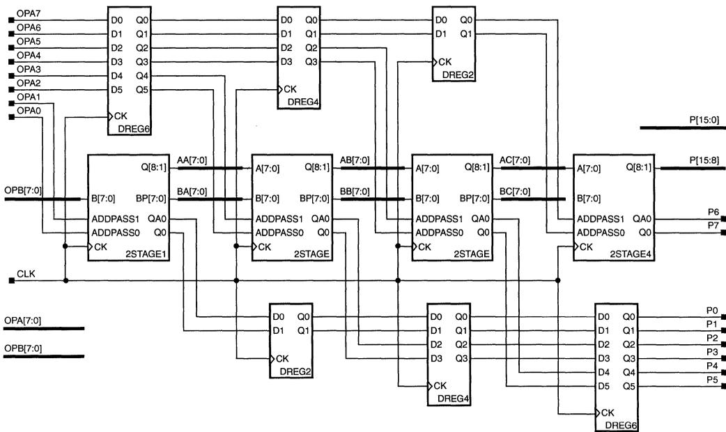
Figure 8. 8 x 8 Multiplier—Pipelined Every Two Stages
