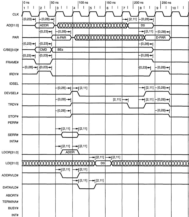
Figure 2. Basic PCI Bus Read Cycle
