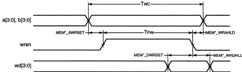
Figure 43. Write Operation
