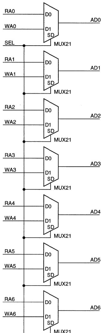
**Figure 3. Address Multiplexer**
