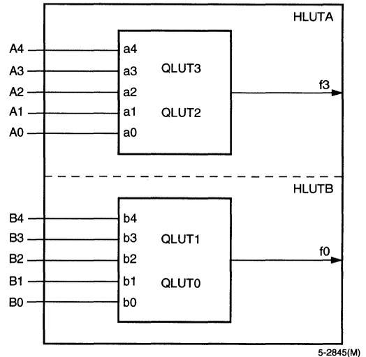
Figure 5. F5 Mode—Two Functions of Five Input Variables
