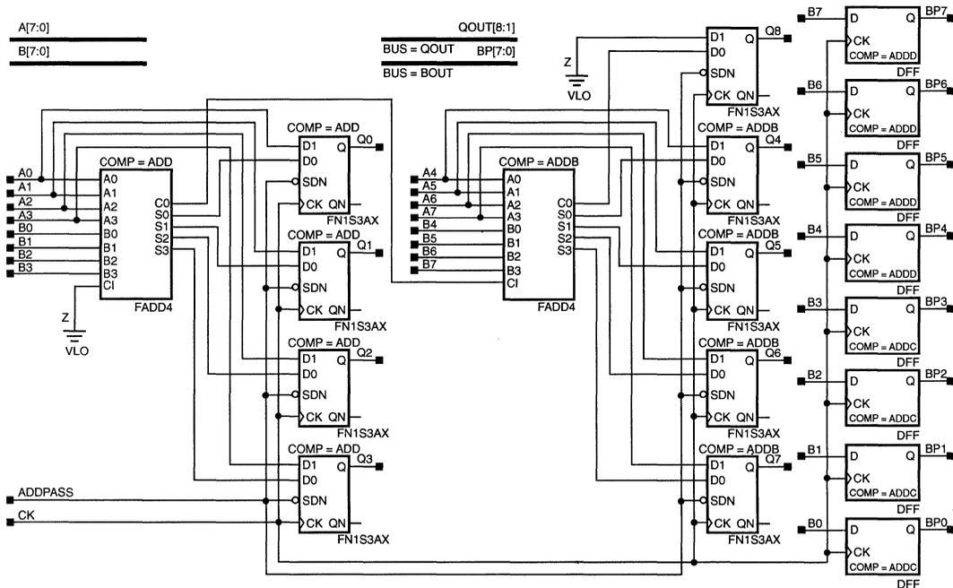
Figure 6. Stages 2—8 of the Pipelined Multiplier
