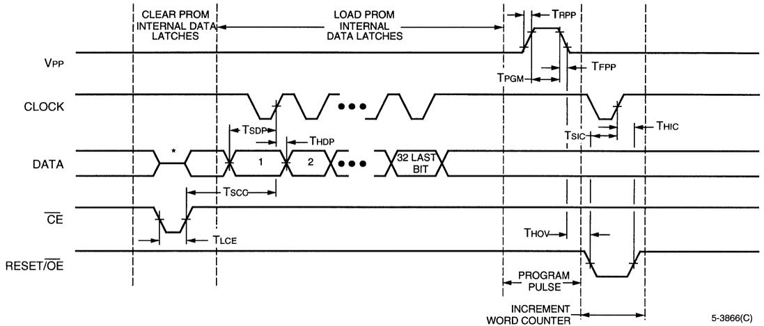
\* The programmer must float the data pin while CE is low to avoid bus contention.
