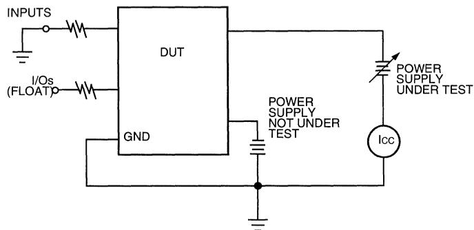
Figure 7. Test 3: Power Supply Overvoltage Test Equipment Hookup
