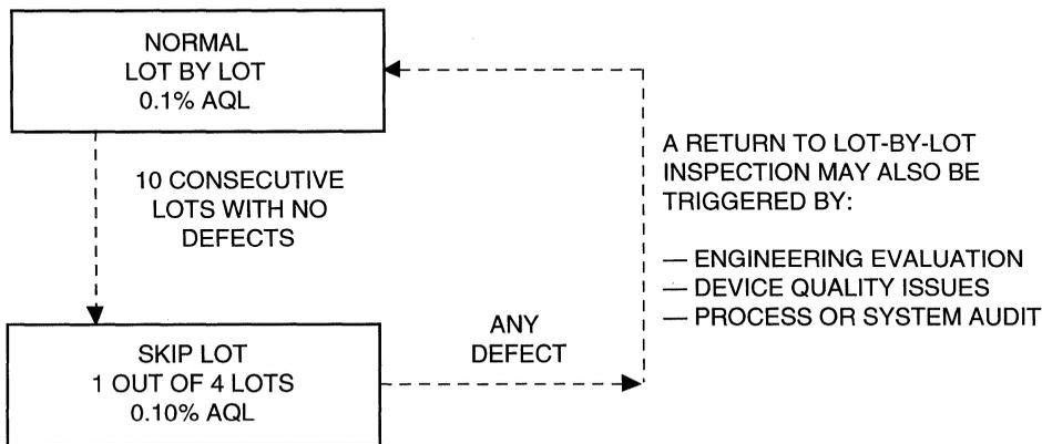
Figure 10. Electrical Test Sampling Level and Flow (Device Code Basis)
