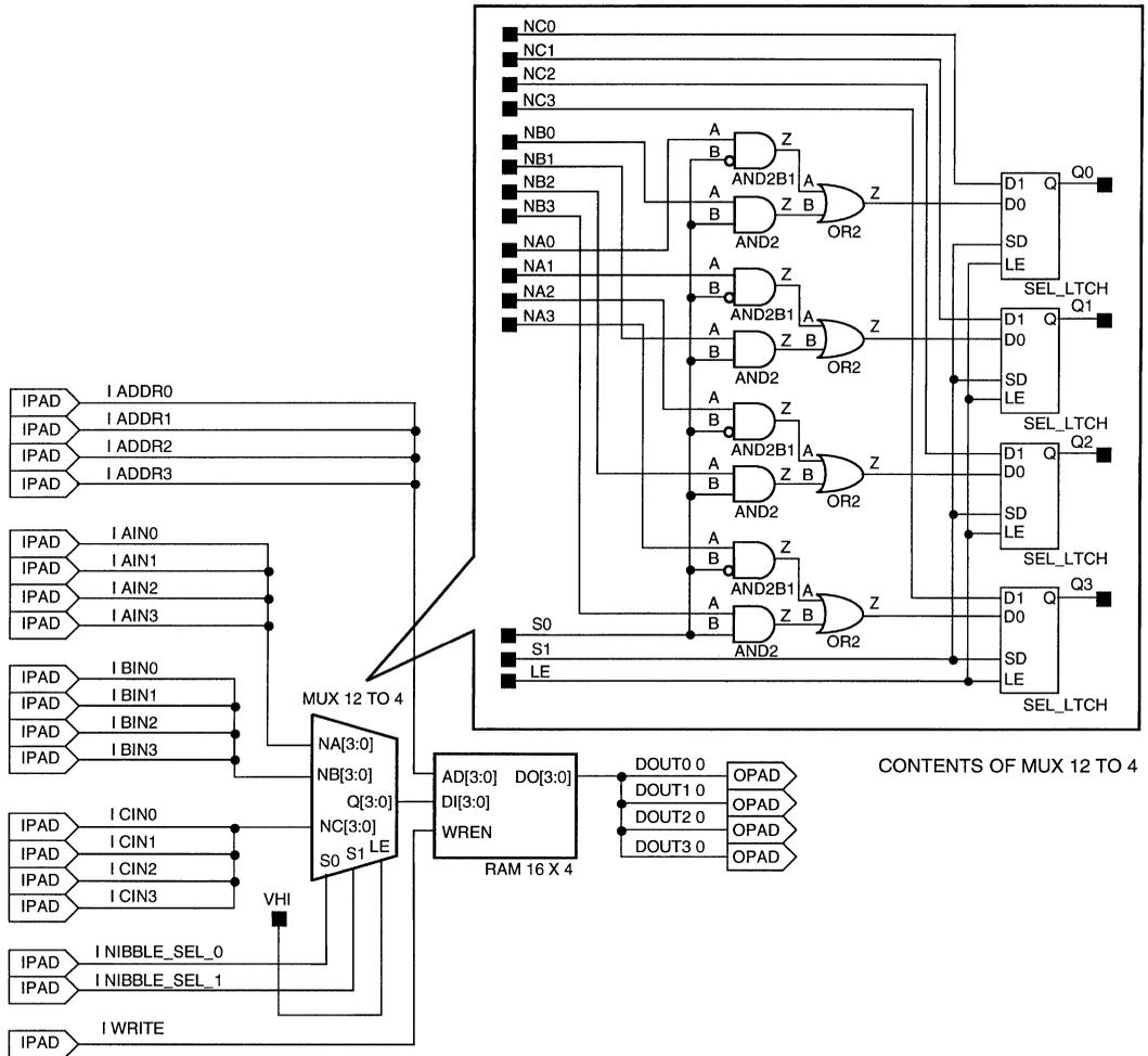
Figure 3. 16 x 4 SRAM Buffer with Triple-Multiplexed Inputs (2 PFUs)
