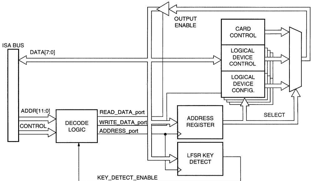
Figure 1. Logic Flow for *Plug and Play* Autoconfiguration
