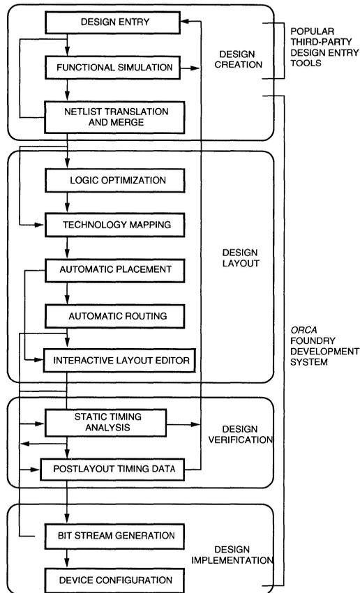
**Figure 2. ORCA Foundry Development System *Viewlogic* Design Flow**
