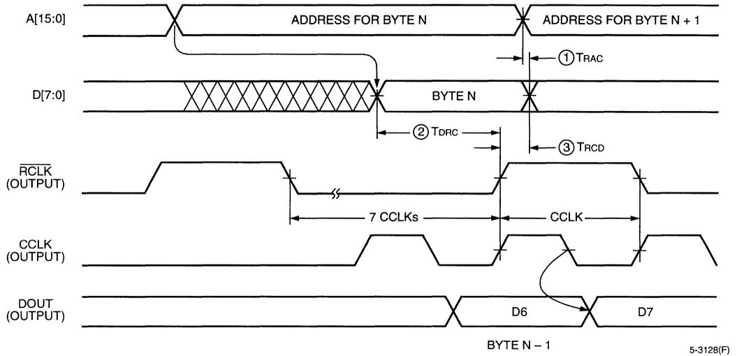
Note: The EPROM requirements in this timing diagram are extremely relaxed; EPROM access time can be longer than 4000 ns. EPROM data output has no hold time requirements.
