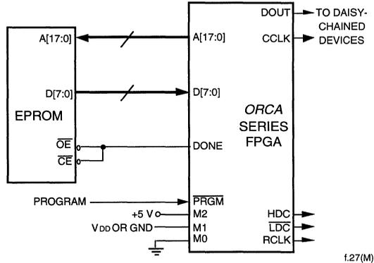
**Figure 28. Master Parallel Configuration Schematic**
