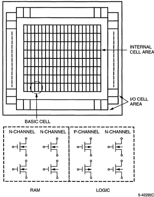
Figure 15. Chip Layout and Internal Cell Configuration
