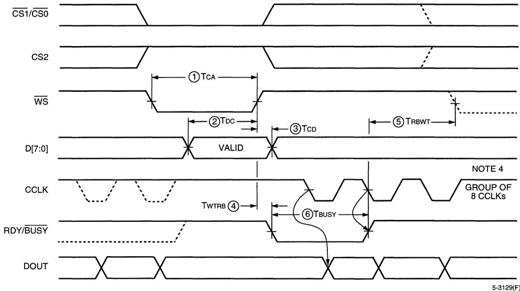
Note: The requirements in this timing diagram are extremely relaxed; data need not be held beyond the rising edge of WS. BUSY will go active within 60 ns after the end of WS. BUSY will stay active for several microseconds. WS may be asserted immediately after the end of BUSY.
