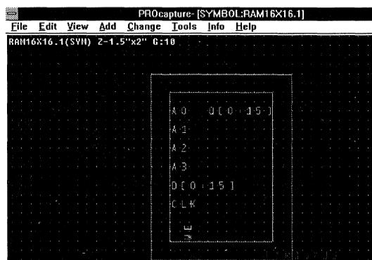
Note the bubble on the *clk* pin. This was caused by the use of the tilde (~). The bubble has no effect on the connectivity; it is only an annotation graphic. The *q[0:15]* and *q[0:15]* pins are wider than other pins since the names were escaped with \\. The pin order will be:
