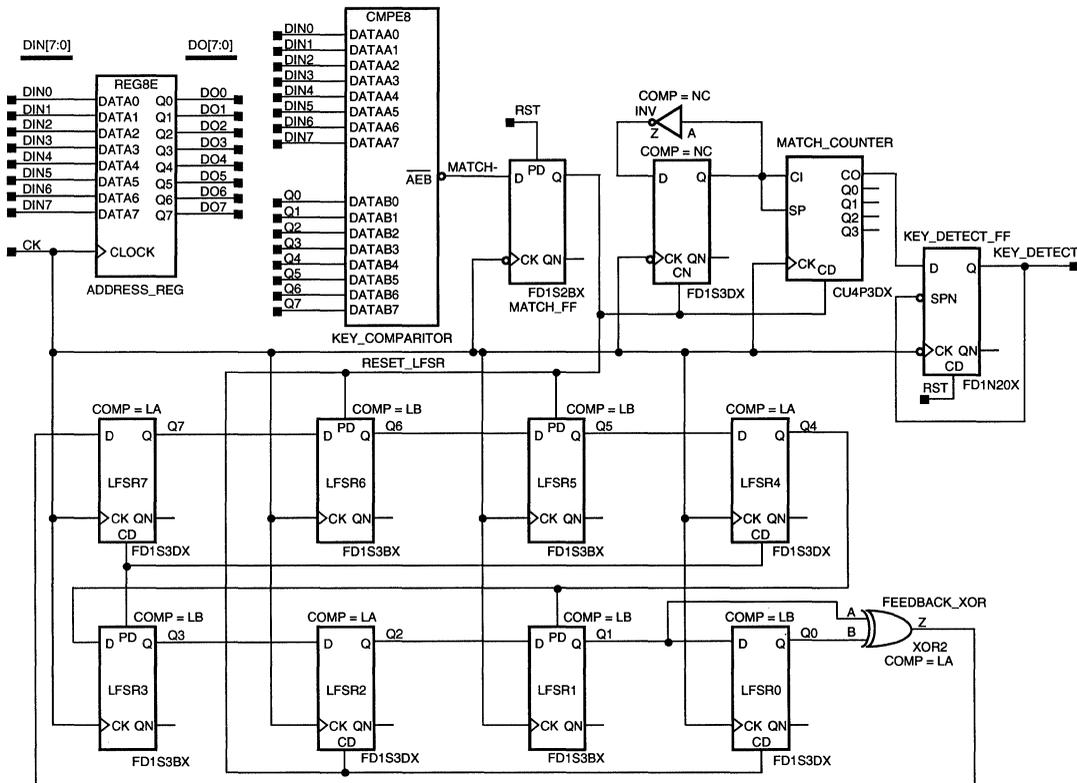
Figure 2. LFSR Initialization Key Circuitry from AT&T's *ORCA Plug and Play* Design Kit Reference Design—Illustrates the Need for Flexible On-Chip Registers/Latches
