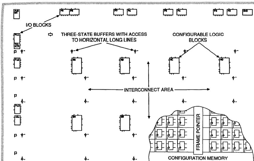
Figure 1. Field-Programmable Gate Array Structure
