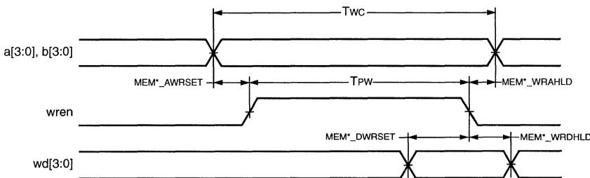
Figure 51. Write Operation
