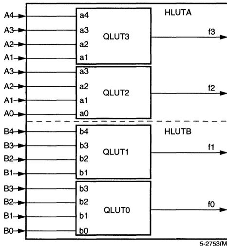
Figure 4. F4 Mode—Four Functions of Four Input Variables
