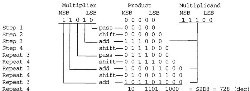
Note: For any binary multiplication, the number of bits needed for the product will be the total of the bits found in both operands. In this case, with two 5-bit operands, the product can be up to 10 bits long. In the 8 x 8 multiplier examples to follow, the product can be as long as 16 bits.
