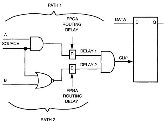
\*  $CLK = (A * SOURCE) * (\sim (B + SOURCE))$ . If A = 1 and B = 0, CLK can be affected by both Path 1 and Path 2.
