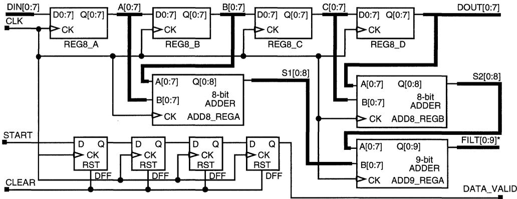
\* Only the MSBs (bits 2—9) are used. The divide-by-4 function is performed in this manner.
