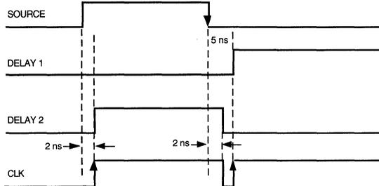
Figure 8. SOURCE Clock with Glitch—Gate Array Design
