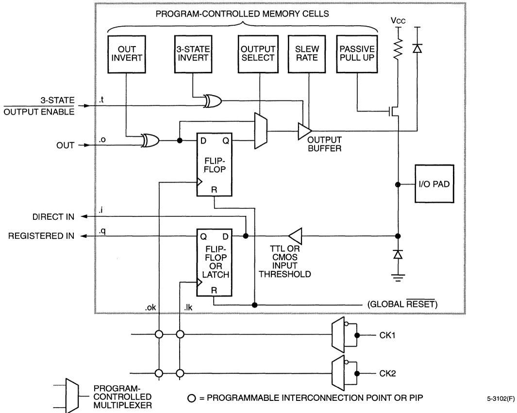
Figure 3. Input/Output Block (IOB)
