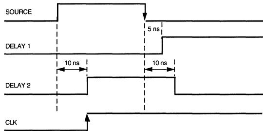
Figure 7. SOURCE Clock Without Glitch—FPGA Design
