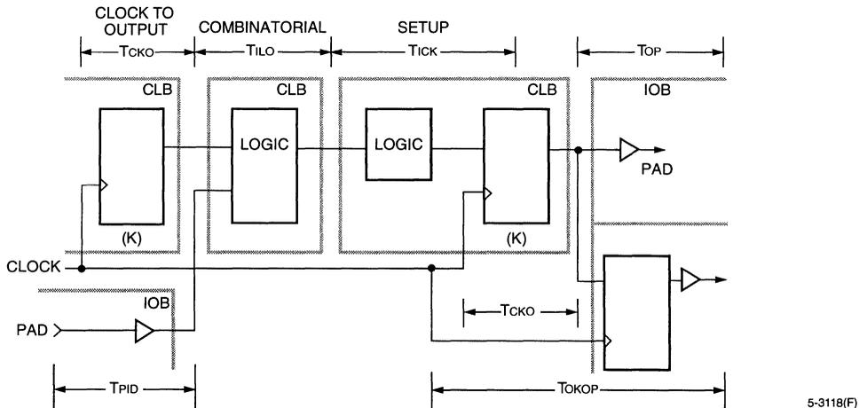
Figure 27. Examples of Primary Block Speed Factors
