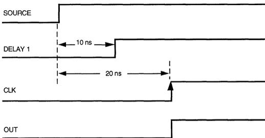
Figure 13. Mixed Data and Clock FPGA Design
