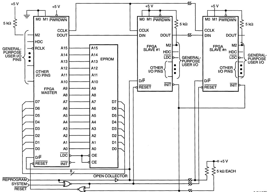
Figure 25. Master Mode with Daisy-Chained Slave Mode Devices
