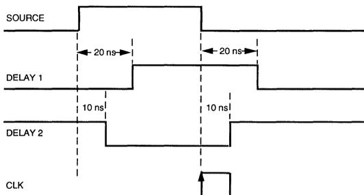
Note: DELAY 1 = 20 ns and DELAY 2 = 10 ns; therefore, there will be a 10 ns clock pulse on the falling edge of SOURCE.
