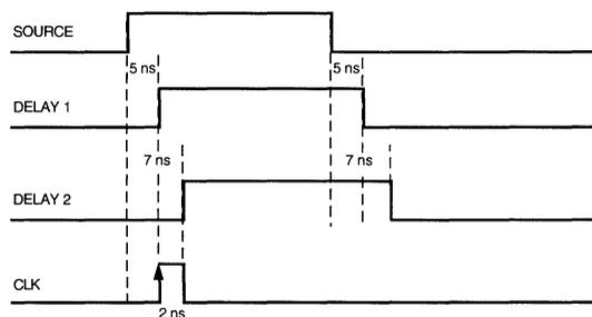
Note: DELAY 1 = 5 ns, DELAY 2 = 7 ns. The gate array now has an unwanted glitch on the rising edge of SOURCE, while the pulse from the falling edge of SOURCE is gone.
