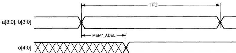
Figure 49. Read Operation—Flip-Flop Bypass
