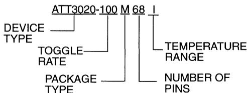
Example: ATT3020, 270 MHz, 68-Lead PLCC, Commercial Temperature
