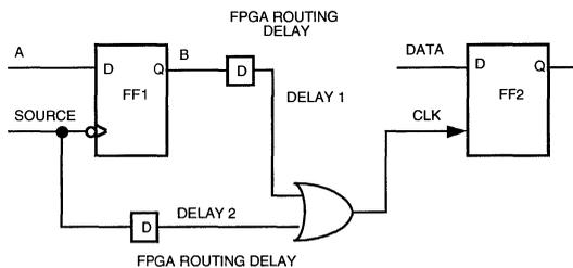
Figure 6. Clock with Reconvergent Sources
