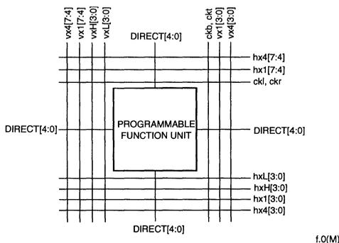
**Figure 15. Single PLC View of Inter-PLC R-Nodes**
