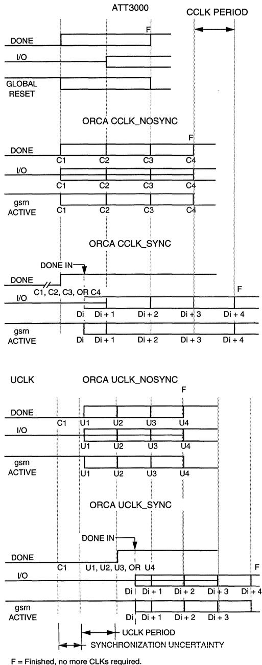
Figure 25. Start-Up Waveform
