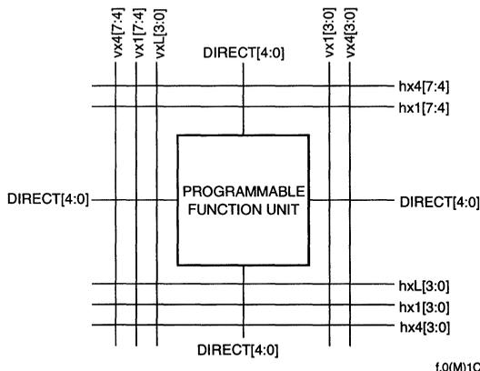
**Figure 15. Single PLC View of Inter-PLC R-Nodes**
