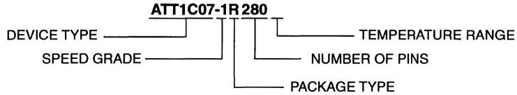
ATT1C07, -1 Speed Grade, 280-pin Ceramic PGA, Commercial Temperature
