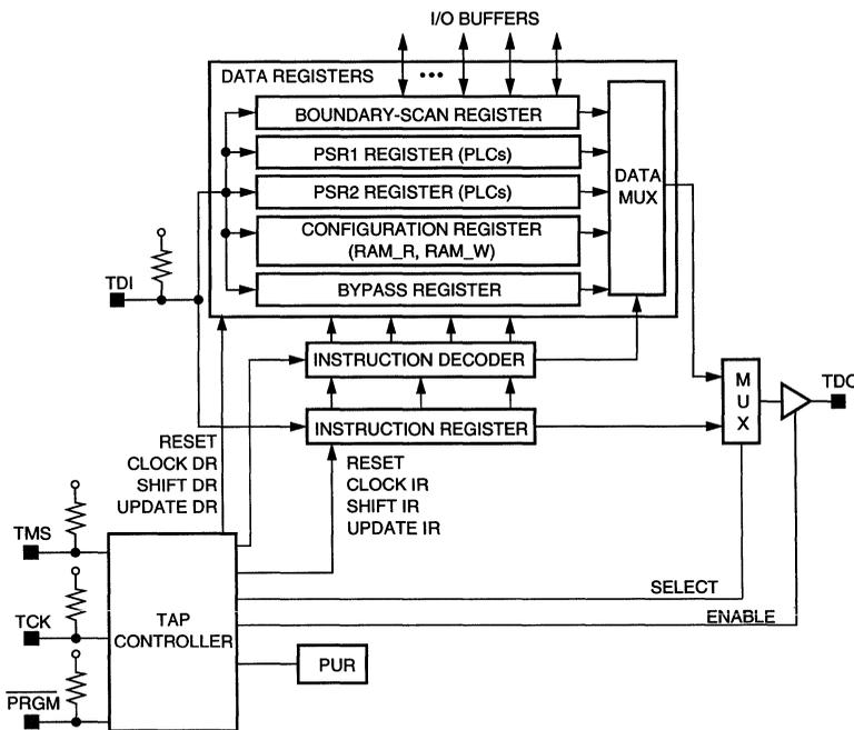
**Figure 37. ORCA Series Boundary-Scan Circuitry Functional Diagram**
