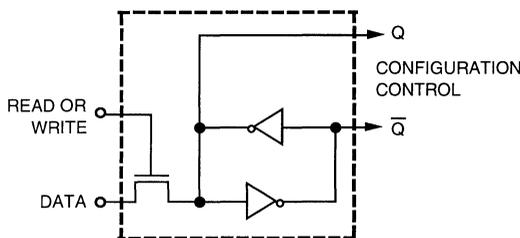
Figure 1. Configuration Memory Cell
