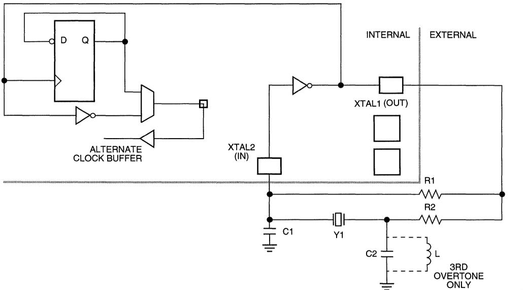
**Figure 7. Crystal Oscillator Inverter**
