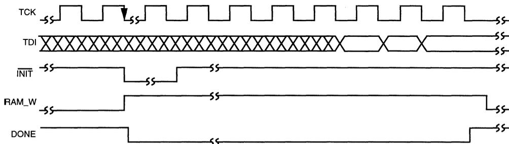
Figure 7. ram\_w Timing Diagram After Configuration
