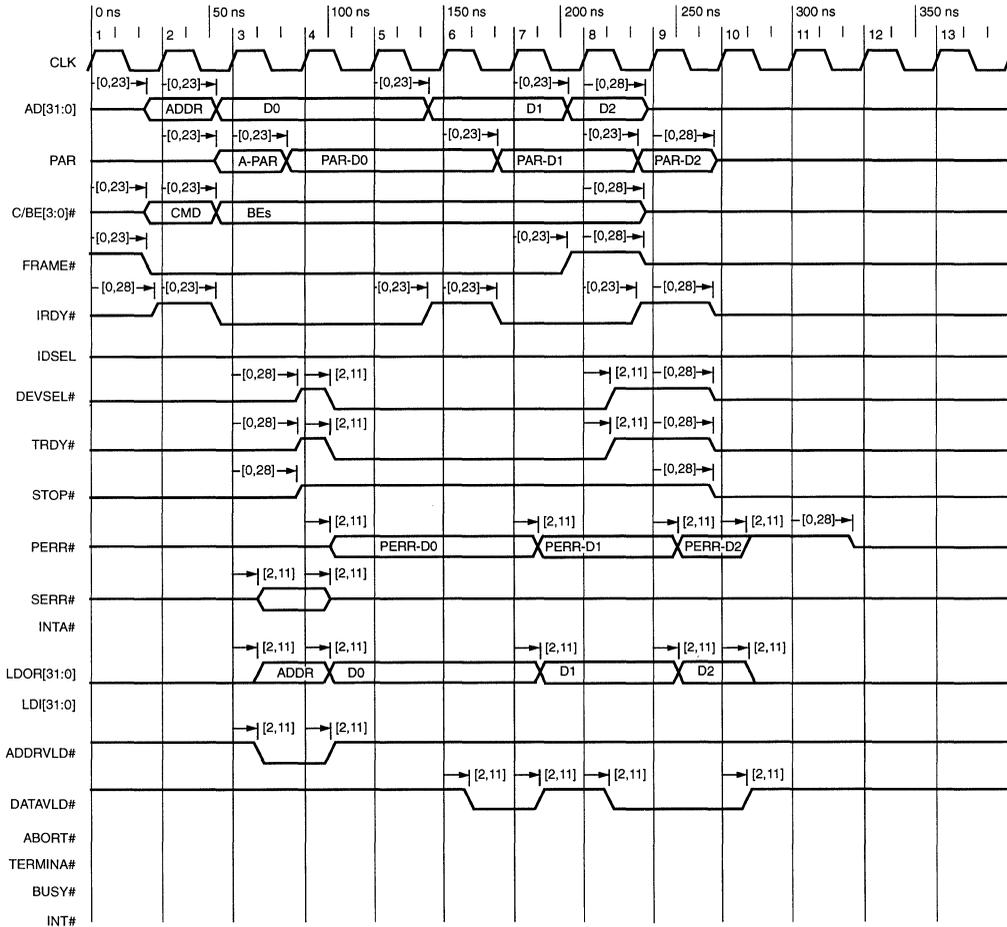
Figure 11. PCI Bus Multiphase Write with Back-End Signals
