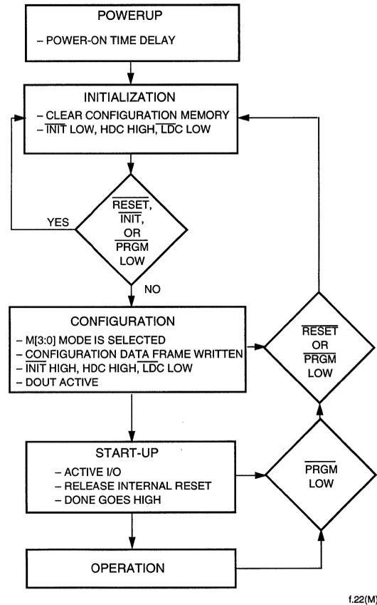
Figure 23. FPGA States of Operation
