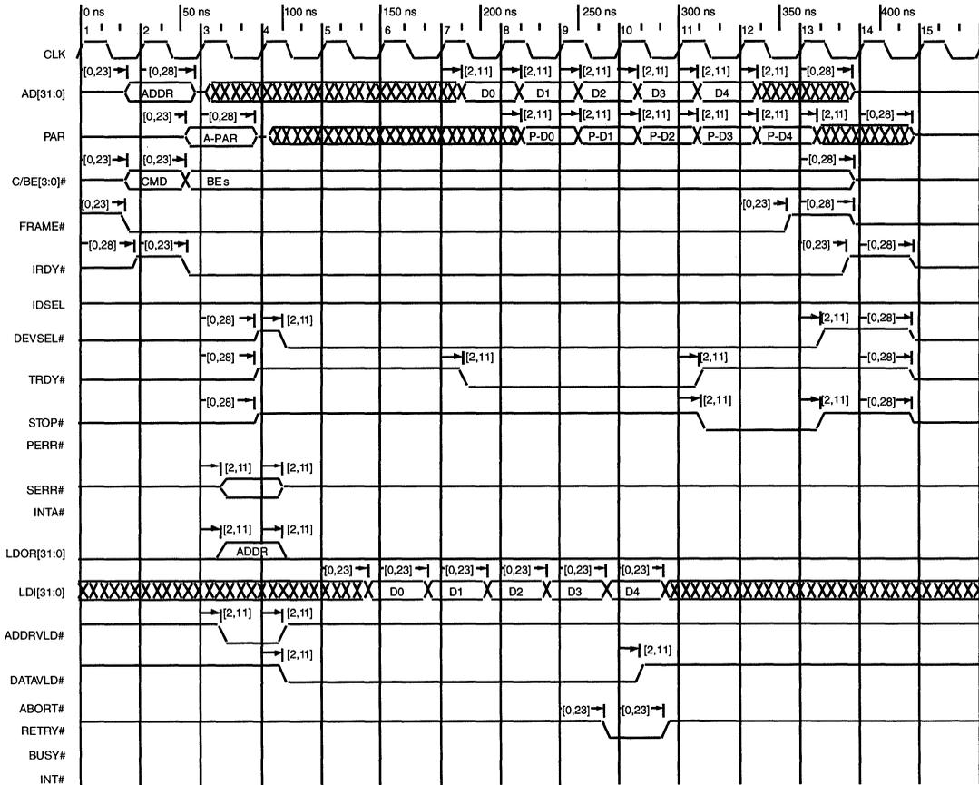
Figure 14. Read Cycle with Retry
