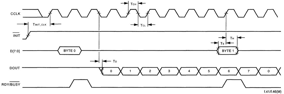
Figure 58. Synchronous Peripheral Configuration Mode Timing Diagram
