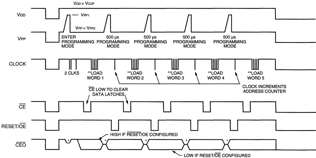
\* The  $\overline{CEO}$  pin is high impedance when  $VPP = VPP1$ .
