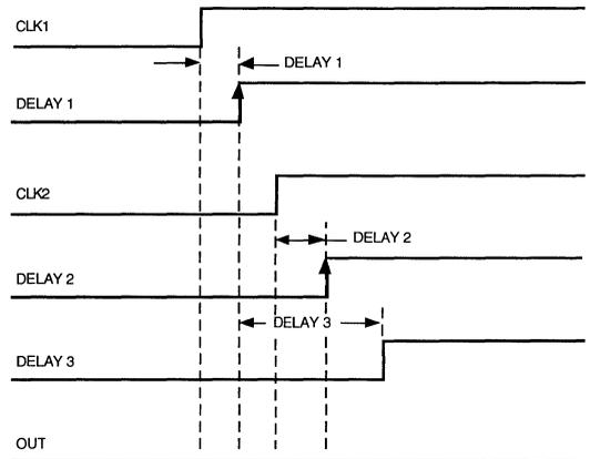
Figure 11. Clock/Data Race Gate-Array Design
