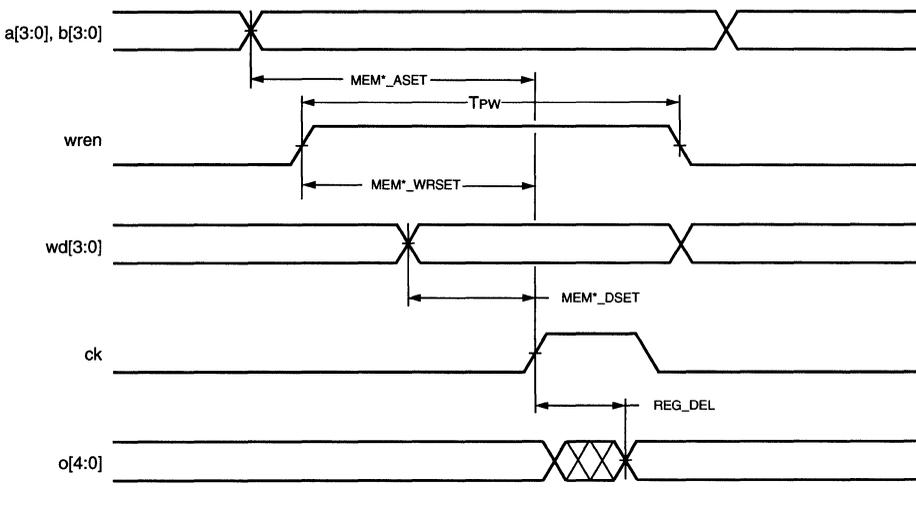
Figure 45. Read During Write—Clocking Data into Flip-Flop
