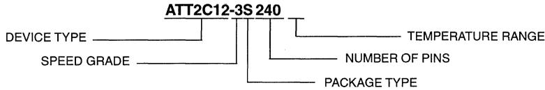
ATT2C12, -3 Speed Grade, 240-pin Shrink Quad Flat Pack, Commercial Temperature.
