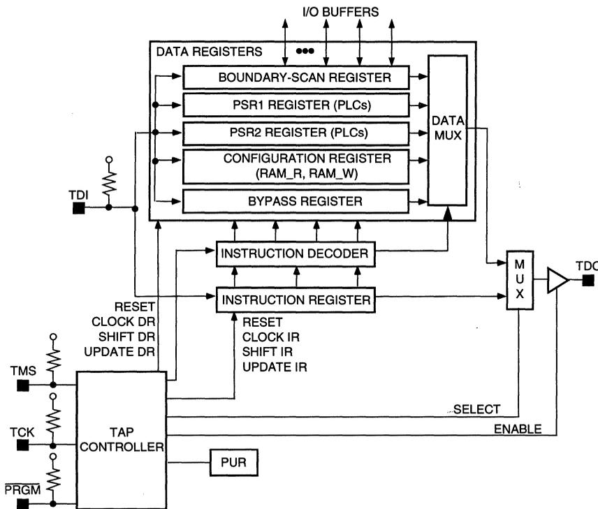
Figure 1. Diagram of Boundary-Scan Function
