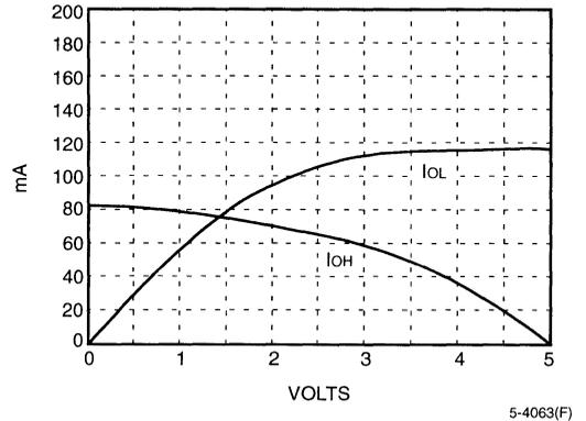
Figure 4. Output Current/Voltage Characteristics for -70, -100, -125, -150 Speed Grades
