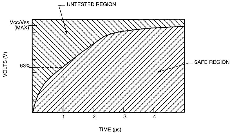
Figure 6. Test 2: Power Supply ( $\Delta V/\Delta t$ ) Limit
