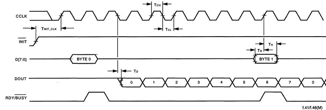
Figure 50. Synchronous Peripheral Configuration Mode Timing Diagram
