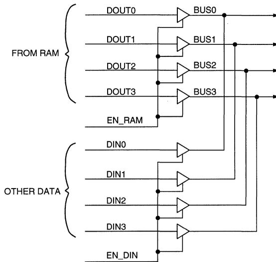
Figure 4. Multiplexing of RAM Outputs Using Tristate Buffers
