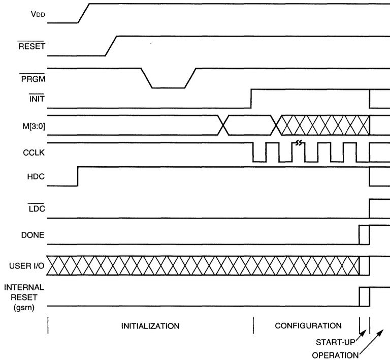
**Figure 24. Initialization/Configuration/Start-Up Waveform**
