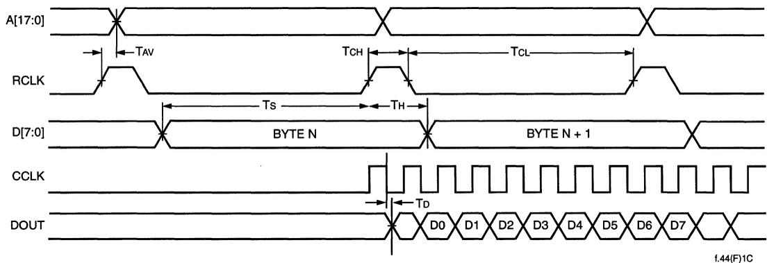
**Figure 48. Master Parallel Configuration Mode Timing Diagram**
