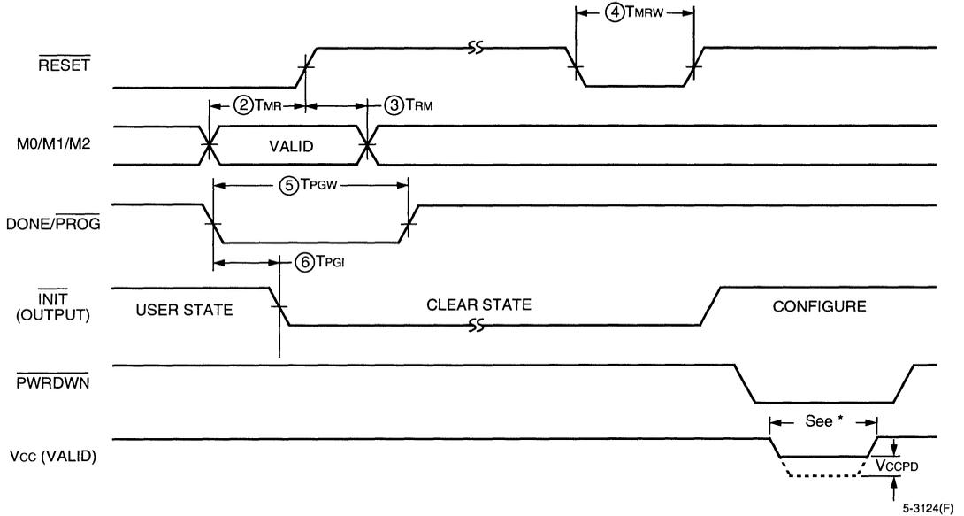
\* At powerup, VCC must rise from 2 V to VCC minimum in less than 25 ms. If this is not possible, configuration can be delayed by holding  $\overline{\text{RESET}}$  low until VCC has reached 4 V. A very long VCC rise time of >100 ms or a nonmonotonically rising VCC may require a >1  $\mu\text{s}$  high level on  $\overline{\text{RESET}}$ , followed by a >6  $\mu\text{s}$  low level on  $\overline{\text{RESET}}$  and  $\overline{\text{DONE/PROG}}$  after VCC has reached 4 V.
