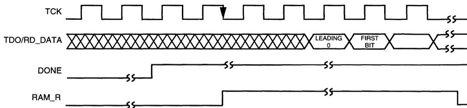
Figure 8. ram\_r Timing Diagram After Configuration
