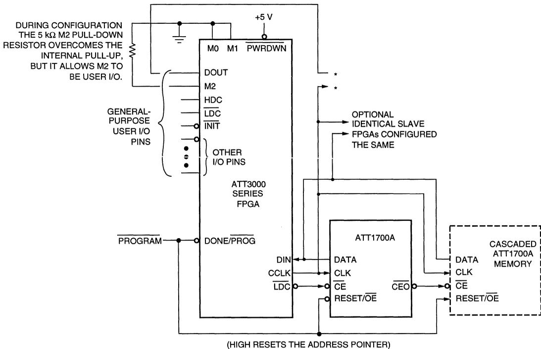
Note: The serial configuration PROM supports automatic loading of configuration programs up to 36/64/128 Kbits. Multiple devices can be cascaded to support additional FPGAs. An early DONE inhibits the data output one CCLK cycle before the FPGA I/O becomes active.
