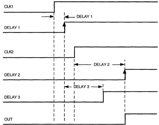
Figure 10. Clock/Data Race FPGA Design
