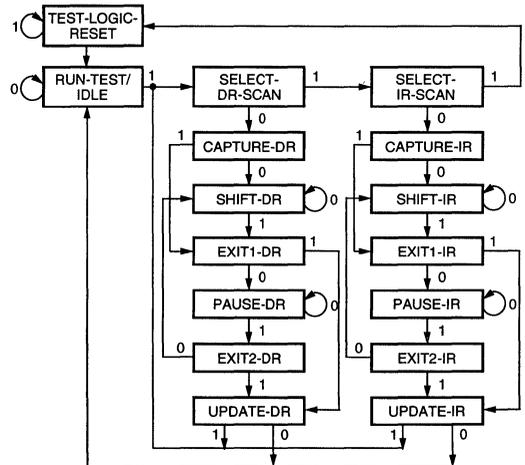
**Figure 2. TAP Controller State Diagram**
