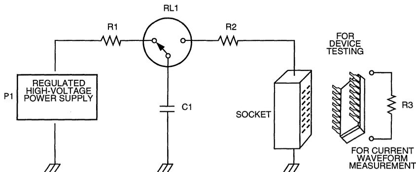
Figure 3. Circuit Schematic of Human-Body ESD Simulator
