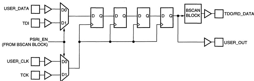
Figure 5. Example of Boundary-Scan User-Defined Scan Path Logic
