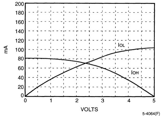
Figure 5. Output Current/Voltage Characteristics for -3, -4, -5 Speed Grades
