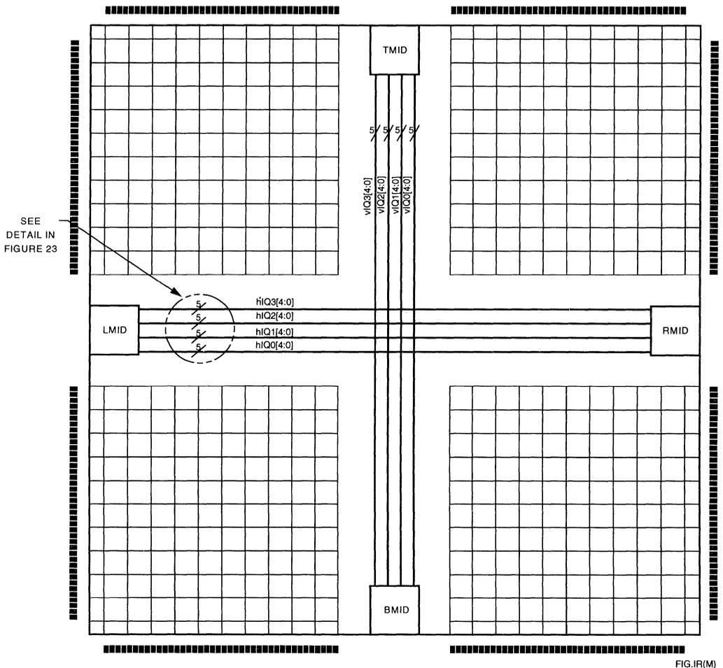
Figure 22. Interquad Routing
