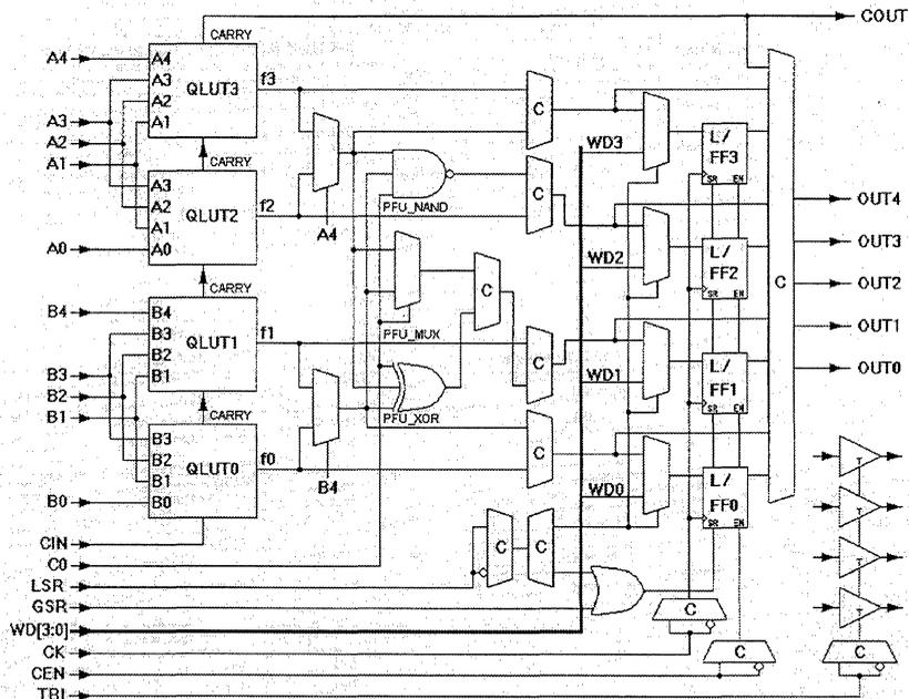
Figure 1. Four Multiplexing Elements in a Single *ORCA* PFU
