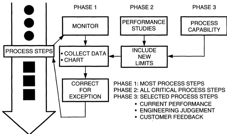
Figure 9. The SPC Process Flow
