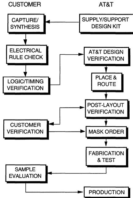
Figure 16. Gate-Array Design Flow
