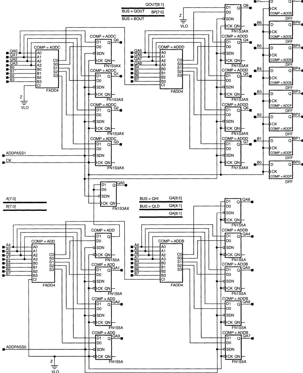
Figure 9. Stages 2—3 of the Partially Pipelined 8 x 8 Multiplier
