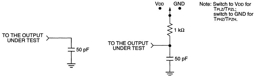
A. Load Used to Measure Propagation Delay B. Load Used to Measure Rising/Falling Edges
