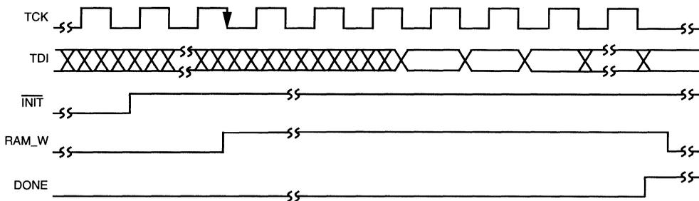
Figure 6. ram\_w Timing Diagram Before Configuration
