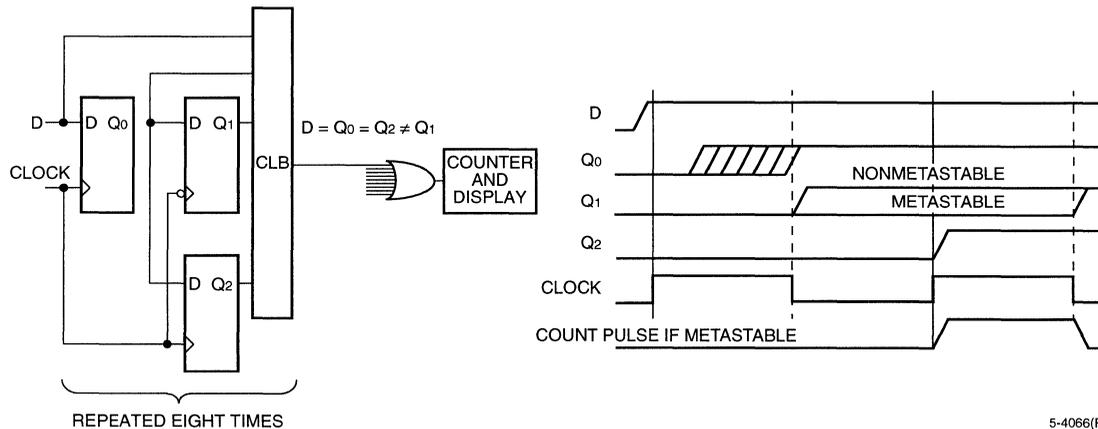
**Figure 8. Metastable Measuring Circuit**
