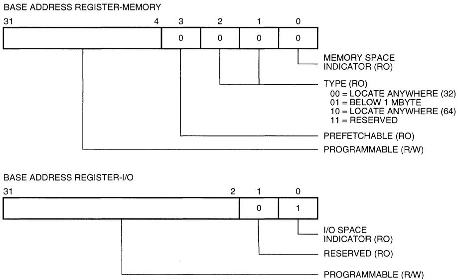
Figure 7. Base Address Registers
