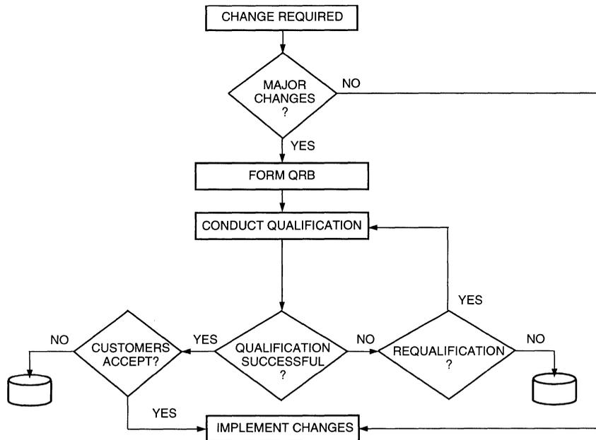
Figure 2. Requalification Process Flow
