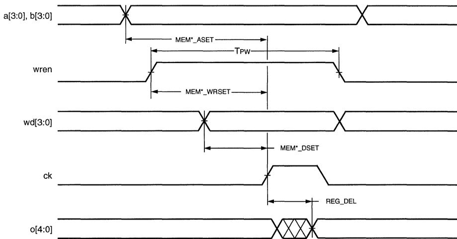
Figure 53. Read During Write—Clocking Data into Flip-Flop
