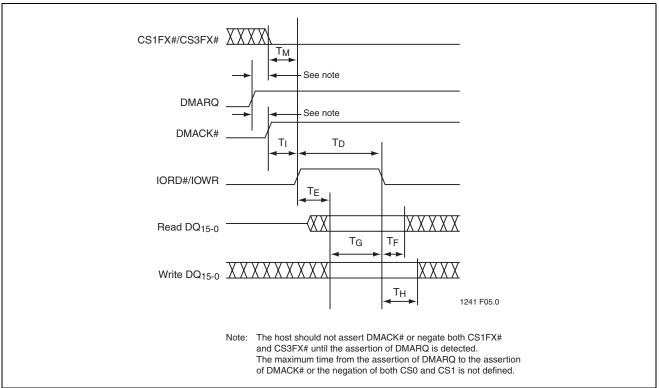
FIGURE 12-4: Initiating a Multi-word DMA Data Transfer
