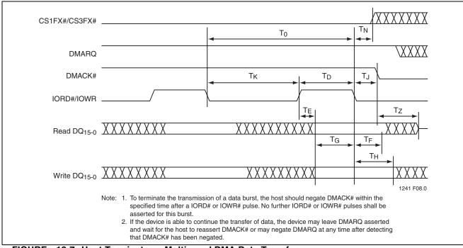
FIGURE 12-7: Host Terminates a Multi-word DMA Data Transfer
