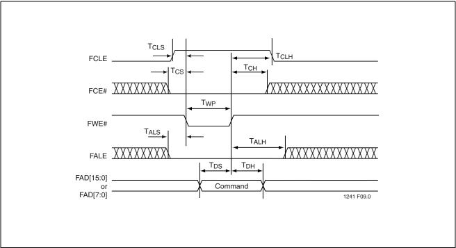
FIGURE 12-8: Media Command Latch Cycle
