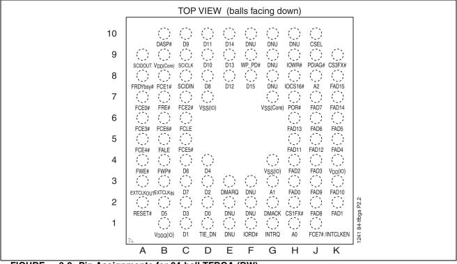
FIGURE 3-2: Pin Assignments for 84-ball TFBGA (BW)
