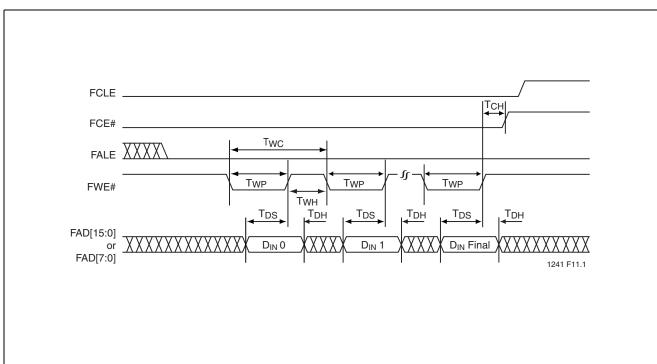
FIGURE 12-10: Media Data Loading Latch Cycle
