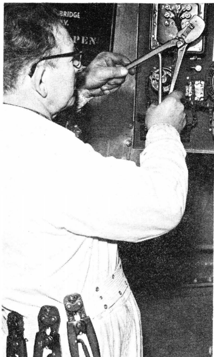
A wide variety of AMP Certi-Crimp hand tools affords convenience of use and uniform control of crimping in the smaller wire sizes.
