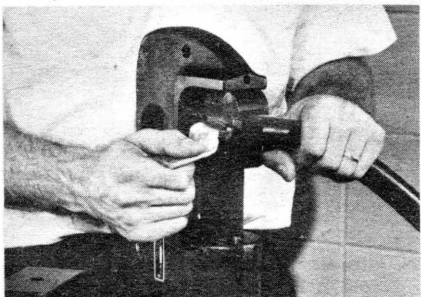
AMPOWER Terminals make possible connections of high tensile strength for wires as large as 1000 MCM.
