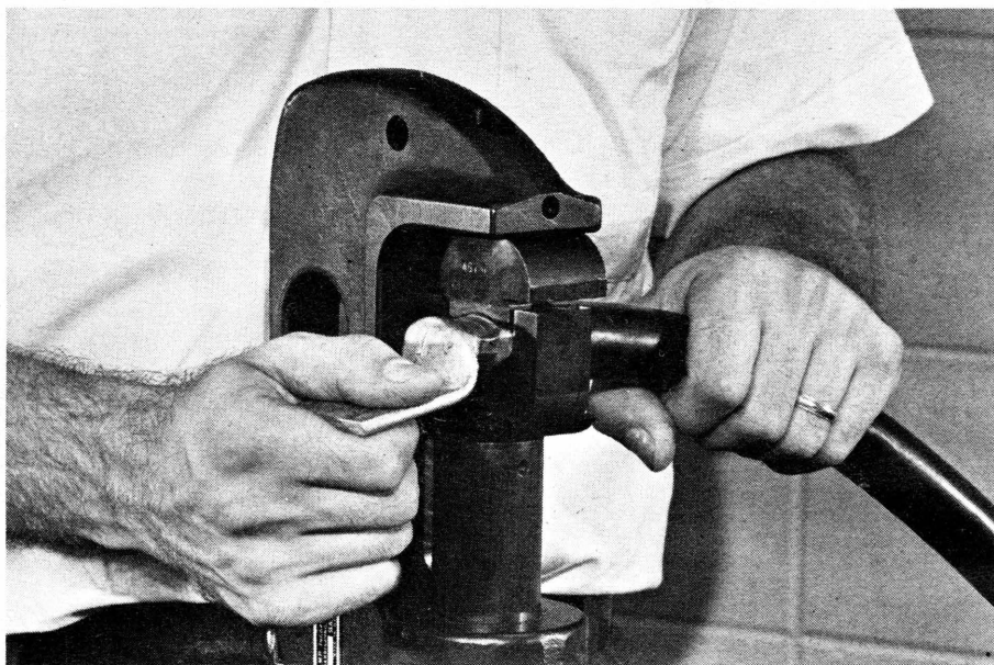
AMPOWER Terminals make possible connections of high tensile strength for wires as large as 1000 MCM in width
