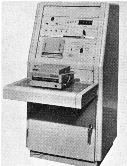
Master Terminal Data Transmission System of Municipal fire alarm box identification features A-MP Card Reader for use in automatic mode of operation
