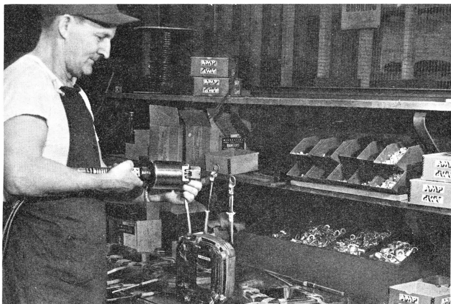
Large wires up to 1000 MCM can be securely crimped in the hydraulically powered A-AMP DYNA-CRIMP tools.
