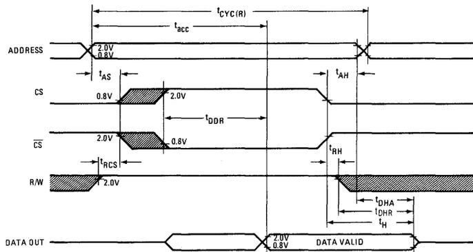
NOTE: CS AND CS-bar CAN BE ENABLED FOR CONSECUTIVE READ CYCLES PROVIDED R/W REMAINS AT  $V_{IH}$
