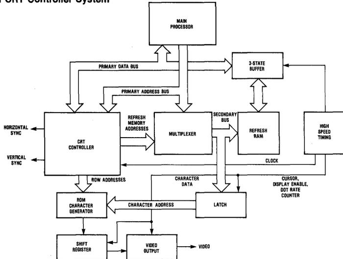
The character address of the cursor is held in a register, so the cursor's position is not lost even when scrolled off the screen.
