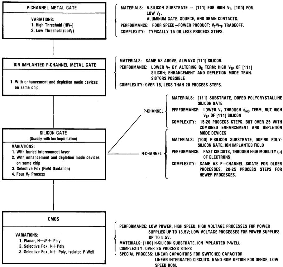
The basic P-Channel metal gate process can be subdivided into two general categories: **High-threshold and low-threshold**. Various manufacturers use different techniques (particularly so with the low threshold process) to achieve similar results, but the difference between them always rests in the threshold voltage  $V_T$  required to turn a transistor on. The high threshold  $V_T$  is typically  $-3$  to  $-5$  volts and the low threshold  $V_T$  is typically  $-1.5$  to  $-2.5$  volts.
