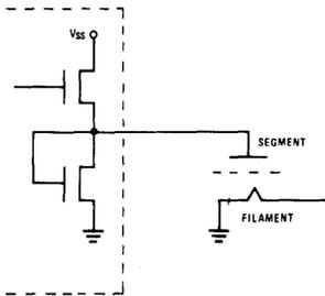
Figure 5. Liquid Crystal Drive
