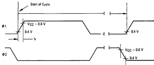
Measurement point for  $\phi 1$  and  $\phi 2$  are shown above. Other measurements are the same as for MC6800.
