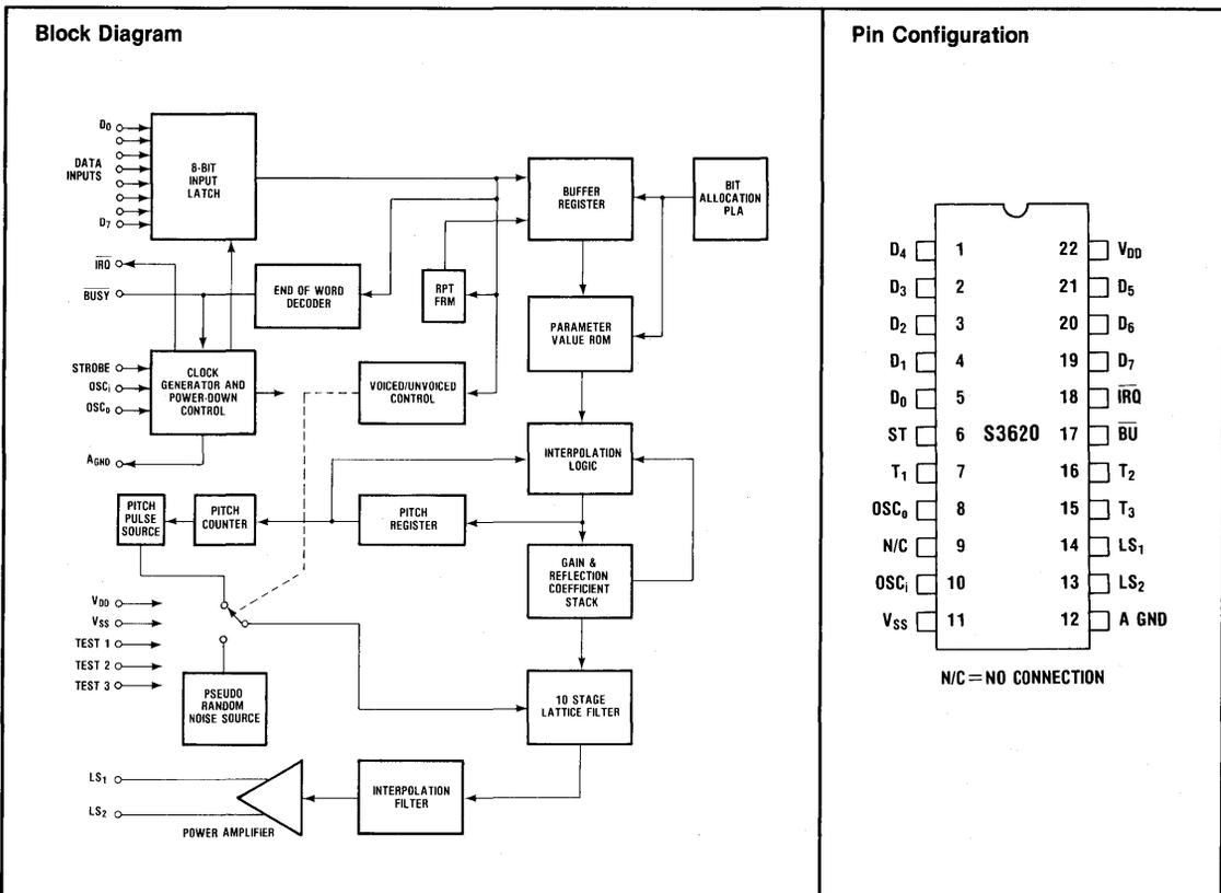
rate is 2.0K bits/sec. max., but typically the average data rate will be reduced to about 1.4K bits/sec. by means of the data rate reduction techniques used internally.
