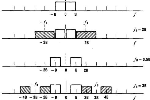
Note that critical sampling avoids aliasing, but in the above example no real life filter can separate the message from the image. One must oversample in real life.
