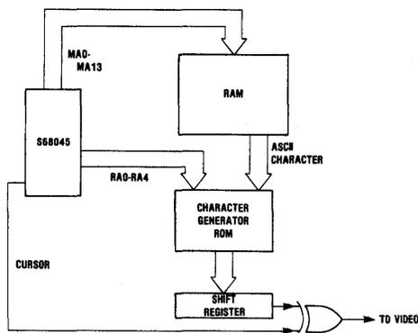
way cursor position is not lost when the display is scrolled.
