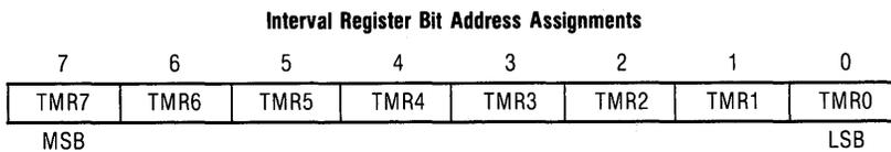
The figure below illustrates the establishment of the interval for the Interval Timer. As an example, if the Interval Register is loaded with a value of  $80_{16}$  ( $128_{10}$ ) the interval at which Timer Interrupts are generated is  $t_{TVL} = t_{int} \cdot 64 \cdot M = (1\mu\text{s}) \cdot (64) \cdot (128) = 8.192 \text{ ms}$ . when  $t_{int} = 1\mu\text{s}$ .
