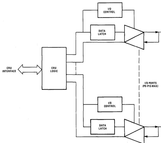
through 15 would normally be the interrupt input lines in this mode, but if any are not needed for interrupts, they may also be read with a CRU input command and interpreted as normal data inputs. A "1" read on the control bit indicates that the 9901 is in the clock mode. Reading bits 1 through 14 completes the event timer
