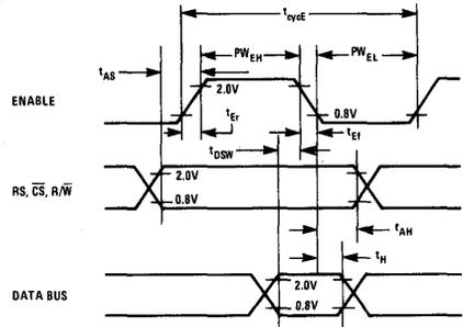
**Figure 3. Input Pulse Width Low**
