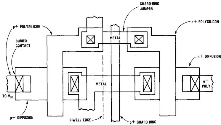
THE FIRST HIGH-PERFORMANCE COMPLEMENTARY-MOS PLANAR PROCESS. ITS DRAWBACKS: TWO TYPES OF POLYSILICON ARE USED, AND THE UNAVAILABILITY OF FIELD IMPLANT DOPING TIES FIELD THRESHOLD TO DEVICE THRESHOLDS.
