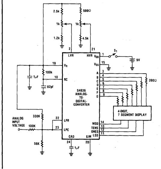
Figure 2. Typical Digital Scale Application
