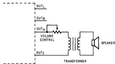
Figure 2-A. Typical Telephone Application of the S2561
