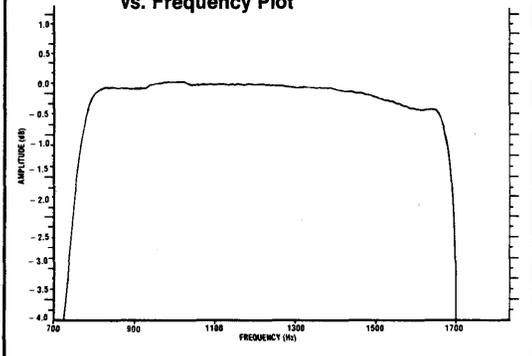
**Figure 4. Typical High-Band Amplitude vs. Frequency Plot**
