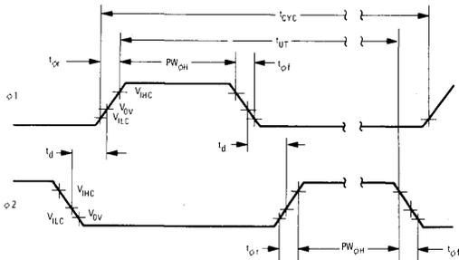
Figure 2. Read/Write Timing Waveform
