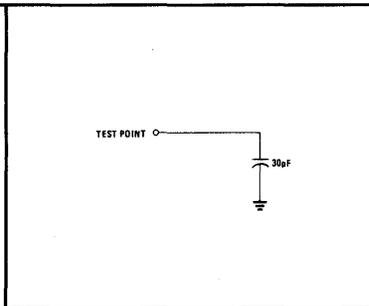
**Figure 3. TTL Equiv. Test Load (Ports A and C)**
