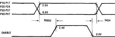
Figure 4. Peripheral CMOS Data Delay Times (Write Mode)
