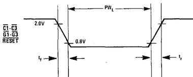
**Figure 4. Input Pulse Width High**
