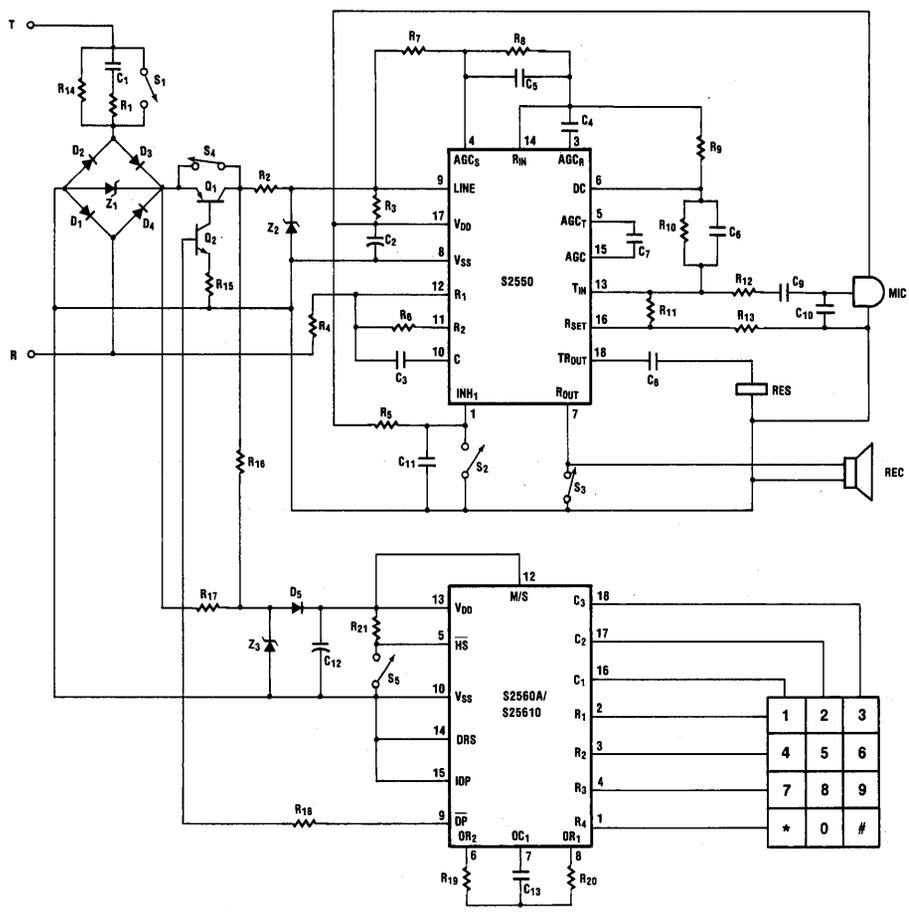
Figure 5. A Typical Application Circuit for an Electronic Telephone With DTMF
