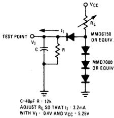
Figure 6. CMOS Equiv. Test Load
