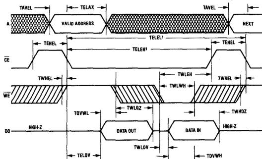
NOTE 1: TELEL & TELEH ARE LONGER THAN THE MINIMUM GIVEN FOR READ OR WRITE CYCLE.
