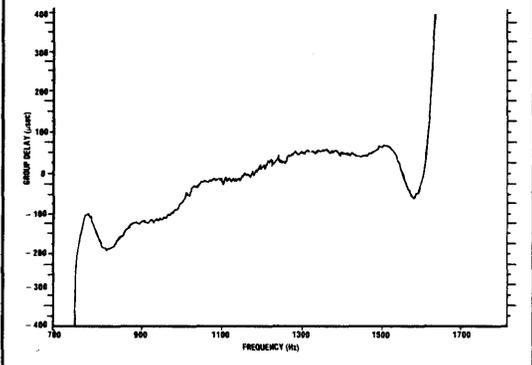
**Figure 5. Typical High-Band Group Delay vs. Frequency Plot**
