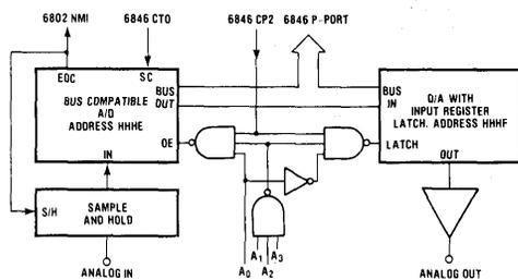
**Figure 14. Interfacing the S28214A with a Microprocessor**
