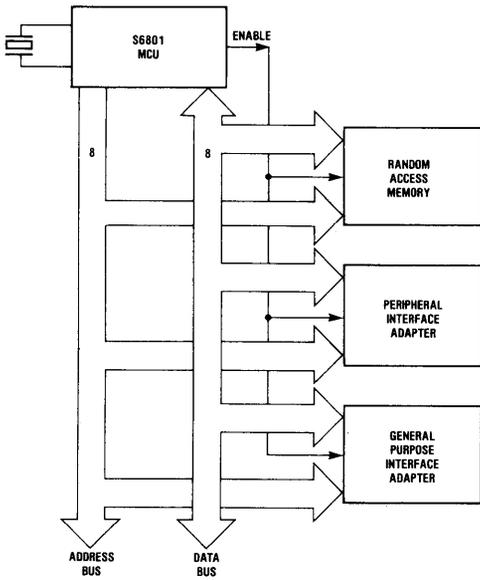
Figure 29. S6801E MCU Expanded Non-Multiplexed Mode
