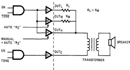
Figure 1-B. Output Stage Connected for Manual Mode Operation
