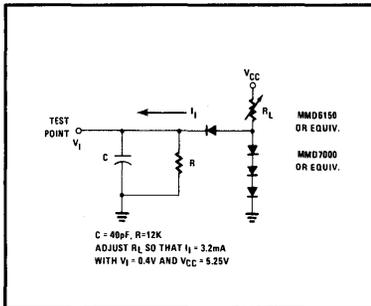
**Figure 2. CMOS Equiv. Test Load (Port A)**
