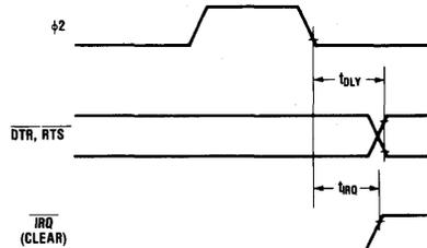
Figure 6b. Transmit Timing with External Clock
