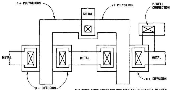
THE THIRD CMOS APPROACH ISOLATES ALL N-CHANNEL DEVICES IN SEPARATE P-WELLS. SINCE THE ISOLATED WELLS MUST BE DOPED MUCH MORE HEAVILY THAN THOSE OF THE UBIQUITOUS-WELL APPROACH,  $n^+$ -TO P-WELL CAPACITANCE IS GREATER AND SWITCHING SPEEDS LOWER. THIS IS AN  $n^+$ -ONLY POLYSILICON PROCESS.
