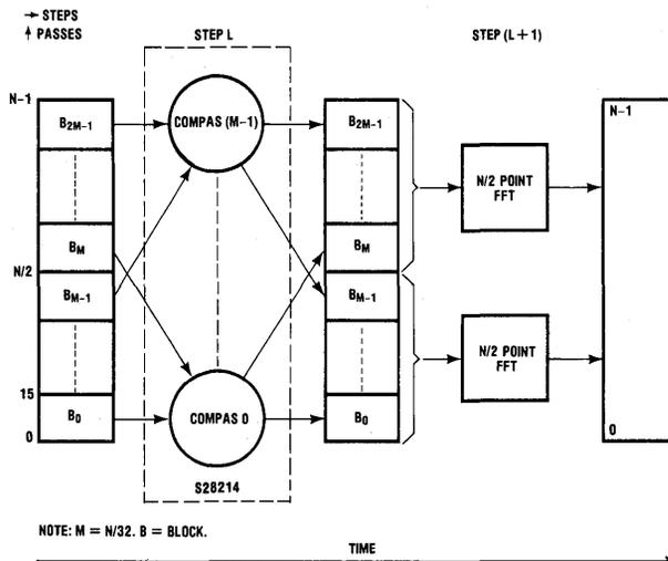
Figure 10. Flow Chart for N Point FFT, Routine "NFFT"
