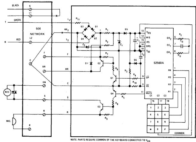
$R_1 = 10\text{-}20\text{k}\Omega$ ,  $R_2 = 2\text{k}\Omega$
