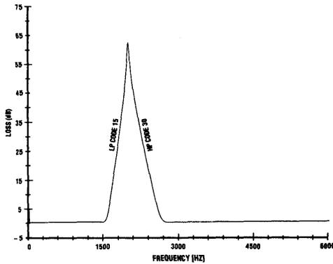
Figure 9. S3528 and S3529 in Parallel
