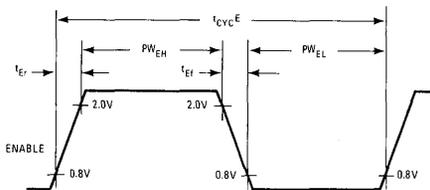
**Figure 2. Bus Read Timing Characteristics**
