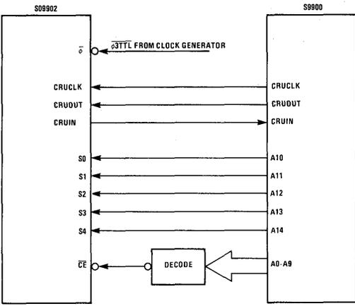
Connection of the ACC to the S9980 CPU's
