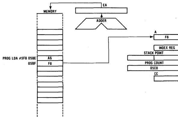
Figure 22. Direct Addressing Example
