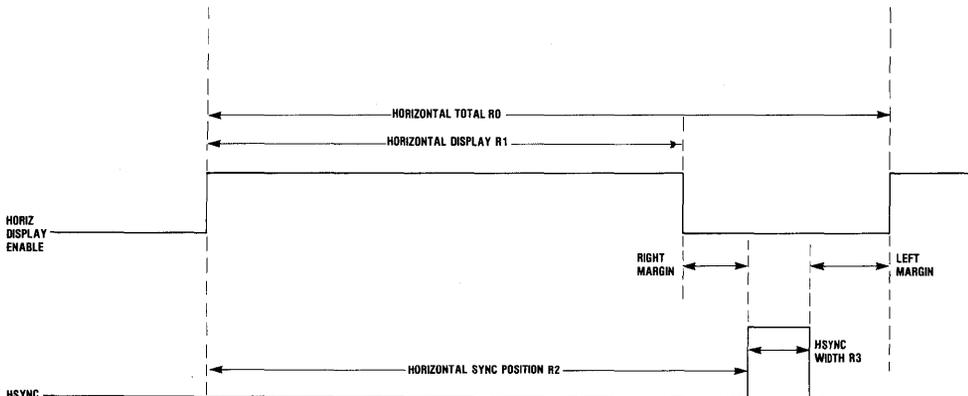
FOR MORE EXACT DIAGRAMS REFER TO THE BACK OF THE DATA SHEET. THE HORIZONTAL DISPLAY ENABLE IS ANDED WITH THE VERTICAL DISPLAY ENABLE TO PRODUCE THE DISPLAY ENABLE AT PIN 18. NOTE THE (a) FIGURE IS TIMED IN TERMS OF INDIVIDUAL CHARACTERS, WHEREAS THE (b) FIGURE IS TIMED IN TERMS OF CHARACTER ROWS.
