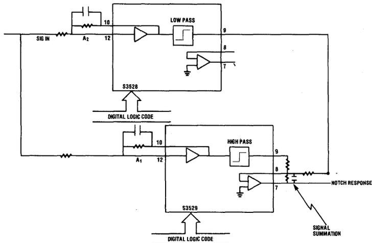
Figure 15. Low Distortion Digitally Tuned Audio Oscillator Application Circuit
