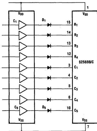
G<sub>1</sub> THRU G<sub>9</sub> ANY TYPE CMOS GATE
