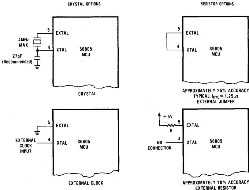
Figure 14. Crystal Parameters
