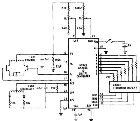
sample interval counter. The display clears to "000," with the most significant digit blanked. After two seconds, approximately, the S4036 begins to process the analog input. The display "rolls-up" from "000" to the digital value of the analog input. This "roll-up" process takes one second. The value on the display at the end of the conversion is held fixed until the  $V_{DD}$  line is pulsed to restart the process.
