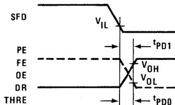
Figure 8. Control Register Load Cycle
