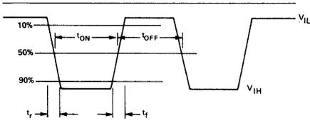
Figure 3. Output Rise and Fall Times
