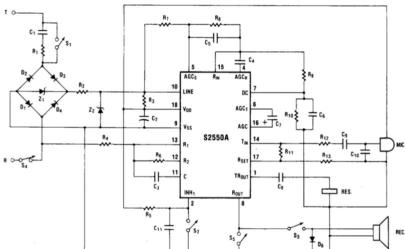
NOTES: CIRCUIT SHOWN WITH CONTACT POSITIONS IN THE ON-HOOK STATE. S1, S2 AND S3 ARE HOOKSWITCH CONTACTS. S4 AND S5 ARE ROTARY DIAL CONTACTS.
