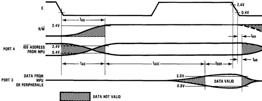
Figure 2. Write Data in Memory or Peripherals
