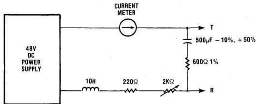
Figure 3. Typical Application Circuit for a Rotary Dial Telephone
