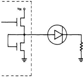
Figure 3. LED Drive — Shunt
