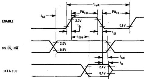
**Figure 2. Bus Write Timing Characteristics
