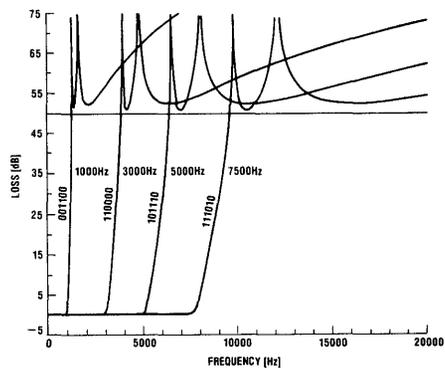
Figure 6. Passband Control Detail, Control = 110010,  $f_c = 3200\text{Hz}$
