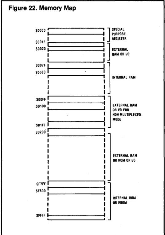
Locations  $\$0100$  through  $\$01FF$  are available in the Expanded Non-Multiplexed Mode. The eight address lines of Port 4 make this 256 word expandability possible. Those not needed for address lines can be used as input lines instead.
