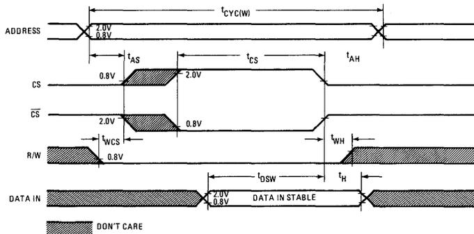
NOTE: CS AND CS-bar CAN BE ENABLED FOR CONSECUTIVE WRITE CYCLES PROVIDED R/W IS STROBED TO  $V_{IH}$  BEFORE OR COINCIDENT WITH THE ADDRESS CHANGE, AND REMAINS HIGH FOR TIME  $t_{AS}$
