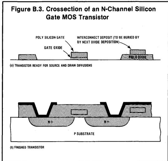
One minor limitation associated with the buried interconnect lines is their location. Because the source and drain diffusions are done after the polysilicon is deposited [see (a) of Figure B.3] the interconnect lines cannot be located over these diffusion regions.
