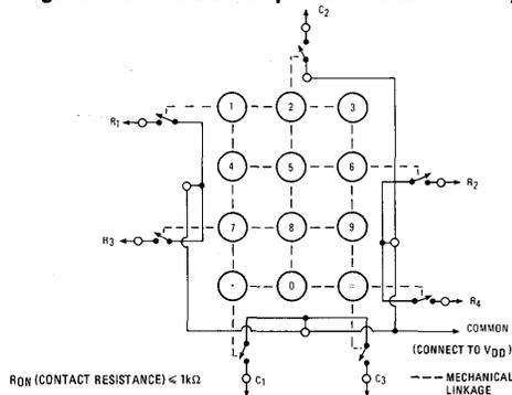
Figure 2. Logic Interface for the S2560
