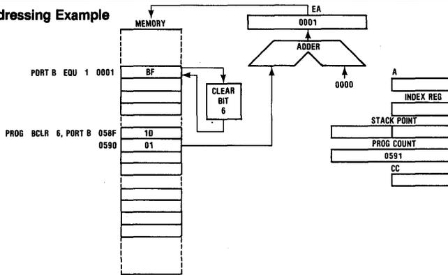
Figure 29. Bit Test and Branch Addressing Example
