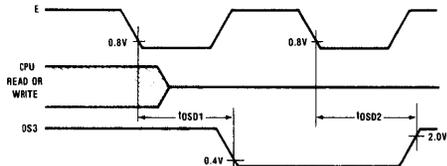
Figure 6. Input Strobe Timing — Single Chip Mode
