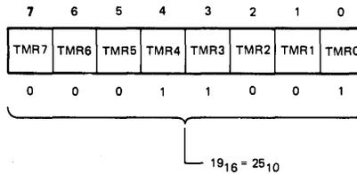
$25 \times 64 \text{ MICROSECONDS} = 1.6 \text{ MILLISECONDS}$
