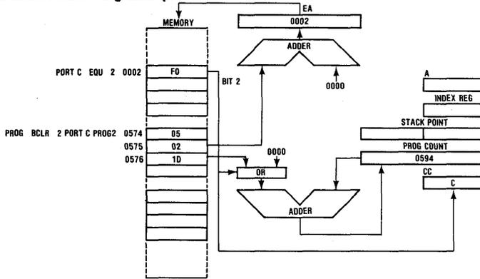
Figure 30. Inherent Addressing Example
