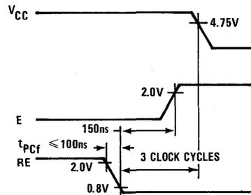
When  $\overline{\text{RESET}}$  is released it must go through the low to high threshold without bouncing, oscillating, or otherwise causing an erroneous  $\overline{\text{RESET}}$  (less than 3 clock cycles). This may cause improper MPU operation.
