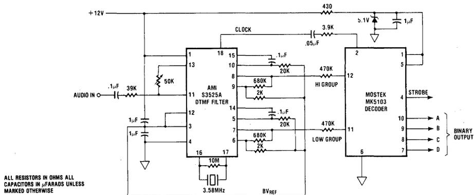
**Figure 5. AMI/Nitron 2 Chip DTMF Receiver**
