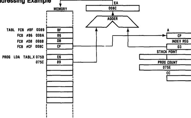
Figure 27. Indexed (16-Bit Offset) Addressing Example
