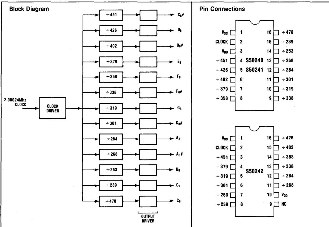
RFI emission and feed-through are minimized by placing the input clock between the  $V_{DD}$  and  $V_{SS}$  pins. Internally the layout of the chip isolates the output buffer circuitry from the divisor circuit clock lines. Also, the
