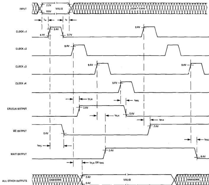
† The number of cycles over which input/output data must/will remain valid can be determined from the number of wait states required for memory access. Note that in all cases data should not change during  $\phi 1$ .
