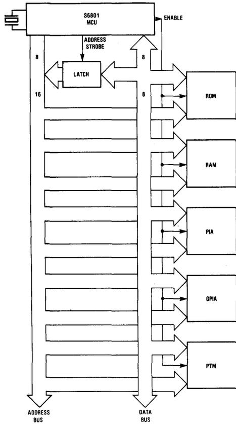
**Figure 31. S6801E MCU Expanded Multiplexed Mode**
