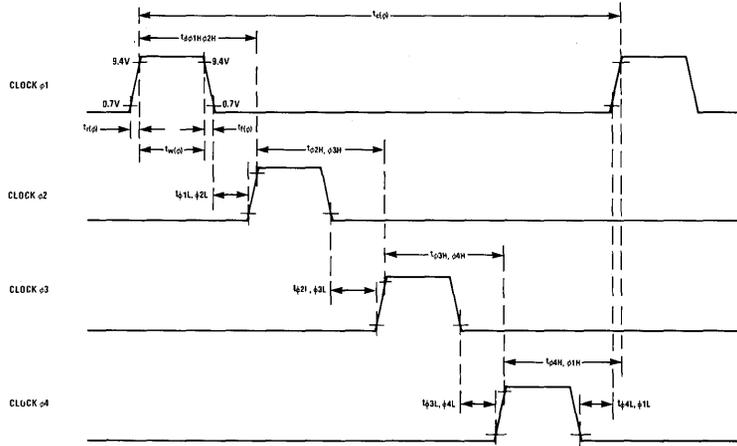
Note: All timing and voltage levels shown on  $\phi 1$  apply to  $\phi 2$ ,  $\phi 3$ , and  $\phi 4$  in the same manner.
