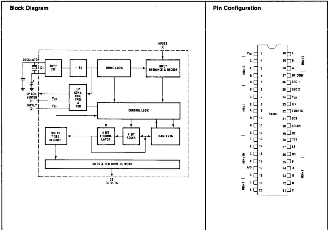
A functional description of the inputs/outputs and registers follows:
