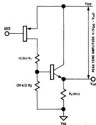
Figure 5. Typical Single Tone Output Amplitude Vs Supply Voltage ( $R_L = 10k$ )
