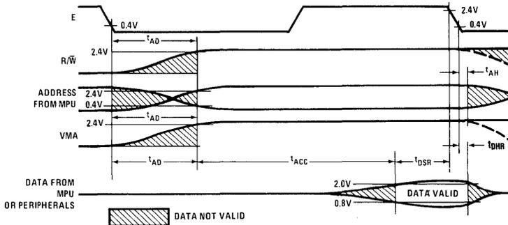
**Figure 2. Write Data in Memory or Peripherals**
