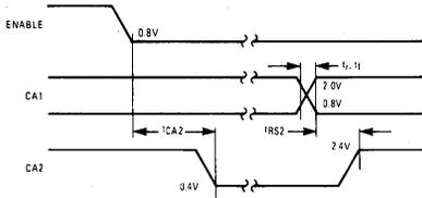
**Figure 11. Peripheral CMOS Delay Times**
