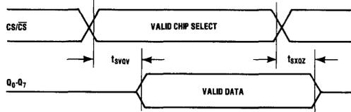
Propagation From Chip Enables (Address Valid)
