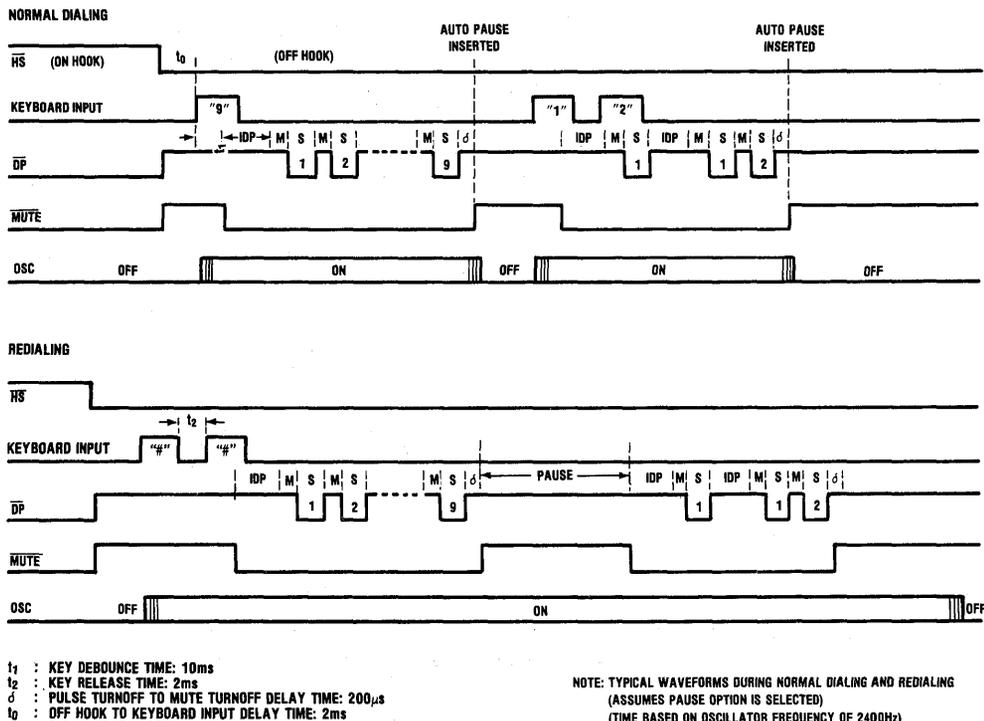
The Inter-Digit Pause (IDP) time is also derived from the oscillator frequency and it is a function of the dialing rate selected by the dial rate select input. If the oscillator is set to 2400Hz so that a dialing rate of 10pps is obtained with  $DRS = V_{SS}$ . Then an IDP of 800ms is automatically selected. Switching the dialing rate to 20pps ( $DRS = V_{DD}$ ) will lower the IDP to 400ms.
