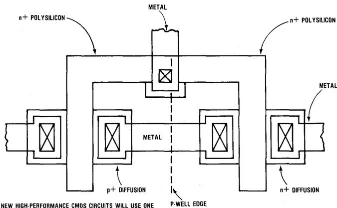
ALL NEW HIGH-PERFORMANCE CMOS CIRCUITS WILL USE ONE TYPE OF POLYSILICON. THIS VERSION HAS A UBIQUITOUS P-WELL: THAT IS, SERIES N-CHANNEL DEVICES SIT IN A COMMON P-WELL, WHICH, IMPLANTED BEFORE FIELD OXIDATION, RUNS UNDER THE FIELD OXIDE. THIS IS AMI'S PREFERRED CMOS PROCESS FORMAT FOR ALL NEW DESIGNS.
