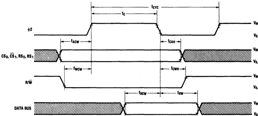
Read Cycle ( $V_{CC} = 5.0V \pm 5\%$ ,  $T_A = 0^\circ C$  to  $+70^\circ C$ , unless otherwise noted)
