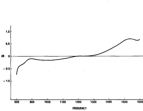
Figure 3. Typical Low-Band Group Delay
