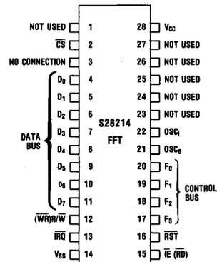
NOTE: PIN FUNCTIONS IN PARENTHESIS APPLY ONLY TO B VERSION
