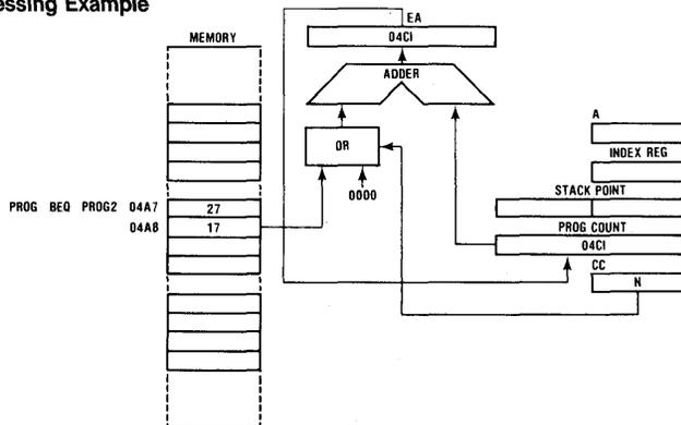
Figure 25. Indexed (No Offset) Addressing Example
