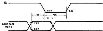
Figure 7. Multiplexed Bus Timing
