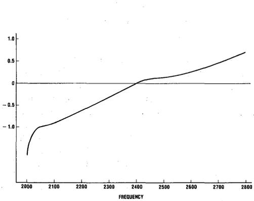
Figure 5. Typical High-Band Group Delay
