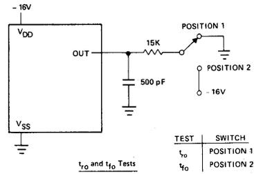
Figure 2. Output Signal DC Loading
