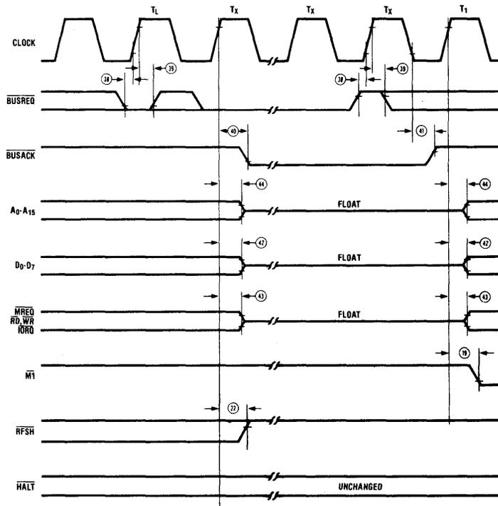
NOTE:  $T_1$  = LAST STATE OF ANY M CYCLE.
