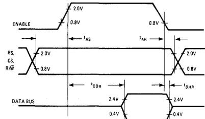
Figure 3. Bus Write Timing Characteristics (Write Information into PIA)
