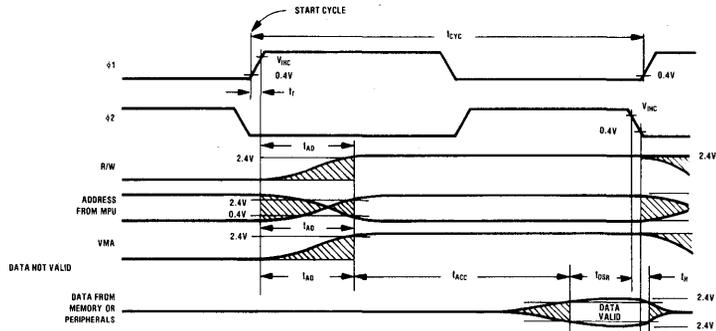
Figure 4. Write Data in Memory or Peripherals
