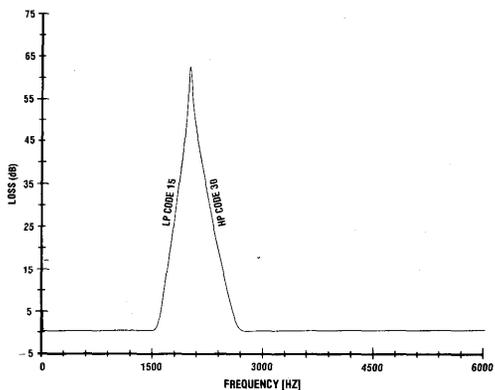
Figure 13. Bandpass Application: General Case Configuration
