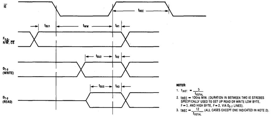
S28214 Timing Specifications (5V ± 5%, T<sub>A</sub> = 0°C – 70°C)
