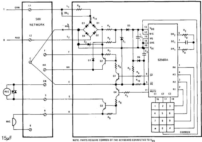
$R_0 = 10\text{-}20\text{k}\Omega$ ,  $R_1 = 150\text{k}\Omega$ ,  $R_2 = 2\text{k}\Omega$
