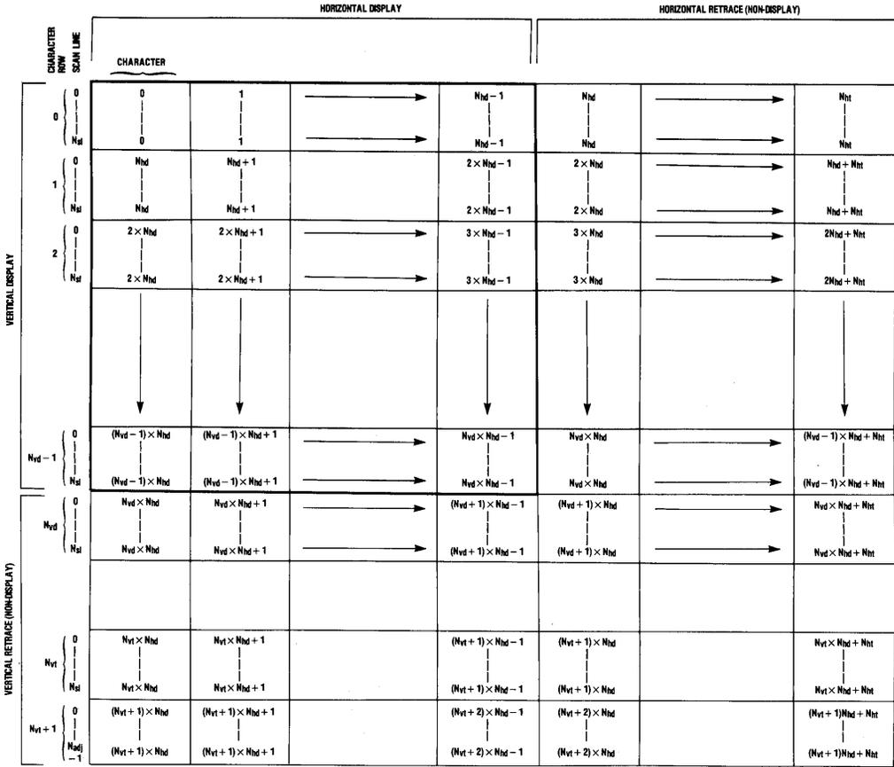
NOTE 1: THE INITIAL MA IS DETERMINED BY THE CONTENTS OF START ADDRESS REGISTER, R12/R13. TIMING IS SHOWN FOR R12/R13 = 0. ONLY NON-INTERFACE AND INTERFACE SYNC MODES ARE SHOWN.
