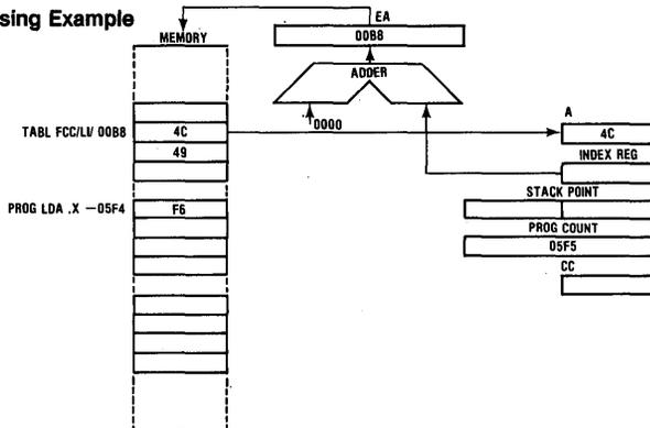
Figure 26. Indexed (8-Bit Offset) Addressing Example
