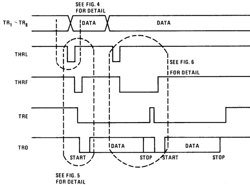
Figure 4. Data Input Load Cycle
