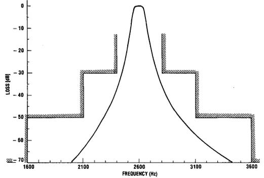
Figure 3. Typical Notch Response
