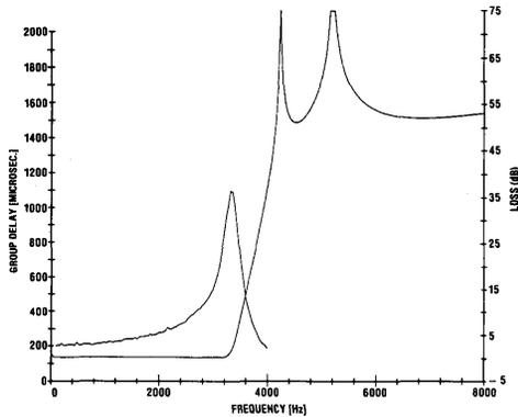
Figure 9. Group Delay, Control = 110010,  $F_c = 3.2\text{kHz}$
