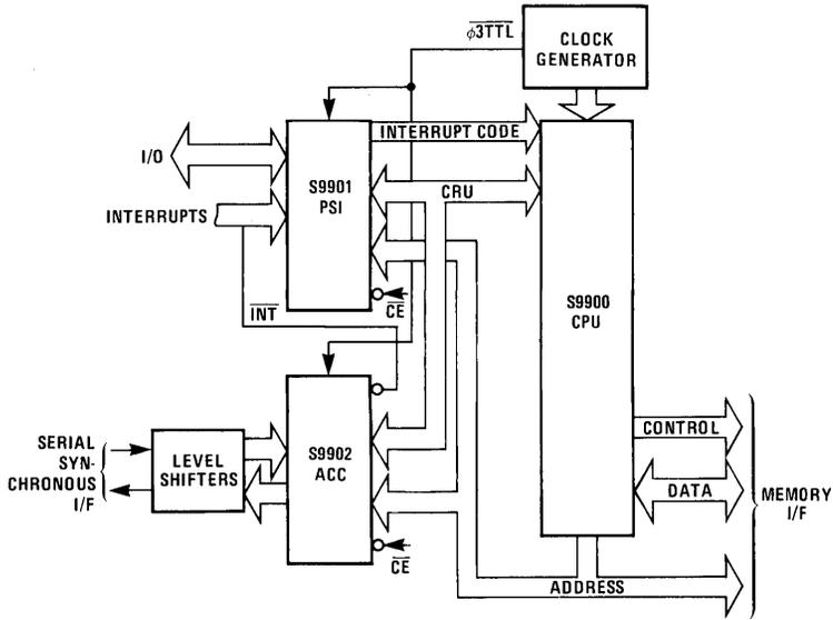
Figure 5. S9902 ACC in an S9980 System
