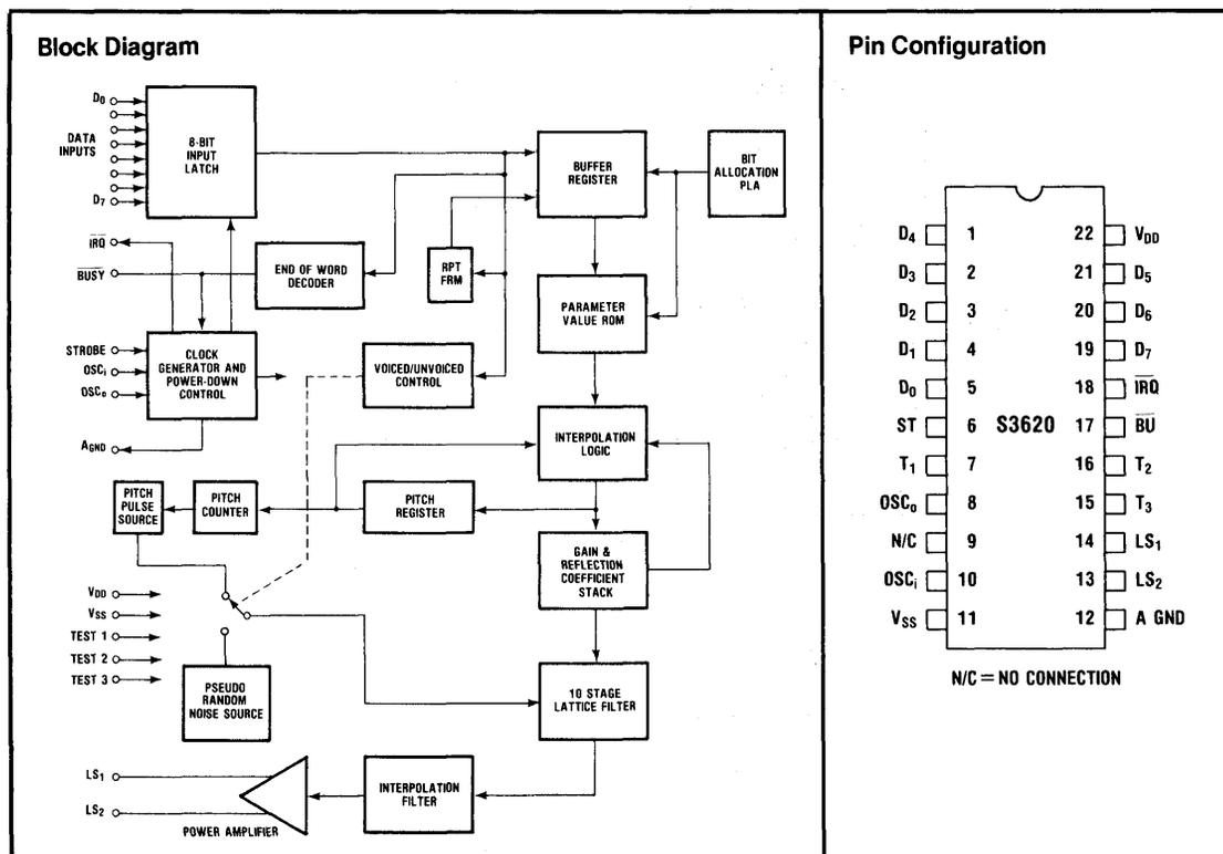
The synthesizer is realized using analog switched-capacitor filter technology and operates at 8K samples/sec. An output interpolating filter and bridge power amplifier give 30mW output power at 6 volts supply and allow the device to be connected directly to a 100Ω loudspeaker.
