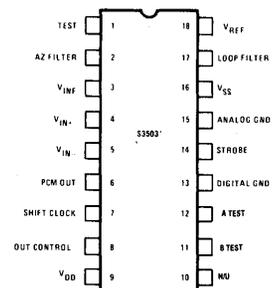
PIN 10, 11, 12 TO VDD FOR NORMAL OPERATION. PIN 1 TO VSS
