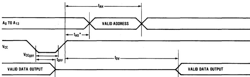
\*  $t_{AS}$  MAY BE A NEGATIVE NUMBER SINCE THE ADDRESS DOES NOT HAVE TO BE VALID WHEN  $V_{CC}$  GOES ON BUT MAY OCCUR AFTERWARDS
