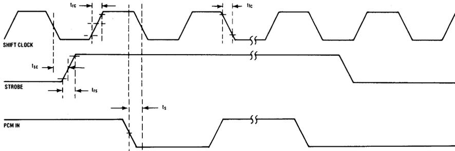
Figure 6-B. Decoder A/B Output Timing
