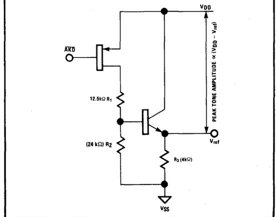
Figure 5. Typical Single Tone Output Amplitude Vs Supply Voltage ( $R_L = 10k$ )
