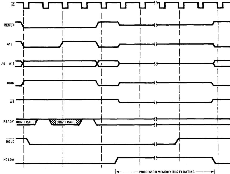
**Figure 5. S9980A/S9981 CRU Interface Timing**
