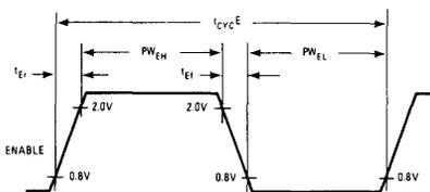
Figure 2. Bus Read Timing Characteristics (Read Information from PIA)
