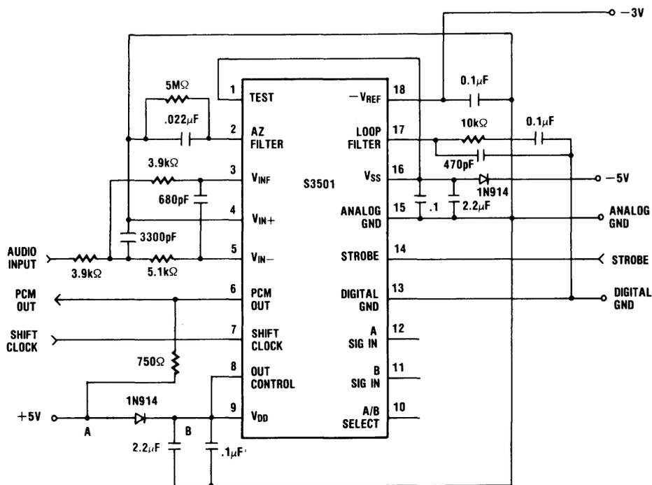
NOTE: TEST PIN 1 MUST BE CONNECTED TO PIN 16 (NOT -5V) TO PREVENT FORWARD BIASING THE PIN.
