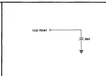
**Figure 3. TTL Equiv. Test Load (Ports A and C)**
