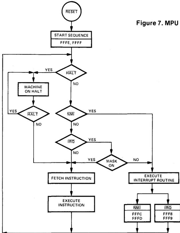
Figure 7. MPU Flow Chart
