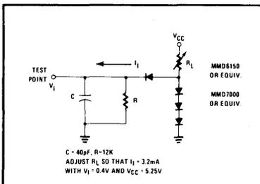
**Figure 2. CMOS Equiv. Test Load (Port A)**
