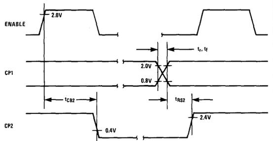
**Figure 8. Input Pulse Widths**
