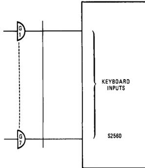
G1 through G7 any CMOS type logic gates
