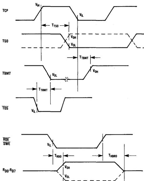
Figure 3. Transmitter Timing Diagram
