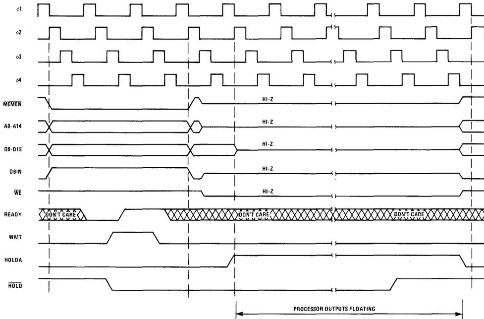
Figure 5. S9900 CRU Interface Timing
