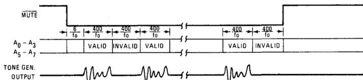
Mute output will reset i) when the number of digits dialed out equals the number of digits entered or equals the maximum selected (8 or 16) or ii) when an access pause is detected. In the normal dialing mode when digits are entered one at a time the mute output will reset between digits provided the time between entered digits exceeds  $\frac{400}{fo}$ . In both the normal dialing or automatic dialing mode tone will be output for a fixed duration of  $\frac{400}{fo}$  (150msec for fo = 8kHz).
