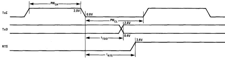
Figure 4. TDSR/RDSR Delays, IRQ Release Delay, RTS and DTR Delay Timing
