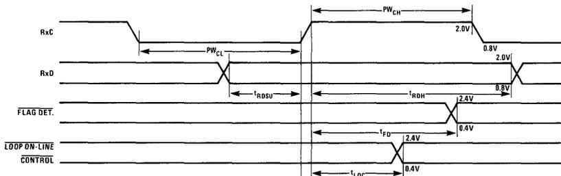
Figure 3. Transmit Data Output Delay and Request to Send Delay Timing
