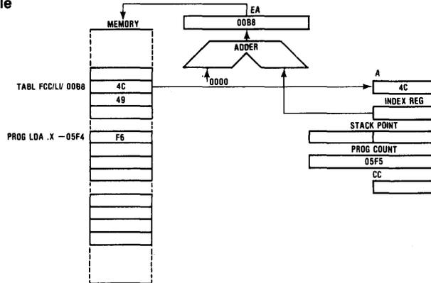
**Figure 26. Indexed (8-Bit Offset) Addressing Example**
