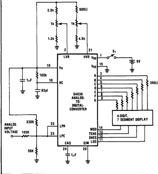
**Figure 2. Typical Digital Scale Application**
