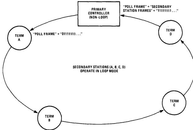
Figure 8B. Example of External Loop Logic
