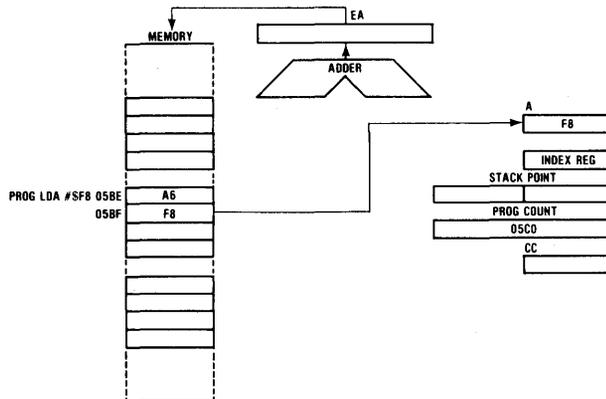
Figure 22. Direct Addressing Example
