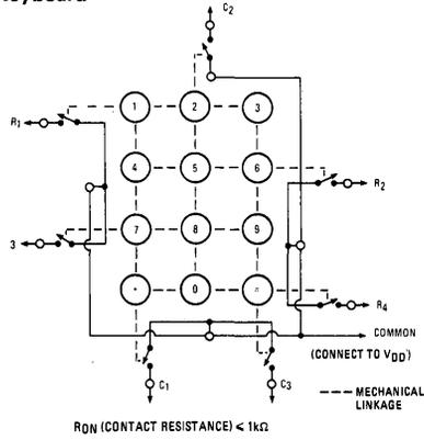
**Figure 2. Logic Interface For the S2560**
