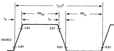
Figure 2. Bus Read Timing Characteristics
