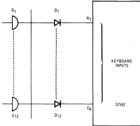
G1 through G12 any CMOS type logic gates.
