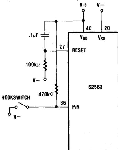
**Figure 6B. Telephone Line Power**
