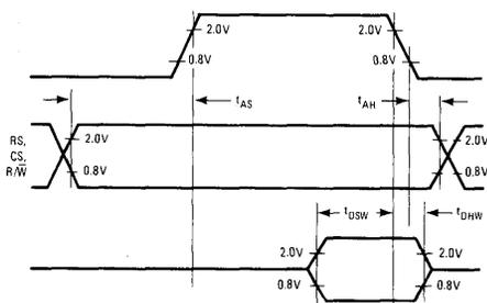
Figure 4. Bus Timing Test Loads
