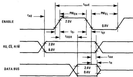
Figure 4. Bus Write Timing Characteristics (Write Information into GPIA)
