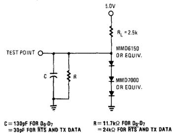
Figure 5. Transmit/Receive Timing
