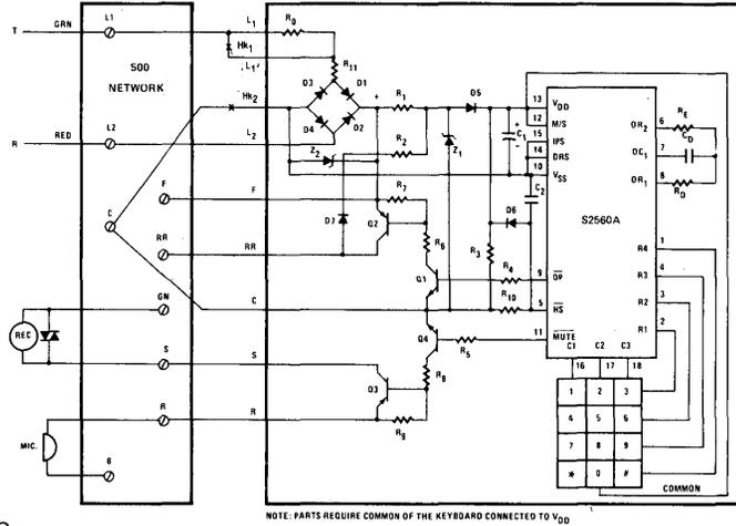
$R_0 = 10\text{-}20\text{M}\Omega$ ,  $R_1 = 150\text{k}\Omega$ ,  $R_2 = 2\text{k}\Omega$
