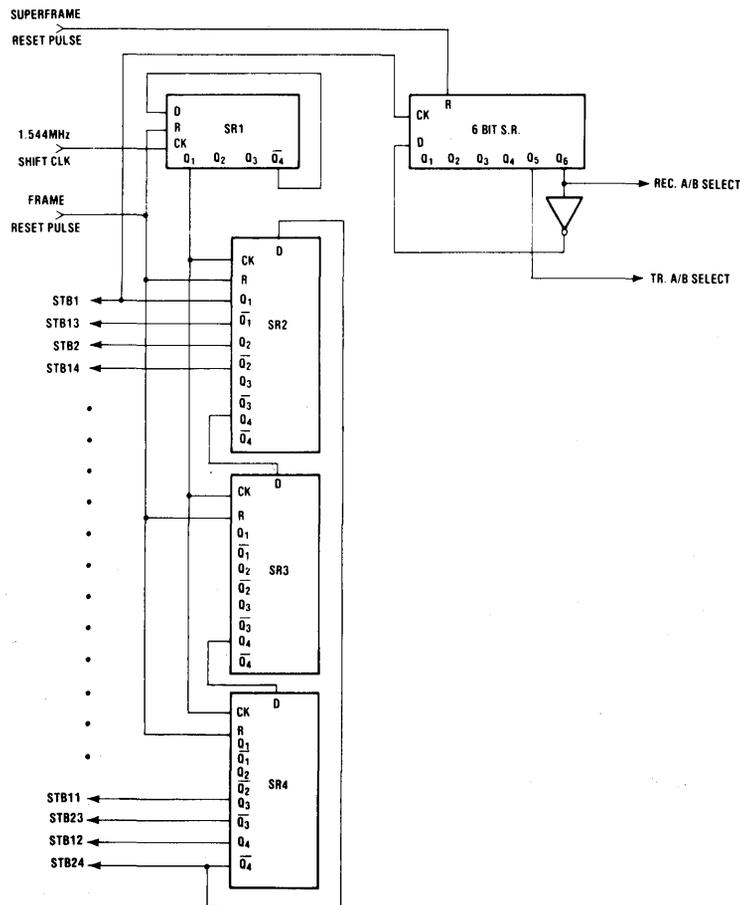
Figure 5A. Generating Timing Signals in a CCITT Carrier System (30 + 2 Channels)
