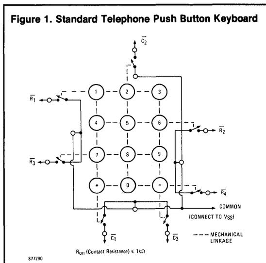
logic levels. Low levels on a row and a column input corresponds to a key closure. The pull-up resistors present on the row and column inputs are in the range of 20kΩ -100kΩ.
