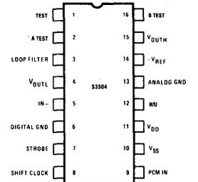
PIN 1 TO DIGITAL GROUND, PIN 2, 16 OPEN FOR NORMAL OPERATION
