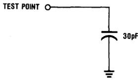
Figure 9. Bus Timing Test Load and Ports 1, 3 and 4 for Single Chip Mode
