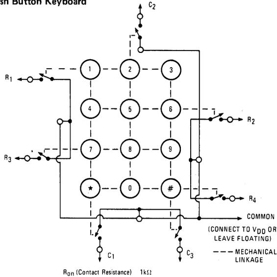
Figure 2. SPST Matrix Keyboard Arranged in the 2 of 8 Row, Column Format
