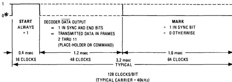
\* "1" MEANS PRESENCE OF A 40kHz CARRIER (SQUARE WAVE); "0" MEANS ABSENCE OF A 40kHz CARRIER (SQUARE WAVE).
