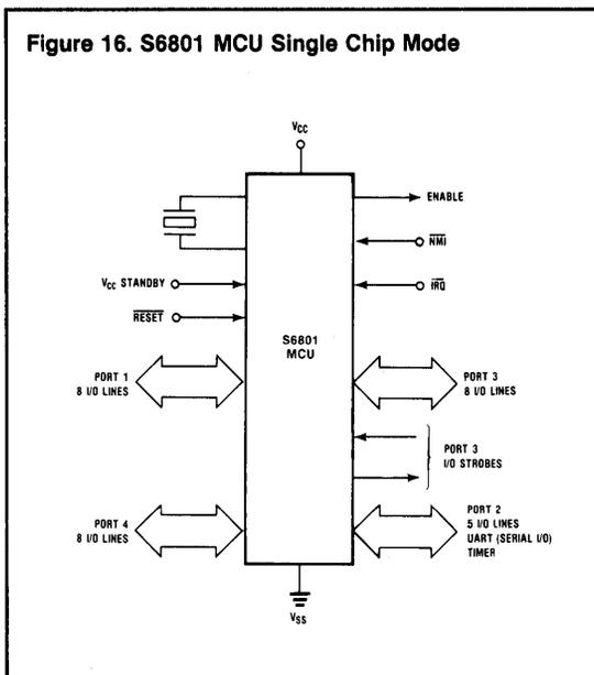
Figure 16a. S6801E MCU Single-Chip Mode
