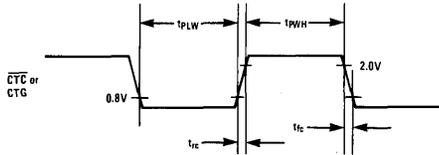
**Figure 9. Input Setup and Hold Times**
