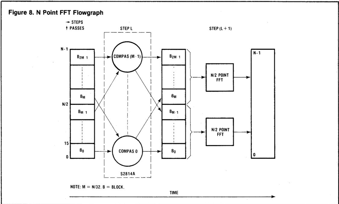
Figure 9. Flow Chart for N Point FFT, Routine 'NFFT'
