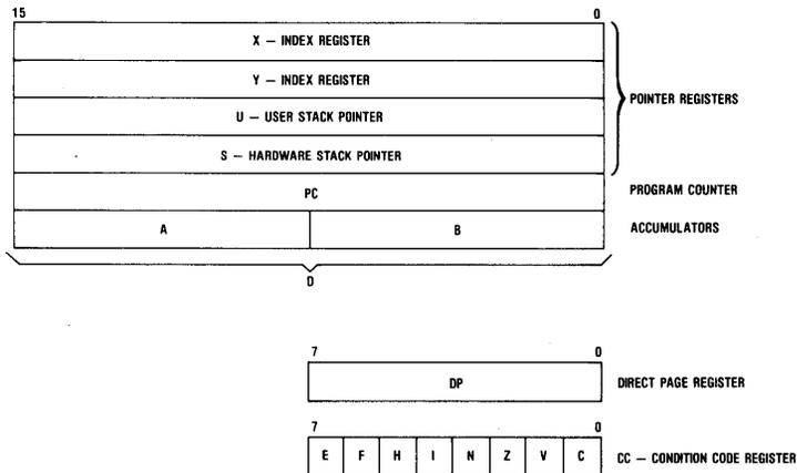
**Figure 5. Condition Code Register Format**
