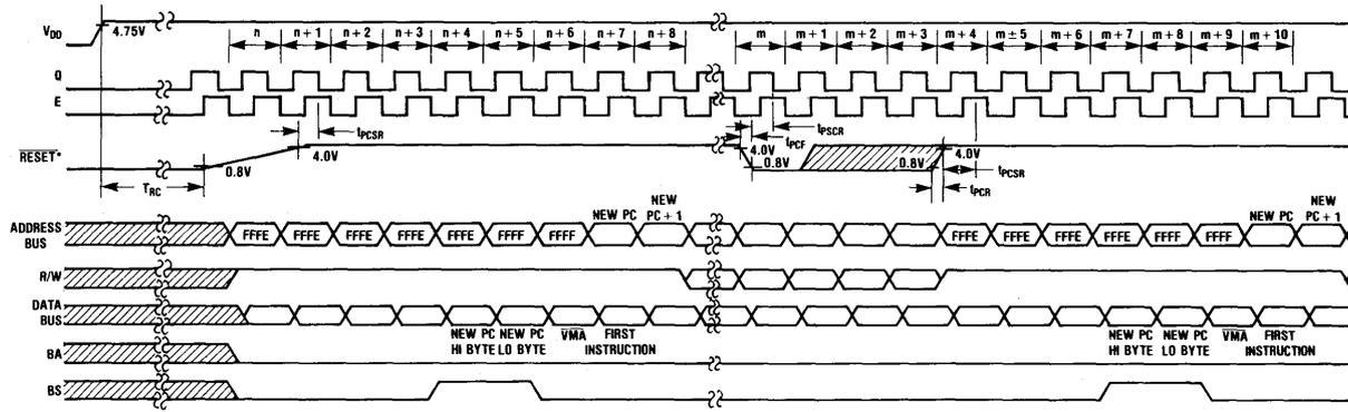
\*NOTE: PARTS WITH DATE CODES PREFIXED BY 7F WILL COME OUT OF RESET ONE CYCLE SOONER THAN SHOWN
