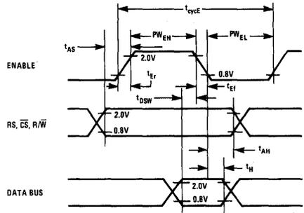
**Figure 3. Input Pulse Width Low**
