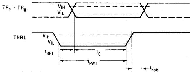
Figure 5. Transmitter Output Timing (1)
