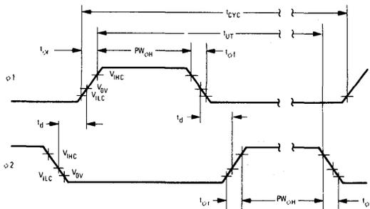
Figure 1. Clock Timing Waveform
