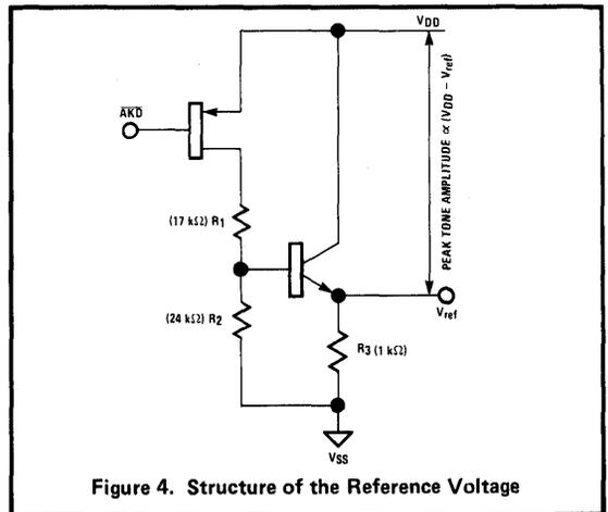
Figure 4. Structure of the Reference Voltage
