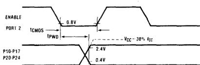
Figure 8. CMOS Load
