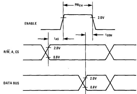
**Figure 4. Peripheral Data and CP2 Delay
