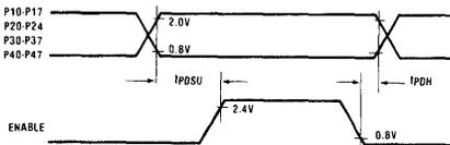
**Figure 4. Peripheral CMOS Data Delay Times
