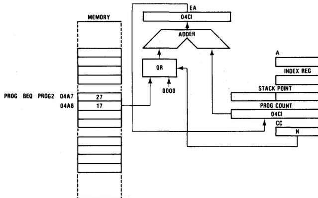
**Figure 25. Indexed (No Offset) Addressing Example**
