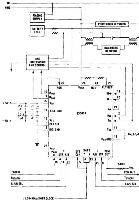
The decoder uses a similar scheme for receiving the A and B signaling bits, with one difference. They are latched to the respective outputs in the same frame in which the A/B select input makes a transition. Therefore, the receive A/B select input must go high at the beginning of frame 6 and go low at the beginning of frame 12.
