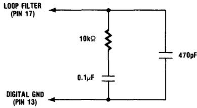
**Figure 9-B. Supply Decoupling for the V<sub>SS</sub> Supply Pin**
