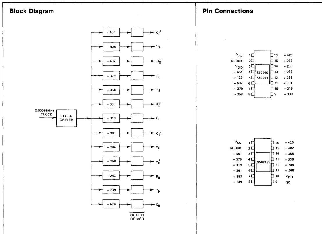
RFI emanation and feed-through are minimized by placing the input clock between the  $V_{DD}$  and  $V_{SS}$  pins. Internally the layout of the chip isolates the output buffer circuitry from the divisor circuit clock lines. Also, the output buffers limit the minimum rise time under no load conditions to reduce the R.F. harmonic content of each output signal.
