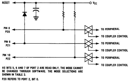
**Figure 15. Quad Analog, Switch/Multiplexer in a Typical S6801 Circuit**
