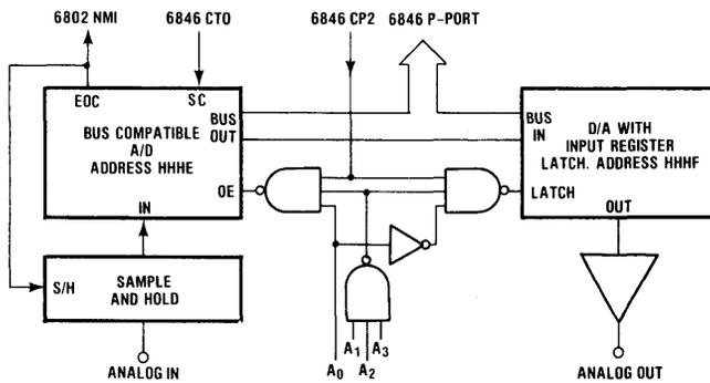
Figure 13. Interfacing the S2814A with a Microprocessor
