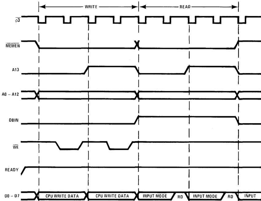
Figure 3b. S9980A/S9981 Memory Bus Timing (One Wait State)
