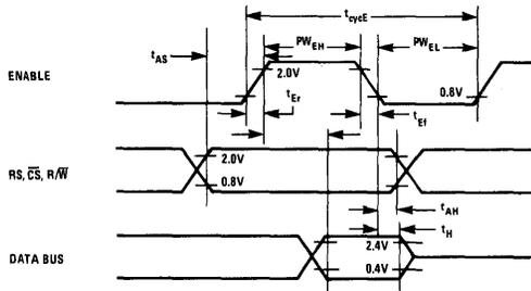
**Figure 2. Bus Write Timing Characteristics
