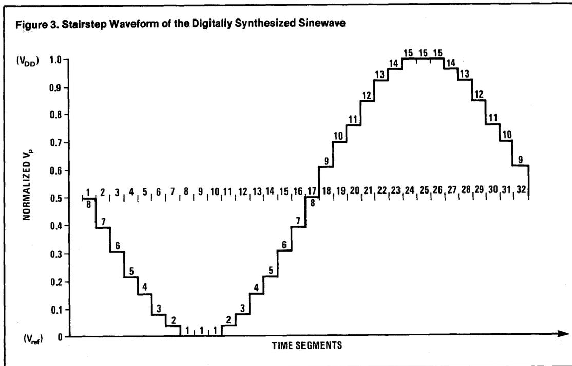
The individual tones generated by the sinewave synthesizer are then linearly added and drive a Darlington NPN transistor connected as an emitter follower to allow proper impedance transformation at the same time preserving signal level.
