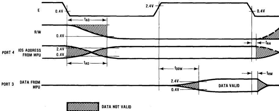
**Ports 1 and 2, and Ports 3 and 4 in the Single Chip Mode**
