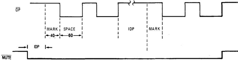
Mute will reset i) when the number of digits dialed out equals either the number of digits entered or the maximum selected (8 or 16) or ii) when an access pause is detected.
