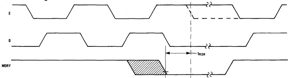
**Figure 13. Typical DMA Timing (< 14 Cycles)**
