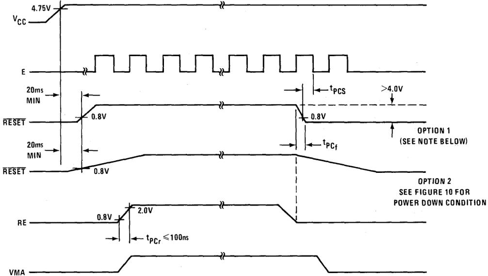
NOTE: IF OPTION 1 IS CHOSEN, RESET AND RE PINS CAN BE TIED TOGETHER.
