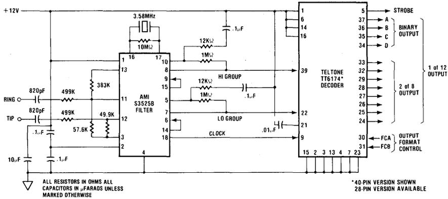
**Figure 4. AMI/Mostek 2 Chip DTMF Receiver**
