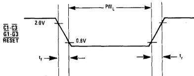
**Figure 4. Input Pulse Width High**
