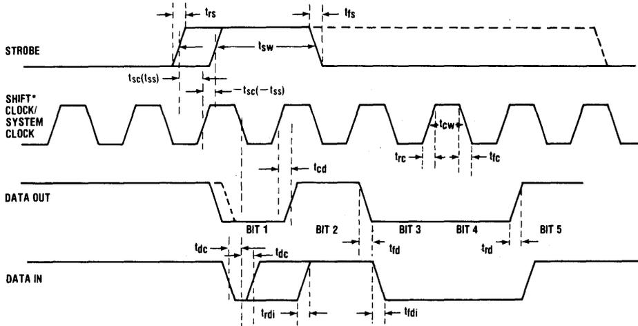
\*In this example the shift clock is the system clock (1.544 or 2.048MHz). In systems where the data shift rate is not the same the relationship of each to the strobe remains the same. The system clock and shift clock need not have coincident edges, but must relate to the strobe within the  $t_{sc}$ ,  $t_{ss}$  timing requirements.
