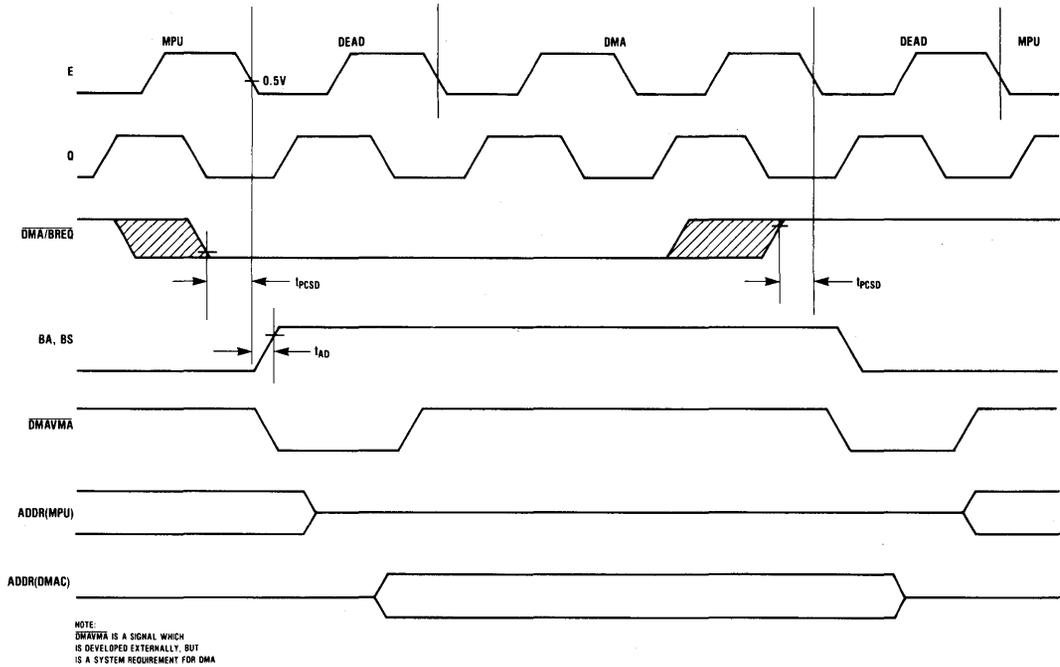
**Figure 14. Auto-Refresh DMA Timing (< 14 Cycles)**
