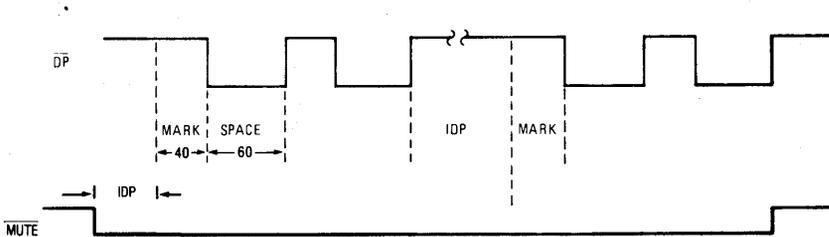
Mute will reset i) when the number of digits dialed out equals either the number of digits entered or the maximum selected (8 or 16) or ii) when an access pause is detected.
