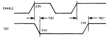
**Figure 14. CB2 Delay Time**
