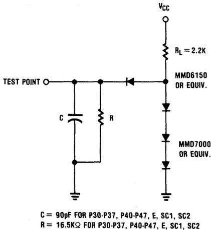
Figure 10. Test Loads for Port 1 Darlington Load (P10-P17)
