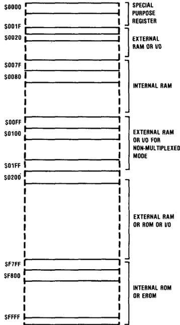
Locations \$0100 through \$01FF are available in the Expanded Non-Multiplexed Mode. The eight address lines of Port 4 make this 256 word expandability possible. Those not needed for address lines can be used as input lines instead.
