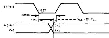
**Figure 12. Peripheral Data and CB2 Delay Times**
