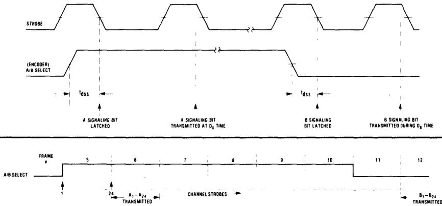
**Figure 2-B. CODEC System Timing Diagram**
