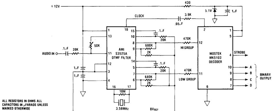
**Figure 5. AMI/Rockwell 2 Chip DTMF Receiver**
