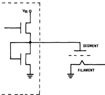
**Figure 5. Liquid Crystal Drive**
