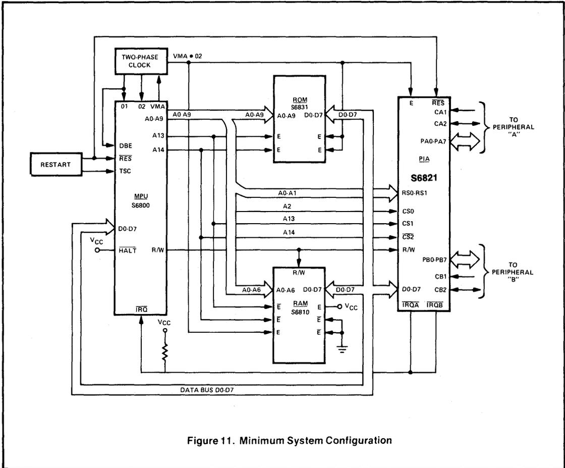
Figure 11. Minimum System Configuration
