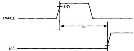
**Figure 6. Peripheral Port Setup Time**
