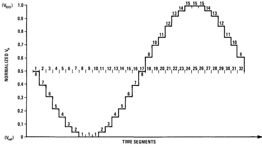
The individual tones generated by the sinewave synthesizer are then linearly added and drive a bipolar NPN transistor connected as emitter follower to allow proper impedance transformation, at the same time preserving signal level.
