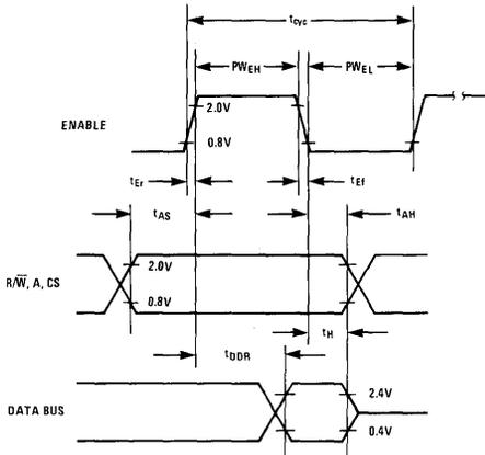
**Figure 3. Bus Write Timing
