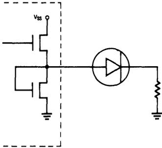
**Figure 3. LED Drive — Shunt**
