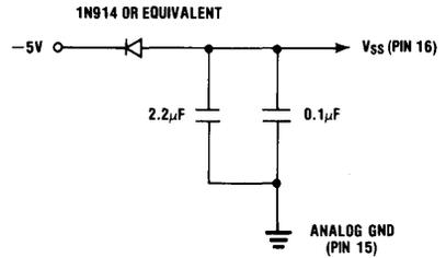
**Figure 9-A. Supply Decoupling for the V<sub>DD</sub> Supply Pin**
