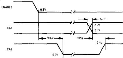
**Figure 11. Peripheral CMOS Data Delay Times**
