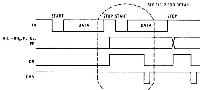
**Figure 2. Timing for Status Flags, RR<sub>1</sub> thru RR<sub>8</sub> and DR**
