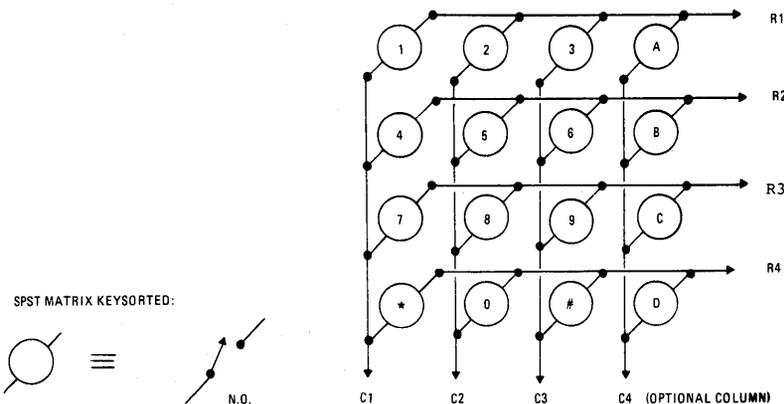
Figure 3. Logic Interface for Keyboard Inputs of the S2559
