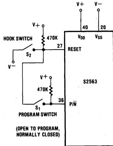
Figure 7. Typical Application of the S2563
