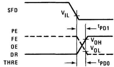
Figure 8. Control Register Load Cycle
