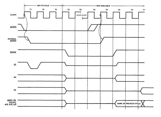
Figure 10. Bus Request/Acknowledge Cycle.
