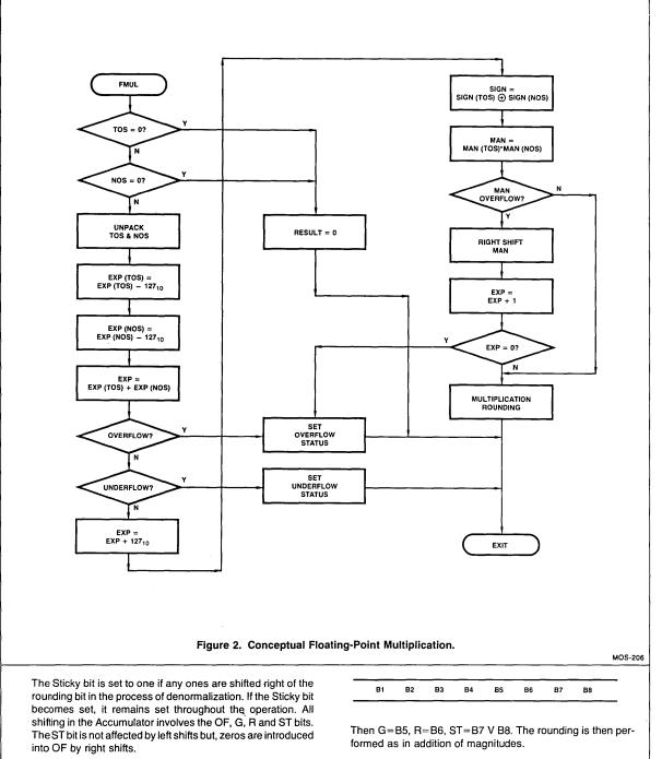
Rounding during addition of magnitudes - add 1 to the G position, then if G=R=ST=0, set B4 to 0 ("Rounding to Even").
