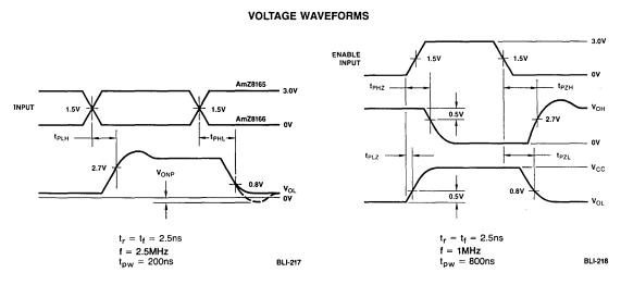
Figure 3. Output Drive Levels.
