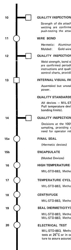
Strength of die attachment, position of die and visual quality of eutectic wetting are confirmed periodically by inspecting random samples and push-testing the attached dice.
