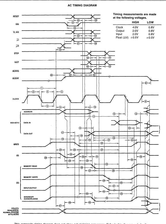
This composite timing diagram does not show actual timing sequences. Refer to this diagram only for the detailed timing relationships of individual edges. Use the preceding illustrations as an explanation of the various timing sequences.
