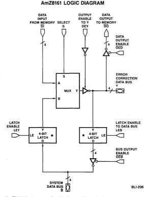
\*AmZ8162 is the same function but non-inverting between the Y bus to the system data bus, B. This is done by making both latches inverting.
