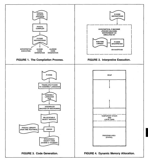
Therefore the total memory space required for data storage dynamically expands and contracts at run time coinciding with function or procedure entries and exists, taking up memory space only as needed. This allows execution of much larger programs than would otherwise be possible.
