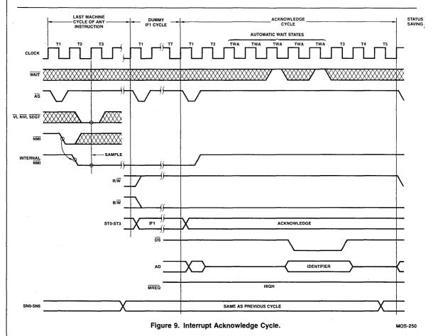
During this dummy IF1 cycle, the program counter is not updated; instead the implied system stack pointer (RR14') will be decremented. Following the dummy IF1 cycle is the actual interrupt/trap acknowledge cycle.
