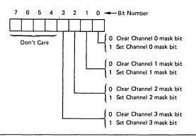
Status Register: The Status registers may be read out of the Am9517A by the microprocessor. It indicates which channels have reached a terminal count and which channels have pending DMA requests. Bits 0-3 are set each time a TC is reached by that channel, including after each Autoinitialization. These bits are cleared by Reset and each Status Read. Bits 4-7 are set whenever their corresponding channel is requesting service.
