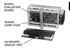
Photo showing use of the AMC 95/6440 Card Cage to house and power the 96/4016 Evaluation Board. Optional Keyboard/Display Unit shown above (or standard CRT Terminal) attaches via cable to edge-card connector. This arrangement provides both convenience and expansion capabilities for specific project and product development.
