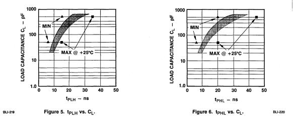
The curves above depict the typical  $t_{PLH}$  and  $t_{PHL}$  for the RAM Driver outputs as a function of load capacitance. The minimums and maximums are shown for worst case design. The typical band is provided as a guide for intermediate capacitive loads.
