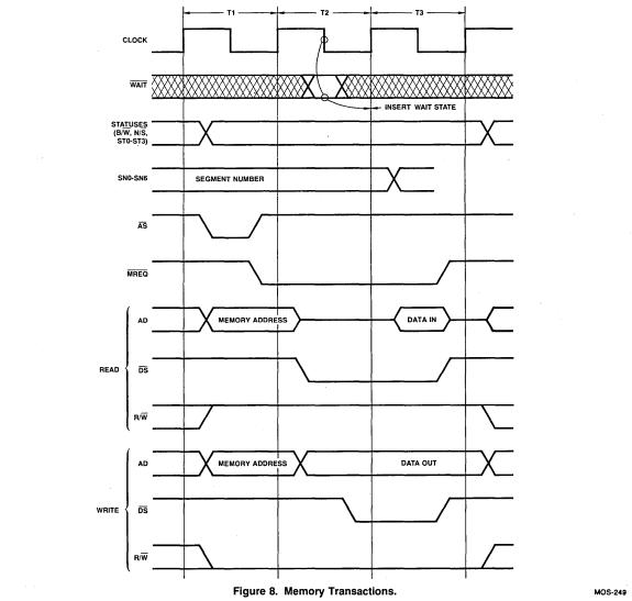
between T2 and T3 by activating the WAIT input LOW. The WAIT input will be sampled during T2 and during every subsequent TW. The ST0-ST3 outputs will reflect the appropriate code for the current cycle early in T1 and the AS output will be pulsed LOW to mark the beginning of the cycle. The N/S output will indicate whether the normal or system address space will be used for the current cycle. As shown in the figure the MREQ output will go LOW during T1 to indicate a memory operation.
