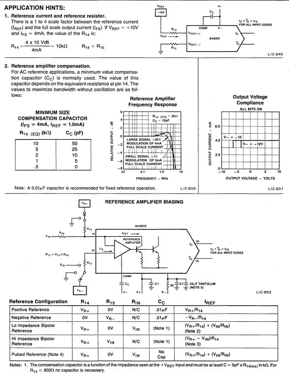
2. For negative values of V<sub>IN</sub>, V<sub>R+</sub>/R<sub>14</sub> must be greater than  $-V_{IN}$  Max/R<sub>IN</sub> so that the amplifier is not turned off. 3. For positive values of V<sub>IN</sub>, V<sub>R+</sub> must be greater than V<sub>IN</sub> Max so the amplifier is not turned off.
