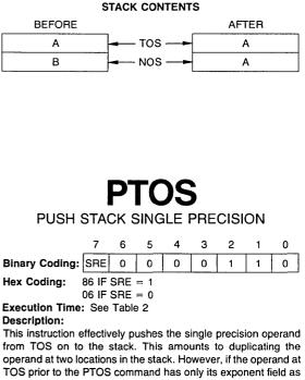
operand at two locations in the stack. However, if the operand at TOS prior to the PTOS command has only its exponent field as zero, the new content of the TOS will all be zeroes. The contents of NOS will be an exact copy of the old TOS. The status bits S and Z are affected to report the sign of the new TOS and if the content of TOS is zero, respectively. The status bits U, V and D will be cleared to zero.
