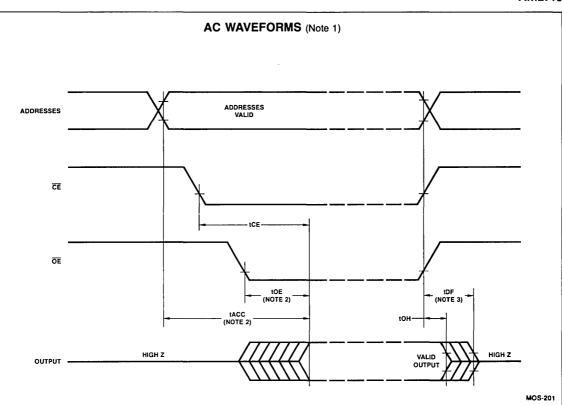
Notes: 1. <u>VCC</u> must be applied simultaneously or before VPP and removed simultaneously or after VPP.
