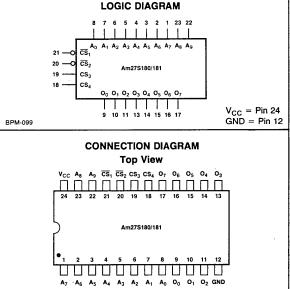
Note: Pin 1 is marked for orientation.
