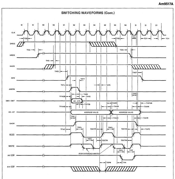
Timing Diagram 3. Active Cycle Timing Diagram.
