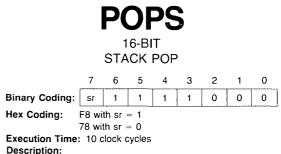
The 16-bit stack is moved up so that the old NOS becomes the new TOS. The previous TOS rotates to the bottom of the stack. All operand values are unchanged. Status Affected: Sign, Zero
