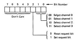
Software requests will be serviced only if the channel is in Block mode. When initiating a memory-to-memory transfer, the software request for channel 0 should be set.
