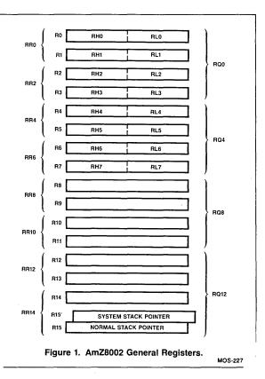
word (32-bit) registers. Similarly, the sixteen registers can be grouped in quadruples RQ0, RQ4, RQ8 and RQ12 to form four 64-bit registers.
