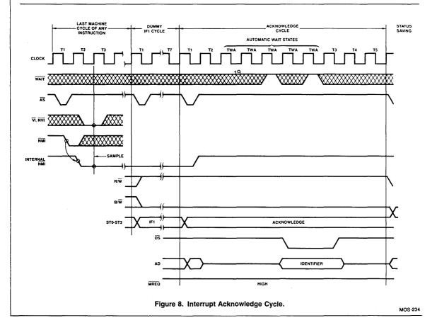
input is HIGH. After completing the last TW state T3 will be entered and the  $\overline{\text{DS}}$  output will go HIGH. The interrupting device should remove the identifier and cease driving the bus. T4 and T5 states will follow T3 to complete the cycle. Following the interrupt acknowledge cycle will be memory transaction cycles to save the status on the stack. Note that the N/S output will be automatically LOW during status saving.
