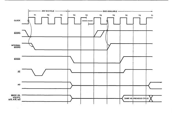
Figure 9. Bus Request/Acknowledge Cycle.
