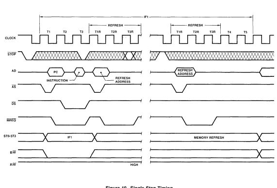
Figure 10. Single Step Timing.
