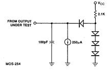
All AC parameters assume a load capacitance of 100pF max, except for parameter 6, TdC(SNv) (50pF max). Timing references between two output signals assume a load difference of 50pF max.
