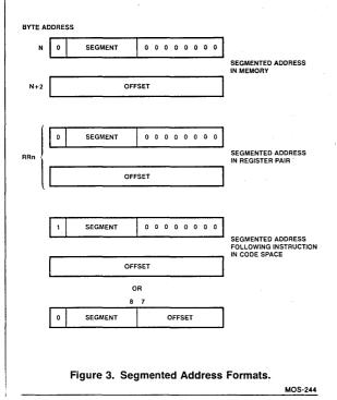
When an effective segmented address is being computed according to the designated addressing mode, the segment number is not affected by any carry from the 16-bit offset.
