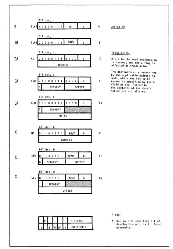
BIT test in a byte (dynamic)
