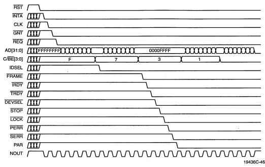
Figure 43. NAND Tree Waveform
