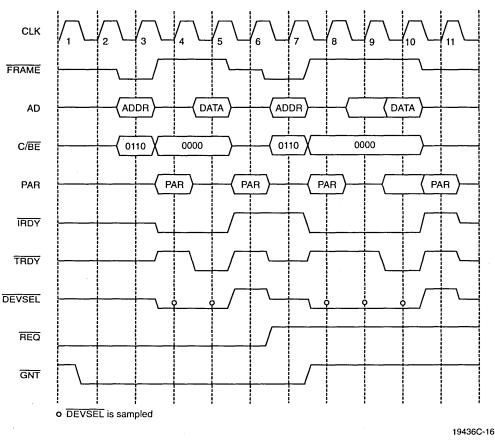
Figure 13. Non-Burst Read Transfer
