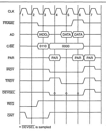
Figure 25. Initialization Block Read In Burst Mode
