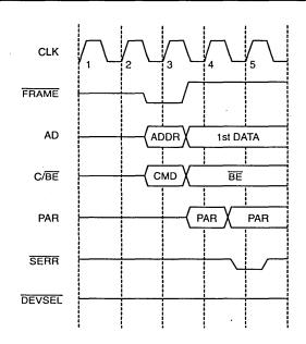
Figure 10. Address Parity Error Response
