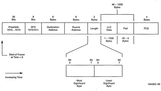
Figure 35. 802.3 Frame And Length Field Transmission Order
