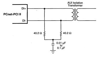
Figure 37. AUI Differential Input Termination
