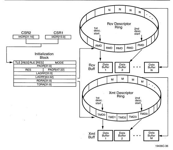
Figure 33. 32-bit Software Model
