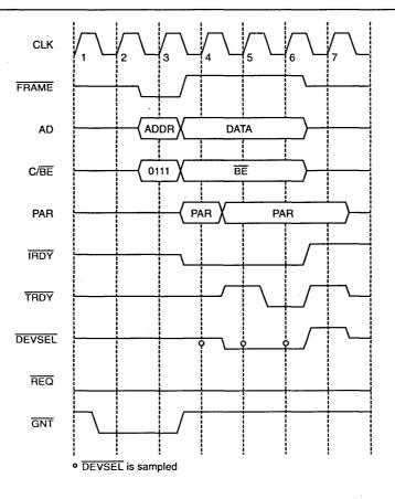
Figure 20. Preemption During Non-Burst Transaction
