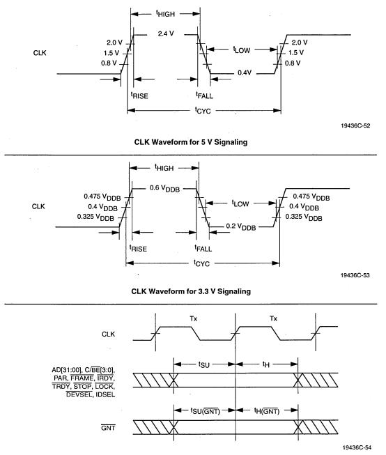
Input Setup and Hold Timing
