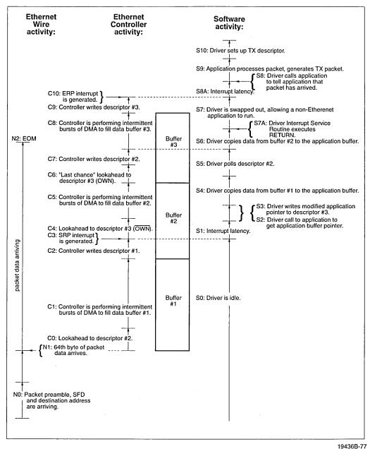
Figure D3. LAPP Timeline for TWO-INTERRUPT Method
