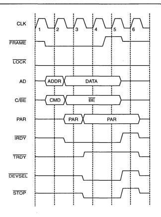
Figure 9. Disconnect Of Slave Cycle When Locked
