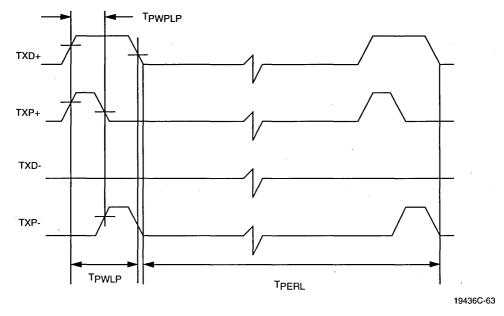
Idle Link Test Pulse
