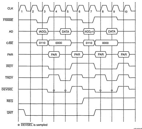
Figure 24. Initialization Block Read In Non-Burst Mode
