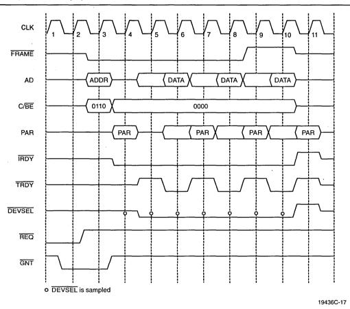
Figure 14. Burst Read Transfer (EXTREQ = 0, MEMCMD = 0)
