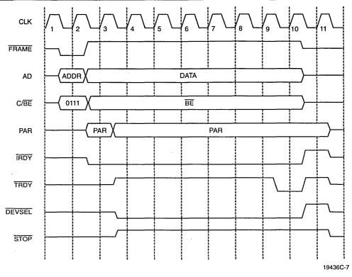
Figure 4. Slave Write Using Memory Command
