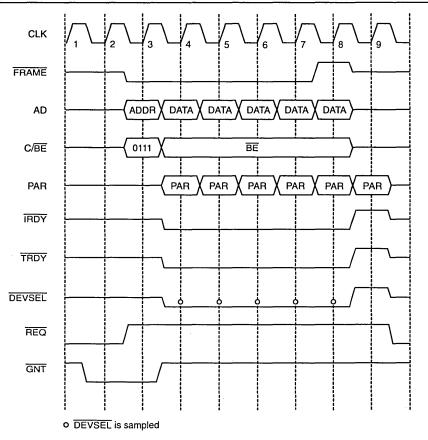
Figure 21. Preemption During Burst Transaction
