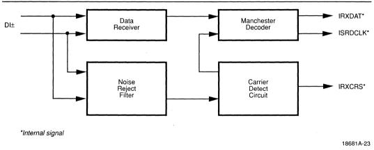
Figure 19. Receiver Block Diagram
