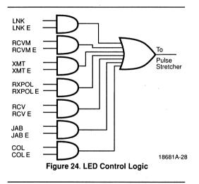
The diagram above shows the LED signal circuit that exists for each LED pin within the Am79C974 controller.
