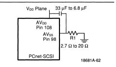
To determine the value for the resistor and capacitor, the formula is:
