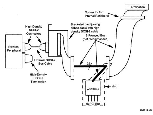
Figure E-2. A Poor Routing Scheme
