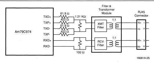
Figure 21. 10BASE-T Interface Connection
