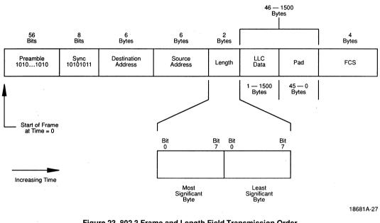
Figure 23. 802.3 Frame and Length Field Transmission Order
