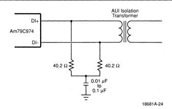
Figure 20. Differential Input Termination
