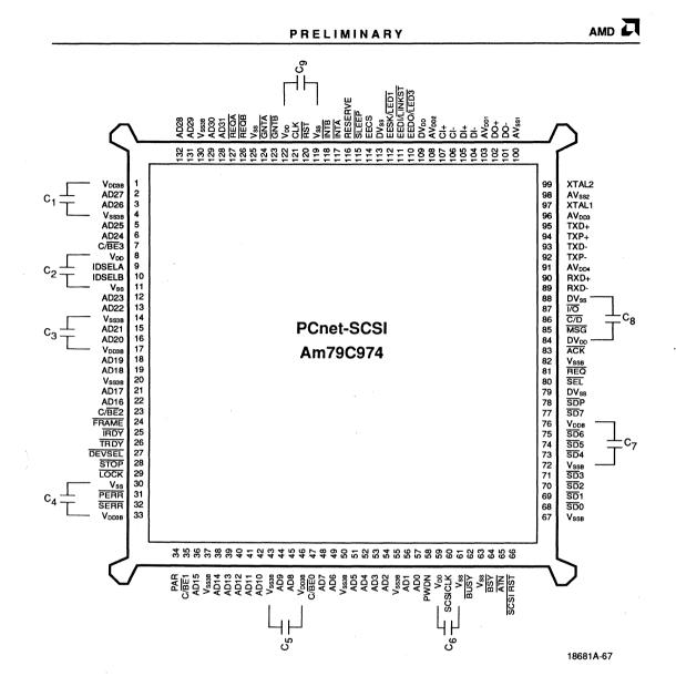
where C1 - C9 are decoupling capacitors.
