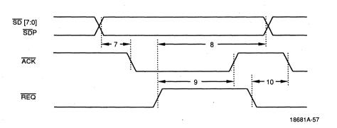
Figure 30. Asynchronous Initiator Transmit
