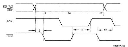
Figure 31. Asynchronous Initiator Receive
