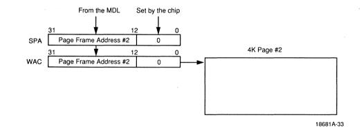
Again when WAC (bits 11:0) reaches the maximum page length count, the Am79C974 resets it to '000h' and increments the WMAC register to the next MDL entry. The operation continues in this way until WMAC register reaches the last MDL entry (Page Frame Address #n in this example).
