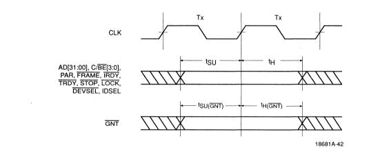
Input Setup and Hold Timing
