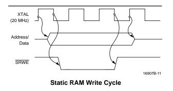
Address and data are valid 20 ns after the rising edge of the first clock period. SRWE goes active 20 ns after the falling edge of the first clock period. SRWE goes inactive 20 ns after the falling edge of the third clock period. Address and data remain valid until the end of the third clock period. Rise and fall times are nominally 5 ns. Non-negative setup and hold times for address and data with respect to SRWE are guaranteed. SRWE has a pulse width of typically 100 ns, minimum 75 ns.
