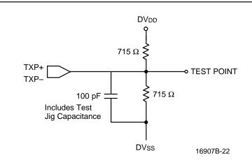
**TXP Outputs Test Circuit**
