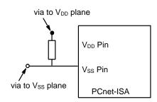
AMD recommends that at least one low-frequency bulk decoupling capacitor be used in the area of the PCnet-ISA controller. 22  $\mu$ F capacitors have worked well for this. In addition, a total of 4 or 5 0.1  $\mu$ F capacitors have proven sufficient around the DV<sub>SS</sub> and DV<sub>DD</sub> pins that supply the drivers of the ISA bus output pins.
