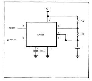
FIGURE 12-15 OSCILLATOR DESIGN USING THE Am555 TIMER
