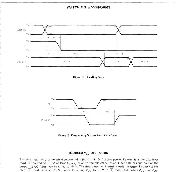
deselection of the chip will not occur until  $t_{OD}$  after  $V_{GG}$  goes back to -9 V.
