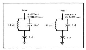
FIGURE 5-4 PARALLEL RESONANT CIRCUITS FOR USE IN Am9080A-1 AND Am9080A-4 MICROCOMPUTERS
