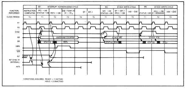
FIGURE 2-17 INTERRUPT TIMING, RESTART INSTRUCTION
