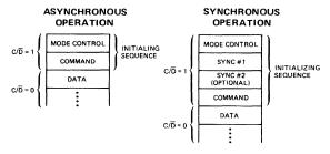
Figure 1. Control Word Sequence for Initialization.
