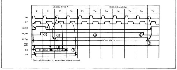
FIGURE 2-13A HOLD TIMING DURING FIVE TIME PERIOD READ OPERATIONS
