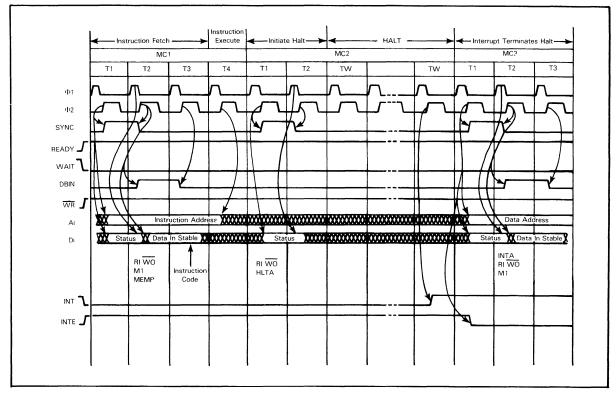
FIGURE 4-19 SIGNAL SEQUENCES AND TIMING FOR INSTRUCTIONS: HLT
