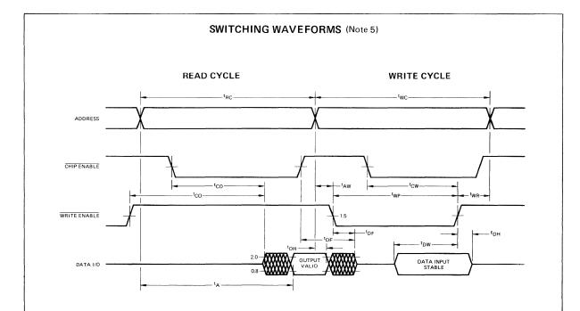
Notes: 1. Output is enabled and  $t_{CO}$  commences only with both  $\overline{CE}$  LOW and  $\overline{WE}$  HIGH.
