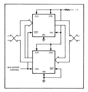
FIGURE 6-5 BIDIRECTIONAL BUS BUFFER
