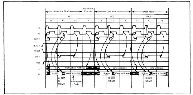
FIGURE 4-11 SIGNAL SEQUENCES AND TIMING FOR INSTRUCTIONS: LXI, JMP, JNZ, JZ, JNC, JC, CPO, JPE, JP, JM
