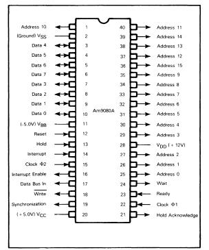
FIGURE 2-2 8080A/9080A CONNECTION DIAGRAM
