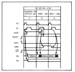
FIGURE 2-7 MEMORY READ MACHINE CYCLE
