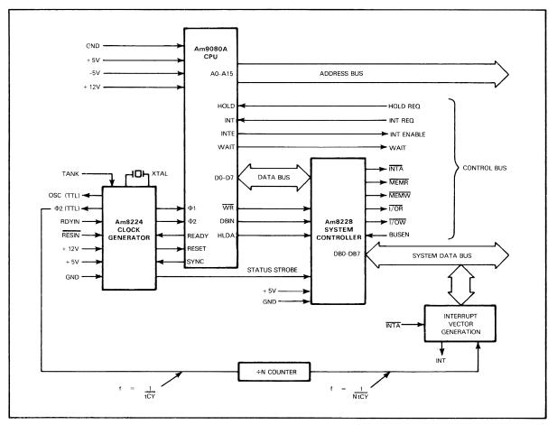
FIGURE 16-3 USE OF AN EXTERNAL COUNTER TO PROVIDE A TIME MARK FOR GENERATING SOFTWARE CONTROLLED DELAY LOOPS
