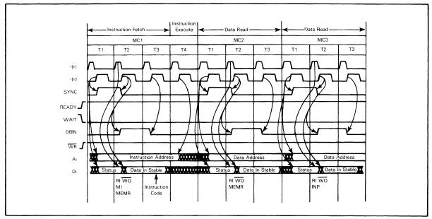
FIGURE 4-17 SIGNAL SEQUENCES AND TIMING FOR INSTRUCTIONS: IN
