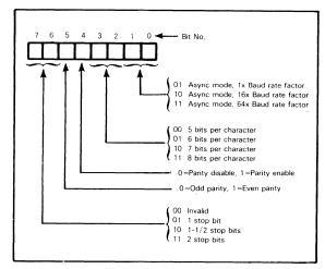
FIGURE 8-5 ASYNCHRONOUS MODE CONTROL CODE
