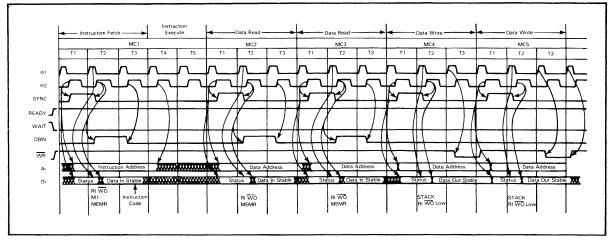
FIGURE 4-15 SIGNAL SEQUENCES AND TIMING FOR INSTRUCTIONS: CALL, CNZ, CA, CNC, CC, CPO, CPE, CP, CM
