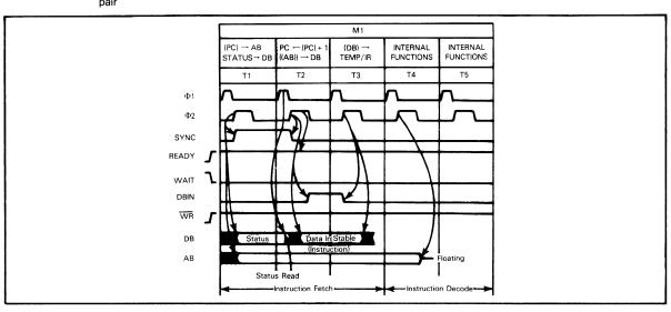
FIGURE 2-6 INSTRUCTION FETCH MACHINE CYCLE
