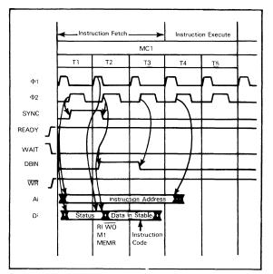
FIGURE 4-2 SIGNAL SEQUENCES AND TIMING FOR INSTRUCTIONS: INR, DCR, MOV REG REG, SPHL, PCH, DCX, INX
