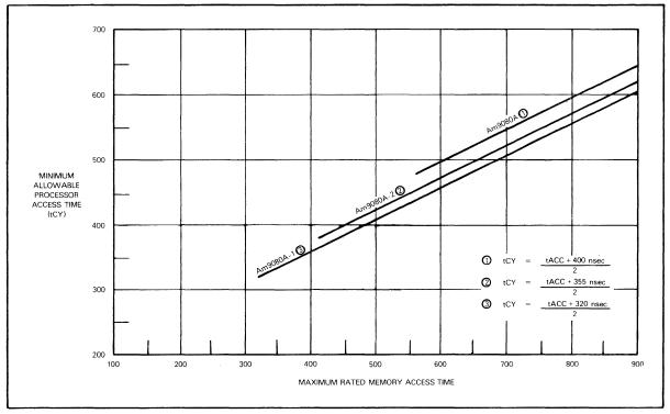
FIGURE 14-4 MINIMUM CYCLE TIMES OF DIFFERENT Am9080A MICROPROCESSORS WITH SMALL MEMORIES
