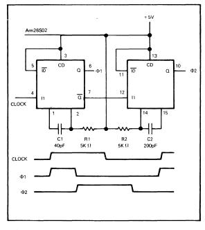
FIGURE 12-9 A MONOSTABLE MULTIVIBRATOR-BASED CLOCK
