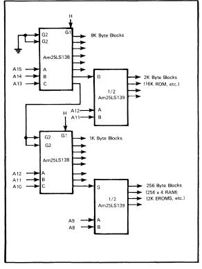
FIGURE 10-4 1-OF-8 AND 1-OF-4 DECODERS IN A DEVICE SELECT NETWORK
