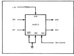
FIGURE 6-4 AN Am8212 CONFIGURED AS A BUS BUFFER
