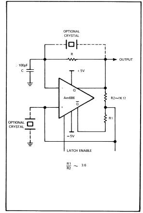
FIGURE 12-12 CLOCK OSCILLATOR USING THE Am686 HIGH SPEED COMPARATOR
