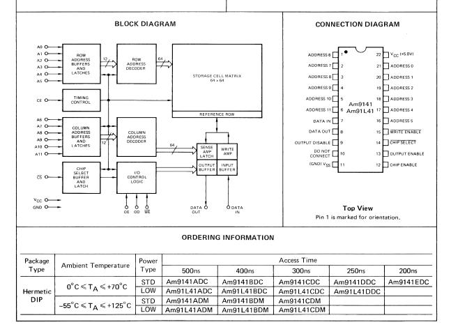
The Am9141 and Am91L41 memories are identical in every respect to their counterparts in the Am9140 and Am91L40 family, with the single exception that the Memory Status output is not functional. Pin 10 on the Am9141/
