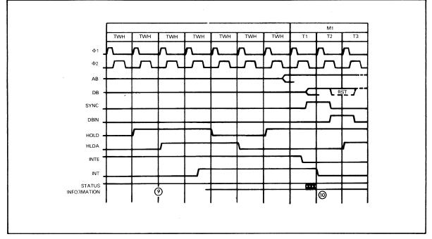
FIGURE 2-20 RELATION BETWEEN HOLD AND INT IN THE HALT STATE
