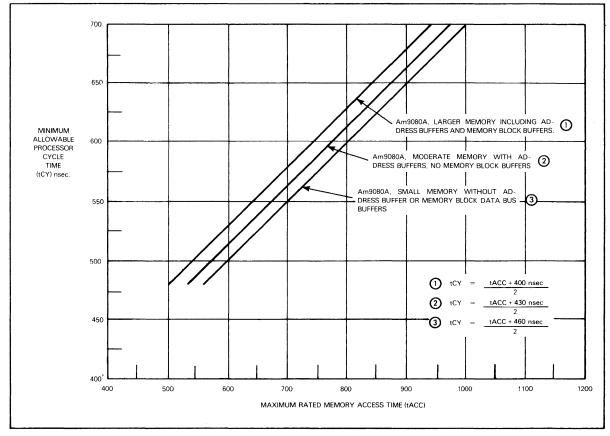
FIGURE 14-3 MINIMUM Am9080A CYCLE TIME VS MEMORY ACCESS TIME FOR THREE MEMORY CONFIGURATIONS
