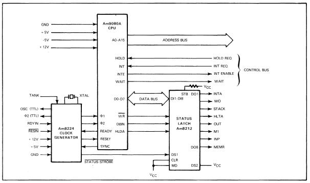
FIGURE 6-9 THE Am8212 USED AS A STATUS LATCH
