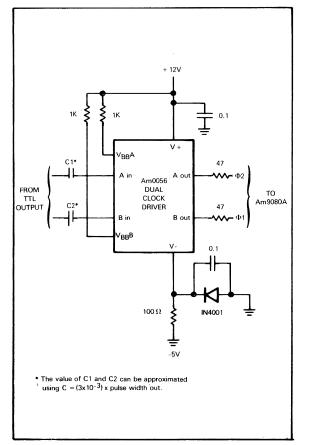
minimal drift and pulse position jitter over an operating range of 1 MHz to 30 MHz. Symmetry of the output waveform is better than 1% at 1 MHz and better than 5% at 25 MHz. Frequency stability is accurate to within 1% of 1 MHz and less than 4% at 25 MHz. These accuracies hold for an operating temperature range between -55°C to + 125°C. When operating the circuit over a restricted temperature range of 0°C to 70°C, the accuracies are improved by a factor of two to one over those stated above.
