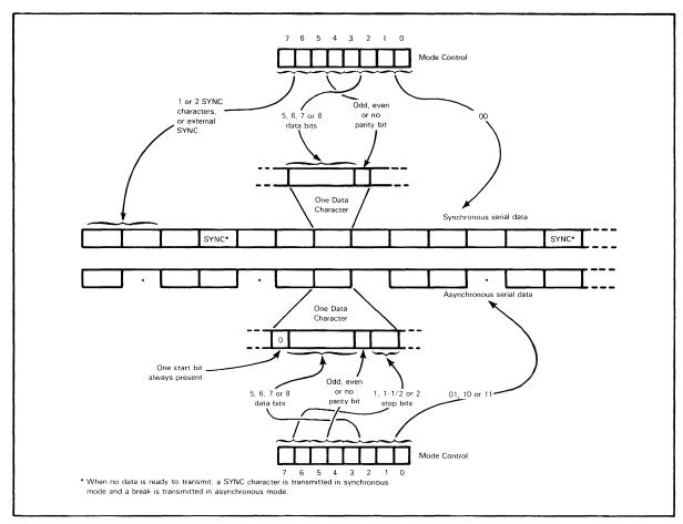
FIGURE 8-6 SYNCHRONOUS AND ASYNCHRONOUS DATA CHARACTERS AS A FUNCTION OF MODE CONTROL
