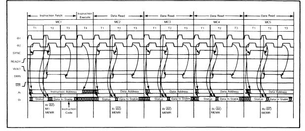
FIGURE 4-6 SIGNAL SEQUENCES AND TIMING FOR INSTRUCTIONS: LHLD
