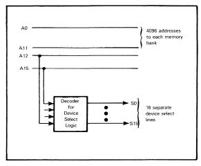
FIGURE 10-2 ADDRESS BUS LINES AND DEVICE SELECT LOGIC
