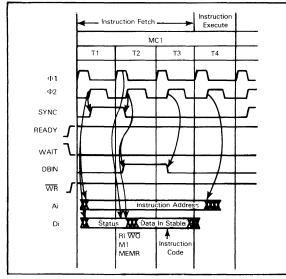
FIGURE 4-1 SIGNAL SEQUENCES AND TIMING FOR INSTRUCTIONS: STC, CMC, CMA, NOP, RLC, RRC, RAL, RAR, XCHG, EI, DI, DAA, ADD R, ADC R, SUB R, SBB R, ANA R, XRA R, ORA R, CMP R
