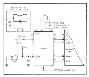
Figure 2. Typical Application with Am8224 and Am9080A.
