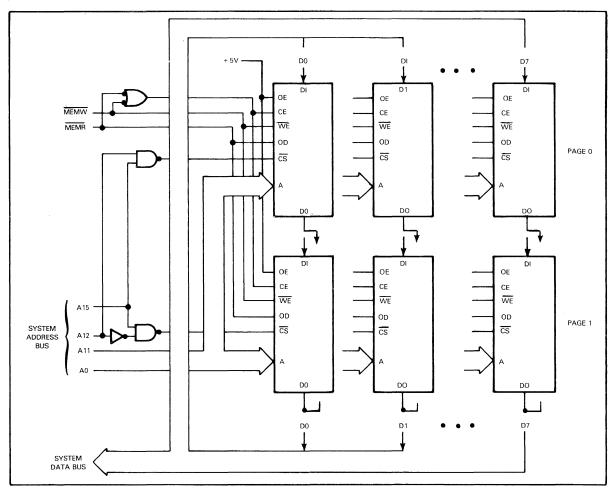
FIGURE 13-6A AN 8K x 8-BIT STATIC RAM USING Am9140 MEMORY DEVICES
