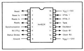
FIGURE 5-2 Am8224 CONNECTION DIAGRAM
