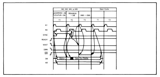
Figure 2-8 MEMORY WRITE MACHINE CYCLE
