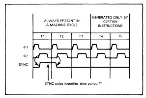
FIGURE 2-4 MACHINE CYCLE TIMING
