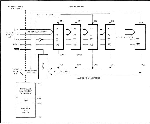
. FIGURE 13-3 A 1K BYTE STATIC RAM USING Am9102 1K x 1-BIT MEMORY DEVICES
