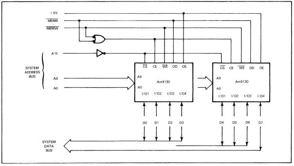
FIGURE 13-5 A 1K X 8-BIT STATIC RAM USING Am9130 MEMORY DEVICES
