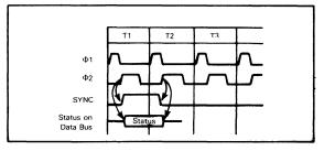
FIGURE 2-5 STATUS OUTPUT DURING T1 OF EVERY MACHINE CYCLE
