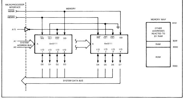
FIGURE 13-2 Am9111 DEVICES USED TO CREATE A 256 x 8-BIT STATIC RAM MEMORY
