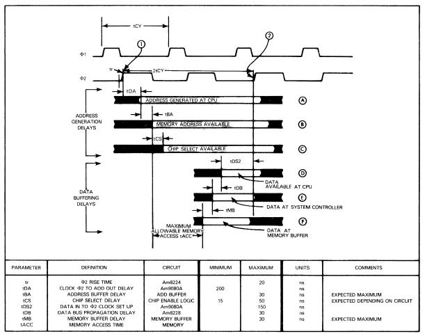
FIGURE 14-2 READ CYCLE TIMING FOR NON-CLOCKED MEMORIES
