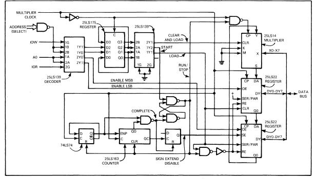
FIGURE 17-4 8-BIT X 8-BIT MULTIPLICATION USING THE Am25LS14 DEVICES
