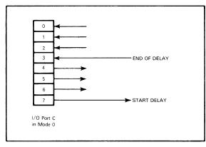
FIGURE 16-1 USING AN Am9555 PPI IN MODE 0 TO CONTROL A TIME DELAY
