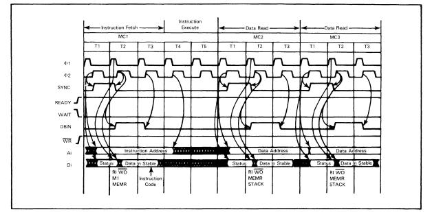
FIGURE 4-16 SIGNAL SEQUENCES AND TIMING FOR INSTRUCTIONS: RNZ, RZ, RNC, RPO, RPE, RP, RM
