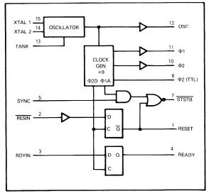
FIGURE 5-1 Am8224 BLOCK DIAGRAM
