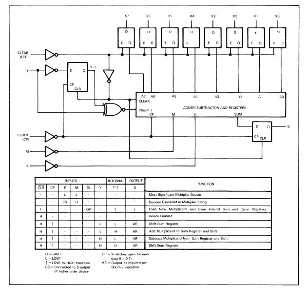
the low order bit of the partial product second line added to the retained lowest order bit of the first partial product line. In this fashion, multiplier bits may be applied at the Y inputs, one at a time, beginning with the low order bit; as each multiplier bit is applied an additional product bit is generated for output at the S pin.
