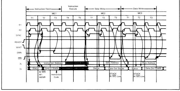
FIGURE 4-7 SIGNAL SEQUENCES AND TIMING FOR INSTRUCTIONS: PUSH, RST
