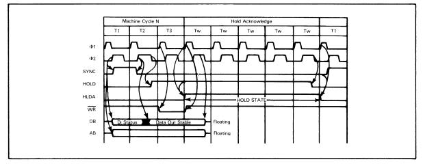
FIGURE 2-14B HOLD TIMING FOR ANY NON-READ OPERATION COMPLETED PRIOR TO ONSET OF HOLD STATE
