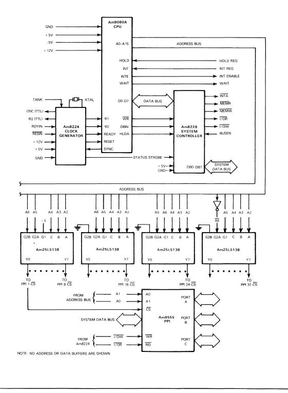
FIGURE 7-4 AM9080A MICROCOMPUTER I/O SYSTEM WITH ADDRESS DECODING FOR 32 I/O PORTS
