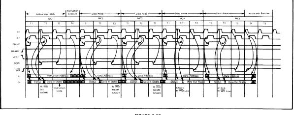
FIGURE 4-10 SIGNAL SEQUENCES AND TIMING FOR INSTRUCTIONS: XTHL
