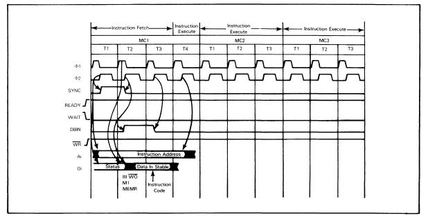
FIGURE 4-9 SIGNAL SEQUENCES AND TIMING FOR INSTRUCTIONS: DAD
