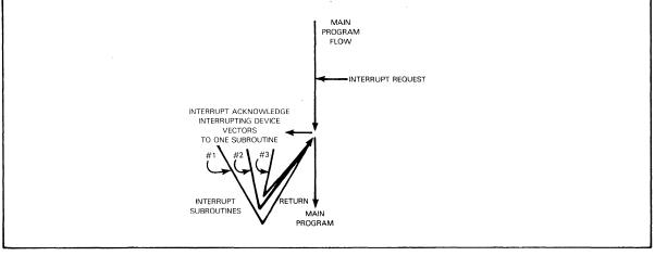
FIGURE 15-4 PROGRAM FLOW WITH SEVERAL INTERRUPTING DEVICES
