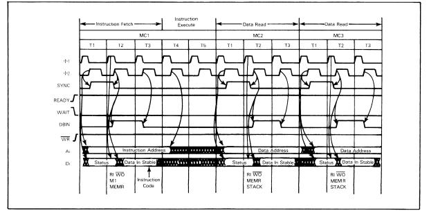
FIGURE 4-8 SIGNAL SEQUENCES AND TIMING FOR INSTRUCTIONS: POP, RET
