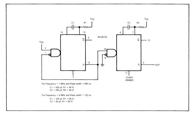
FIGURE 12-13 OSCILLATOR DESIGN USING A DUAL MONOSTABLE MULTIVIBRATOR Am26123
