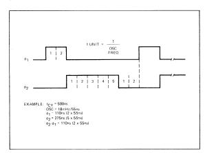
Figure 1. Clock Generator Waveforms.
