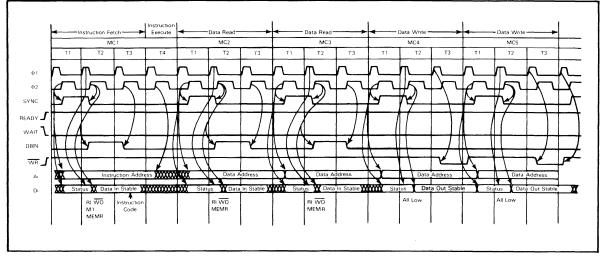
FIGURE 4-14 SIGNAL SEQUENCES AND TIMING FOR INSTRUCTIONS: SHLD
