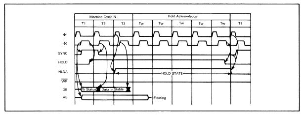
FIGURE 2-14A HOLD TIMING FOR READ IN A THREE TIME PERIOD READ MACHINE CYCLE
