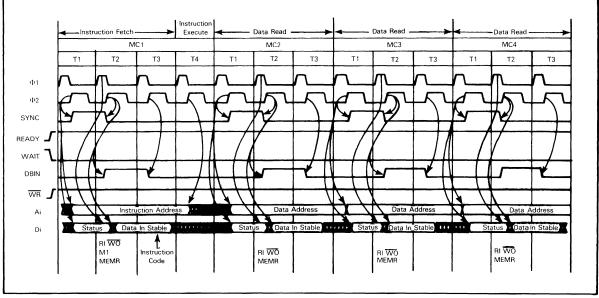
FIGURE 4-13 SIGNAL SEQUENCES AND TIMING FOR INSTRUCTIONS: LDA
