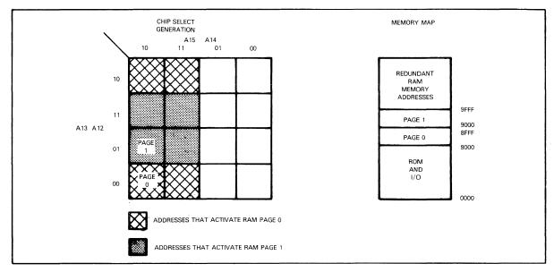
FIGURE 13-6B ADDRESS ASSIGNMENTS FOR THE MEMORY OF FIGURE 13-6A
