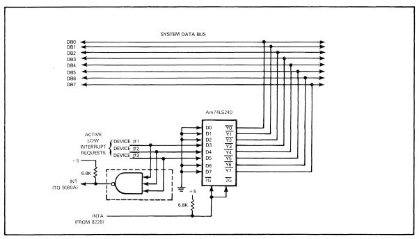
FIGURE 15-5 Am9080A MICROCOMPUTER WITH THREE INTERRUPTS
