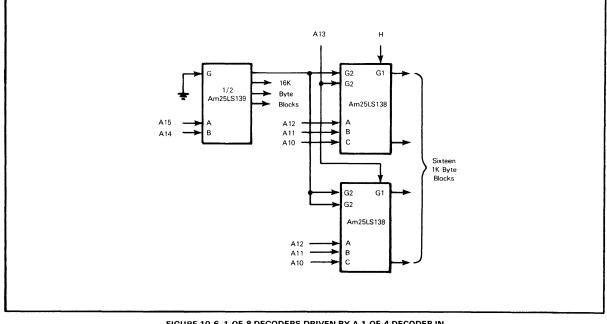
FIGURE 10-6 1-OF-8 DECODERS DRIVEN BY A 1-OF-4 DECODER IN A DEVICE SELECT NETWORK
