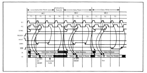
FIGURE 4-18 SIGNAL SEQUENCES AND TIMING FOR INSTRUCTIONS: OUT
