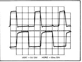
FIGURE 12-5 WAVEFORMS GENERATED BY CIRCUIT OF FIGURE 12-4
