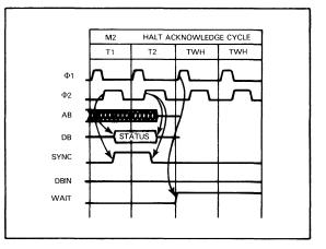
FIGURE 2-9 HALT ACKNOWLEDGE MACHINE CYCLE
