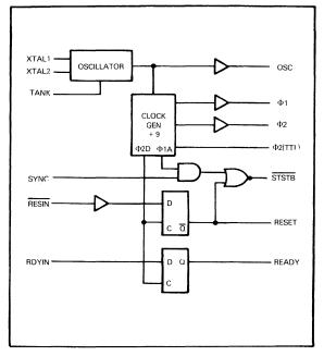
FIGURE 12-2 Am8224 CLOCK GENERATOR BLOCK DIAGRAM
