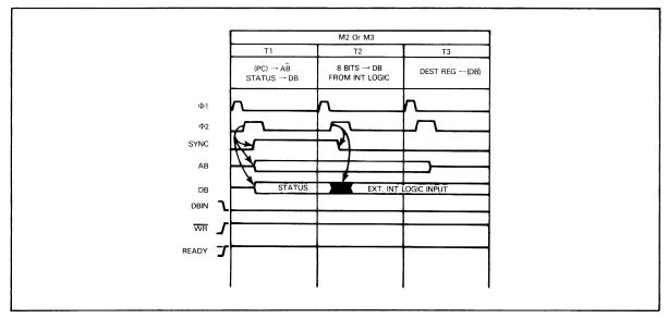
FIGURE 2-10 NULL MACHINE CYCLE TIMING
