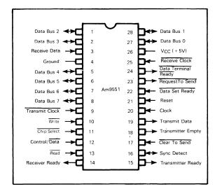
FIGURE 8-2 Am9551 CONNECTION DIAGRAM
