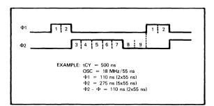
The clock waveforms are buffered to provide the high level clock signals required by the 8080A/9080A CPU. A separate TTL compatible  $\Phi 2$  is provided to be used by other microcomputer components.
