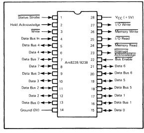
FIGURE 5-7 Am8228/8238 CONNECTION DIAGRAM
