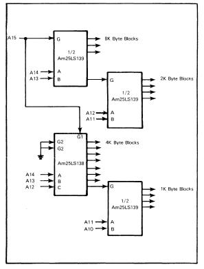
FIGURE 10-5 ANOTHER MIXED 1-OF-8 AND 1-OF-4 DECODER NETWORK FOR DEVICE SELECT LOGIC
