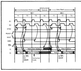
FIGURE 4-4 SIGNAL SEQUENCES AND TIMING FOR INSTRUCTIONS: LDAX, MOV REG M, ADI, ACI, SUI, SI, ANI, XRI, ORI, CPI, MVI R, ADD M, ADC M, SUB M, SBB M, ANA M, XRA M, ORA M, CMP M
