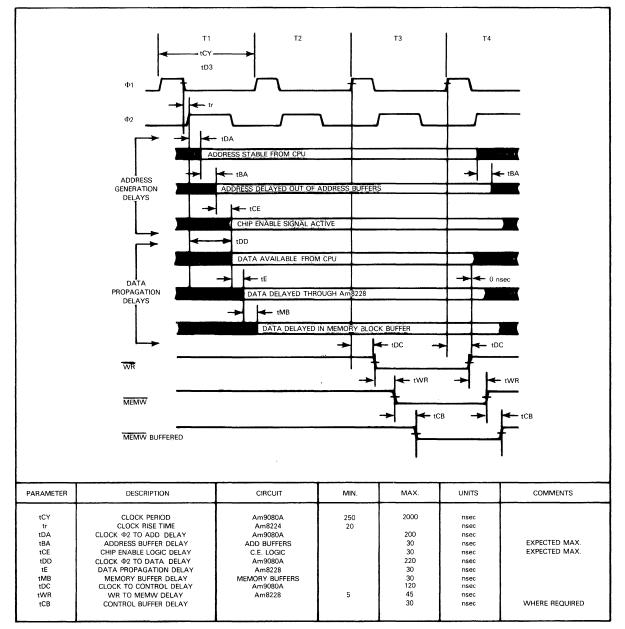
FIGURE 14-8 MEMORY WRITE CYCLE TIMING
