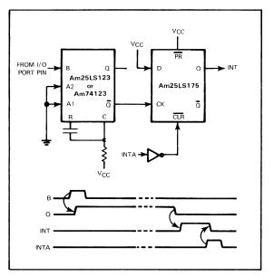
FIGURE 16-2 USING A MONOSTABLE MULTIVIBRATOR TO GENERATE A TIME DELAY
