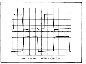
FIGURE 12-10 WAVEFORMS GENERATED BY CIRCUIT OF FIGURE 12-9
