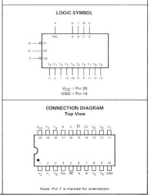
One-of-Eight Decoder With Three-State Outputs And Polarity Control
