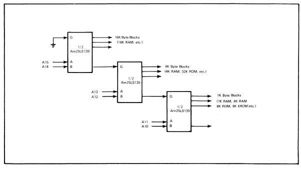
FIGURE 10-3 Am25LS139 DEVICE SELECT NETWORK
