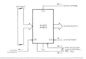
$(\overline{DS}_1 \text{ input})$  then the status data will be latched into the Am3212 • Am8212. The mode signal is tied high so that the output on the latch is active and evabled all the time.
