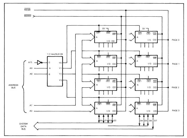
FIGURE 13-4A 1K x 8 RAM MEMORY CONSTRUCTED WITH Am9111 MEMORIES
