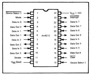
FIGURE 6-2 Am8212 CONNECTION DIAGRAM
