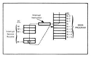
FIGURE 2-16 INTERRUPT PROGRAM FLOW
