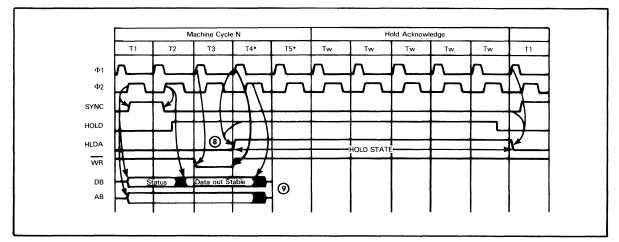
FIGURE 2-13B HOLD TIME PERIOD DURING FIVE TIME PERIOD WRITE OPERATIONS
