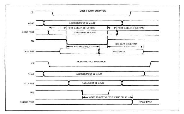
FIGURE 7-6 MODE 0 INPUT AND OUTPUT TIMING
