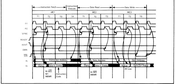
FIGURE 4-3 SIGNAL SEQUENCES AND TIMING FOR INSTRUCTIONS: DCR M, INR M, MVI M
