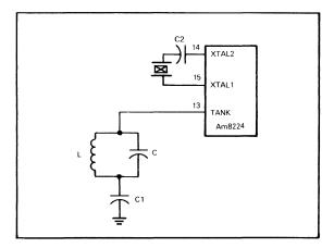
FIGURE 5-3 SCHEMATIC OF PARALLEL RESONANT CIRCUIT
