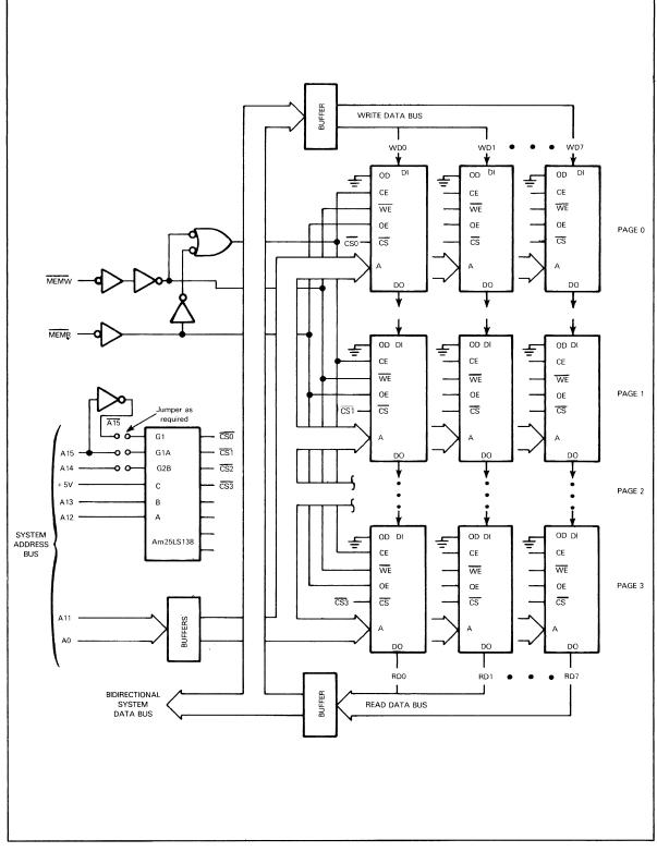
FIGURE 13-7A A 16K x 8-BIT MEMORY USING Am9140 MEMORY DEVICES
