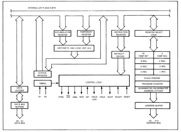
FIGURE 2-1 Am9080A FUNCTIONAL BLOCK DIAGRAM
