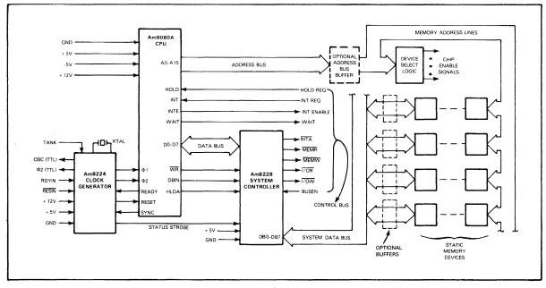
FIGURE 13-1 AN Am9080A STATIC MEMORY GENERAL CONFIGURATION
