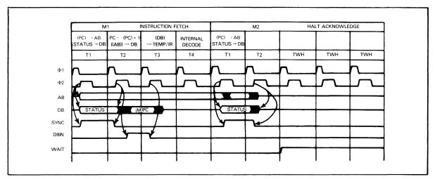
FIGURE 2-15 HALT TIMING
