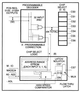
desired chip select active range. Effectively, any input bit may be compared for zero, one or don't care in determining an address match. Thus, the need for two bits per input (26 inputs x = 52 bits) to encode these possibilities.
