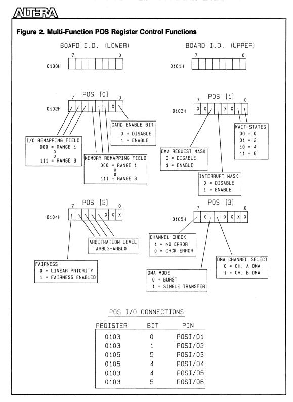
select decode block. In this way the PS/2 can control address response ranges for the card and associated memory / I/O resources as it configures the system. This is used to eliminate address conflicts between cards without mechanical setting of DIP switches or jumpers, an error-prone process. The use of such mechanical arrangements in fact violates the Micro Channel specification.
