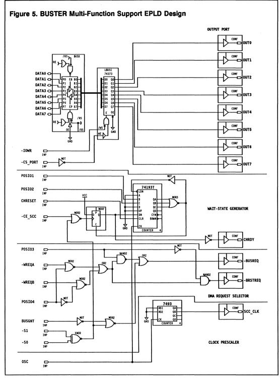
the two -W/REQx outputs of the SCC as inputs, and generates either a -BRSTREQ or -BUSREQ line for the EPB2002. The DMA request mode is controlled by a POS register bit as outlined earlier. A POS register bit selects which channel is the DMA requestor. DMA requests can also be permanently disabled by another POS bit for interrupt-driven mode on both channels. Interrupt-driven operation may be used on one channel while DMA operation is employed on the other.
