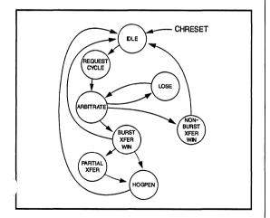
The basic arbitration process is straightforward. When ARB/-GNT goes high, all adapters wishing control of the bus place their arbitration levels on the ARB0-3 lines. (All adapter outputs are wire-ORed together). If a value lower that the arbitration level of a given adapter is detected on the ARB0-3 lines by that adapter, it
