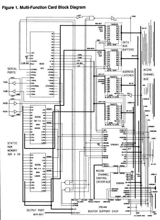
on the MC Bus. This clock divider is implemented in a small portion of an EPB1400. The OSC line provides a precision clock input of frequency 14.31818 Megahertz. The clock divider generates a 3.58 MegaHertz output for the SCC. As a result, a local oscillator is not needed for the SCC.
