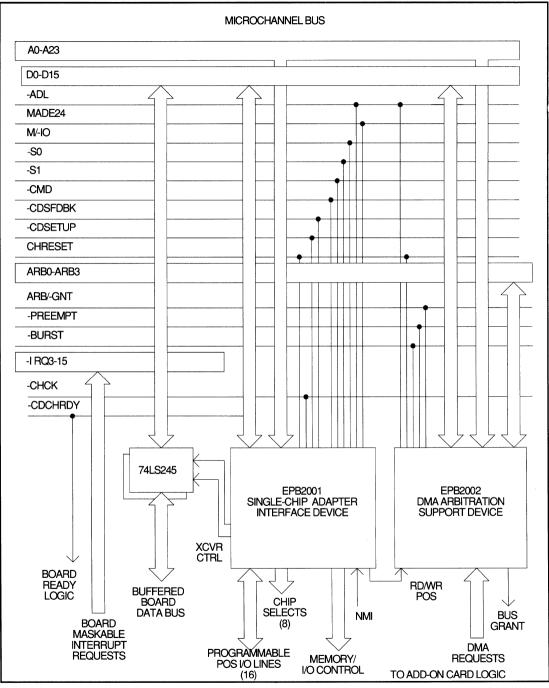
Figure 1. MICRO CHANNEL INTERFACE CONNECTION
