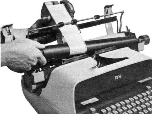
Fig. 9—Placing 1B Cartridge in Typewriter
