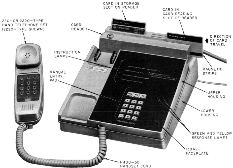
Fig. 1—5000AM Transaction I Telephone Set Base Equipped With 220- or 2220-Type Hand Telephone Set
