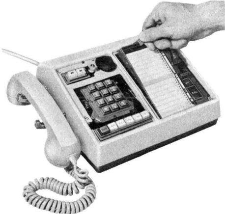
Fig. 8—Removal of 1B Cartridge
