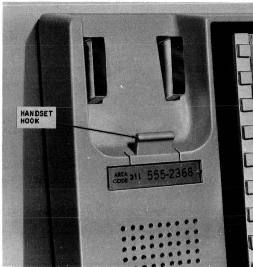
Fig. 9—960A01M Telephone Set With Handset Hook Reversed for Wall Mounting
