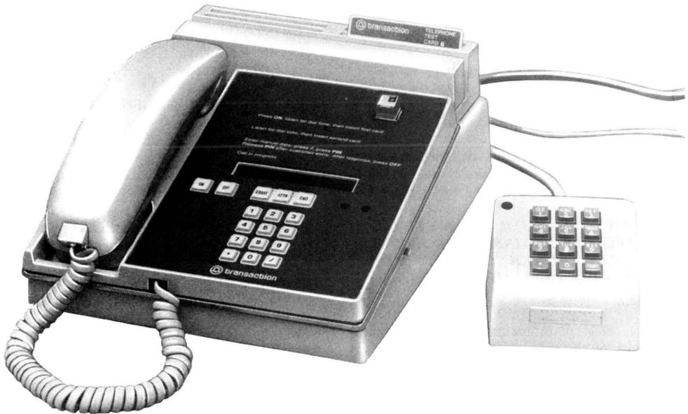
Fig. 9—Transaction II Telephone Set With 5000A Dial Installed
