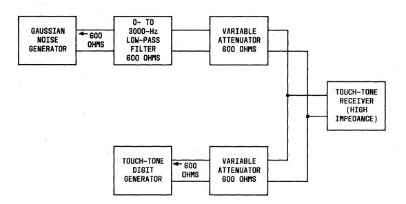
Fig. 45—Gaussian Noise Test of TOUCH-TONE Receiver
