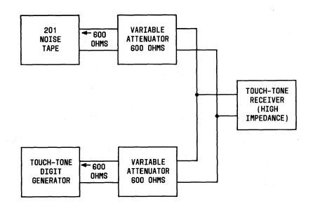
Fig. 47—Impulse Noise Test TOUCH-TONE Receiver
