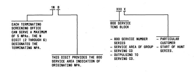
Fig. 3—800 Service Address—Terminating Screening Office
