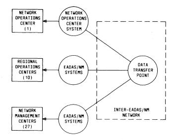
Fig. 3—Network Management Data Transfer Arrangement
