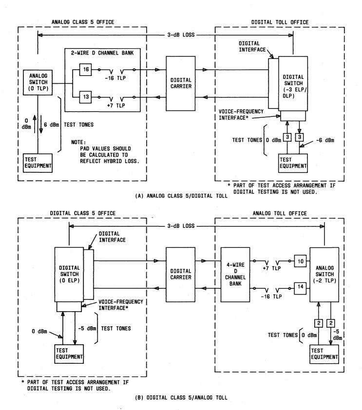
Fig. 12—Provision of Combination Toll Connecting Trunks
