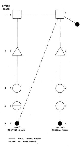
P, Q', or Q are therefore permissible. Trunk groups to R, S, or T can be justified only by the switching function 4 loads at those switching systems, ie, for the end offices homed directly on R, S, or T.
