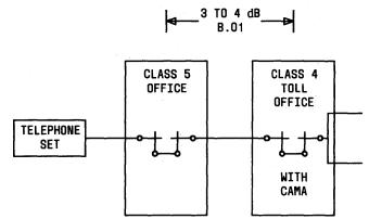
Fig. 5—Current Standard CAMA Arrangement
