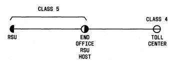
Fig. 1—Standard RSU/Host Office Classification and Homing Arrangements
