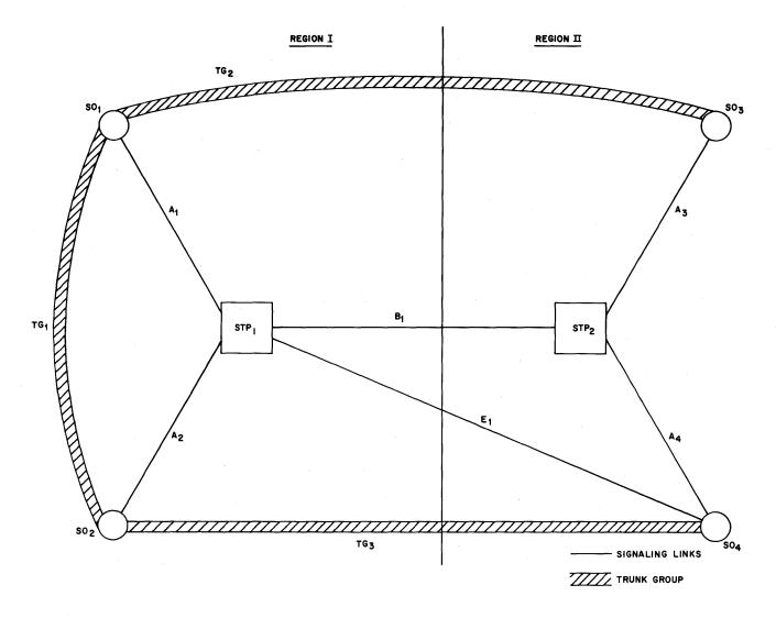
Fig. 2—Basic (Nonredundant) Signaling Network Structure
