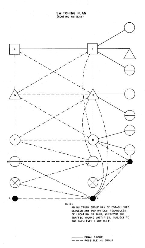
Fig. 1—Standard Routing Plan High-Usage Trunking Patterns
