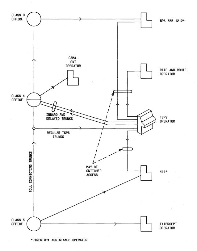
Fig. 1—Typical Topology of Operator Systems
