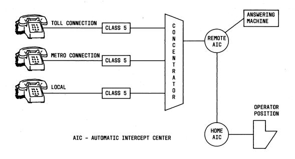
Fig. 19—Typical Automatic Intercept System
