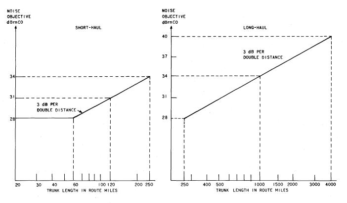
MEAN CARRIER PERFORMANCE OBJECTIVE FOR MESSAGE-CIRCUIT NOISE (STANDARD DEVIATION AT ANY TRUNK LENGTH = 4 dB)
