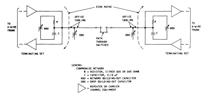
Fig. 22—Switching of 4-Wire Trunks at a 2-Wire Switching Office
