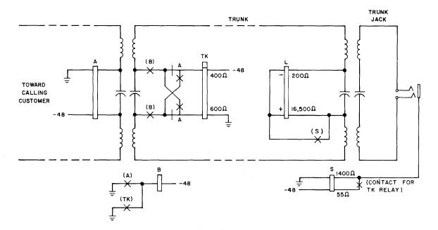
Fig. 11—Reverse Battery, High-Low Signaling
