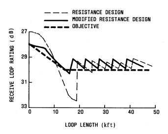
Fig. 21—Receiving Loop Rating
