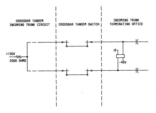
Fig. 41—Incoming Trunk Circuit Without Balanced Windings on Supervisory Relay
