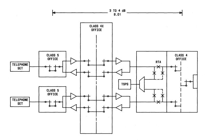
Fig. 8—Class 4X Office TSPS/RTA Arrangement
