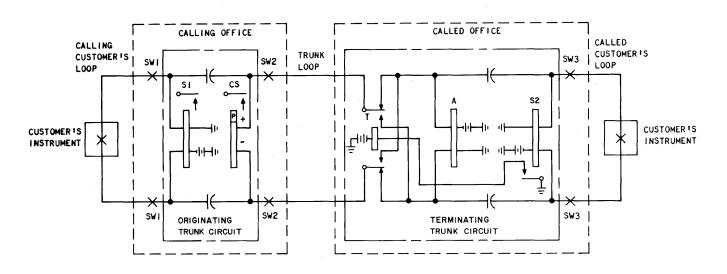
Fig. 6—Reverse Battery Signaling
