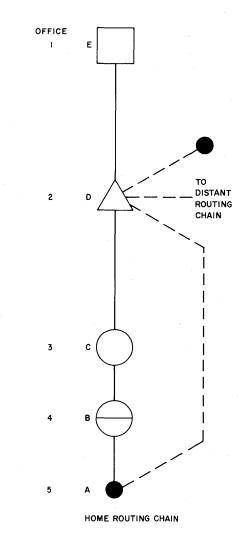
Fig. 3—Application of One-Level Limit Rule to Establish a Trunk Group Between an End Office and a Distant Regional Center
