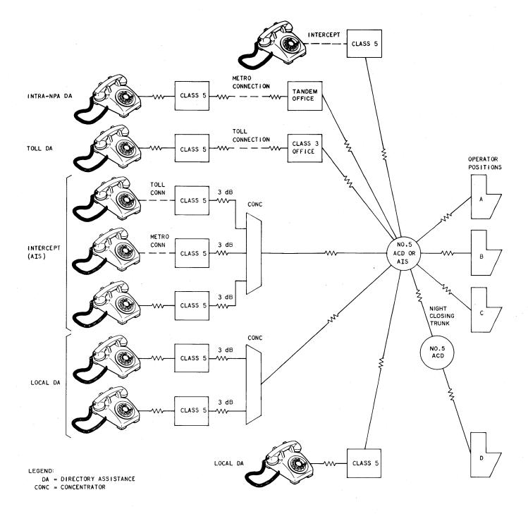
Fig. 18—Loss Plan for No. 5 Automatic Call Distribution
