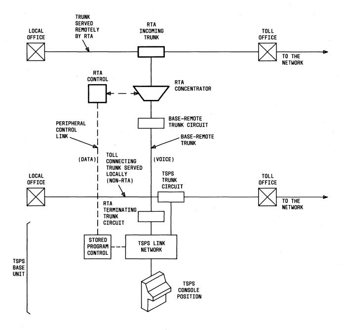
Fig. 4—Remote Trunk Arrangement
