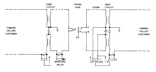
Fig. 9—High-Low Signaling
