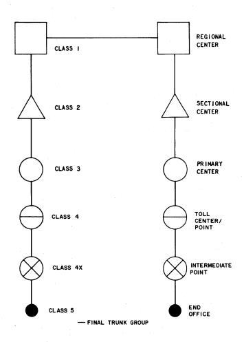
Fig. 1—Switching System Classification and Homing Arrangements
