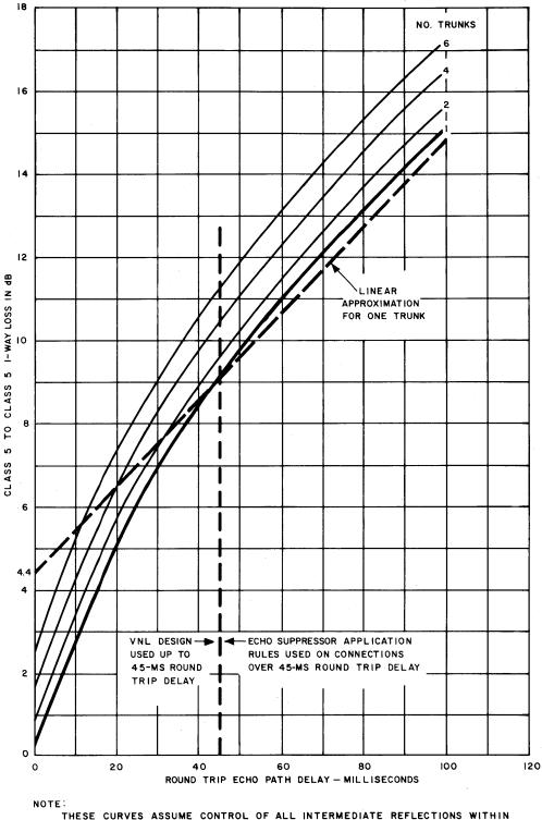
THESE CURVES ASSUME CONTROL OF ALL INTERMEDIATE REFLECTIONS WITHIN THE CONNECTION (THROUGH 4-WIRE CIRCUITS AND 4-WIRE SWITCHING OR THEIR EQUIVALENTS IN 2-WIRE TOLL OFFICES MEETING THROUGH AND TERMINAL BALANCE OBJECTIVES FOR VNL OPERATION).
