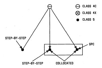
Fig. 9—Current Standard Arrangement for Terminating Traffic
