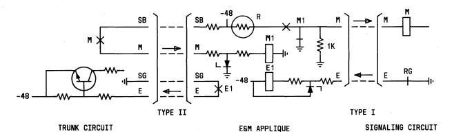
Fig. 21—Type II to Type I Conversion
