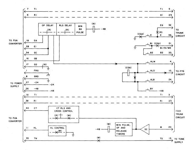
Fig. 34—FBB Signaling Auxiliary Module
