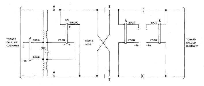
Fig. 10—High-Low, Reverse Battery Signaling
