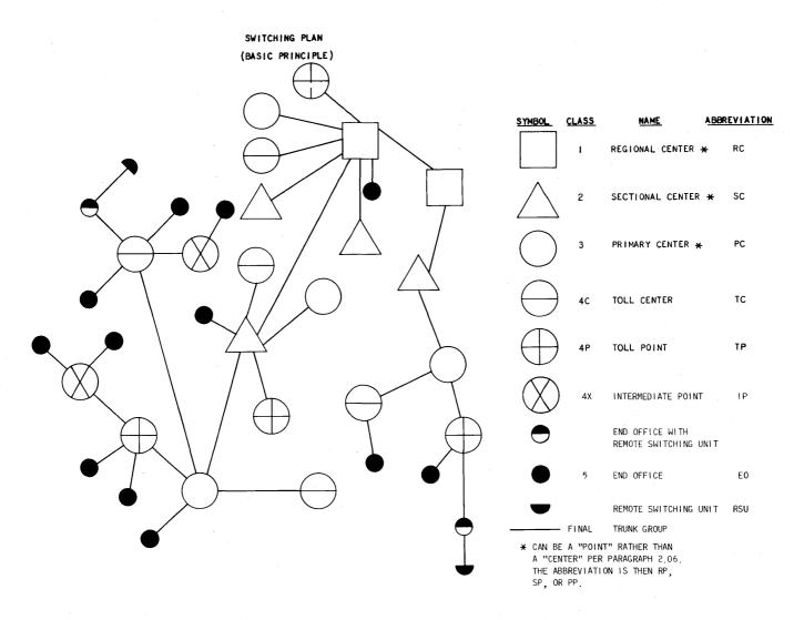
Fig. 2—Typical Switching System Groupings
