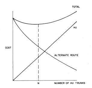
Fig. 2—Relationships Involved in Alternate Routing Arrangement
