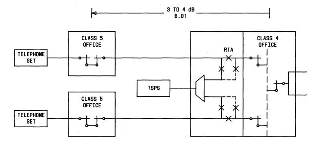
Fig. 7—Current Standard TSPS/RTA Arrangement
