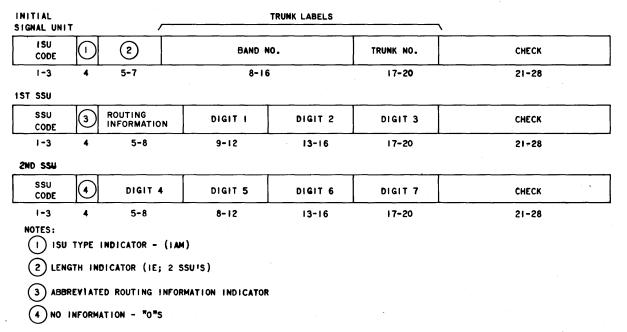
FIG. 5(8) - INITIAL ADDRESS MESSAGE (WITH ABBREVIATED ROUTING INFORMATION)
