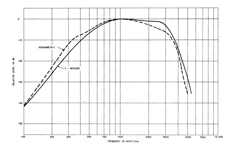
Fig. 24—Comparison Between Psophometric and C-Message Weighting
