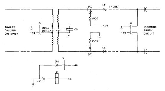
Fig. 8—Battery and Ground Pulsing with Loop Supervision
