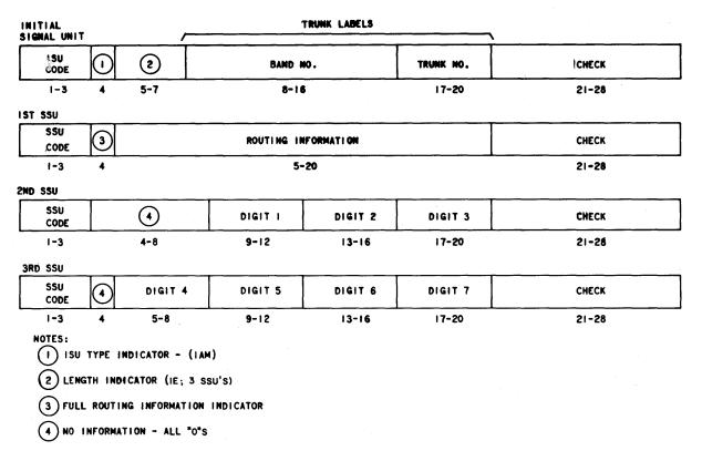
FIG. 5(A) - INITIAL ADDRESS MESSAGE (WITH EXPANDED ROUTING INFORMATION )
