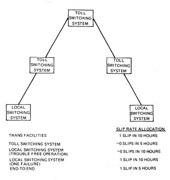
THIS ALLOCATION ALLOWS MARGIN FOR SYNCHRONIZATION LINKS TO FAIL WITHOUT VIOLATING END-TO-END OBJECTIVE
