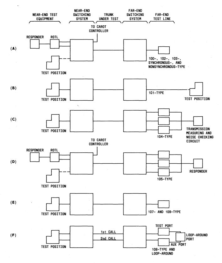
Fig. 1—Test Line Arrangements for Interoffice Trunk Testing
