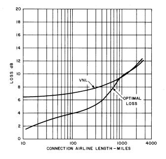
Fig. 7—Optimal Loss Compared With VNL
