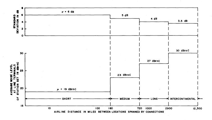
Fig. 25-Noise Objectives for Customer-to-Customer Connections
