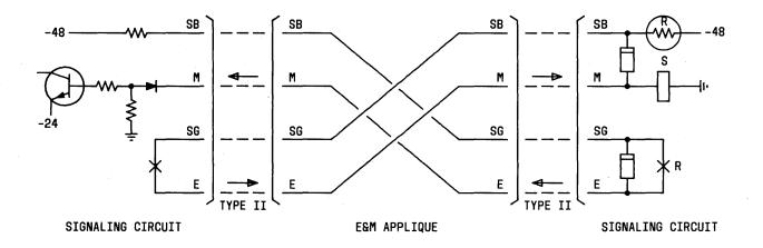
Fig. 26—Signaling Circuits Back to Back—Type II
