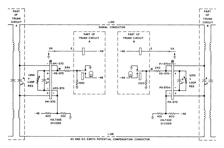
Fig. 30—DX Signaling Circuit
