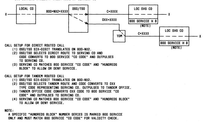
Fig. 4—800 Service Routing—Intrastate—NX2 per Local Serving Central Office
