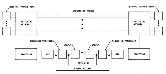
FIG. I(B) - FUNCTIONAL BLOCK DIAGRAM - CCIS SYSTEM
