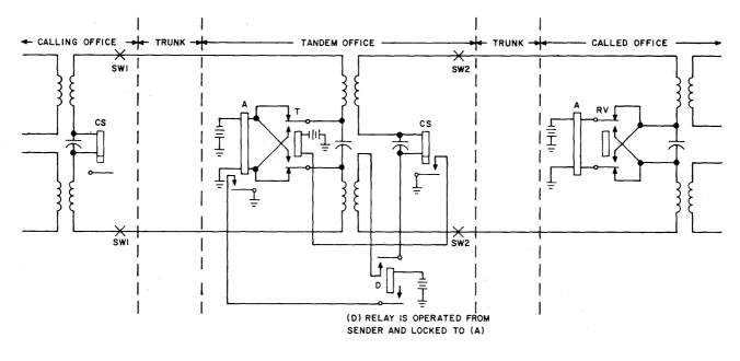
Fig. 7—Repeated Reverse Battery Signaling
