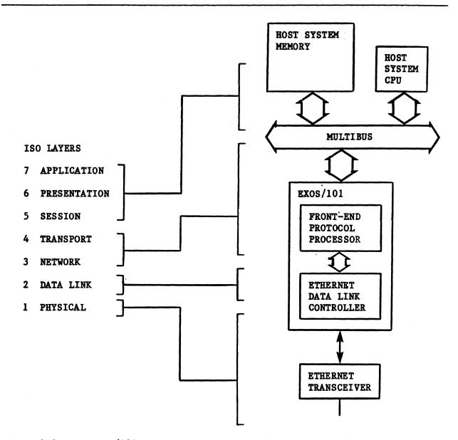
Figure 1-1: An EXOS/101 Front-End Processor Mode Implementation
