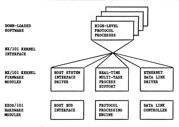
Figure 1-3: NX/101 Software Architecture
