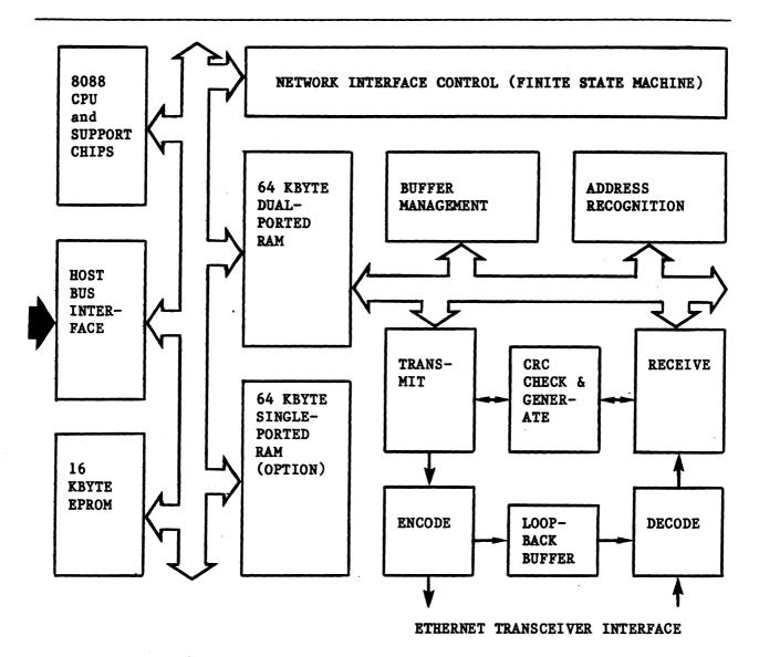
Figure 1-2: EXOS/101 Block Diagram
